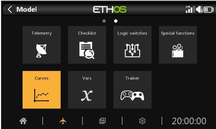
Curves may be used to modify the control response in the Mixes or Outputs. While the standard Expo curve is available directly in those sections, this section is used to define any custom curves that may be required. The 'Add curve' function may also be reached from the Mixes and Outputs edit screens directly.
