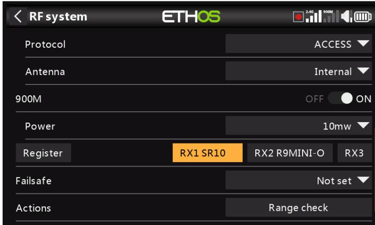
With an SR10 Pro registered and bound, go to RF System and tap on the 'SR10' button.
