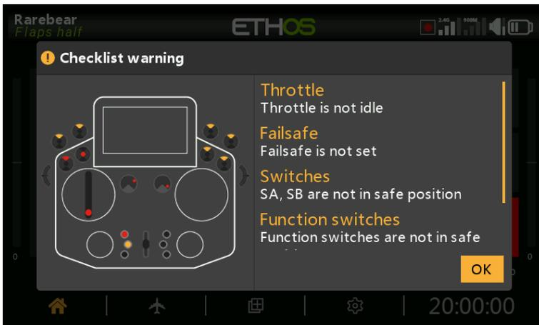
The default checks include radio is in silent mode, failsafe not set, switches and pots check, radio low battery, RTC battery low, etc. The switches check shows the direction the switch should be moved, please refer to the red dots in the warning screen example above.
