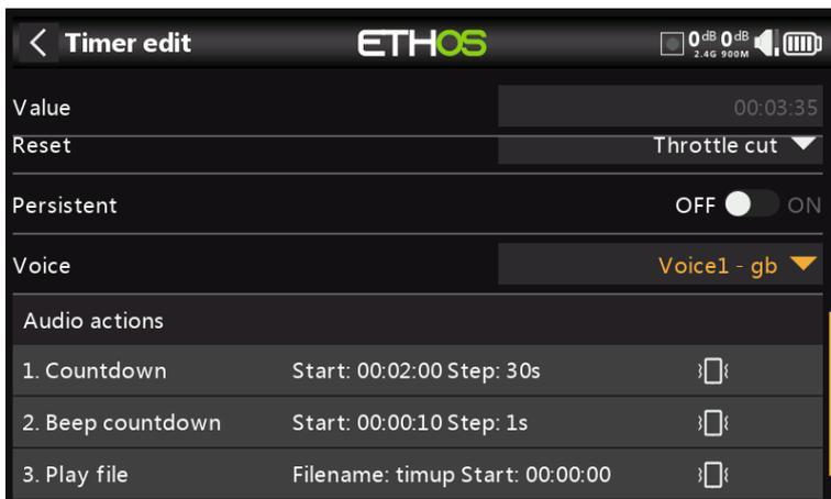
The timer will be reset by the System Event 'Throttle cut'. It is not persistent, so it will also be reset at power on.
