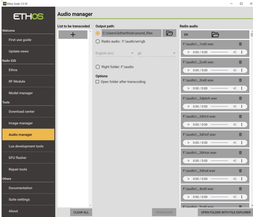
Click on the '+' button in the 'List to be transcoded' window to browse and select the audio files to be converted. This process can be repeated to add audio files to the list.
