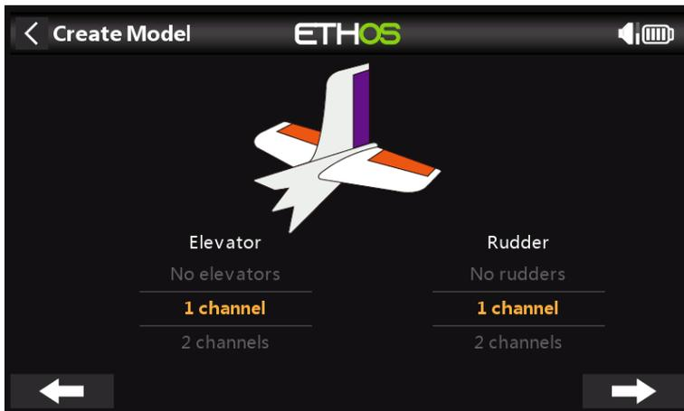
Accept the default 1 channel for Elevator and 1 channel for Rudder.
