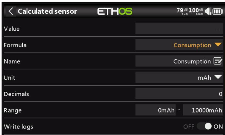
The Consumption calculated sensor allows the energy consumed by your motor to be calculated from a current sensor such as the FAS series.
