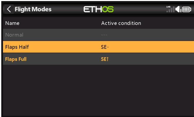
For our example we have configured the default flight mode as Normal, and added two additional flight modes named Flaps Half (switch SE-mid) and Flaps Full (switch SE-Up).
