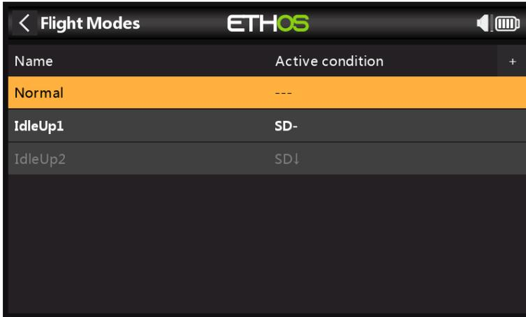
We will use flight modes to configure the three flight modes needed for Normal, Idle Up 1 and Idle Up 2. For our example we have renamed the 'Default flight mode' to 'Normal', and added two additional flight modes for Idle Up 1 and 2 on switch SD.
