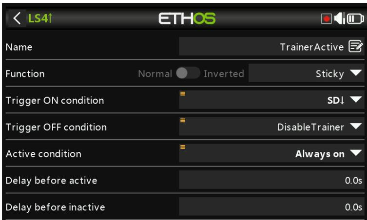
Configure a Sticky logic switch so that it is set by trainer switch SD down, and reset when stick movement is detected or the trainer switch is not in the down position.
