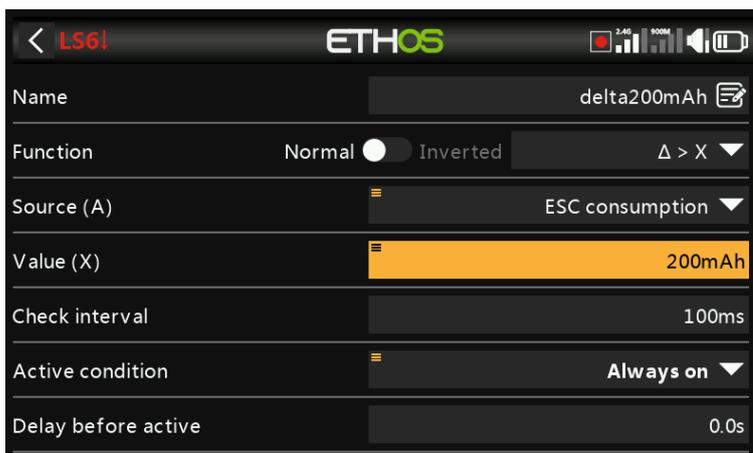
The condition is True if the change in value 'd' (i.e. delta) of the selected source 'A' is greater than or equal to the user defined value 'X', within the 'Check interval'. If the 'Check interval' is set to '---', then the check interval becomes infinite.
