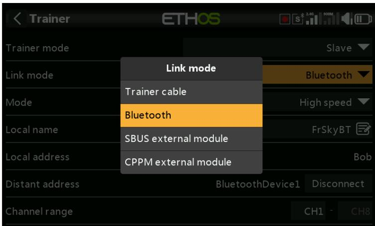
The trainer link can be either via trainer cable, Bluetooth, or SBUS or CPPM external module. The trainer cable should be a 3.5mm mono audio lead.
