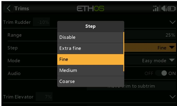
The trim step parameter allows trims to be disabled, or to configure the granularity of the trim switch steps, from 'Extra fine' through Fine, Medium, Coarse, Exponential or Custom. The Exponential setting gives fine steps near the center, and coarse steps further out. Custom allows the trim step to be specified as a percentage.
