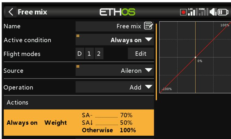
When switch is not in the middle or down positions, the weight will be 100%
