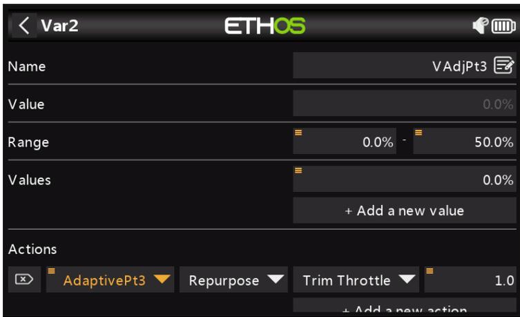
The Var named VAdjPt3 has a range of 0-50% (which should be sufficient for compensation, but may be increased if necessary). It has an action defined to repurpose the throttle trim to adjust the Var's value with a step size of 1.0% when the AdaptivePt3 logic switch defined in step 4 above is active. (Note: It will be active when the flap control has a value between -45% and 45%.)
