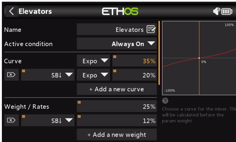
In a similar way to the Ailerons, we can set up rates and expo for the Elevator. We will use elevator rates/weights of 25% and 12%. We will use the same Expo values as for aileron.
