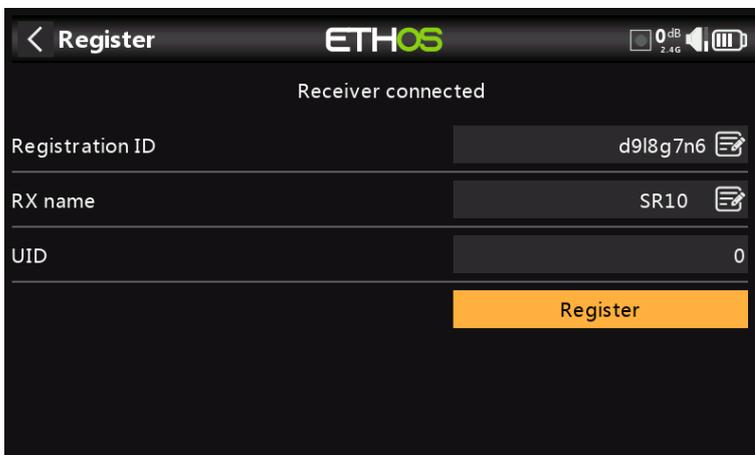
The 'Waiting for receiver...' message changes to 'Receiver connected', and Rx Name field will be filled in automatically.
