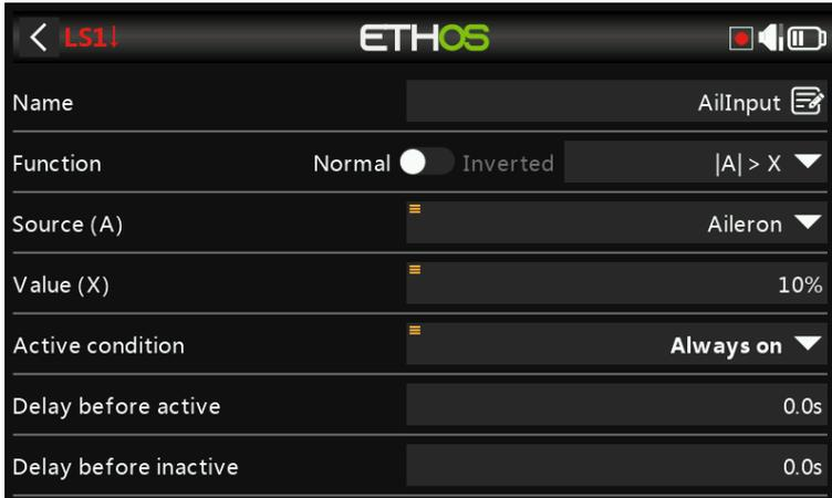
The logic switch will become True if the absolute value (i.e either positive or negative) of the aileron stick moves more than 10% from the mid position.
