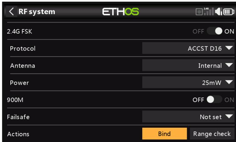
1. Initiate the binding process by selecting [Bind]. A voice alert will announce 'Bind' every few seconds to confirm that you are in bind mode.
