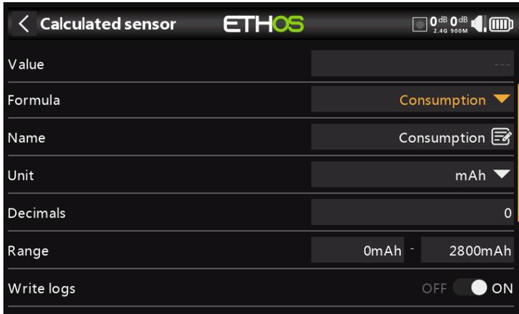
Configure the Consumption sensor to use 'mAh' units, and set the range to suit your Lipo, e.g. 2800mAh.
