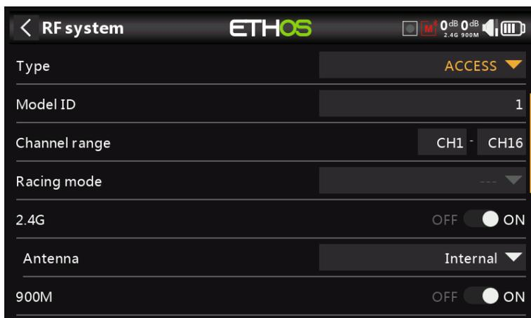
ACCESS changes the way receivers are bound and connected with the transmitter. The process is broken into two phases. The first phase is registering the receiver to the radio or radios it is to be used with. Registration only needs to be performed once between each receiver / transmitter pair. Once registered, a receiver can be bound and re-bound wirelessly with any of the radios it is registered with, without using the bind button on the receiver.
