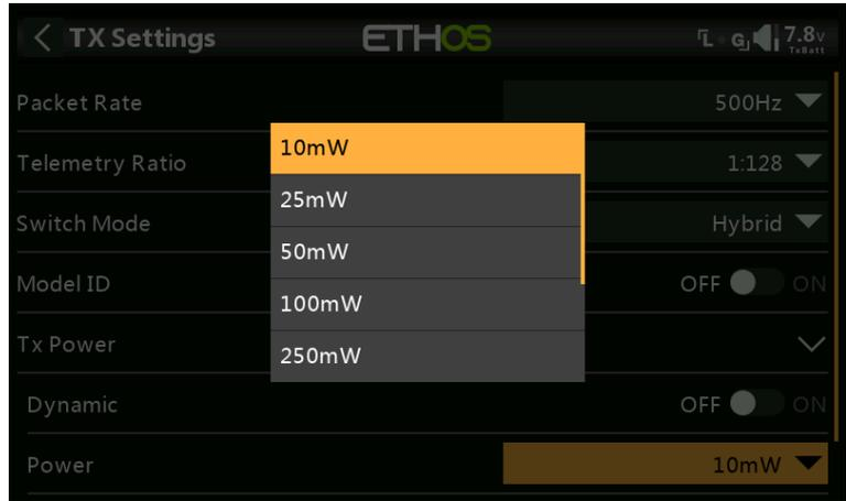
Available power settings are 10mW, 25mW, 50mW, 100mW, 250mW, 500mW or 1000mW.
