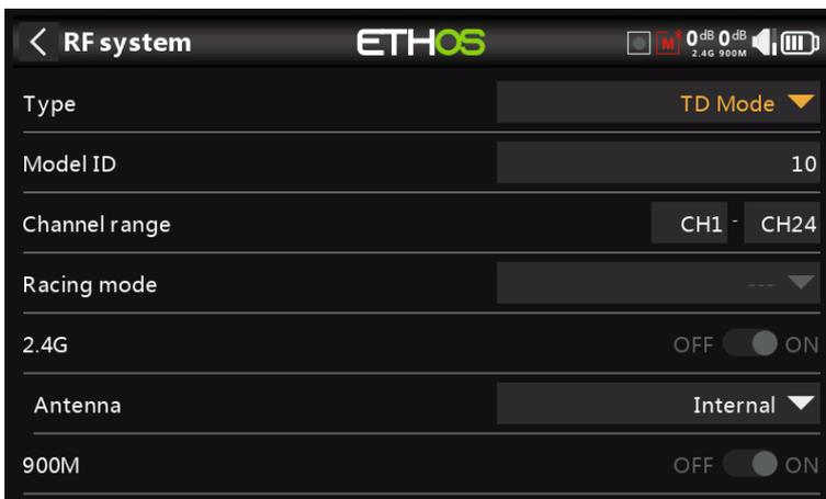
ACCESS and TD MODE change the way receivers are bound and connected with the transmitter. The process is broken into two phases. The first phase is registering the receiver to the radio or radios it is to be used with. Registration only needs to be performed once between each receiver / transmitter pair. Once registered, a receiver can be bound and re-bound wirelessly with any of the radios it is registered with, without using the bind button on the receiver.
