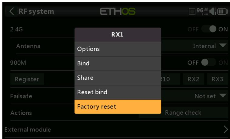
Tap on the Reset button to Reset the receiver back to factory settings and clear the UID. The receiver is unregistered with X20.
