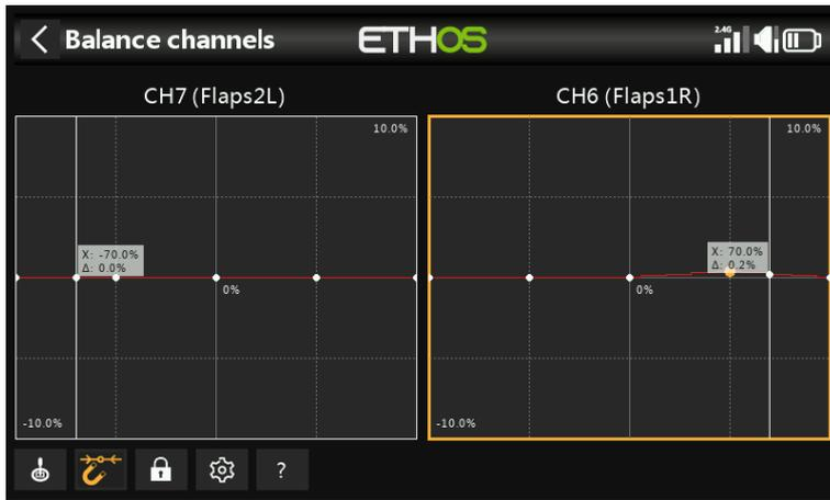
Tap on a channel graph (or scroll to it and press ENTER) to edit the balance curve. The PAGE key will switch between the channels while editing.
