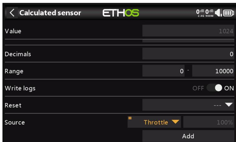
This example is simply to show the internal calculation value of a source. We will use a custom calculated sensor with the source set to Throttle. With the throttle at 100%, we can see that the internal value is +1024.
