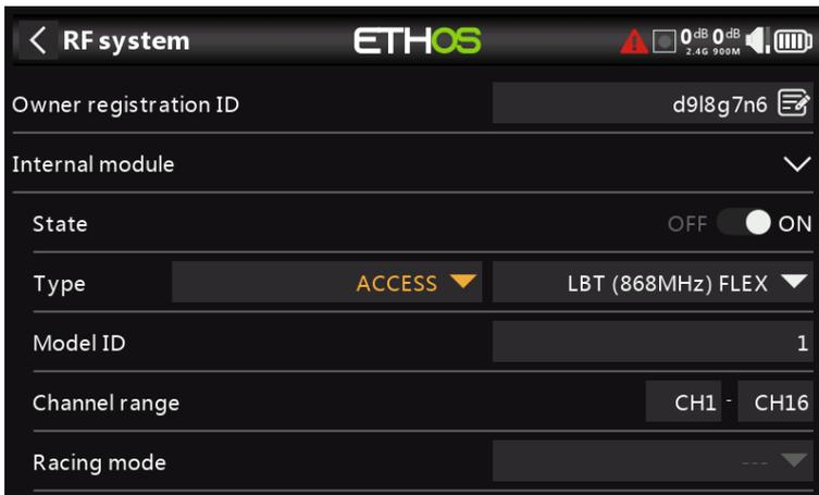
The configuration screens change as shown above. Under Type you now have two columns. The first one is for selecting the FrSky protocol (ACCESS, ACCST D16, or TD mode).
