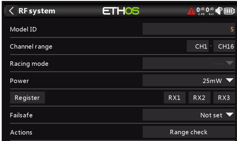
When you create a new model, the Model ID is automatically allocated. The Model ID must be a unique number because the Smart Match function ensures that only the correct Model ID will be bound to. This number is sent to the receiver during binding, so that it will then only respond to the number it was bound to. The Model ID can be changed manually. Note also that the Model ID is changed when the model is cloned.
