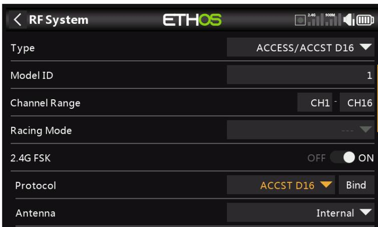
This mode is only supported in the X20 Pro. An ACCST D16 receiver may be used in conjunction with a 900M redundant receiver.
