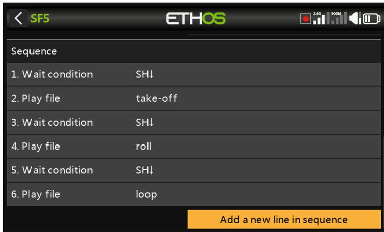
This example shows the use of 'Wait condition' to pause the sequence until switch SH is moved to the down position.
