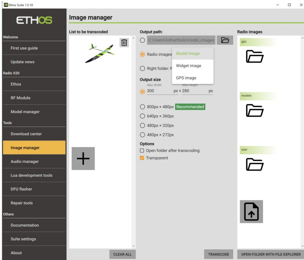
Click on the '+' button in the 'List to be transcoded' window on the left to browse and select the image to be transcoded (converted). This process can be repeated to add images to the list. Please note that TIFF format is not supported.
