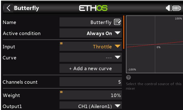
We will be using the Throttle stick as the input control, so we can set the Input to 'Throttle'.
