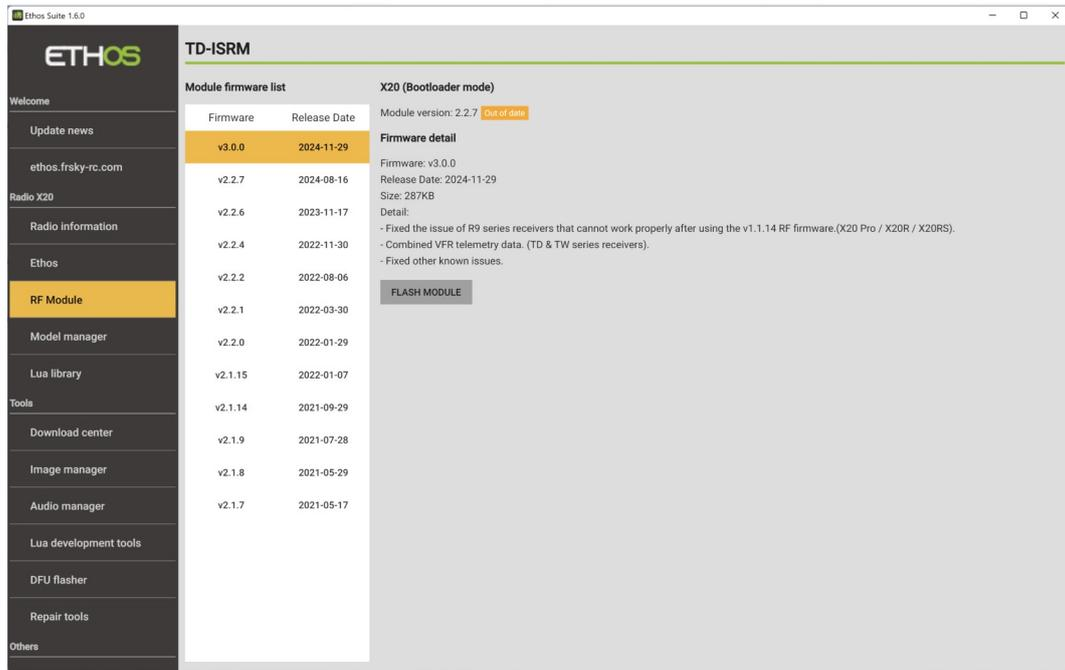
The RF module manager is used to update the RF module firmware.
