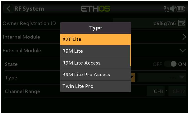
Currently the following external FrSky modules are supported: XJT Lite, R9M Lite, R9M Lite Access, R9M Lite Pro Access, TWIN Lite Pro and PPM. For third party modules please refer to the next section.
