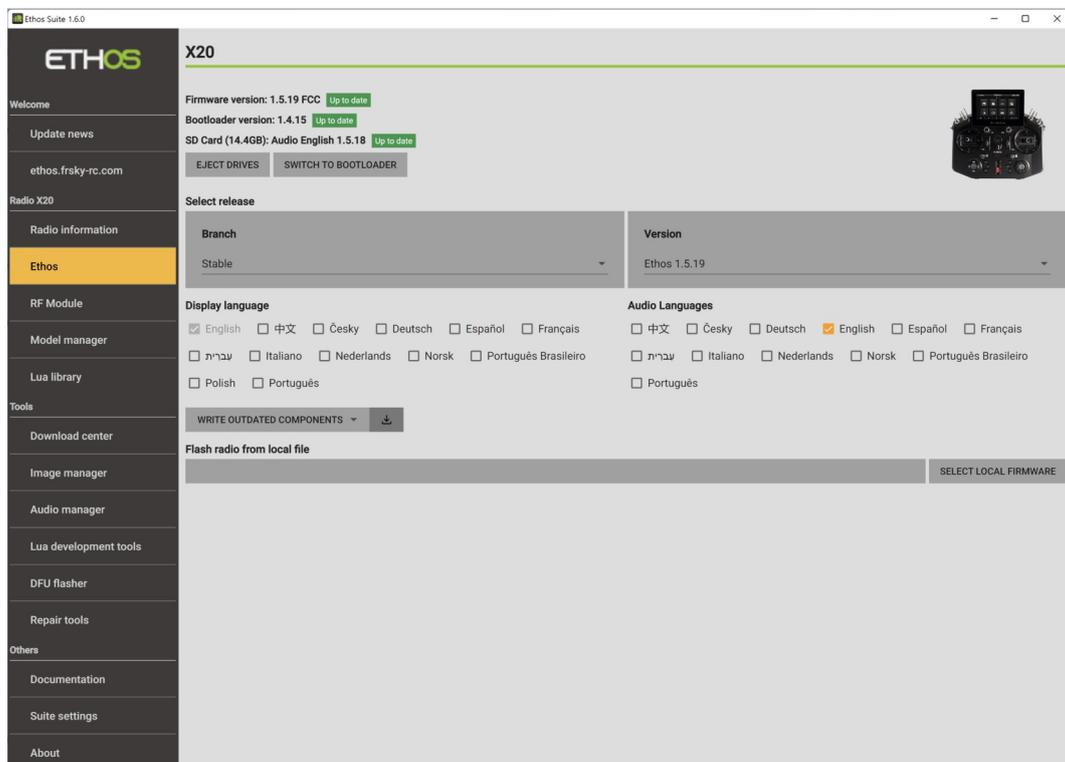
A 'Switching to firmware' message pops up, then the radio will reboot into Ethos mode and display a round green USB icon. The top of the page changes from 'X20 (Bootloader Mode)' to just 'X20' to indicate that Ethos Suite is now running in Ethos Mode.
