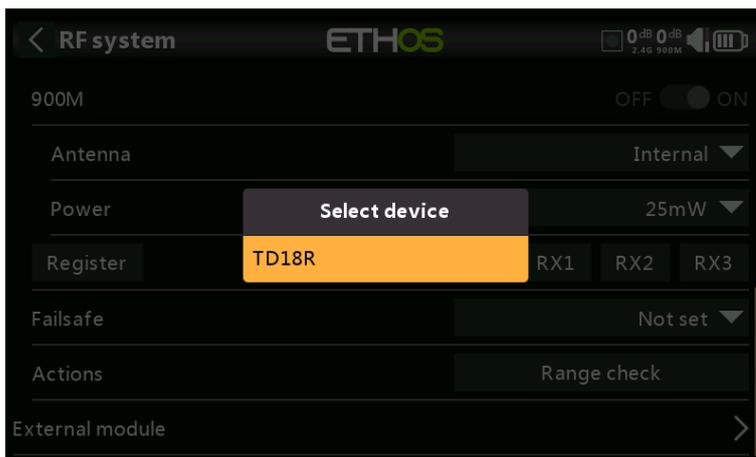
6. A message box will pop up 'Select device' and the name of the receiver you have just powered on. Scroll to the receiver name and select it.
