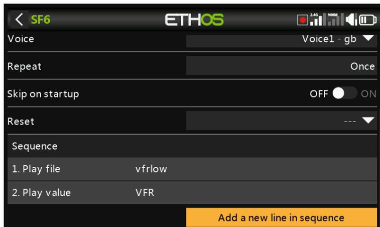
In the example above, the active condition is logic switch VFRlow. When it becomes active, 'Play file' is used to play a VFR low warning sound file called 'vfrlow.wav', which is then followed by 'Play value' playing the minimum VFR value recorded (from Telemetry).
