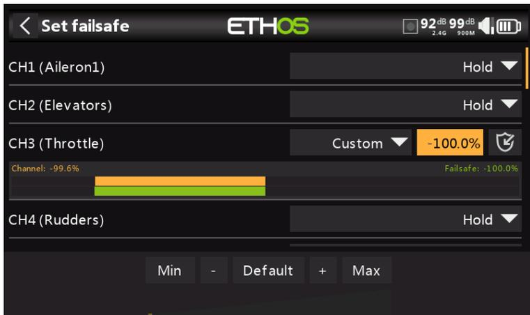
Custom allows moving the servos to custom predefined positions. The position for each channel can be defined separately. Each channel has the options of Not Set, Hold, Custom or No Pulses. If Custom is selected, the channel value is displayed. If the set icon with an arrow is tapped, the current value of the channel is used. Alternatively, a fixed value for that channel can be entered by tapping on the value.
