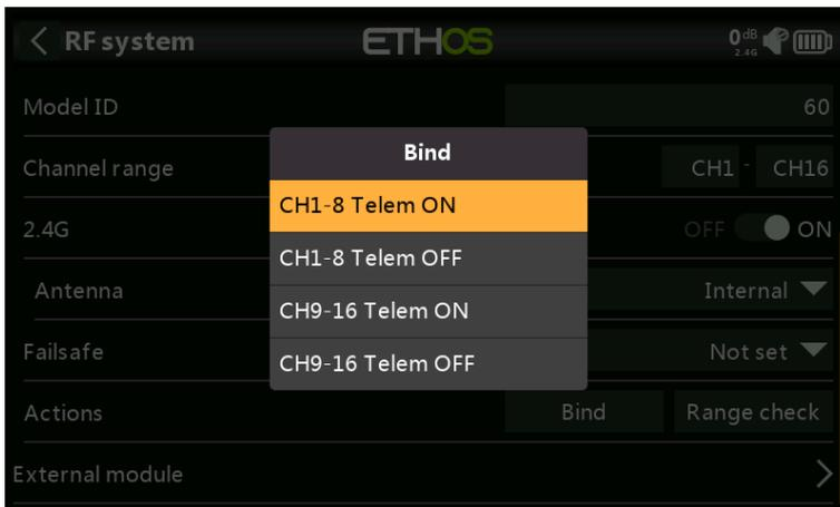
There are 4 modes with the combinations of Telemetry on/off and channel 1-8 or 9-16. This is useful when using two receivers for redundancy or to connect more than 8 servos using two receivers.
