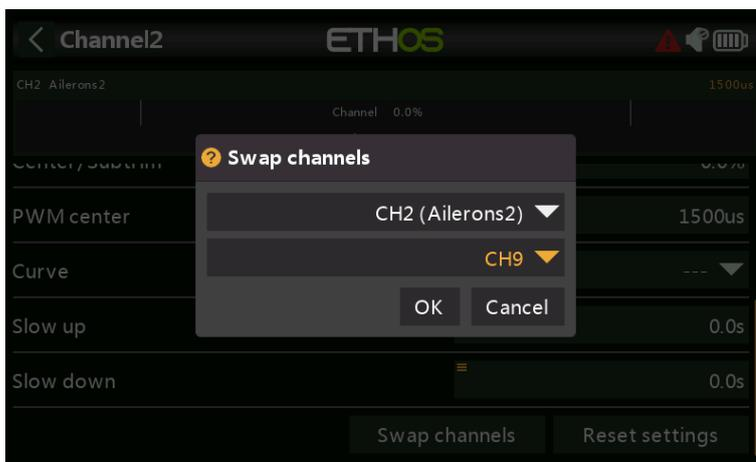
c) The swap dialog opens with the first channel (i.e CH2 Aileron2) already filled in. Select CH9 as the channel to be swapped.
