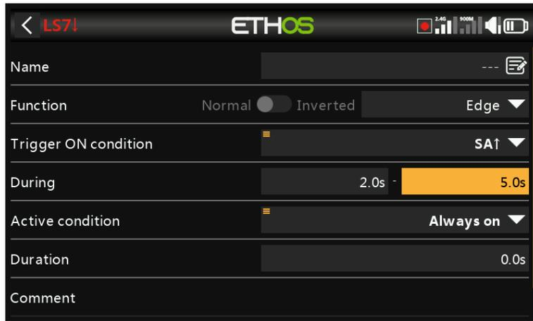
In the example above the logic switch will become True for the 'Duration' period if the 'Trigger On condition' goes from False to True, and then goes from True to False after at least 2 seconds but no later than 5 seconds.
