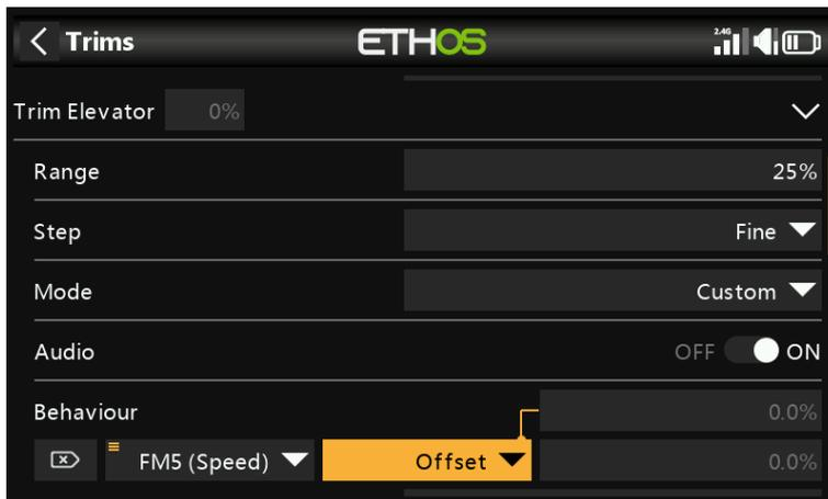
We configure the first behavior as 'Offset + Default' with condition 'FM5(Speed)'. When FM5(Speed) mode is selected, any trim adjustments will be saved as an offset to the base mode trim value in FM0(Cruise). Therefore the trim in FM5(Speed) will be separate but also dependent on the base trim.
