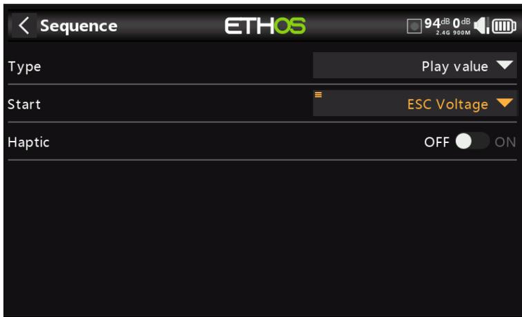
Under 'Sequence' add a 'Play value' command to speak the value of the ESC Voltage telemetry sensor.
