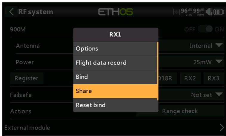
The Share feature provides the ability to move the receiver to another Tandem radio having a different 'Owner registration ID'. When the Share option is tapped, the receiver green LED turns off.
