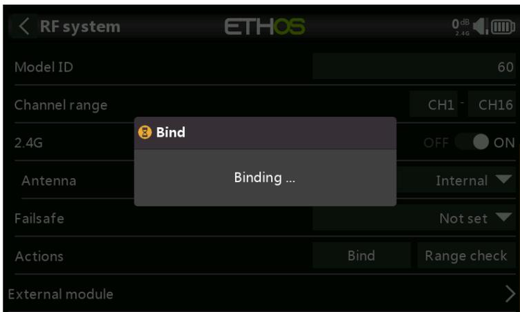
2. Power up the receiver, putting it into bind mode as per the receiver instructions. (Generally done by holding down the Failsafe button on the receiver during power up.)
