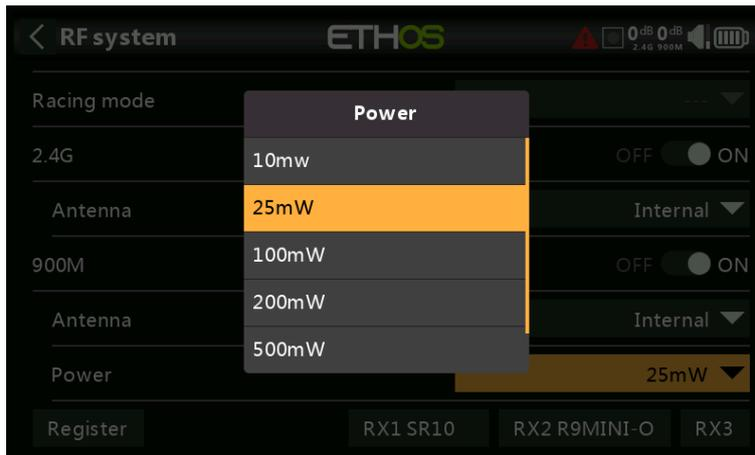
Both versions allow configuration of different power levels.
