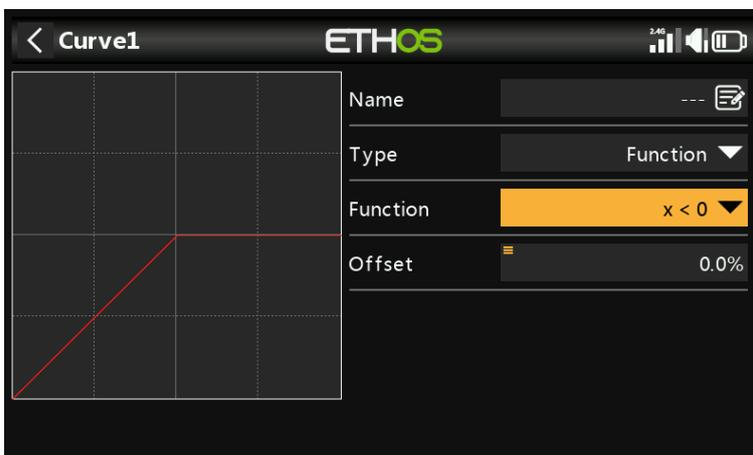
If the source value is negative, then the curve output follows the source.
