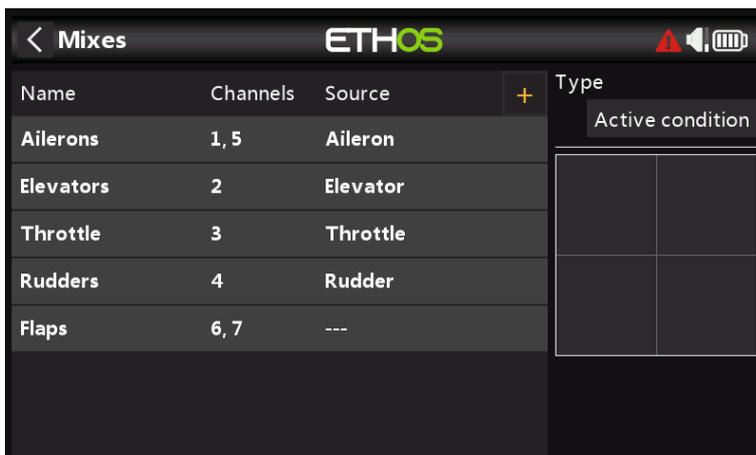
The wizard has created two Ailerons on channels 1 and 5, followed by the Elevator, Throttle, Rudder and Flaps channels. Note for the Flaps the '---' denotes that no control source has been assigned to them yet.
