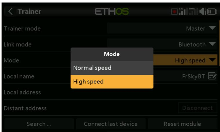
Allows selection between normal speed and high speed for the Bluetooth link. For lower latency the high speed setting should be used if both radios support it.
