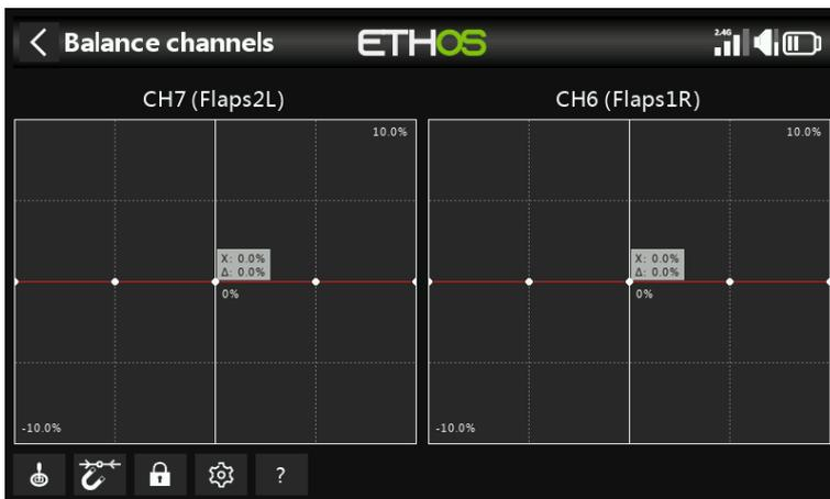
The channels will be displayed in the order of selection. In this example, CH7 Flap Left was selected first, then CH6 for Flap Right. The mix outputs are shown along the X axes, while the balance adjustment differential values are shown on the Y axes.
