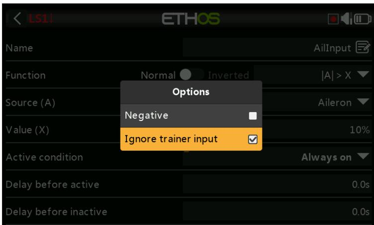
Long press on the Aileron source and select 'Ignore trainer input' so that the student's aileron movements will not trigger the logic switch.
