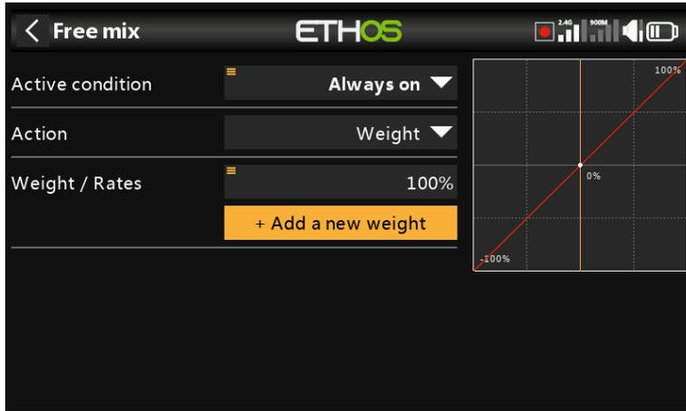
Tap on 'Add a new weight' to add additional weights. For example, to create multiple rates, simply add more 'Weight' actions made conditional by for example a 3 position switch.
