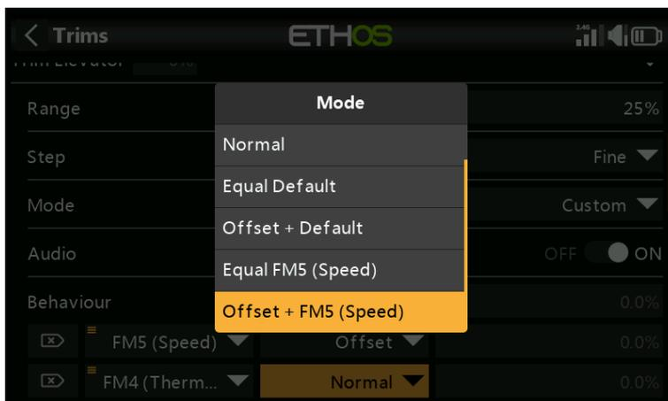
Note that when we configure the second behavior, we now get additional 'Equal FM5(Speed)' and 'Offset + FM5(Thermal)' options in the drop-down dialog. These are due to the first behavior we have configured above.
