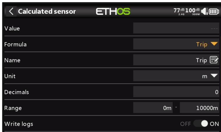
The Trip calculated sensor allows the accumulated distance between GPS coordinates to be calculated from a GPS sensor.
