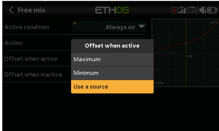
A trim may be assigned to a free mix by using the trimmer as a source (long press on the value field) for the Offset parameter.
