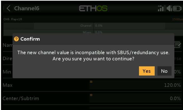
If using more than 125% on the main receiver driving PWM outputs, and this receiver enters failsafe, the servo positions then received from a redundant receiver via SBUS are limited to 125%.
