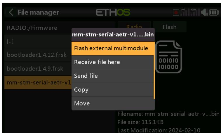
Copy the multimodule firmware file to the Firmware folder on the radio, then use File Manager to browse to the file. Tap on the highlighted filename, and select 'Flash external multimodule'. Flashing will commence, with a bar chart showing progress.
