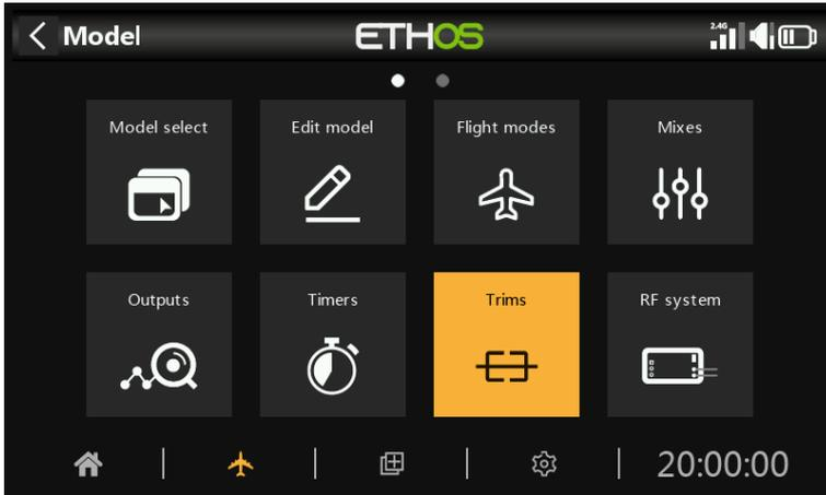
The Trims section allows you to configure the trim range and trim step size, or to configure custom trim behavior for each of the 4 control sticks. It also allows cross trims and instant trim to be configured.
