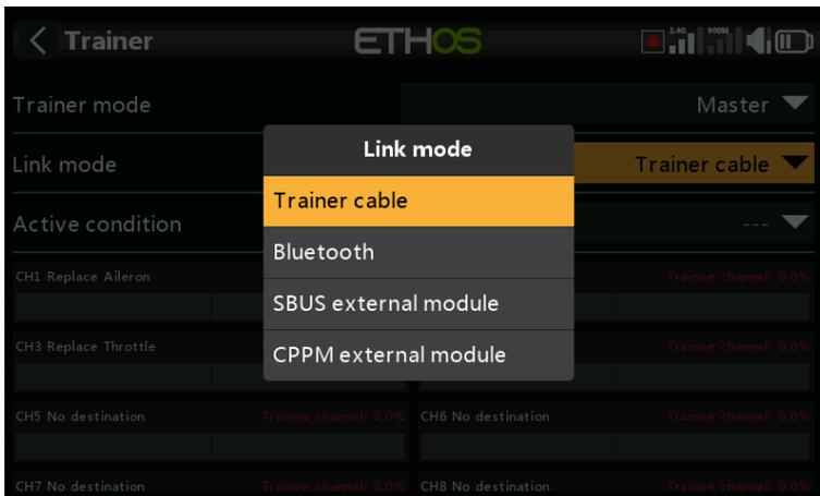
The trainer link can be either via trainer cable, Bluetooth, or SBUS or CPM external module.
