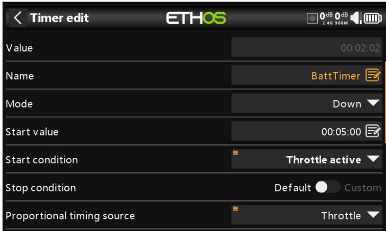
Tap on Timer 1 in the Model / Timers section, and select Edit. In this example we are configuring a Down counting timer, with a Start Value of 5 minutes. The timer will run whenever the System Event 'Throttle active' is True, provided it is not being held in reset.
