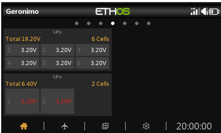
The Lipo widget displays the total pack voltage and the number of cells, as well as the individual cell voltages.
