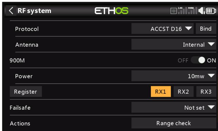
Tap 'Bind' to start binding the 900M receiver.
