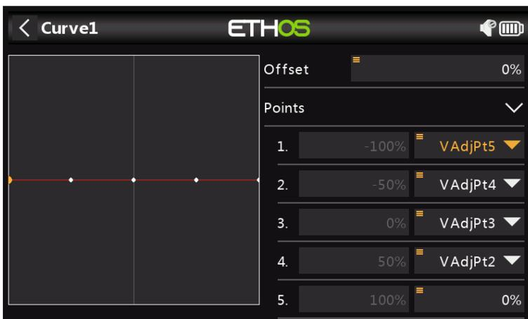
Long press Enter on each of the curve value points 1 to 4, and use the 'Use a source' option to assign the Vars VAdjPt5 through to VAdjPt2 as shown in the above example.
