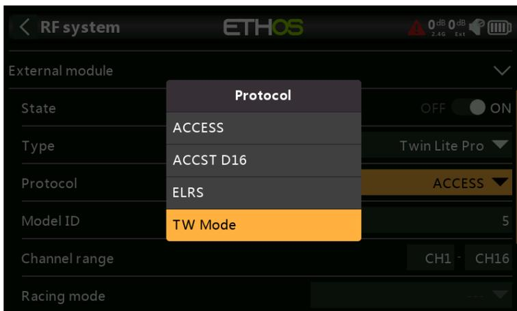
Transmission mode of the TWIN Lite Pro RF module. In addition to the TW mode, this module also supports ACCST D16, ACCESS, and ELRS 2.4G modes.
