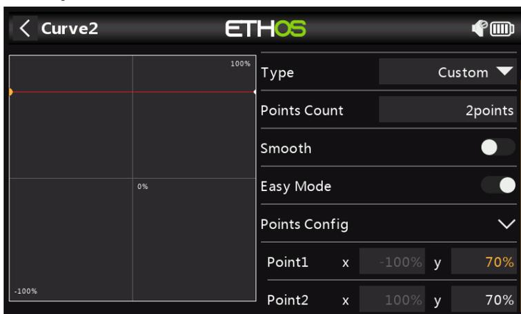
Idle Up 1 is used for most flying. The straight line curve means that we will have a constant throttle setting to keep the rotors spinning at a steady rate. The final throttle value may need to be determined in flight. The helicopter's motion will be controlled by the Collective Pitch and Aileron (roll) and Elevator (pitch) controls.
