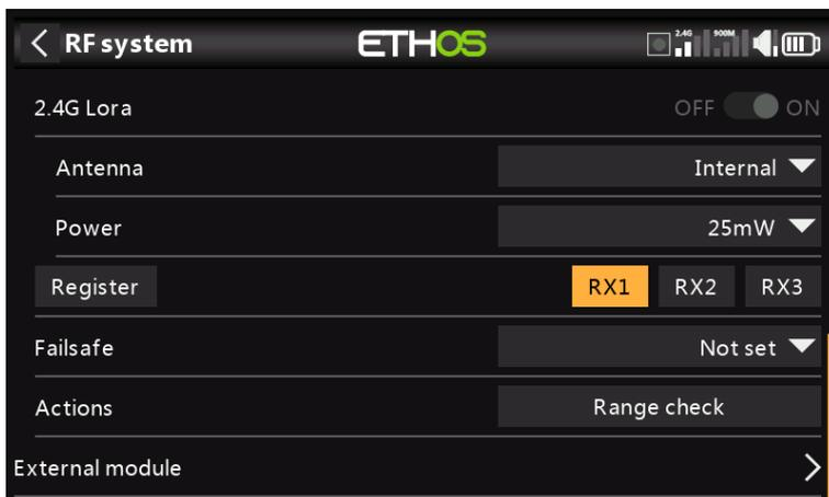
Receiver binding enables a registered receiver to be bound to one of the transmitters it has been registered with in phase 1, and will then respond to that transmitter until re-bound to another transmitter. Be certain to perform a range check before flying the model.
