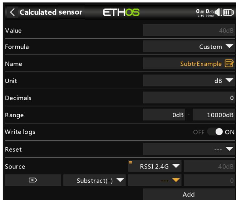
In this example we start with the RSSI 2.4G source, and then add a Subtraction function.
