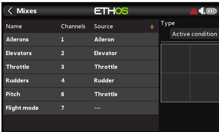
The wizard has created Ailerons, Elevators, Throttle and Rudder in the AETR sequence as expected, and created Pitch on channel 5 and Flight Mode on channel 6.
