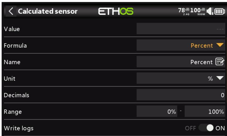
The Percent calculated sensor allows sensor values to be converted to a percentage.
