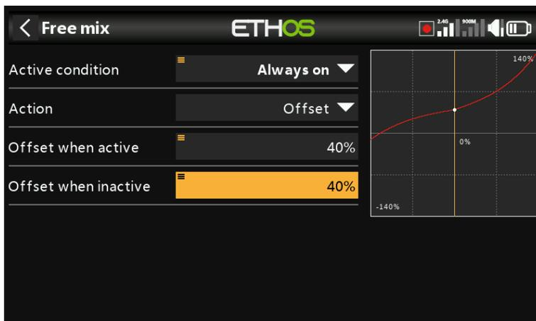
An offset will shift the mix output up or down by the offset value entered here. Negative values are allowed.
