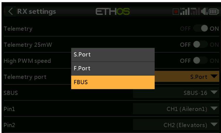
Scroll down to the 'Telemetry Port' parameter and select FBUS. The Telemetry Port on the receiver will now operate on the FBUS protocol. The Xact servos can now be daisy-chained off this FBUS port. Since the servos only have a single connector, F.Port 2.0 multichannel extenders such as the FP2CH4, FP2CH6 or FP2CH8 can be used to extend the FBUS wiring.
