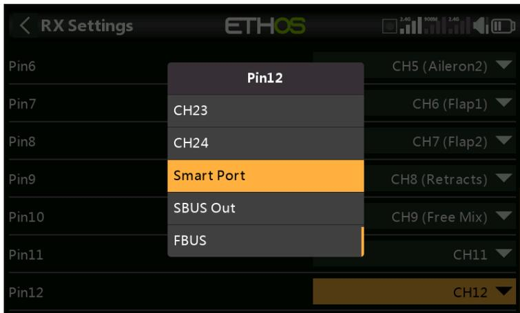
*Pin1-12 Options:* Gives the ability to remap radio channels to the receiver pins. In addition, each output port may be reassigned to Smart Port, SBUS Out, or FBUS (previously known as F.Port2) protocols.
