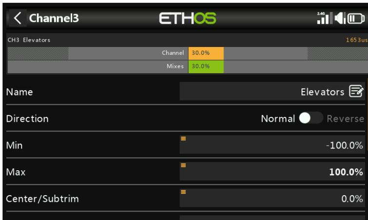
When adjusting the min/max output limits, the end to be adjusted is highlighted bold.
