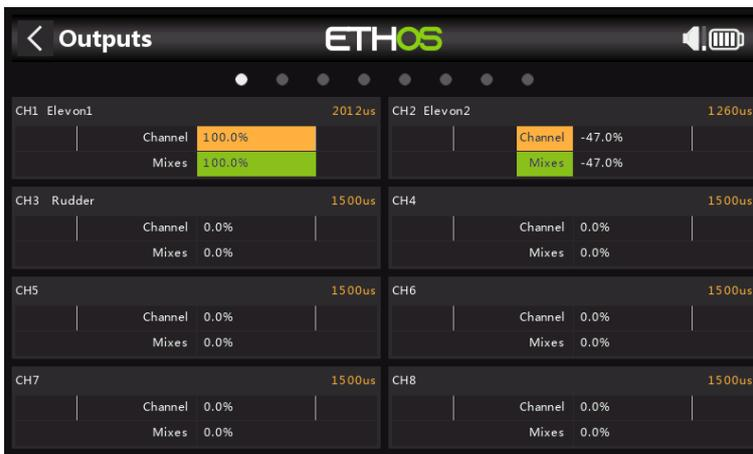
This example shows that full right aileron has been applied as well as full down elevator so channel 1 is at  $75+25 = 100\%$ , while the left down-going aileron is at  $72-25 = 47\%$  due to aileron differential.
