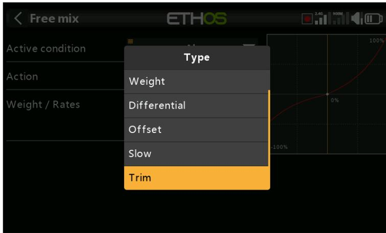
To add a trim to the mix, select 'Trim' from the actions drop-down menu. This is simpler than adding the trim under the Offset action.
