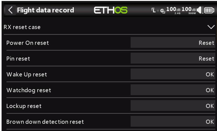
Power On reset, output Pin reset, and the results of wakeup, watchdog timer, lockup detection and power brown out detection.
