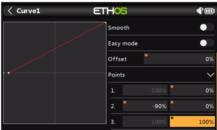
As soon as you add your own curve to the Butterfly mix, the internal offset that makes the source control operate from 0 to 100 is removed. This means our curve must also transform the source control to go from 0 to 100.
