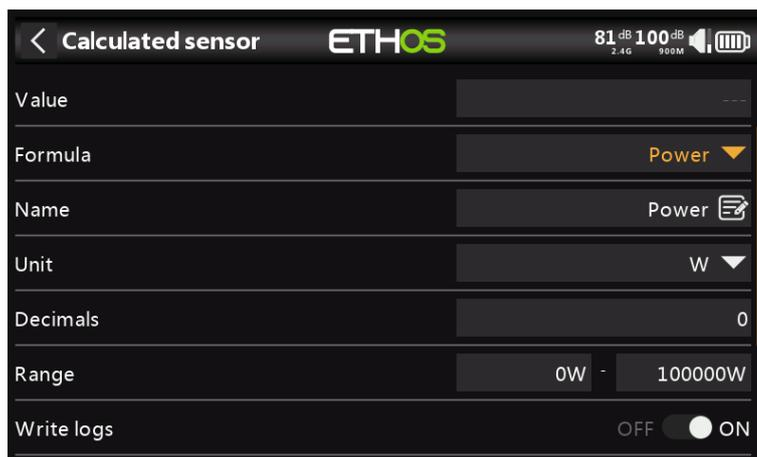
The Power calculated sensor allows power to be calculated from a voltage and a current source.
