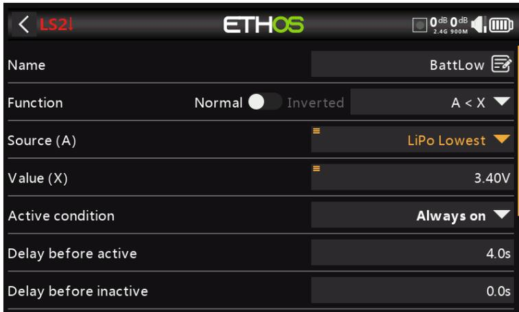
Set the Value to something like 3.4V, and 'Delay before active' to 4 seconds. The Logical Switch will become True/Active when the lowest cell voltage remains below 3.4 per cell for 4 seconds or more. A threshold of 3.4V under load will recover to around 3.7V when no longer under load.
