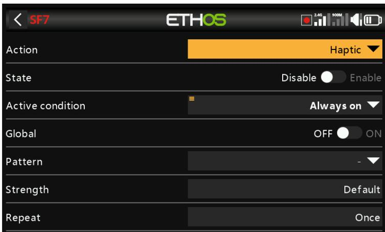
This special function assigns haptic vibration
