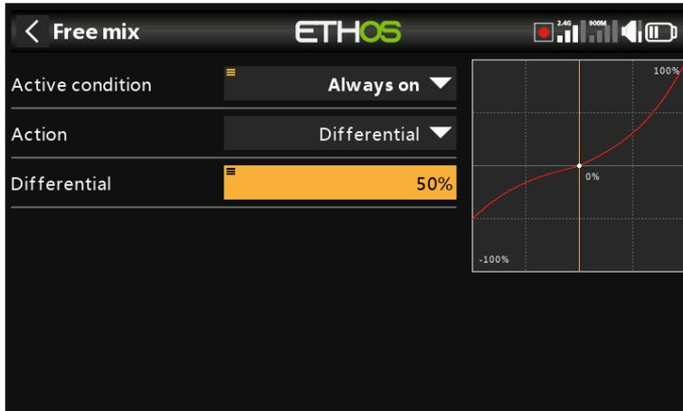
A positive value will result in the mix output having less downward travel. (Default = 0. Range -100 to +100). With a value of 50% downward travel is half of the upward travel, as can be seen in the example above.
