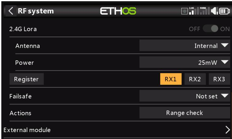
3. Receiver 1 [Bind]: Initiate the binding process by selecting [RX1], then select Bind from the drop-down list. A voice alert will announce 'Bind' every few seconds to confirm that you are in bind mode. A popup will display 'Waiting for receiver...'
