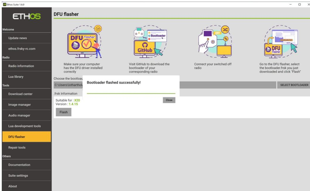
Now connect your switched off radio off to the PC with a USB lead. Click on the 'Flash' button to flash the selected bootloader. It will report success when completed.
