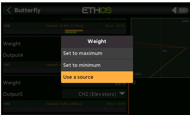
Now go back to the Butterfly mix, scroll right down and long-press [ENT] on the Weight for the Elevator Output, then select 'Use a source'.
