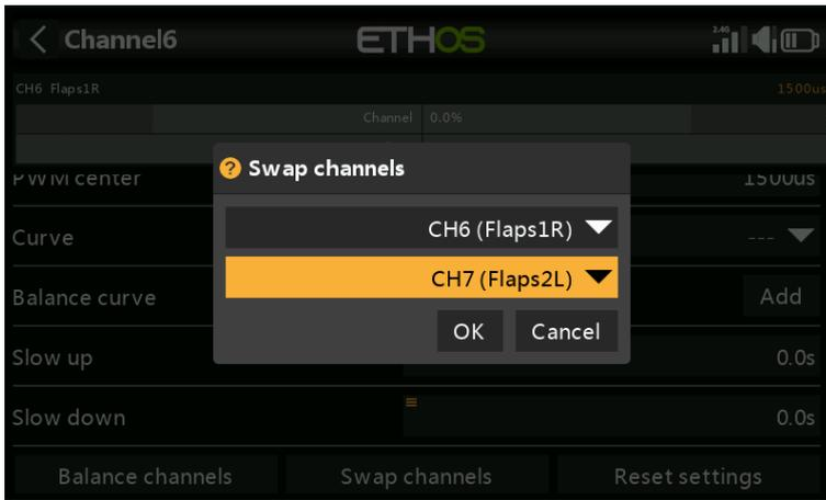
The swap dialog opens with the first channel already filled in. Select the channel to be swapped, and click OK. Note that the swap takes place immediately. All mixes etc will be adjusted accordingly.
