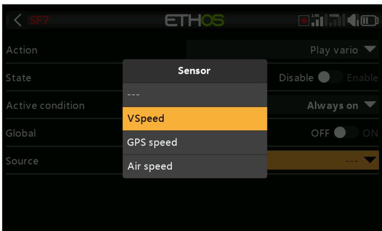
The default is normally the VSpeed sensor on FrSky varios, but any sensor with units of m/s can be used.
