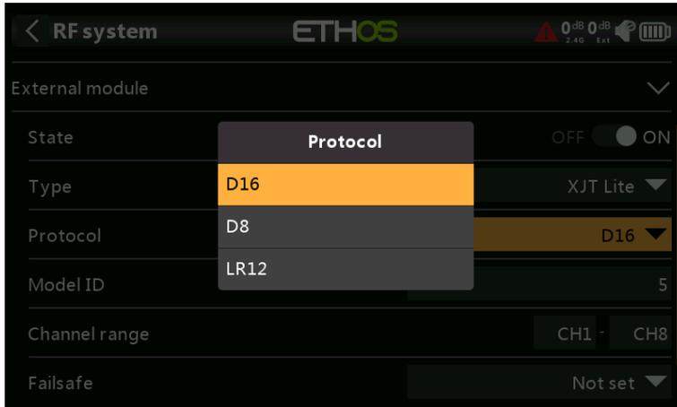
The XJT Lite can operate in D16 (up to 16 channels), D8 (up to 8 channels) or LR12 (up to 12 channels) modes.
