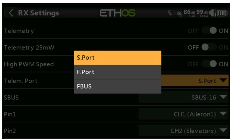
*Port*: Allows selection of the SmartPort on the receiver to use either S.Port, F.Port or the FBUS (F.Port2) protocol. The F.Port protocol was developed with the
