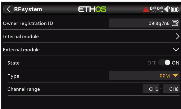
The External RF Module can operate in PPM mode.
