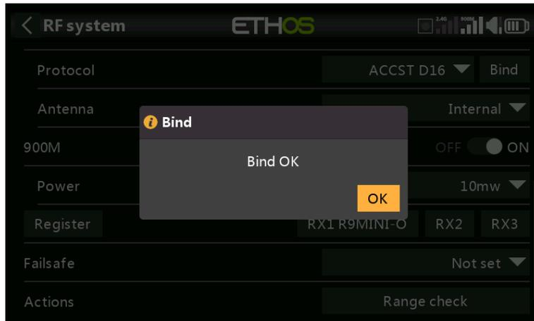
Tap on OK. Ensure that the Green LED on the redundant receiver is ON. The redundant receiver is now bound.
