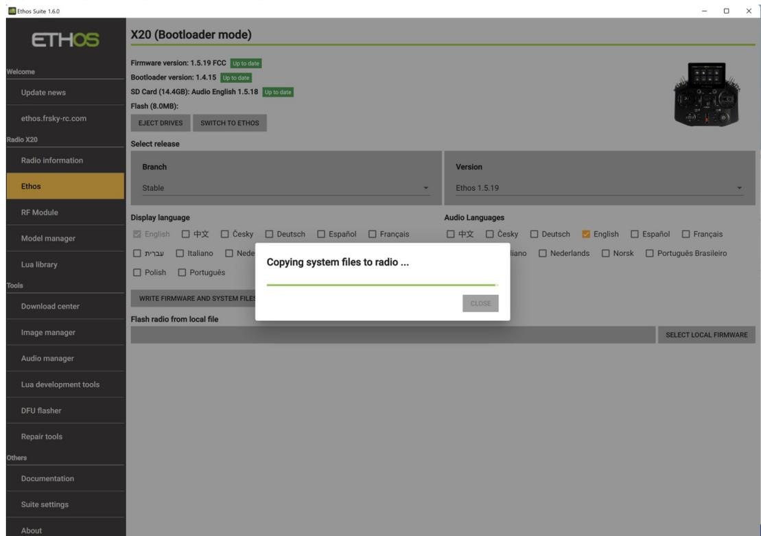
Ethos Suite will then automatically download the corresponding release of system bitmap files to the radio. These no longer have to be managed separately.
