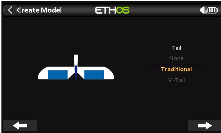
Accept the default Traditional Tail (which has Elevator and Rudder).
