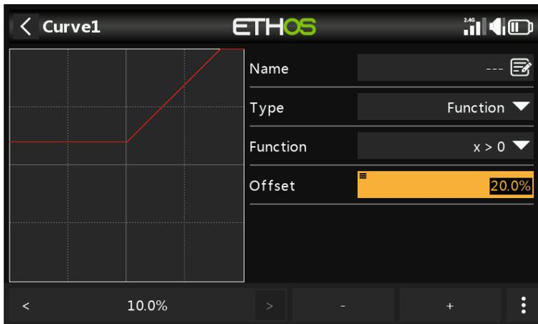
Note that all curves can have a positive or negative offset which will shift the curve upwards or downwards on the Y axis. Curves offsets and Y value have a one decimal precision.
