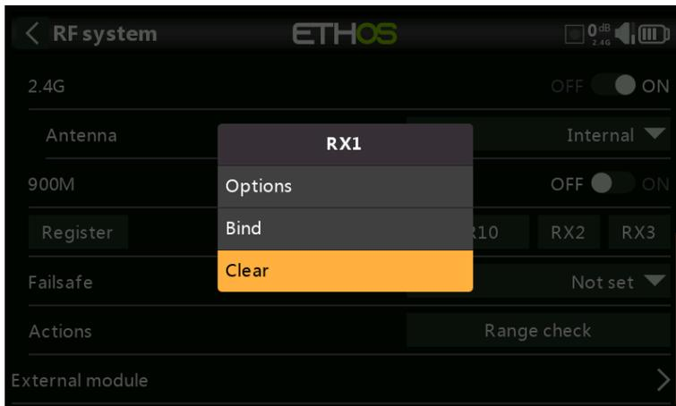
With the receiver powered off, tap the RX1, 2 or 3 button to bring up receiver options.
