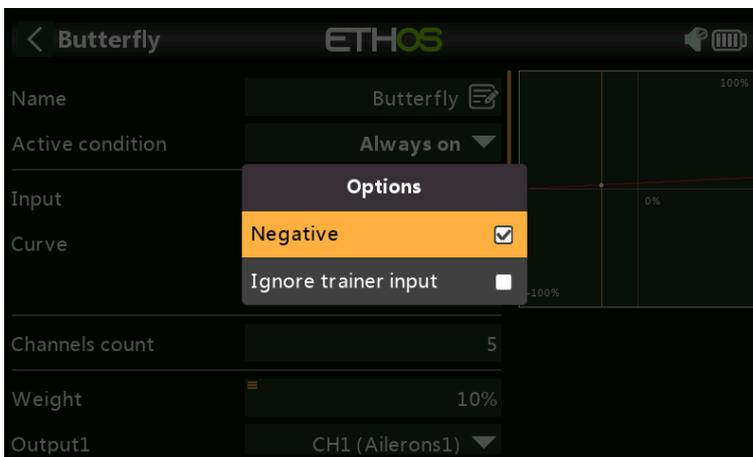
By default the Throttle input is at maximum when the stick is fully up. For the Butterfly mix we want it to be 0 when the stick is fully up, so we will invert the input. Long press on 'Throttle' for the Invert dialog.
