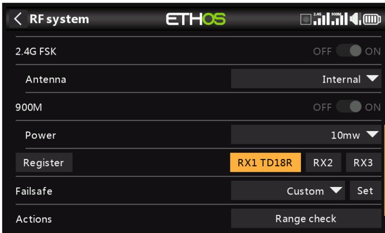
With an TD-R18 Tandem receiver registered and bound, go to RF System and tap on the 'TD18R' button.
