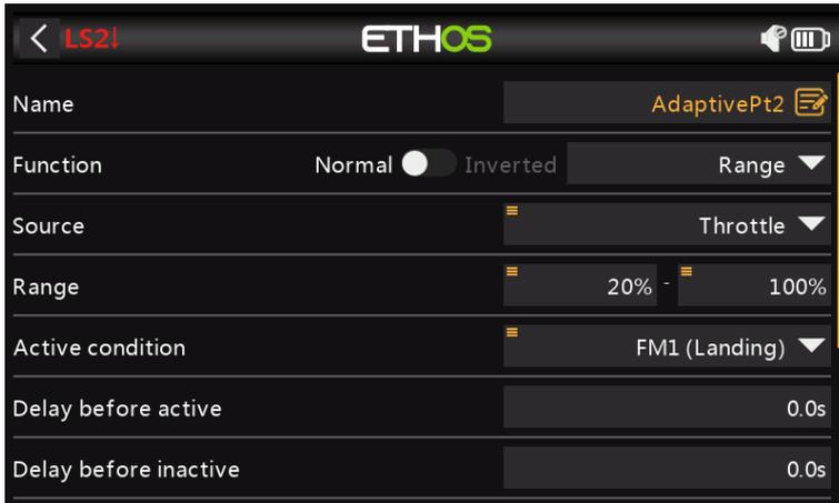
Set up a logic switch AdaptivePt2 with the flap (i.e throttle) stick as source, and a range of 20% to 100%. Making the range up to 100% allows adjustment of point 2 even with no flaps. Please refer to the setup explanation in step 6 below.
