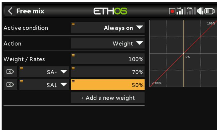
In the example above two extra weights (or rates) have been added using switch SA.
