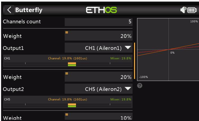
Normally for butterfly or crow braking, the ailerons are set to go up a modest amount, say 20%, while the flaps go down a large amount. This combination creates a lot of drag, and is very effective for braking. (In the above example the top graph line is at 20% for the ailerons, the other channels are still at 10%.) The vertical yellow line shows that the Throttle stick is fully down, i.e. at the full Butterfly position, so the Aileron outputs are at 20%.
