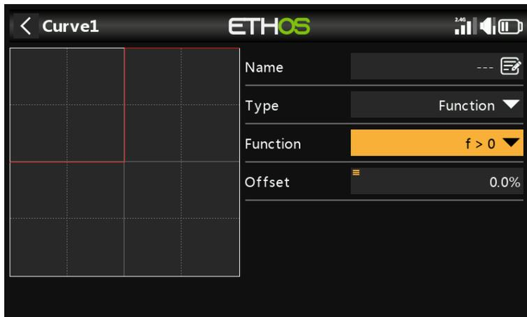
If the source value is negative, then the curve output is 0.
