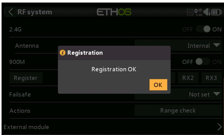
5. Turn the receiver off. At this point the receiver is registered, but it still needs to be bound to the transmitter to be used. It is now ready for binding.
