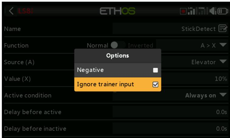
In logic switches the sources may have this option set to ignore sources coming from the trainer input. A typical application is where a logic switch is configured to detect movement of the master trainer's sticks (e.g. Elevator stick) to allow for instant intervention if things go wrong. This option is needed to prevent the student stick inputs from triggering the logic switch.
