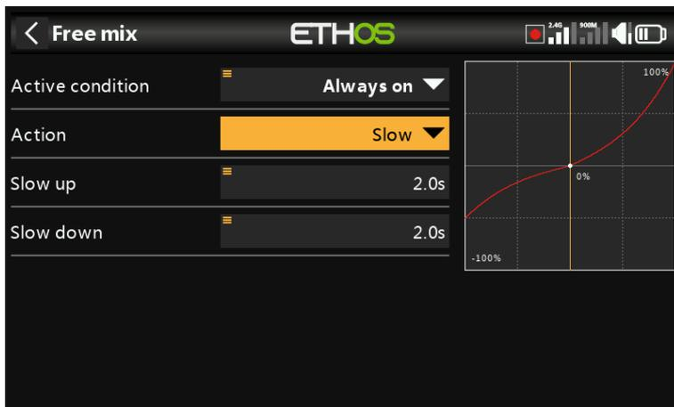
Response of the output can be slowed down with regard to the input change. Slow could for example be used to slow retracts that are actuated by a normal proportional servo. The value is time in seconds that the output will take to go from 0 to +100%.
