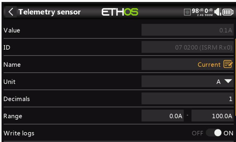
In this example a FAS100 was used, so the Range is set to 0-100A.
