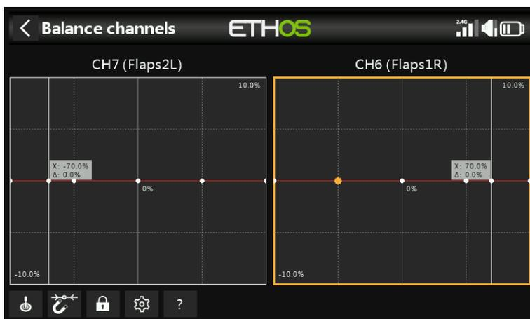
In the example above, the Magnet option has been deselected. The curve point to be adjusted is highlighted, and can be moved using the 'SYS' and 'DISP' keys.
