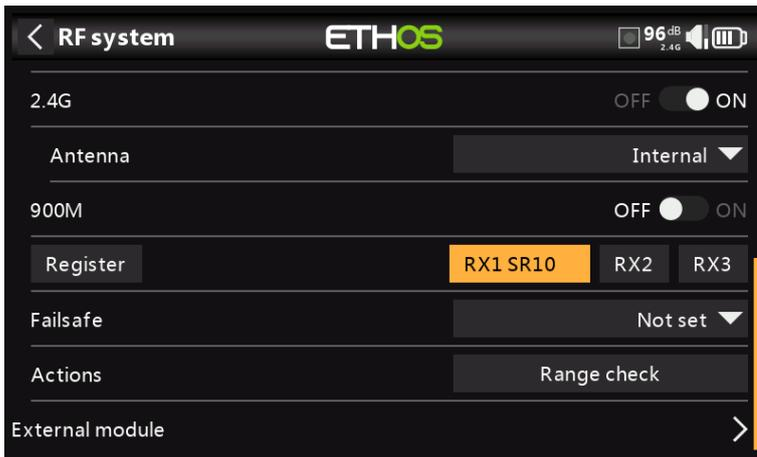
With the receiver powered on, tap the RX1, 2 or 3 button to bring up receiver options and other receiver operations:
