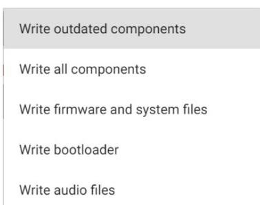
Alternatively, clicking on the 'Write outdated components' option itself will open a drop-down list showing the alternative options to write all components, or to only write the firmware and system files (needed to run the firmware), or the bootloader, or the audio files individually.
