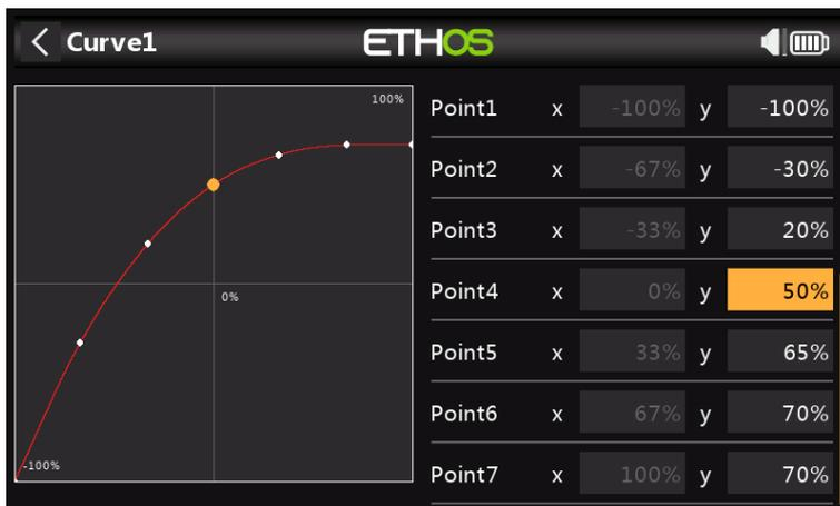
Normal mode is used for spool up and take off, so the curve starts at -100% (motor off) and then smoothly increases for take off. The final curve values may need to be determined in flight.
