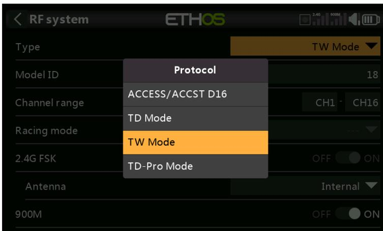
The way receivers are bound and connected with the transmitter is broken into two phases. The first phase is registering the receiver to the radio or radios it is to be used with. Registration only needs to be performed once between each receiver / transmitter pair. Once registered, a receiver can be bound and re-bound wirelessly with any of the radios it is registered with, without using the bind button on the receiver.
