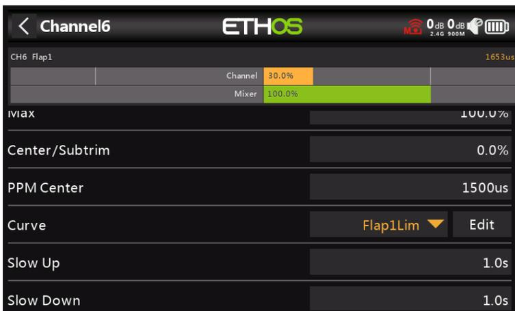
In a similar way the Flap1 channel can have a 'Flap1Lim' curve assigned to it. In addition, Slow Up and Slow Down could be set to 1 second, so that the flaps move to the new position slowly.
