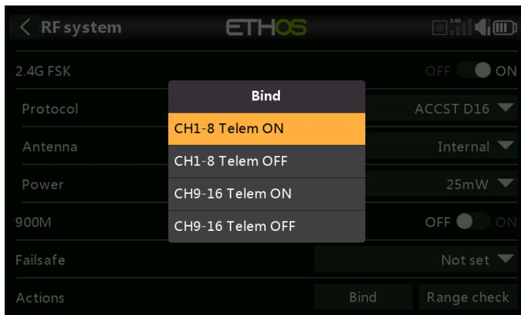
In D16 mode a pop-up menu will open during bind to allow selection of the operation mode of the receiver. There are 4 modes with the combinations of Telemetry on/off and channel 1-8 or 9-16. This is useful when using two receivers for redundancy or to connect more than 8 servos using two receivers.
