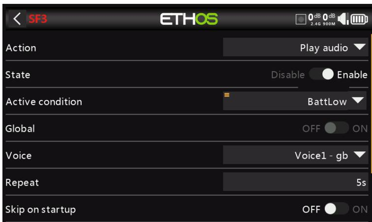
Now add a special function to speak the value of 'ESC Voltage' every 5 seconds when the logical switch BattLow becomes True..
