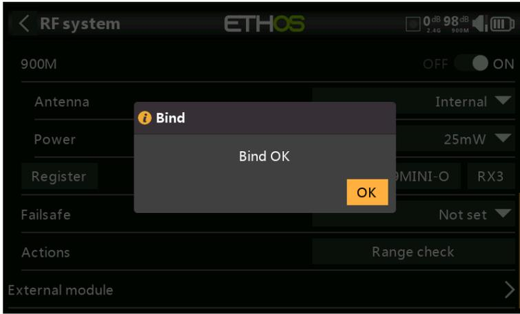
9. Tap on OK. Ensure that the Green LED on the redundant receiver is ON. The redundant receiver is now bound.
