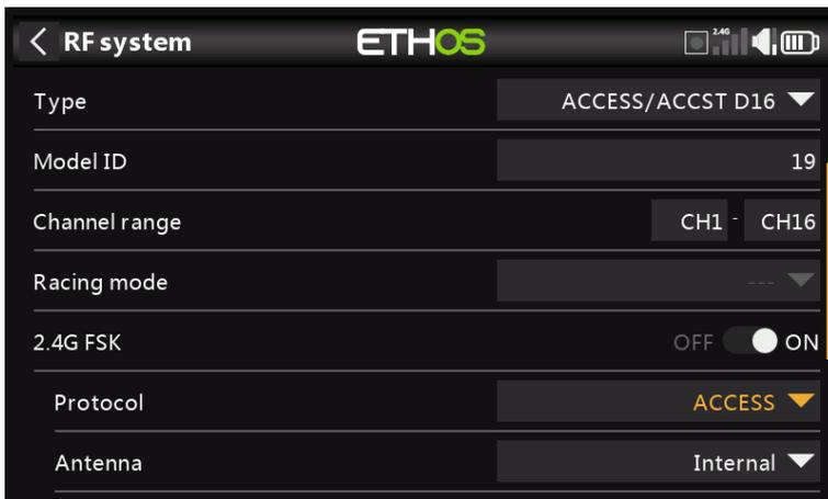
This mode is similar to the ACCESS mode in the X20. Up to a total of three ACCESS or 900M receivers may be bound. Please refer to the [X20 ACCESS](#) section for setup details.
