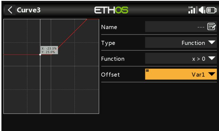
The above example shows the Offset parameter of a curve of type "Function" driven by a Var, which could possibly be adjusted in flight by a reassigned Trim.
