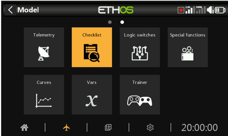
The Checklist function provides for a set of preflight checks. This is a group of safety features that take effect when powering up the radio and/or loading a model from the model list.
