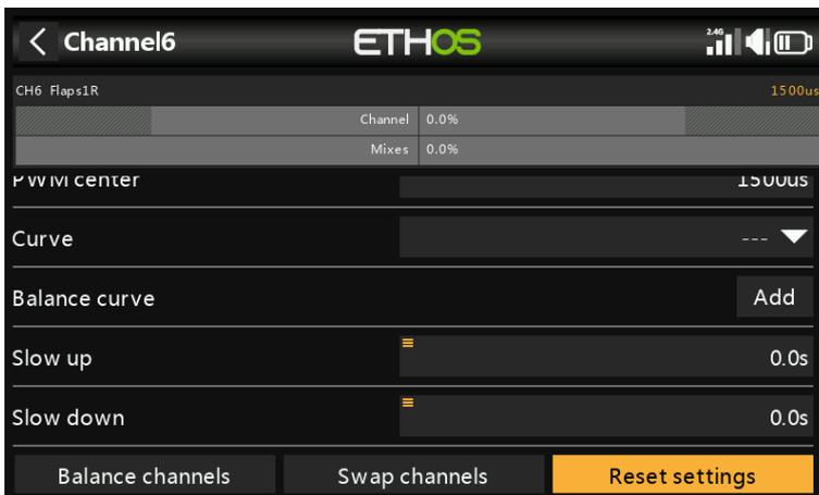
Reset settings will clear all parameters for the Output channel if the channel is no longer required. A confirmation dialog will avoid accidental resetting.
