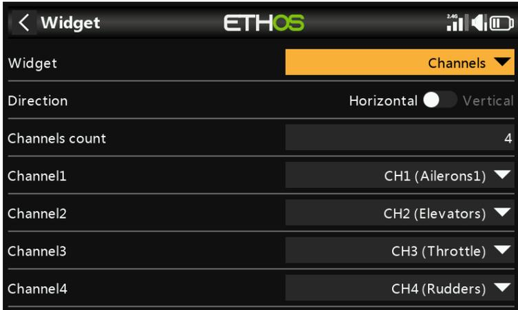
The Channels widget allows up to 8 channels to be displayed in bar chart format, with either horizontal or vertical bars.
