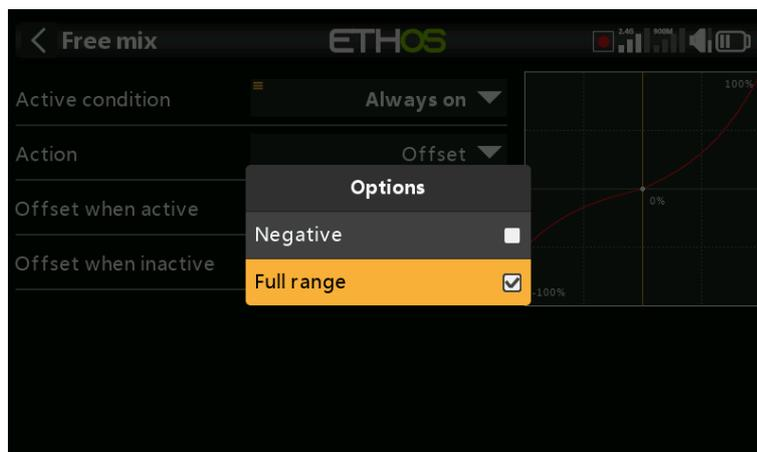
By default trims have a range of +/- 25%. When used as a source, trims can optionally be changed to full range +/- 100% (long press Enter on the trim).
