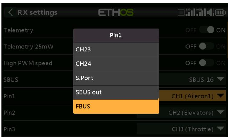
Scroll down and tap on the Pin1 parameter, and select FBUS as the option for Pin1, to change the default PWM connection to the FBUS protocol.
