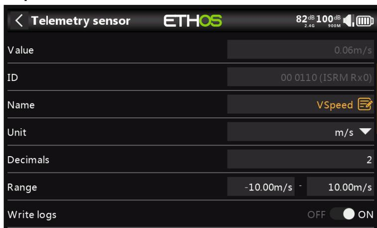
Vspeed is the vertical speed of the model measured by a vario sensor.
