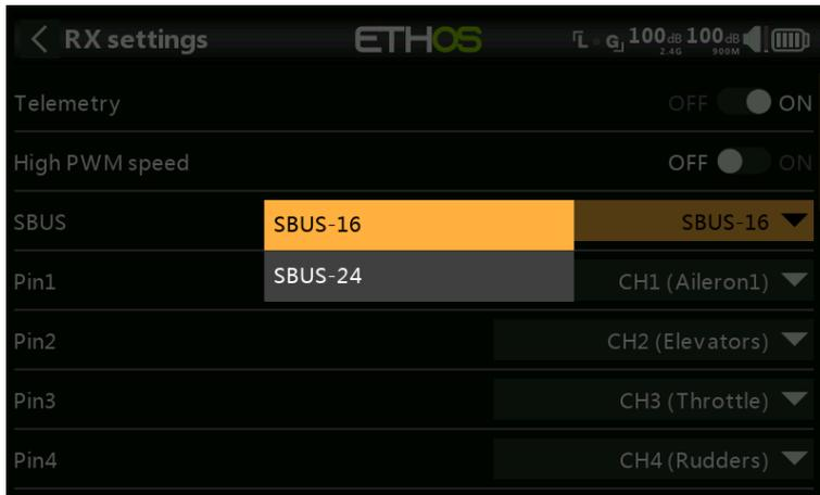
*SBUS*: Allows selection of SBUS-16 channel or SBUS-24 channel mode. Be aware that all connected SBUS devices have to support the SBUS-24 mode in order to activate the new protocol. SBUS-24 is an FrSky development of the SBUS-16 Futaba protocol.
