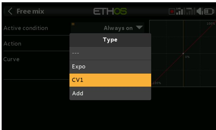
Any previously defined curve may also be selected (for example CV1 in the example above). The mix output will then modified by this curve.
