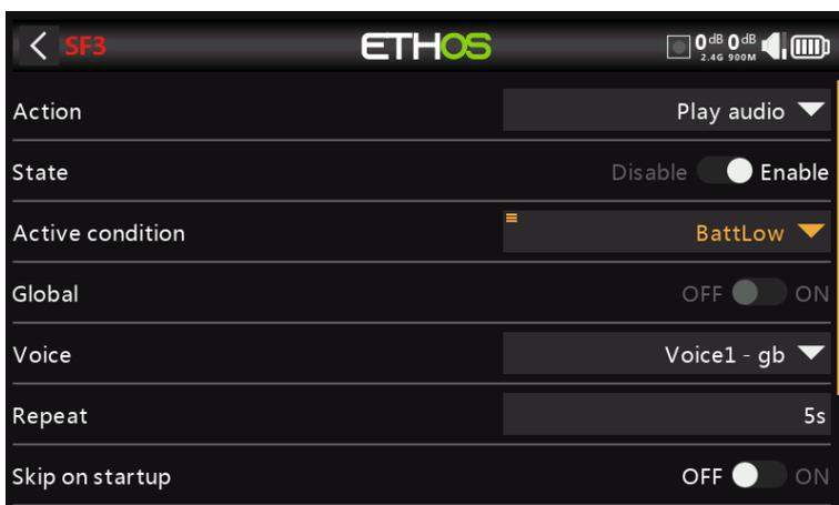
Add a special function to speak the value of the LiPo total voltage every 5 seconds when its value drops below the threshold of 3.4V per cell for 4 seconds as set up in the logical switch above.
