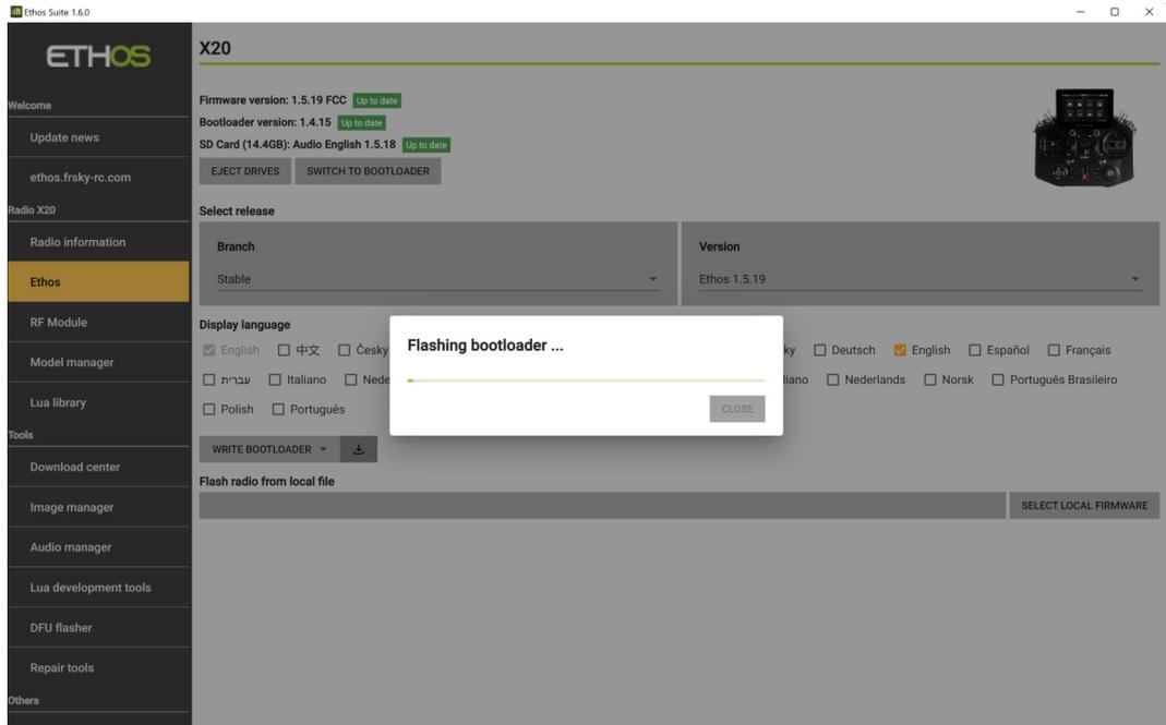
Select the 'Write bootloader' option, then click on the dark grey download button next to the selected option. Ethos Suite will download the latest bootloader to the radio, which will be shown in the versions list after completion. In the example above bootloader 1.4.15 was re-written.
