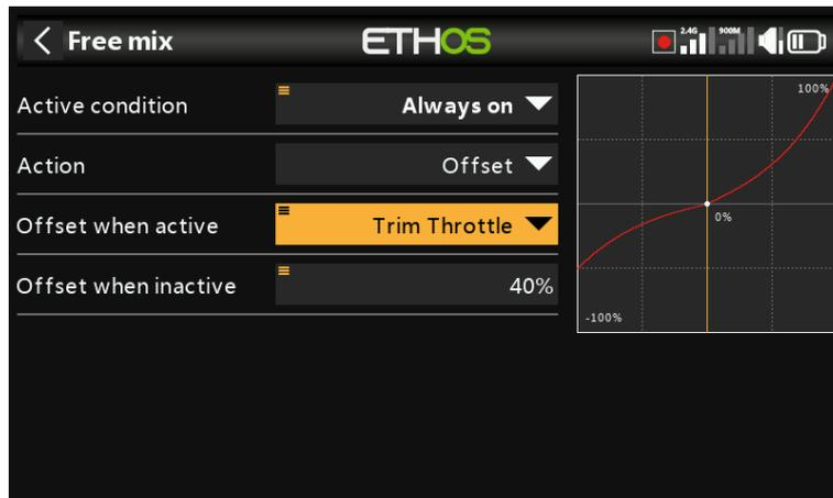
In the example above, the throttle trim has been selected as the source for adjusting the Offset.
