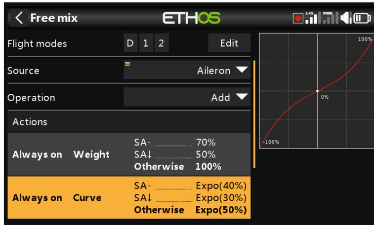
With the SA switch in the mid position, the weight rate is 70% while the expo is 40%. With the SA switch in the down position, the weight rate is 50% while the expo is 30%. With the SA switch in the default (up) position, the default weight rate is 100% while the default expo curve is 40%.
