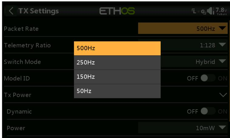
Packet rate allows a compromise to be made between range and latency. A higher packet rate results in lower latency, but at the cost of range.
