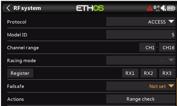
The Failsafe mode determines what happens at the receiver when the transmitter signal is lost.
