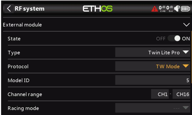
In terms of binding, TW Mode is similar to ACCESS in the way receivers are bound and connected with the transmitter. The process is broken into two phases. The first phase is registering the receiver to the radio or radios it is to be used with. Registration only needs to be performed once between each receiver / transmitter pair. Once registered, a receiver can be bound and re-bound wirelessly with any of the radios it is registered with, without using the bind button on the receiver.
