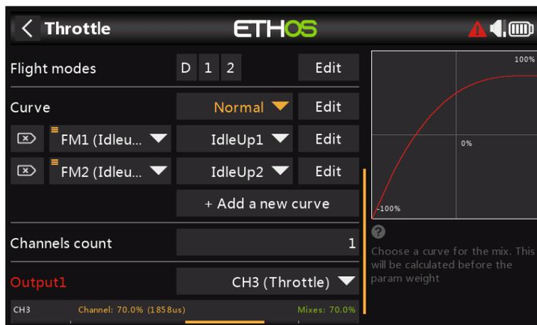
We can now configure the Throttle mix for the three throttle curves, controlled by the flight modes.
