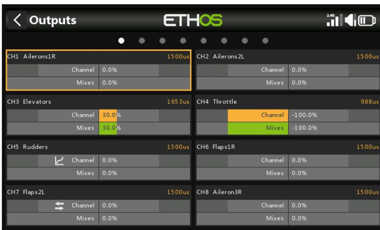
The Outputs screen shows two bar graphs for each channel. The lower (green) bar shows the value of the mixes for the channel, while the upper (orange) bar shows the actual value (in both % and  $\mu\text{s}$  terms) of the Output after the Outputs processing, which is what is sent to the receiver. In the example above you can see that both the mixes and output values for CH4 Throttle are at -100%.
