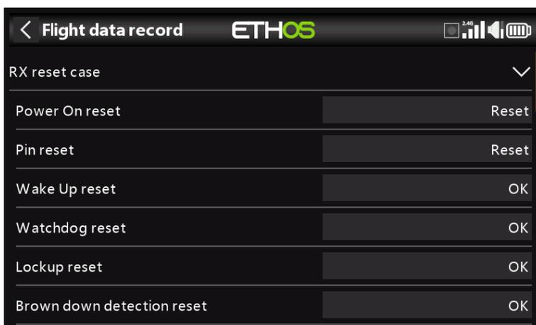
Provides a log of receiver health, including power on reset, output pins reset, and results of wakeup, watchdog timer, lockup detection and power brown out detection.
