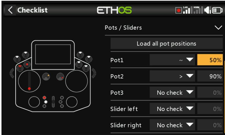
Defines whether the radio requests the pots and sliders to be in predefined positions at startup. The desired pot values can be entered for each pot.
