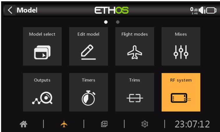
This section is used to configure internal and/or external RF modules, including the 'Owner registration ID'.
