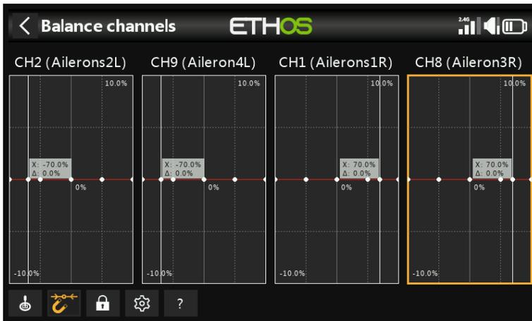
Up to 4 channels may be balanced simultaneously.
