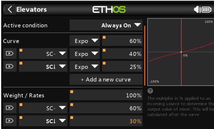
In a similar way to the Ailerons, we can set up triple rates and expo for the Elevator and Rudder on switch SC.
