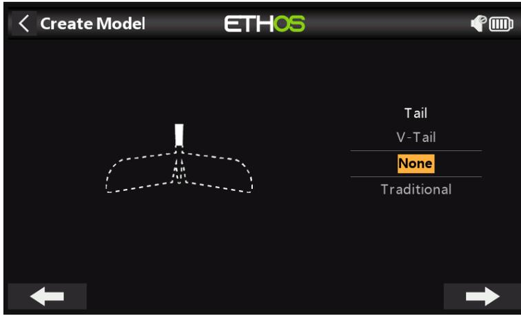
Select 'None' for the Tail. This will create an elevon mix using Aileron and Elevator inputs.
