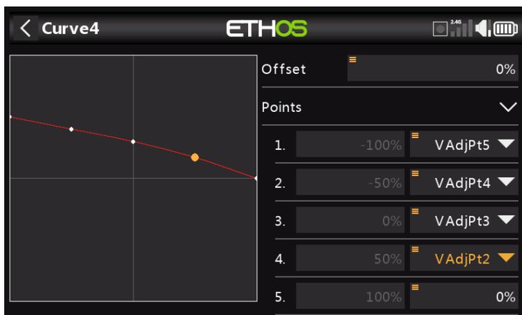
Starting from the right, point number 5 is always zero, which means that no compensation is applied when the flap stick is fully up (at +100%) and no flaps are deployed.
