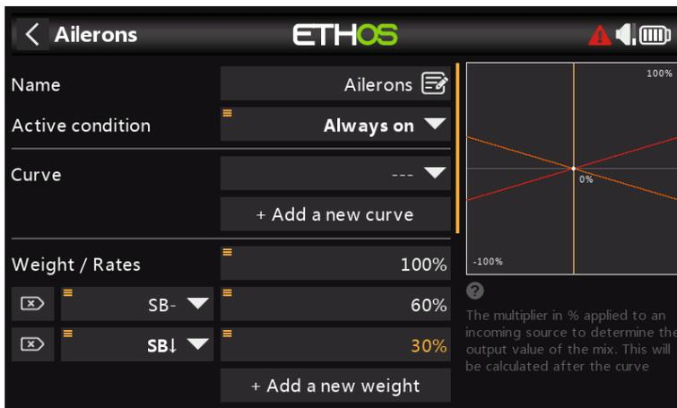
Click on 'Add a new weight', and set up a 30% Rate for switch SB in the down position. The vertical axis in the graph on the right now shows that only 30% of throw is available in this switch position.
