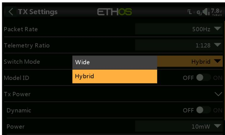
The Switch Mode setting controls how the AUX channels AUX1-AUX8 (channel 5 to 12) are sent to the receiver. The first 4 main channels are always 10-bit. The options are Hybrid & Wide.
