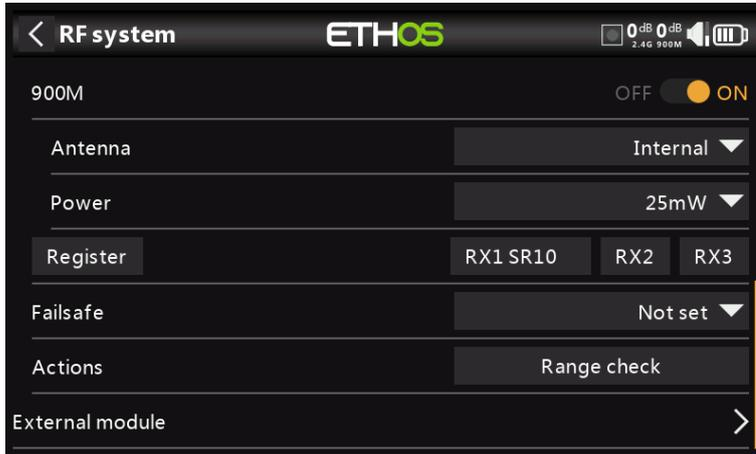
2. Enable the 900M internal RF module.
