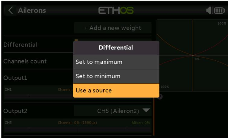
However, you can assign the differential to a pot, allowing you to optimize the value in flight. Long press Enter to bring up the Options dialog, and select 'Use a source'.
