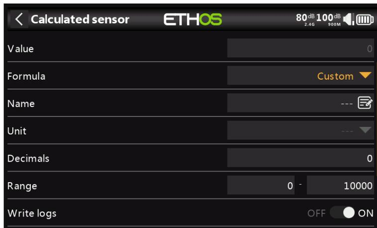
The Custom calculated sensor allows a user defined sensor to be calculated from multiple sources.
