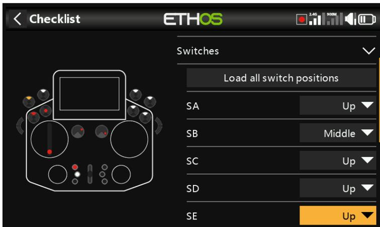
For each switch, you can define whether the radio requests that switches to be in the desired predefined positions. If switches have been given user defined names in System / Hardware / 'Switches settings', the names will be displayed.
