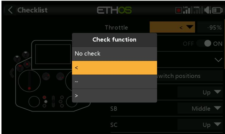
To enable throttle check, select the operator to be used. The options are '<' less than, '~' approximately equal, or '>' greater than. The preflight check will warn you if the throttle stick is outside of the value set in the value parameter.
