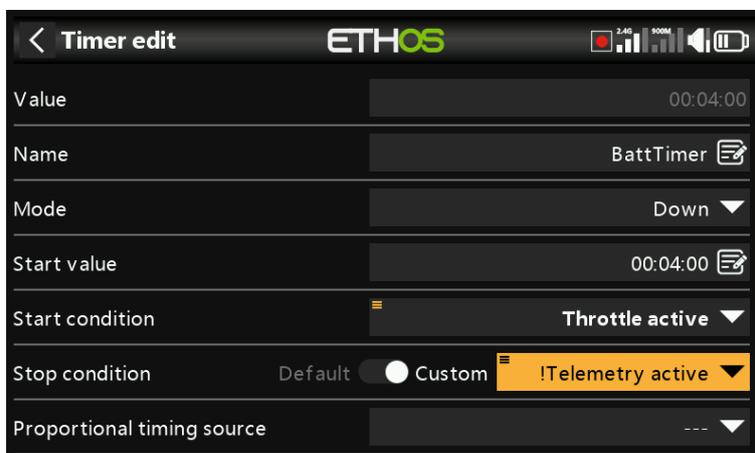
If it is not 'default', once the timer is running, the stop condition controls the timer. The timer stops running while the stop condition is True, but continues running while the stop condition is False.
