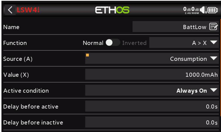
In addition, you can set up another logic switch to trigger a call out of Consumption every 10 seconds once a threshold such as your low limit has been reached. In our example, a threshold of 1000mAh has been set for a 1200mAh LiPo.
