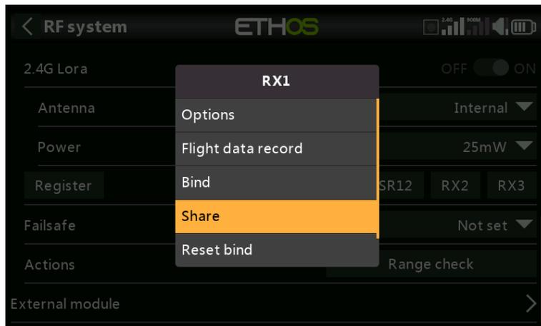
The Share feature provides the ability to move the receiver to another TW mode radio having a different 'Owner registration ID'. When the Share option is tapped, the receiver green LED turns off.
