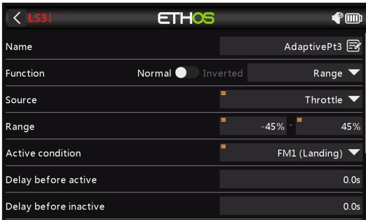
Set up a logic switch AdaptivePt3 with the flap (i.e throttle) stick as source, and a range of -45% to 45%.
