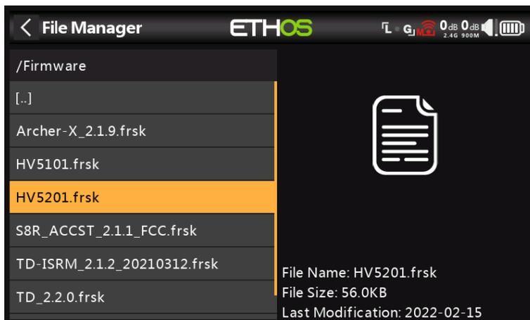
Got to System / File Manager and scroll to the relevant firmware file. In the example above we have chosen the update file for the Xact HV5201 servo. The file date is 2022-02-15, which is for the v2.0.1 version.
