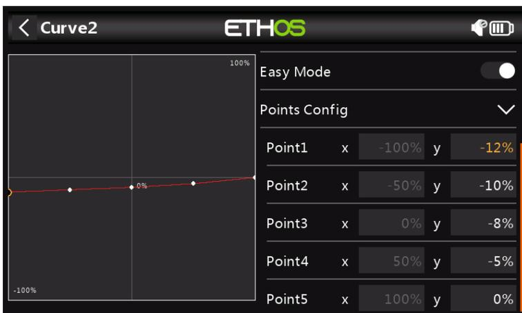
In this example EleComp has initial values of -12%, -10%, -8%, -5% and 0%. If your aircraft does not have an elevator compensation curve specified, these points will need to be determined empirically.
