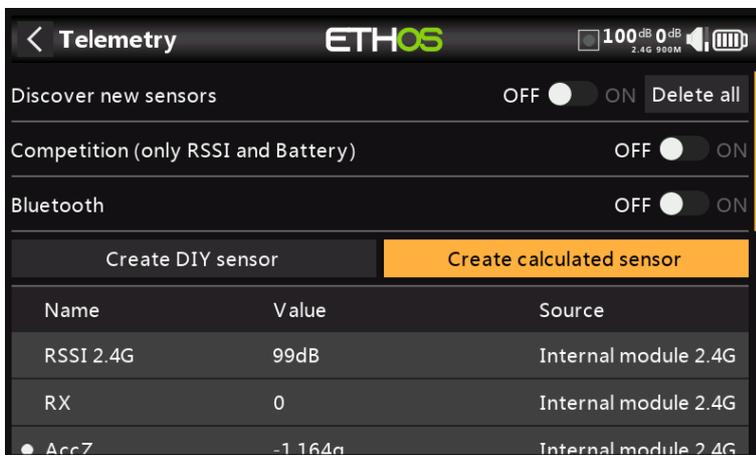
In Telemetry click on 'Create Calculated Sensor'.
