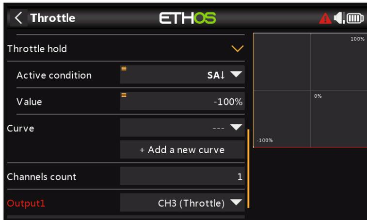
'Throttle hold' is used to cut the motor in an emergency from any throttle position. When the throttle hold active condition is met, the throttle output is instantly reduced to -100% (or the value entered). As can be seen in the graph above, the throttle output has been cut to -100% even though the throttle stick is above the half way mark.)
