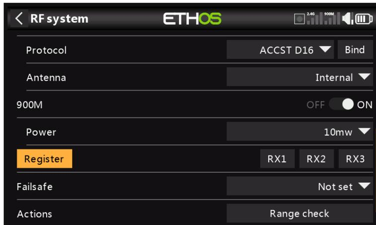
If your receiver has not yet been registered, initiate the registration process by selecting [Register]. The steps are the same as those described in the [ACCESS](#) section.
