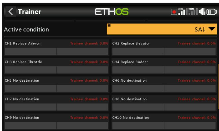
Control of the model can be transferred to the student radio by a switch or button, a function switch, logic switch, trim position, or flight mode.
