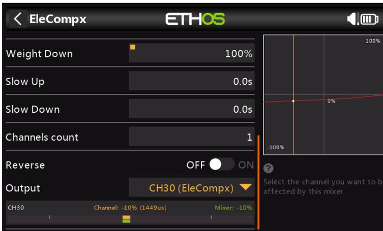
Finally assign the EleCompx mix output to a high channel such as CH30.
