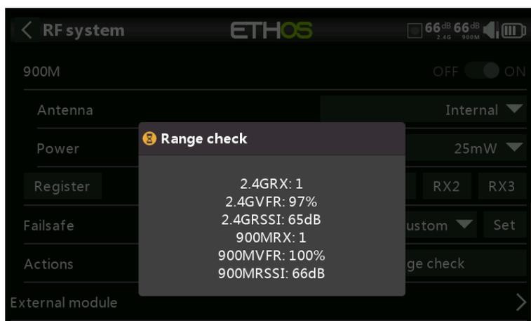
A voice alert will announce 'Range check' every few seconds to confirm that you are in range check mode. A popup will display the receiver number, and the VFR% and RSSI values to evaluate how reception quality is behaving. When the range check is active, it reduces transmitter power, which in turn reduces the range for range testing. Under ideal conditions, with both the radio and receiver at 1m above the ground, you should only get a critical alarm at about 30m apart.
