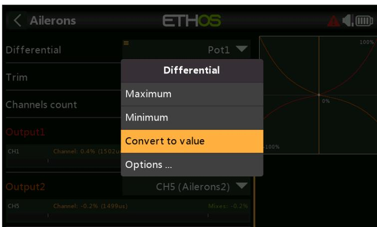
After optimizing aileron differential in flight, you can easily make the pot value your permanent setting. Long press Enter to bring up the Options dialog, and select 'Convert to value'.
