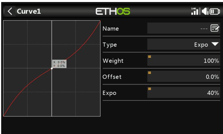
A positive value will soften the response around 0, while a negative value will sharpen the response around 0. Softening the response around mid stick helps to avoid over controlling the model, especially for beginners.
