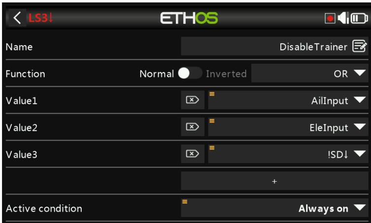
Configure an OR logic switch to become True when either the aileron or the elevator stick is moved, or when the trainer switch SD is switch to the off position (i.e. when switch SD is Not in the down position).
