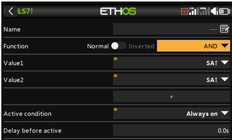
The AND function can have multiple values. The condition is True if **all** the sources selected in Value 1, Value 2 ... Value(n) are true (i.e. ON).
