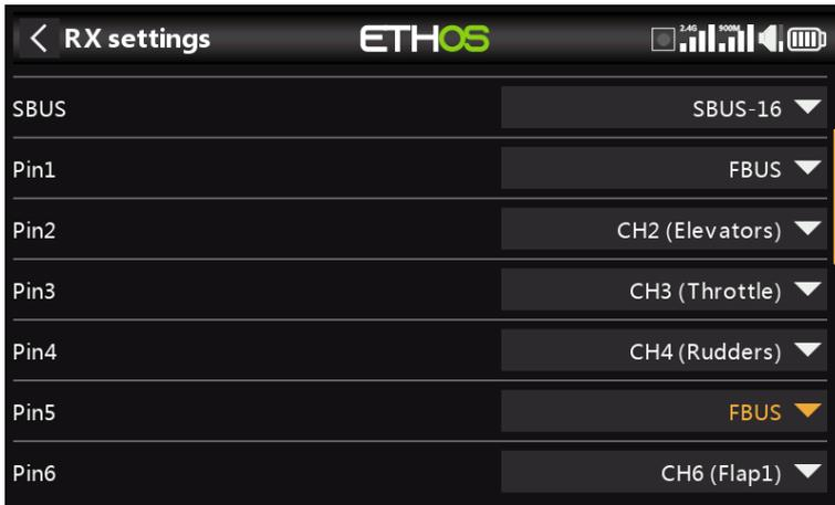
The R18 receiver is now ready to operate two Xact servos plugged into Pin1 and Pin5 via the FBUS protocol. You can reassign as many ports as required to FBUS, which avoids having to use multichannel extenders.
