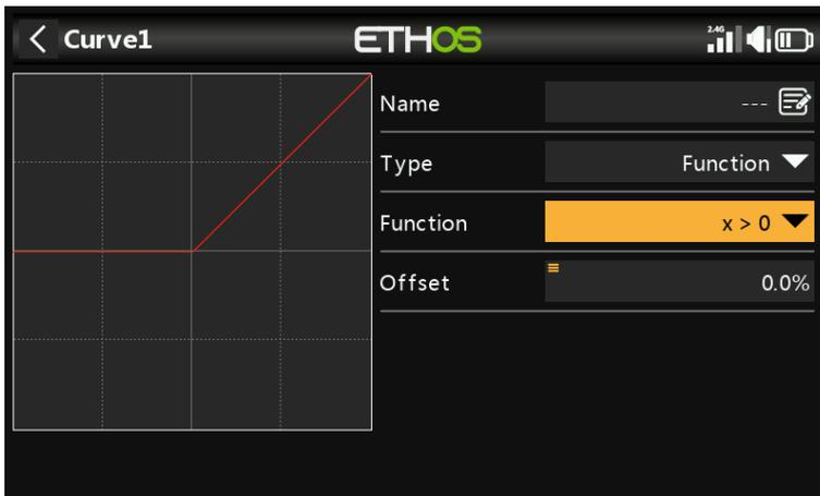
If the source value is positive, then the curve output follows the source.
