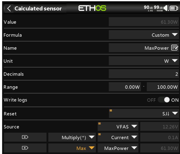
In the simple example above, a voltage sensor VFAS and a current sensor Current have been multiplied to calculate the power. Then a Max function is added by referencing the current value of our custom sensor 'MaxPower' to calculate the maximum value. The Value field shows 61.3W which was the maximum reached during the test.
