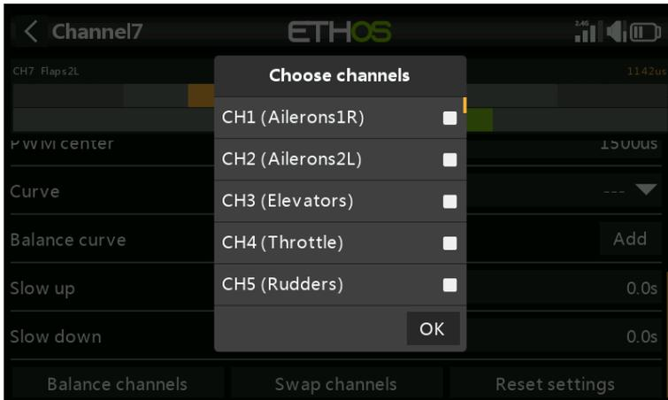
When activated, the channels to be balanced are chosen.
