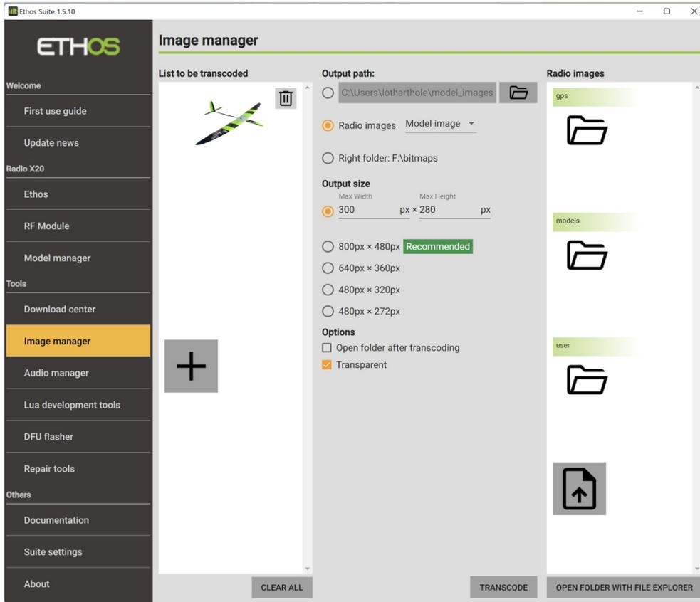
The Image manager can be used to transcode images to the correct size, and to manage the image folders on the radio.
