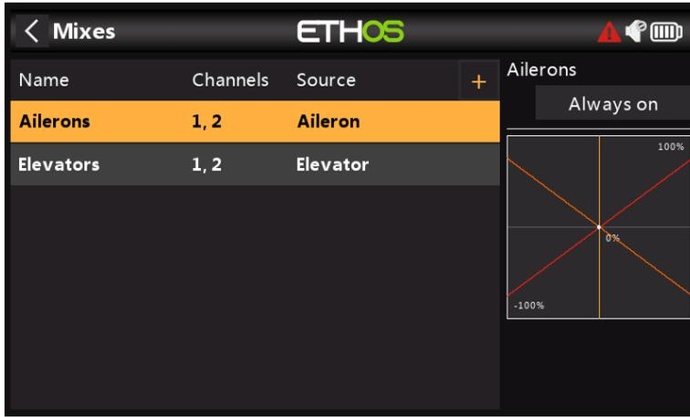
The wizard has created an Ailerons mix on channels 1 and 2, followed by an Elevators mix also on channels 1 and 2. This means both input controls will act on the two elevon channels.
