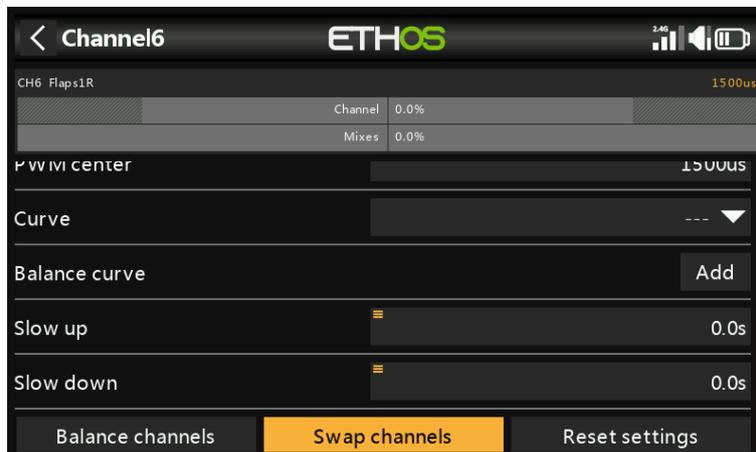
This feature allows two output channels to be swapped.
