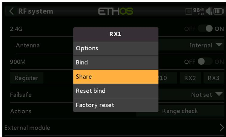
The Share feature provides the ability to move the receiver to another ACCESS radio having a different 'Owner registration ID'. When the Share option is tapped, the receiver green LED turns off.
