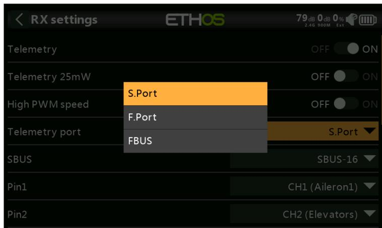
*Port:* Allows selection of the SmartPort on the receiver to use either S.Port, F.Port or the FBUS (F.Port2) protocol. The F.Port protocol was developed with the Betaflight team to integrate the separate SBUS and S.Port signals. FBUS (F.Port2) also enables one Host device to communicate with several Slave devices on the same line. For more information about the port protocol, please refer to the protocol explanation on the official FrSky website.
