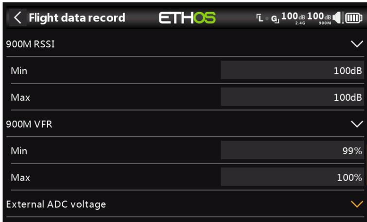
Min and max values of 900M RSSI and VFR (Valid Frame Rate) levels since power up.
