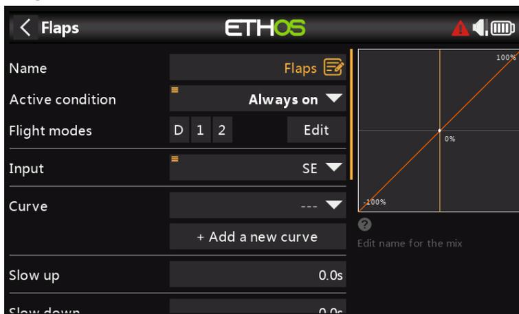
In this example we assign the flaps to switch SE, and increase both output channel weights to 100%.
