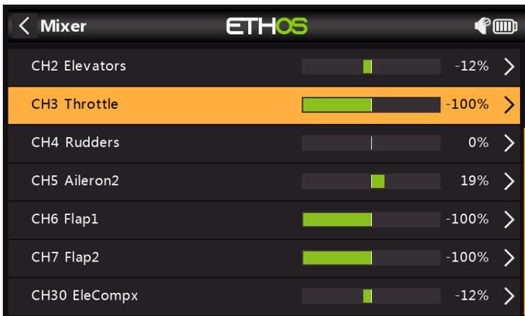
Switching to the 'View by Channel' view allows you to see the effect of moving the throttle stick on all the other channels together, which is much easier for debugging etc.
