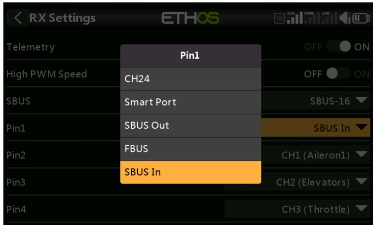
Pin 1 may also be set SBUS IN. Please note in the above example that the channels have been bumped down by one to make room for having SBUS IN on port 1 (CH1 Aileron1 is on pin 2).
