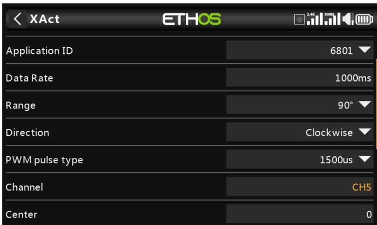
We also need to assign the channel number we want this servo to respond to, in this example CH5. Scroll down and change the Channel to CH5.
