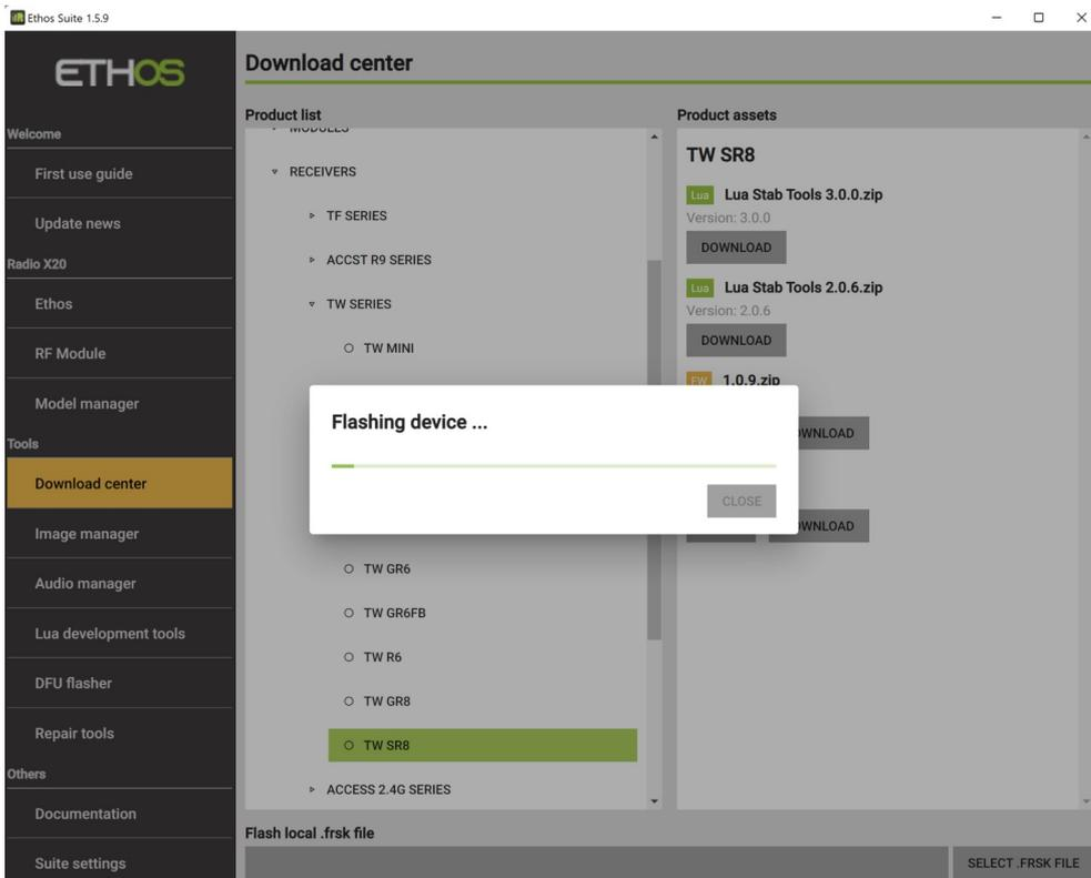
In the example above, after connecting the receiver to the radio via an SPort cable connection, the 'Flash' button was pressed to start flashing the desired firmware version. A 'Flashing device' progress bar appears.
