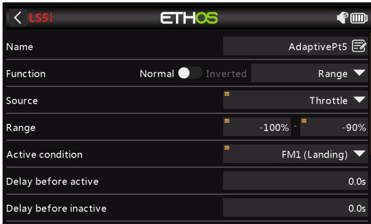
Set up a logic switch AdaptivePt5 with the flap (i.e throttle) stick as source, and a range of -100% to -90%.
