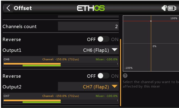
Move the flap stick to the fully deployed position. The screen above shows that the mixer outputs have moved by 180% (i.e. the Weight setting) from +80% down to -100%.
