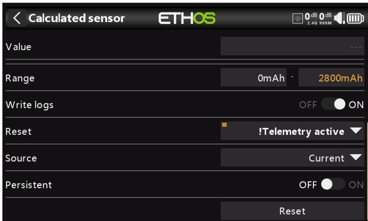
Select a suitable Reset condition, such as system event '!Telemetry Active'. First select 'Telemetry Active', and then long press Enter on it to bring up the option menu, and select 'Invert'. The sensor will be reset when telemetry is lost when the model is switched off.
