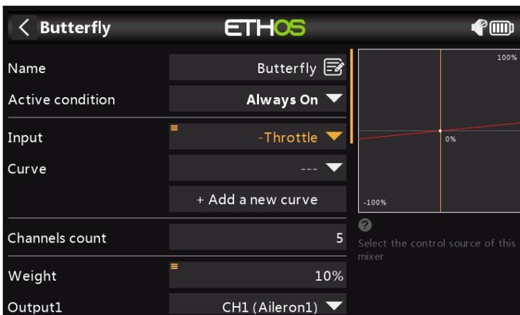
With the Throttle stick fully up, the Input now sits at 0 (see above). The Input parameter now says '-Throttle' to indicate that it has been inverted.
