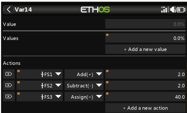
In this example above, function switch FS3(edge) will assign a value of 40% to the Var, and FS1(edge) will increase its value by 2 with every button press until the Range maximum is reached, and FS2(edge) will similarly decrease its value by 2 until the Range minimum is reached. Please note that the edge option must be selected (long press on the FS) so that the action is only performed when the function switch changes state.
