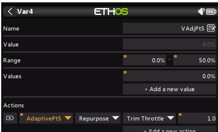
The Var named VAdjPt5 has a range of 0-50% (which should be sufficient for compensation, but may be increased if necessary). It has an action defined to repurpose the throttle trim to adjust the Var's value with a step size of 1.0% when the AdaptivePt5 logic switch defined in step 4 above is active.
