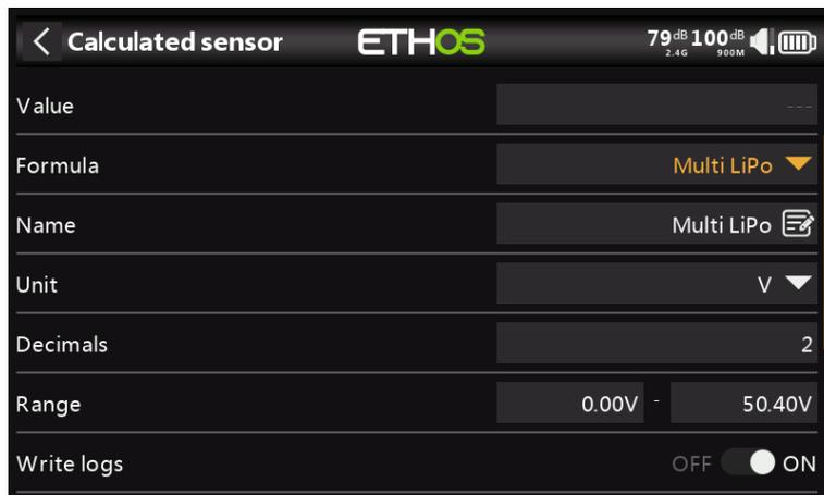
The Multi Lipo calculated sensor allows two lipo sensors to be cascaded for monitoring lipos greater than 6S.
