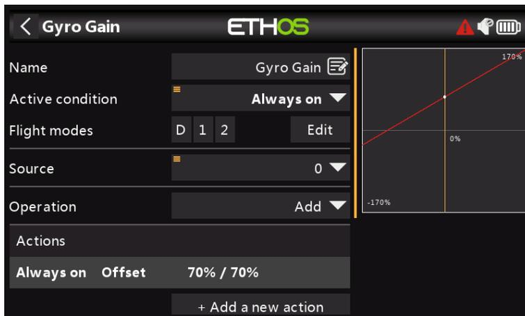
Gyro Gain is typically a fixed value, so we set the Source to Special Value – 0, and then dial up the required gain value using Offset. The final gain value may need to be determined in flight. Assign the Output channel to 5.
