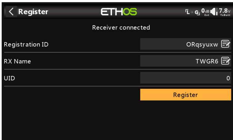
The 'Waiting...!' message changes to 'Receiver Connected', and Rx Name field will be filled in automatically.
