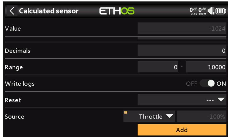
With the throttle at -100%, we can see that the internal value is at -1024. So the internal value of a source is between +/-1024 when the source is +/-100%.
