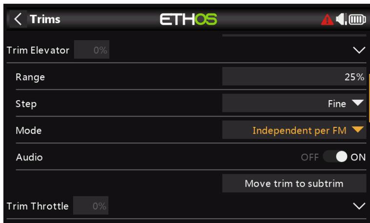
Next we go the Trims section, and change the Elevator stick to have 'Independent trims per flight mode'. This then allows you to have independent elevator compensation for the two flaps deployed settings. The Elevator Trim Switch will automatically switching between the settings as you operate the flaps on switch SE.
