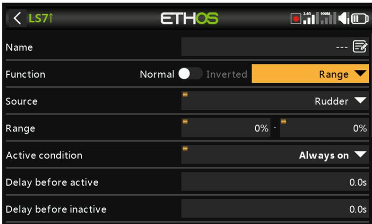
The condition is True if the value of the selected source 'A' is within the range specified.
