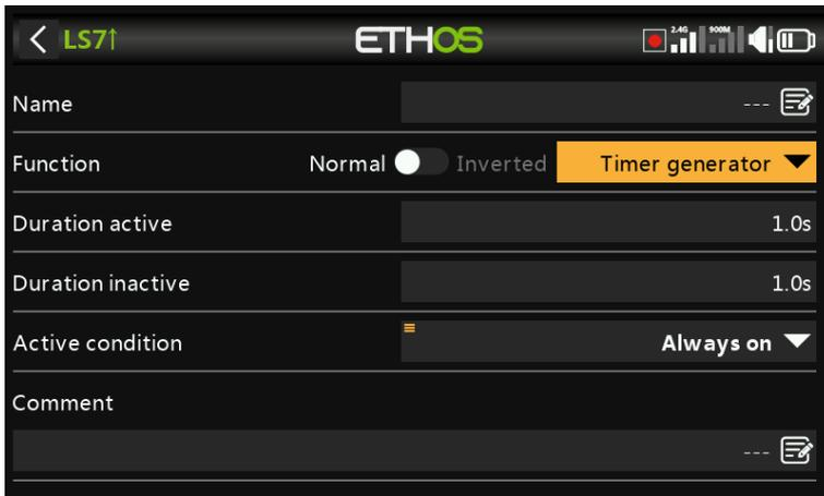
The logical switch toggles on and off continuously. It switches on for time 'Duration active', and off for time 'Duration inactive'.
