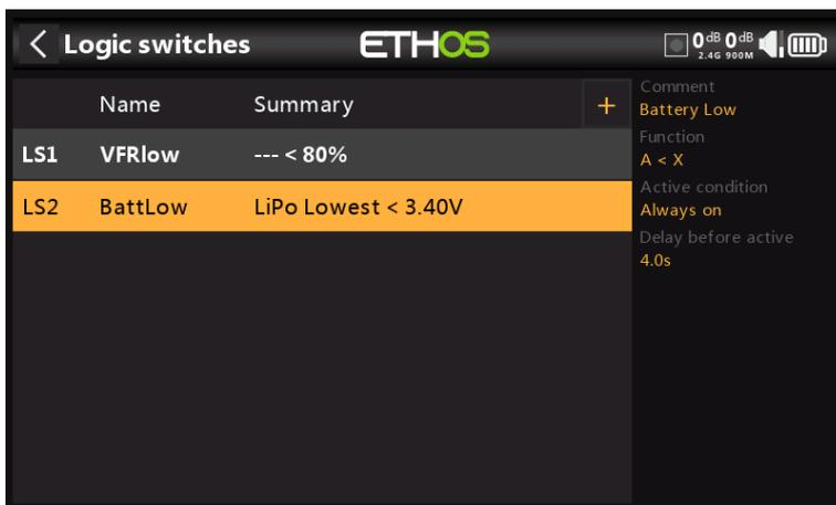
The completed Logical Switch for battery low is shown above.
