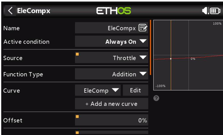
Next we define a high mix which will convert our compensation curve into a variable value suitable as a weight in the Butterfly mix. Use a Free Mix, with throttle as source and attach the curve EleComp. Let's call it EleCompx.
