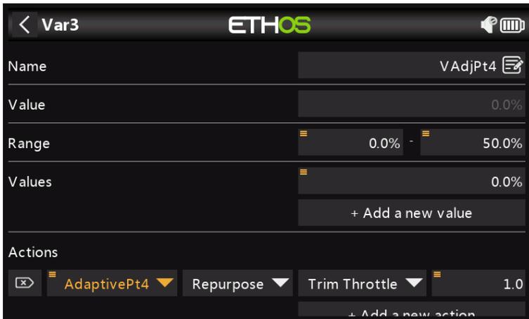
The Var named VAdjPt4 has a range of 0-50% (which should be sufficient for compensation, but may be increased if necessary). It has an action defined to repurpose the throttle trim to adjust the Var's value with a step size of 1.0% when the AdaptivePt4 logic switch defined in step 4 above is active. (Note: It will be active when the flap control has a value between -90% and -20%.)
