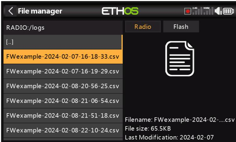
To view log files, navigate to the /Logs folder on eMMC or the SD card with File Explorer, then tap on the desired log file and select open.
