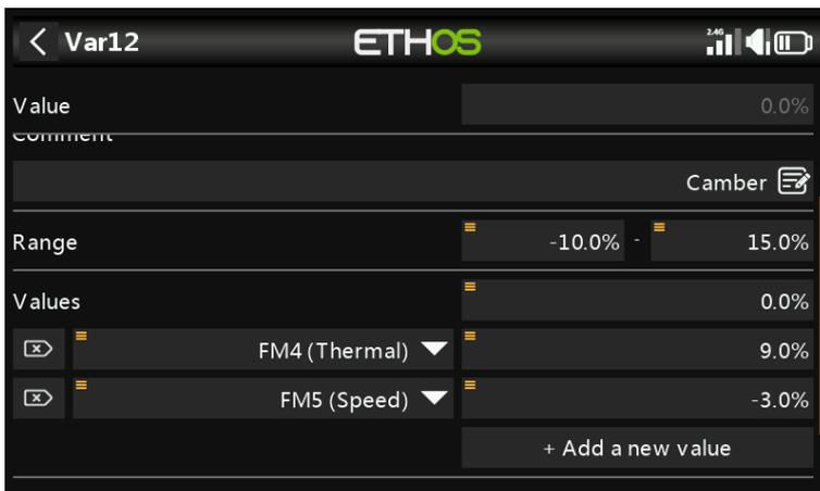
Each Var can hold multiple values depending upon the active conditions (such as flight modes) configured. In the example above, while the Thermal flight mode FM4 is active, Var12 has a value of 9%. When the Speed flight mode FM5 is active, Var12 will have a value of -3%.
