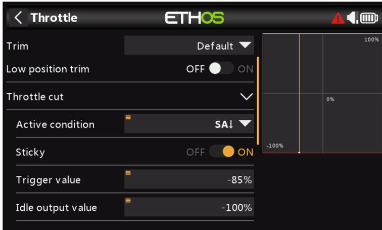
However, if the 'Sticky' is enabled, then the throttle will be cut the instant switch SA goes down, as shown in the example above.
