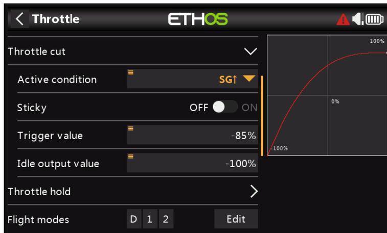
If we assign switch SG-up to the Throttle Cut function and it's Sticky to 'ON', then the throttle will be cut as soon as you flip the switch to the 'Up' position. However, due to the Sticky setting the throttle can only be armed with the throttle stick in the low (off) position.
