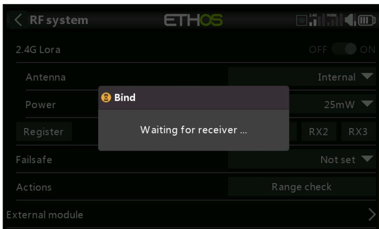
4. Power up the receiver without touching the F/S bind button. A message box will pop up 'Select device' and the name of the receiver you have just powered on.
