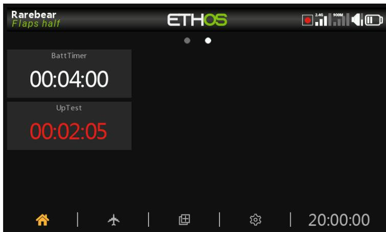
If the timer has been set to count Up, the alarm value parameter sets the value at which the timer elapses. The timer continues to count, but the value goes red in the timer widgets.
