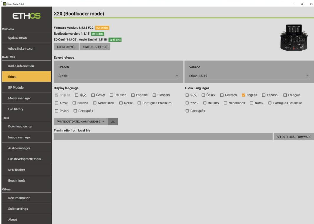
The example above shows that an X20 is connected in Bootloader Mode, which allows the radio to be updated.
