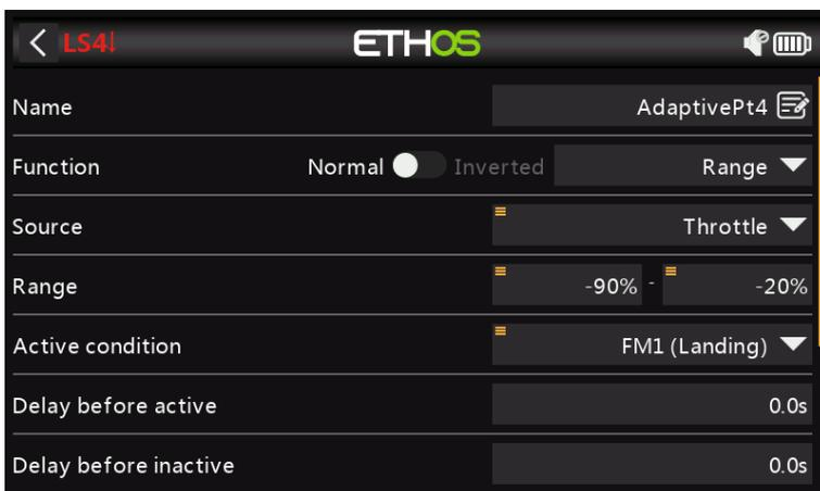
Set up a logic switch AdaptivePt4 with the flap (i.e throttle) stick as source, and a range of -90% to -20%.
