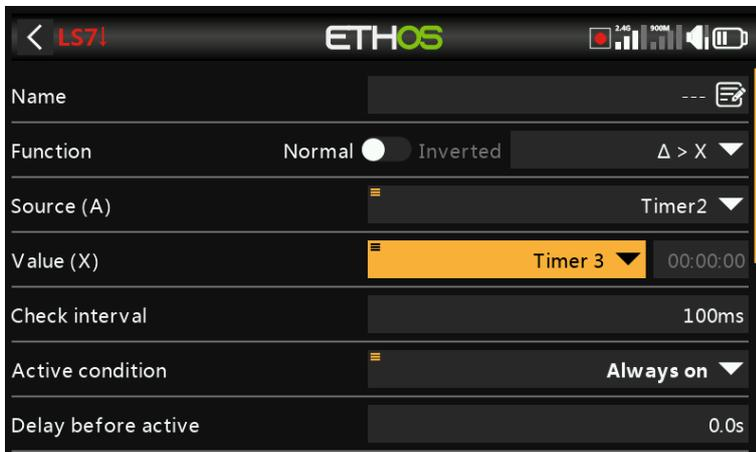
Normally source (A) is compared to a fixed Value (X). However, comparison of two same-format (i.e. having the same units) sources is allowed. For example, two timers, or two voltages, or two RPM sources may be compared.
