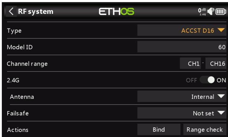
Mode ACCST D16 is for the ACCST 16ch two-way full duplex transmission, also known as the "X"-mode. For use with the legacy "X" series receivers.
