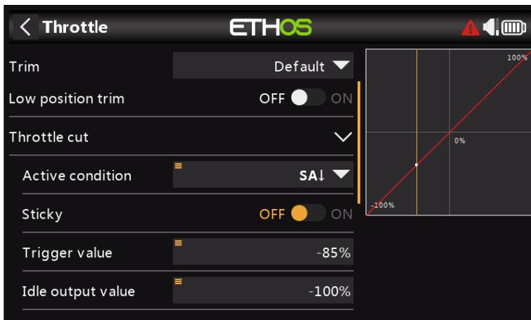
Throttle cut provides a throttle safety latching mechanism. Once the active condition has been satisfied in our example with switch SA in the down position (switch SA down is shown in bold to indicate that it is active), the throttle output will be held at -100%
