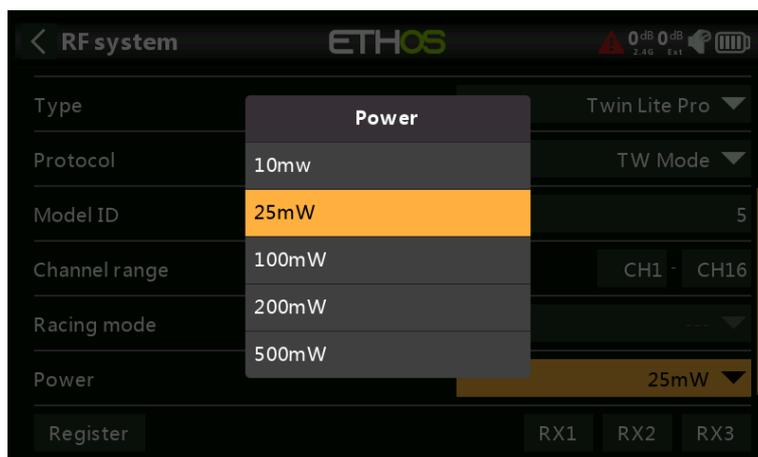
Select the RF Power desired between 10, 25, 100, 200, 500mW.
