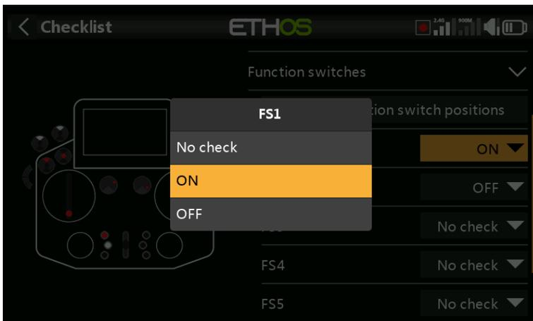
For each function switch, you can define whether the radio requests that switches to be in the desired predefined positions. The options are shown above.
