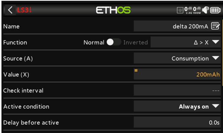
Add a new Logical Switch using the Delta ( $d>X$ ) function to monitor the Consumption sensor, and become True/Active every time the consumption reaches say 200mAh, or a convenient fraction of the battery capacity.
