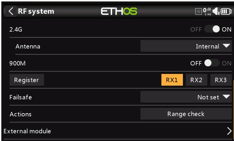
3. Receiver 1 [Bind]: Initiate the binding process by selecting [RX1], then select Bind from the drop-down list.
