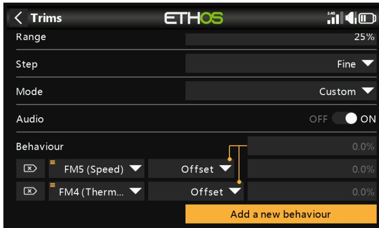
Similar to the first, we configure the second behavior as 'Offset + Default' with condition 'FM4(Thermal)'. When FM4(Thermal) mode is selected, any trim adjustments will be saved as an offset to the base mode trim value in FM0(Cruise). Therefore the trim in FM4(Thermal) will be separate but also dependent on the base trim.
