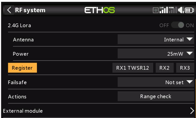
3. If your receiver has not yet been registered, initiate the registration process by selecting [Register]. Otherwise, skip down to the Bind section.
