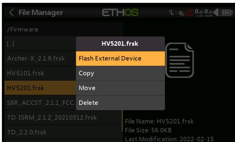
Plug the servo lead into the S.Port connection at the top of the radio. The white or yellow lead goes to the side with a notch. Tap on the highlighted filename, and select 'Flash External Device'. Flashing will commence, with a bar chart showing progress.
