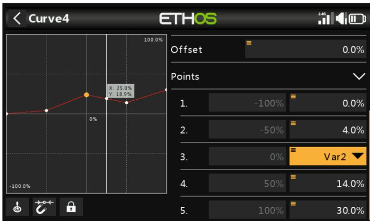
In this example above the middle curve point is being driven by a Var, which again could be adjusted in flight by a reassigned Trim. Please refer to the [VARs](#) section for more details.
