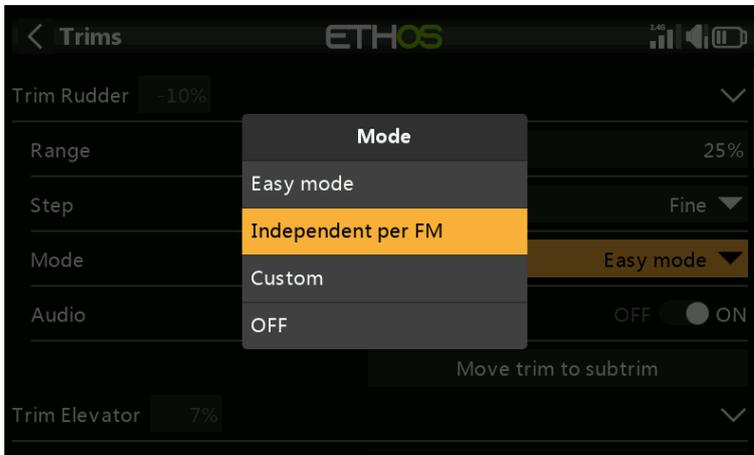
With the 'Independent trim per flight mode' option, the trim affects the active flight mode only. This option is normally used for the elevator trim, since the elevator trim required will typically vary for each flight mode due for example to differences in wing camber. In fact, this is often the main reason for implementing flight modes!
