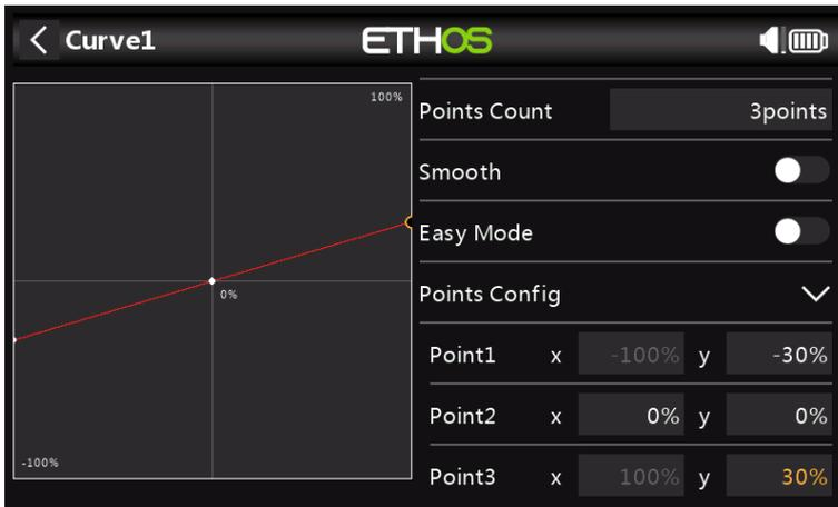
It is a good idea to use +/- 30% initially, and then adjust the curve to suit the servo and linkages with the model powered up. This should ensure that the servo will not be driven beyond its mechanical limits, which would overload the servo and lead to failure. The curve midpoint is edited to achieve the surface neutral position.
