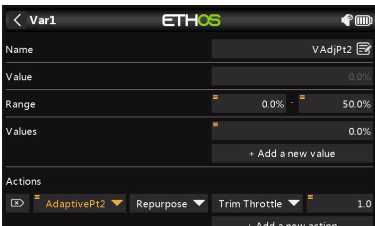
The Var named VAdjPt2 has a range of 0-50% (which should be sufficient for compensation, but may be increased if necessary). It has an action defined to repurpose the throttle trim to adjust the Var’s value with a step size of 1.0% when the AdaptivePt2 logic switch defined in step 4 above is active. (Note: It will be active when the flap control has a value between 20% and 90%.)
