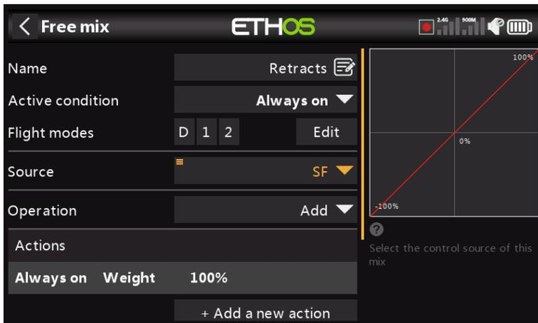
For this example name the Free Mix as 'Retracts'. The mix can always be on, and the Source can be switch SF.
