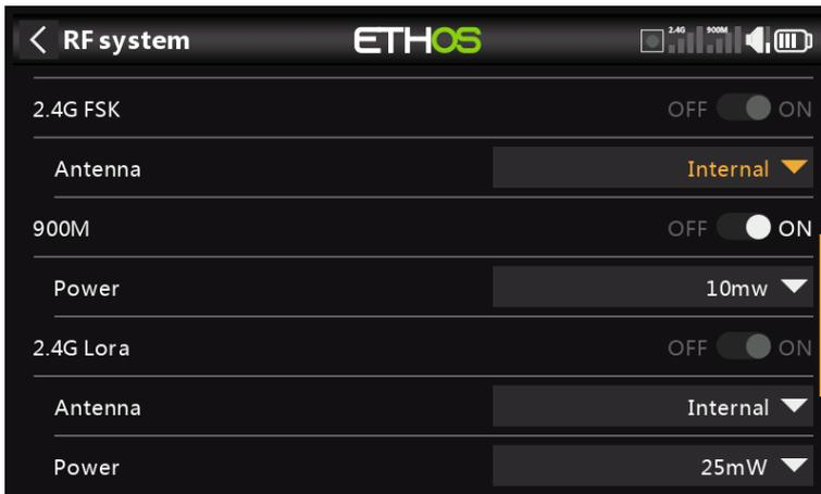
2. Enable the 900M internal RF module. Note that the 900M RF module operates on the internal antenna only.
