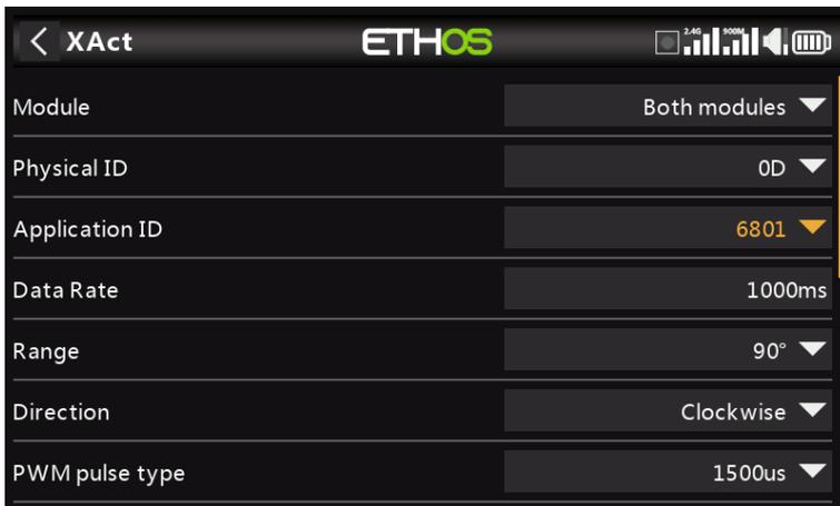
For the second servo we need to change the default Physical ID of 0C to an unused slot, please refer to the [Physical ID table](#) in the Telemetry section. We will choose 0D hex for this example.
