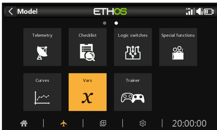
Variables (Vars) can be used to name and store a model's settings parameters in a way which can then be referenced elsewhere in the radio programming including the mixes. Vars can be thought of as containers that hold information.
