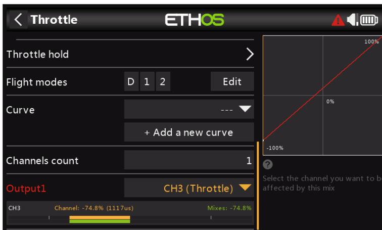
For glow and gas we use 'Low position trim' to adjust the idle speed. The idle speed can vary depending on the weather, etc., so having a way to adjust the idle speed without impacting the full throttle position is important.
