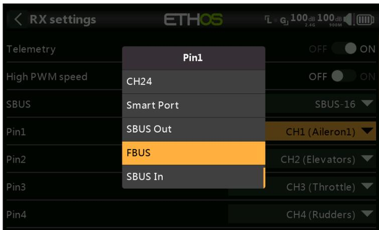
*Pin1 to Pin(nn)*: The receiver Options dialog also gives the ability to Remap channels to the receiver pins. In addition, each output port may be reassigned to Smart Port, SBUS Out, or FBUS (previously known as F.Port2) protocols. Additionally, output port 1 may be reassigned as an SBUS In port.
