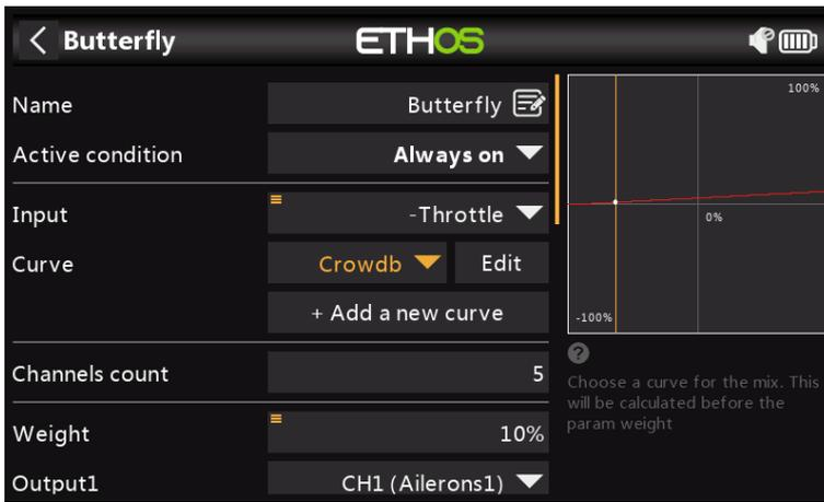
The throttle input now has a dead band applied to it.
