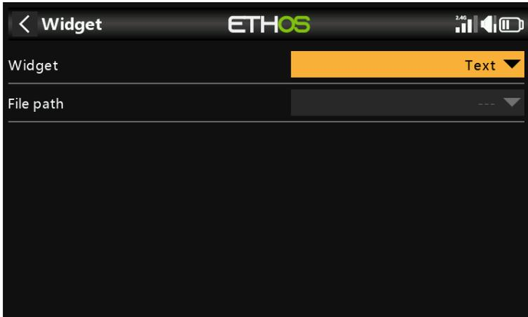
The text widget will display the contents of a text file. The markdown format is supported.
