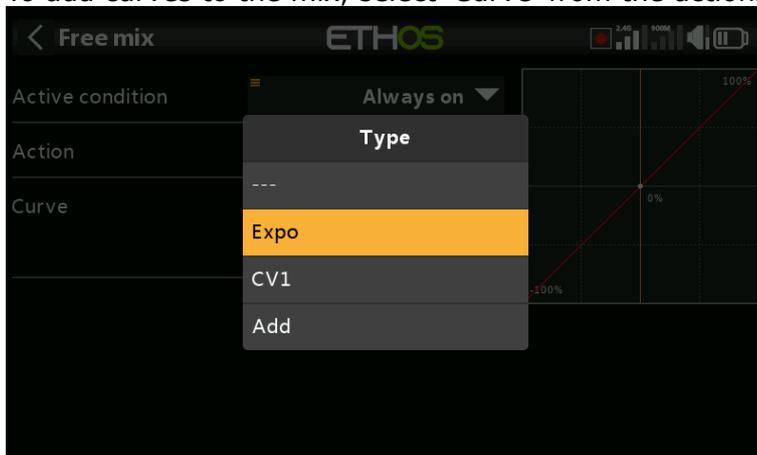
A standard curve option is Expo, which by default has a value of 0, which means the response is linear (i.e. no curve). A positive value will soften the response around 0, while a negative value will sharpen the response.
