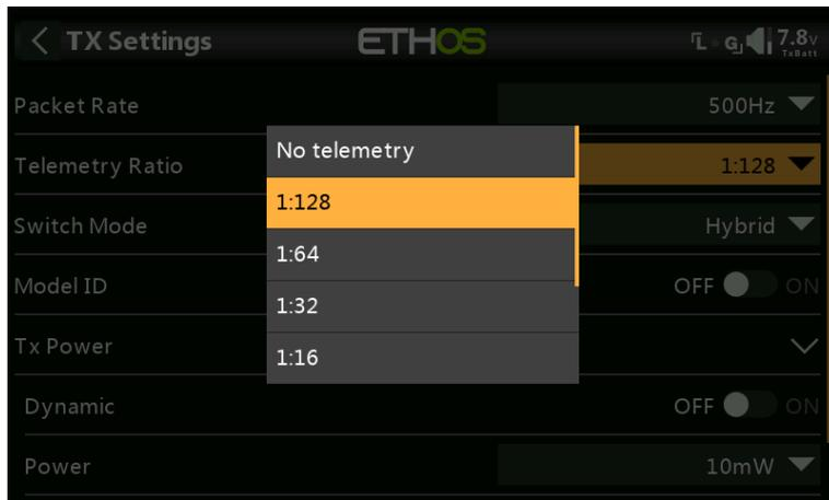
The Telemetry Ratio determines how often telemetry data is sent. For example, 1:64 means telemetry data is sent every 64 frames. The options are 1:128, 1:64, 1:32, 1:16, 1:8, 1:4 and 1:1.
