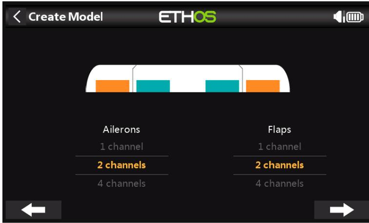
Accept the default 2 channels for Ailerons, and select 2 channels for Flaps.
