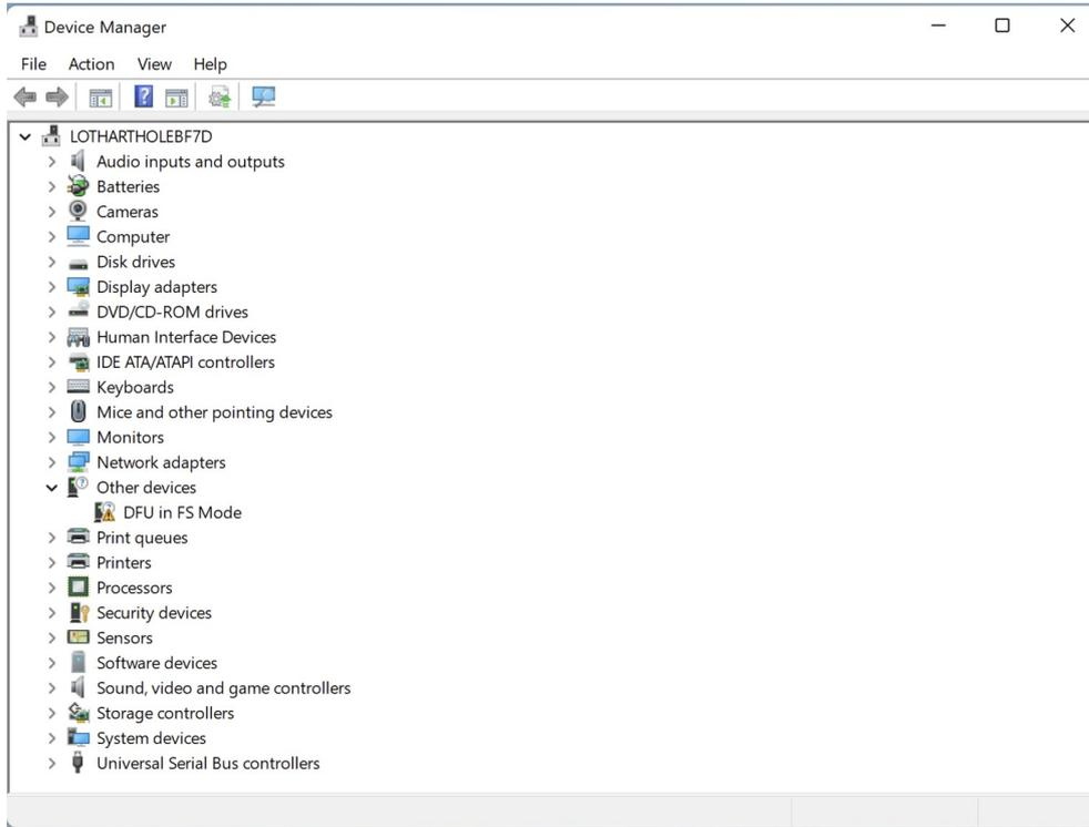
Check Device Manager to see if your DFU device (i.e. your radio) is recognized and working. In this situation programs like the Impulse Driver Fixer can be used to correct the driver. It can be downloaded from <https://impulserc.com/pages/downloads>. For more information please see also this [Ethos Suite Update](#) post.
