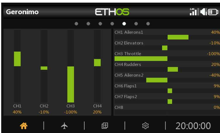
The example above shows two Channels widgets, the left one showing 4 channels vertically, while the right one shows 8 channels horizontally.
