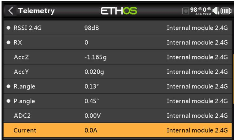
Connect the telemetry port of the FASxxx current sensor to your receiver via an S.Port cable, and enable the 'Discover new sensors' option in Model / Telemetry. The additional sensors include 'Current' as shown in the example above.
