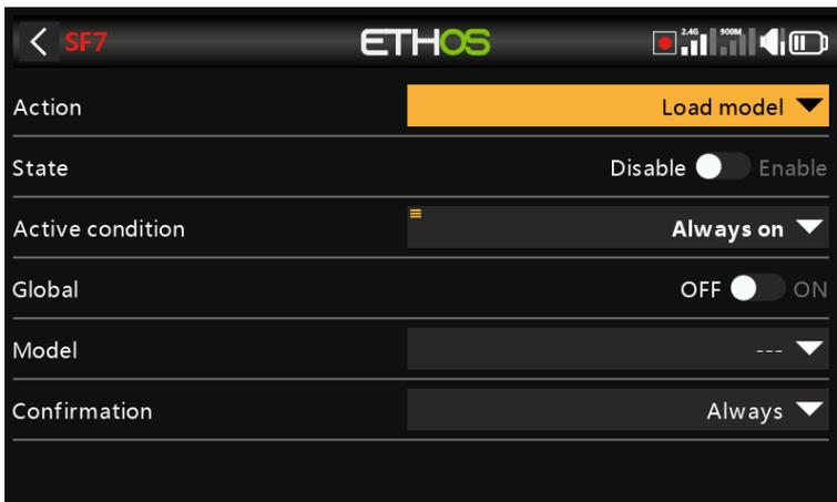
This special function will load a specified model when the 'Active condition' is met.
