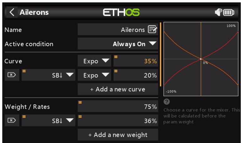
In the Rates examples above you can see that the output response is linear. To avoid the response being too twitchy at the stick centers, you can use an Expo curve to reduce the control surface movement at center stick and to increase it as the stick moves further from center. The Weasel recommended Expo values are 35% for high and 20% for low, so we will add a curve that will be active on the SB switch down position. The graph now shows a curved response which is flatter at stick center.
