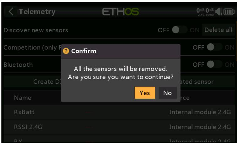
Turning this mode on will delete all sensors except RSSI and RxBatt. The radio must be power cycled before sensors can be rediscovered with this setting in the off position.
