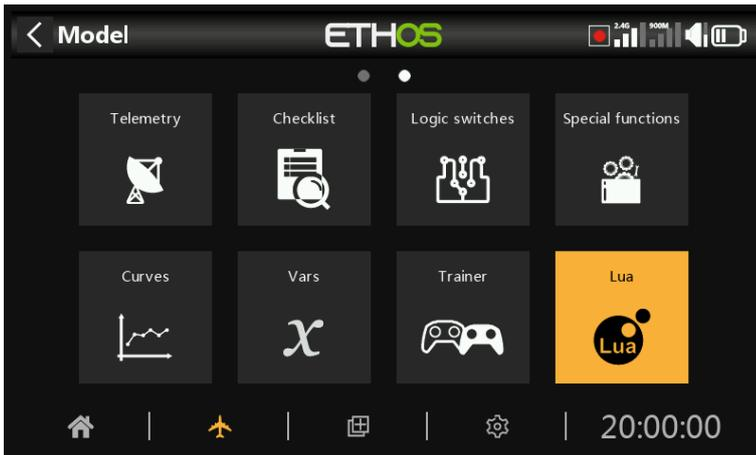
This page is used to manage Lua sources and tasks on a per-model basis. This icon only appears if the radio finds task or source Lua scripts in the scripts folder at startup.
