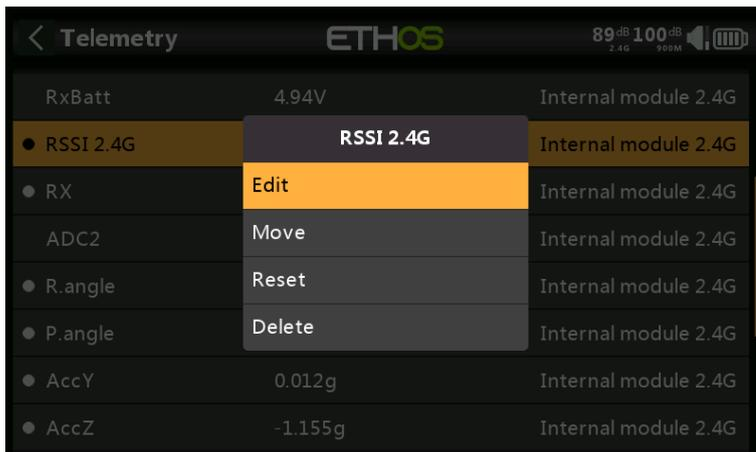
Tap on a sensor, then select 'Edit' from the popup dialog to edit the sensor settings. Alternatively select 'Move' to reorder sensors, 'Reset' to reset the sensor or 'Delete' to remove it.
