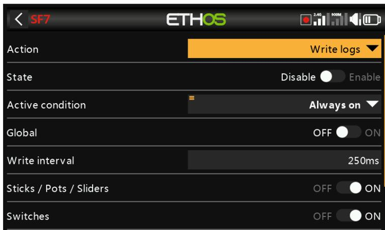
Log files are stored in a '.csv' format in the 'Logs' folder on the SD card or eMMC. The RTC time and date are logged with the data, and are important to make sense of the data by separating the log data into sessions.
