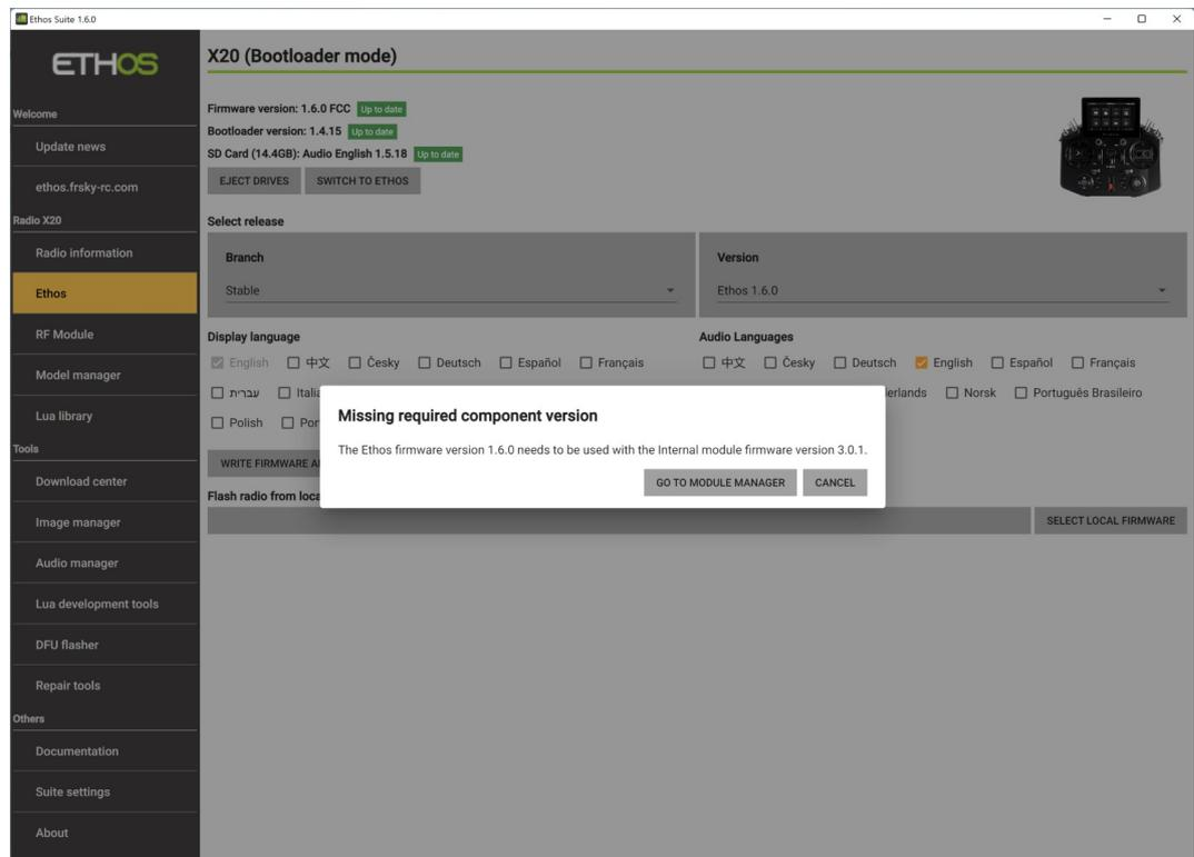
If your internal RF module is not on version 3.0.1 or later, you will need to upgrade the RF module before you will be able to continue to install 1.6.0 or later.
