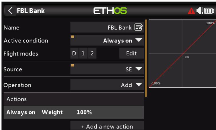
The Spirit FBL unit has three settings Banks that can be used to set up different configurations. The Bank switching is great for switching between flight styles, different sensor gains for low or high RPMs, or for Beginner, Acro or 3D. Alternatively it can be used just for tuning your settings.
