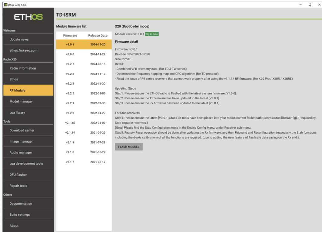
Ethos v1.6.0 or above requires a mandatory upgrade of the internal RF module to v3.0.1. This occurs automatically when clicking on 'Go to Module manager' during the firmware upgrade to Ethos 1.6.0, see above.
