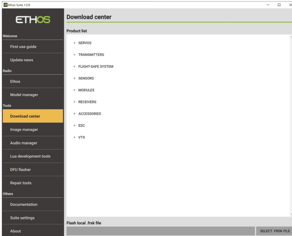
The download centre can be used to download any firmware from the FrSky download site, and to use the radio as a proxy to flash any module, sensor, servo, or receiver directly from Ethos Suite.
