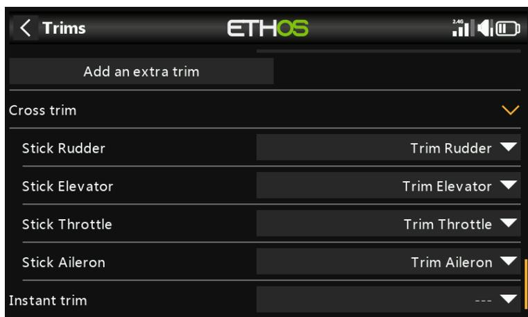
Cross trims can be set up for each trim stick, so you can nominate which trim switch to use for each stick. (The T5 and T6 trims are available on the X20 Pro and X18 only.)
