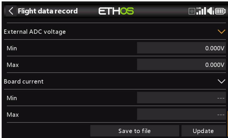
Min and max values of the AIN analog input port, and the receiver board current since power up.
