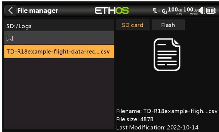
Tap on 'Save to file' to save the data to a .csv file in the Logs folder. The file can be read by a text editor or more conveniently by for example LibreOffice.
