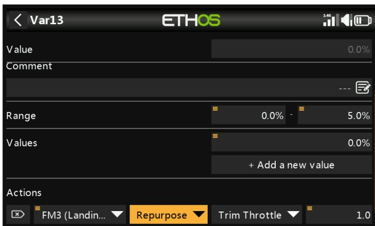
In the example above, an action has been defined to repurpose the Throttle trim for camber compensation during the Landing flight mode FM3 only. A range of 0 - 25% has been set to keep the Var between reasonable limits. A trim step value to one decimal may be defined, e.g. 1.0% in the example above.
