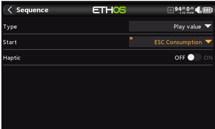
Under 'Sequence' add a 'Play value' command to speak the value of the ESC Consumption telemetry sensor.
