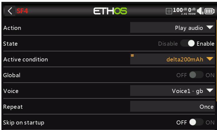
Add a 'Play audio' special function call up our 'delta200mAh' logic switch to speak the value of Consumption every time the logic switch becomes True.
