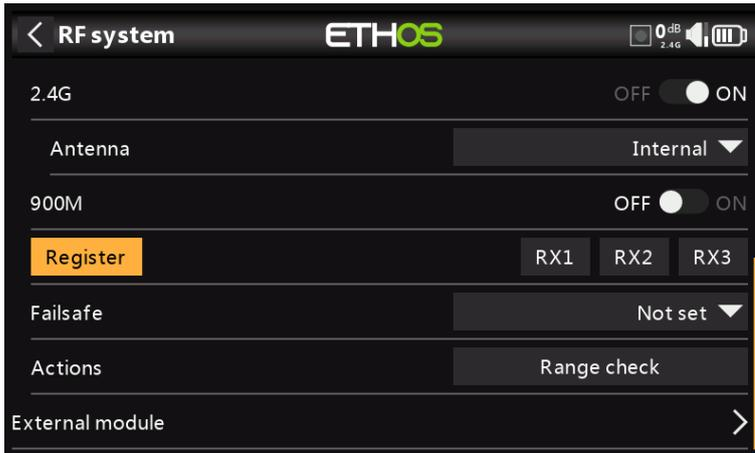
1. If your receiver has not yet been registered, initiate the registration process by selecting [Register]. Otherwise, skip down to the Bind section.
