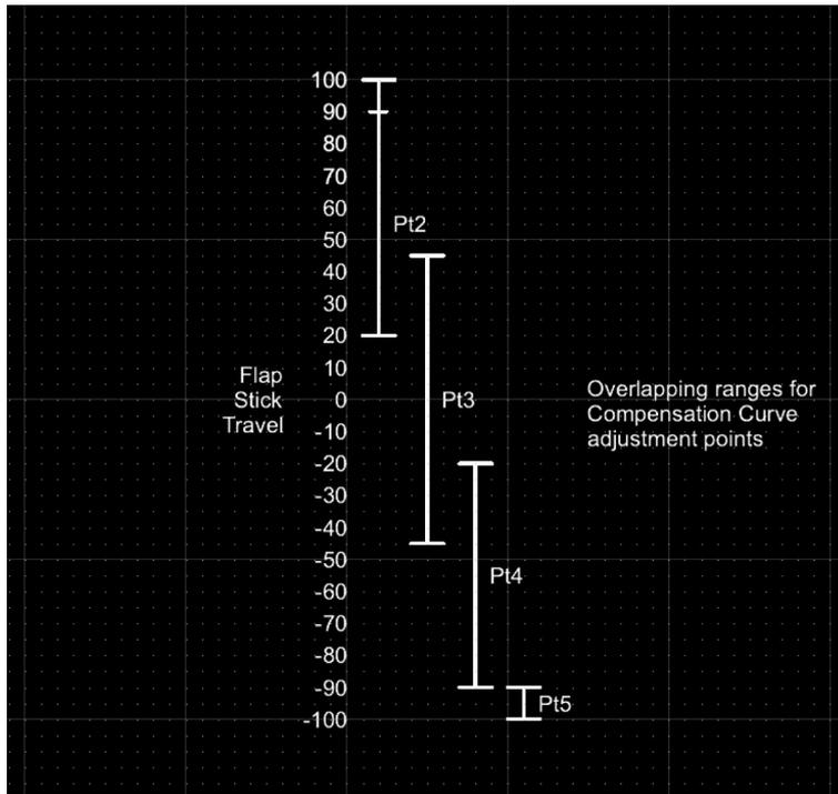
Please refer to the above diagram for the overlapping ranges chosen for the compensation curve adjustment points. These ranges were defined by Mike Shellim for his 'Crow-aware adaptive elevator trim' developed for OpenTX (see rc-soar.com) and are used with his kind permission.
