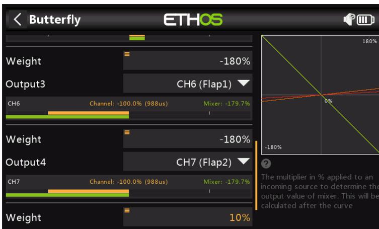
Flaps are unusual in that a very large downward deflection is needed, with very little or no upward movement. This may be achieved by sacrificing some upward travel in favor of downward travel. In practice the flap servo horns may be offset from neutral by say 20 or 30 degrees.
