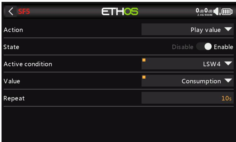
Set up a special function to play the value of Consumption every 10 seconds once LSW4 triggers when the 1000mAh threshold has been reached.
