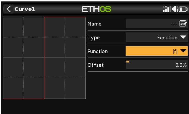
If the source value is negative, then the curve output is -100%.
