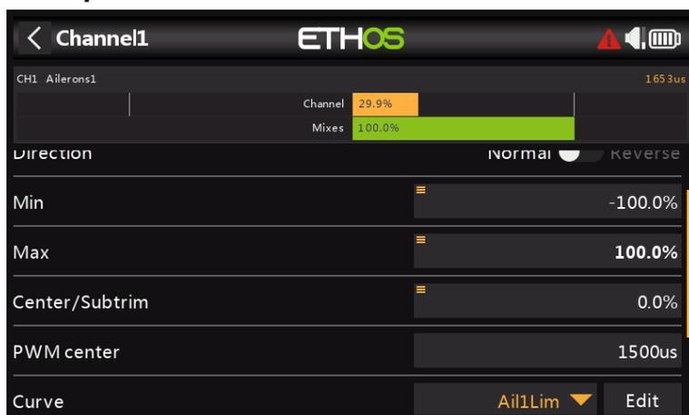
Start by adjusting the servo center points using the PPM Center adjustment, after optimizing the mechanical linkages.
