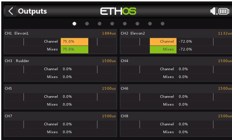
The example above shows that full right aileron has been applied, so channel 1 is at 75%, while the left down-going aileron is at 72% due to aileron differential.
