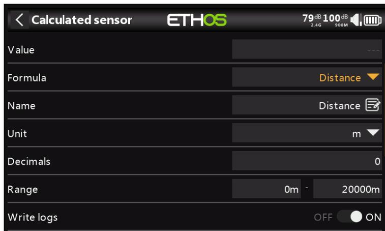
The Distance calculated sensor allows the distance traveled to be calculated from a GPS sensor.
