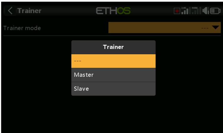
The Trainer function can be configured as master or slave. In master mode, up to 16 controls may be transferred from the student radio to the master radio when the 'Active condition' set above is active. In slave mode a configurable number of channels are transferred to the master.
