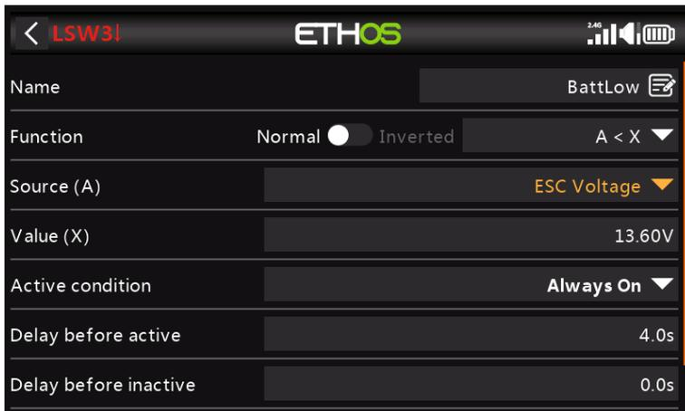
Add a new Logical Switch to monitor the 'ESC Voltage', and to become True/Active when the 'ESC Voltage' voltage remains below 3.4 per cell for 4 seconds. In the example a 4S LiPo is being monitored, so the threshold is set to  $3.4 \times 4 = 13.6V$ . A threshold of 3.4V under load will recover to around 3.7V when no longer under load.
