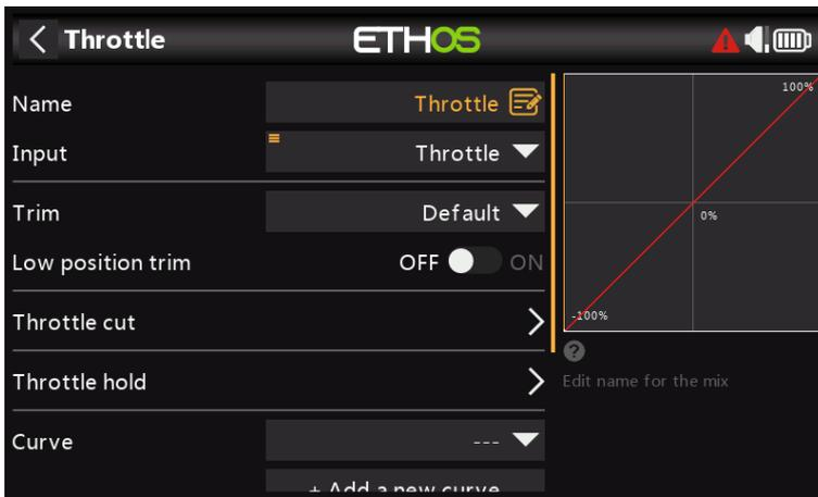
For the throttle we will leave the Input on the throttle stick. We do not need rates or expo, but we do need a safety switch so that the motor will not start unexpectedly. This is extremely important, because model engines and motors can cause serious injury or death.
