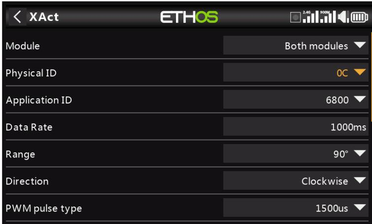
Confirm that the default Physical ID is 0C hex, and the Application ID is 6800 hex. For the first servo we can leave the Physical ID and the Application ID at the default values.
