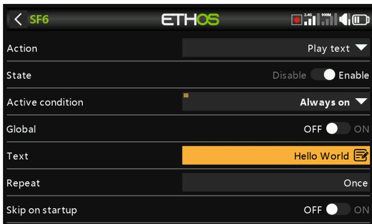
This special function utilizes an internal hardware TTS (Text-To-Speech) processor to generate spoken text from the user specified text string, rather than playing previously prepared .wav files.
