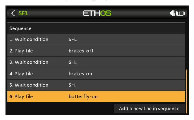
And it's possible to configure a Reset condition which restarts the sequence from the beginning at any moment.
