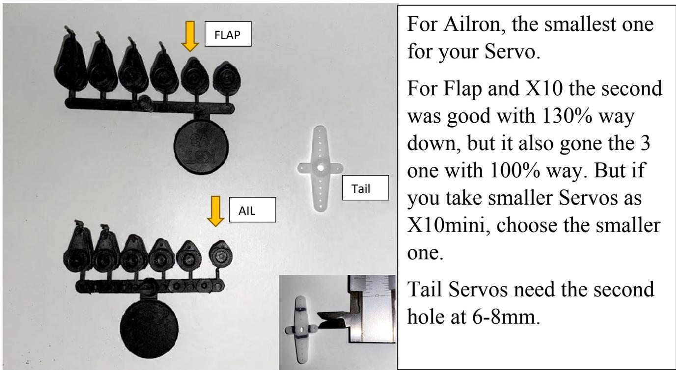
Make sure that you make all lever in 90 degree angle on your servos, and prepare the servoframes that it will be fit in the servo bays. The movement way from the linkage are 5mm for Aileron and 8mm for Flap for the full way.
