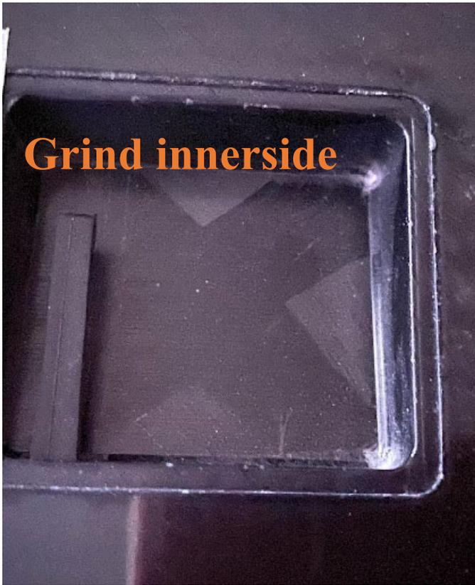
Grind the inner side from the servo bays. The servo connection from the middle wing are ready glued in the mould, you have only glue in the inner part from the fuselage and from the tip wings.
