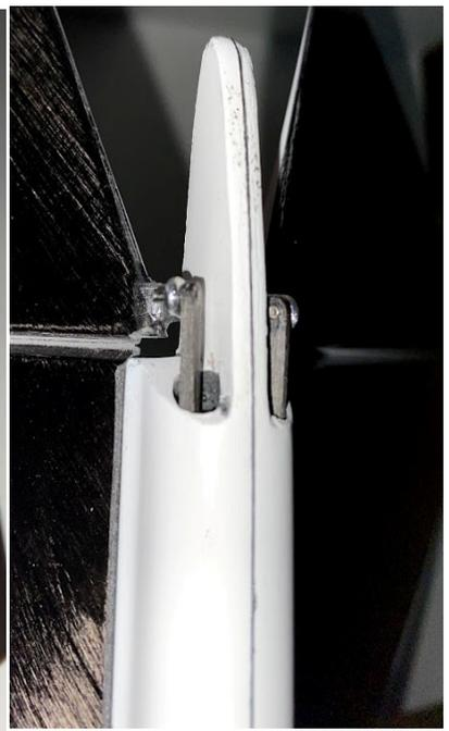
You see on the pictures below the tail servo mount. The linkage must be shorten tot he right lenght and grind. Be carefully that the Vtail pushrods have the right angle to go in the ruder hole.
