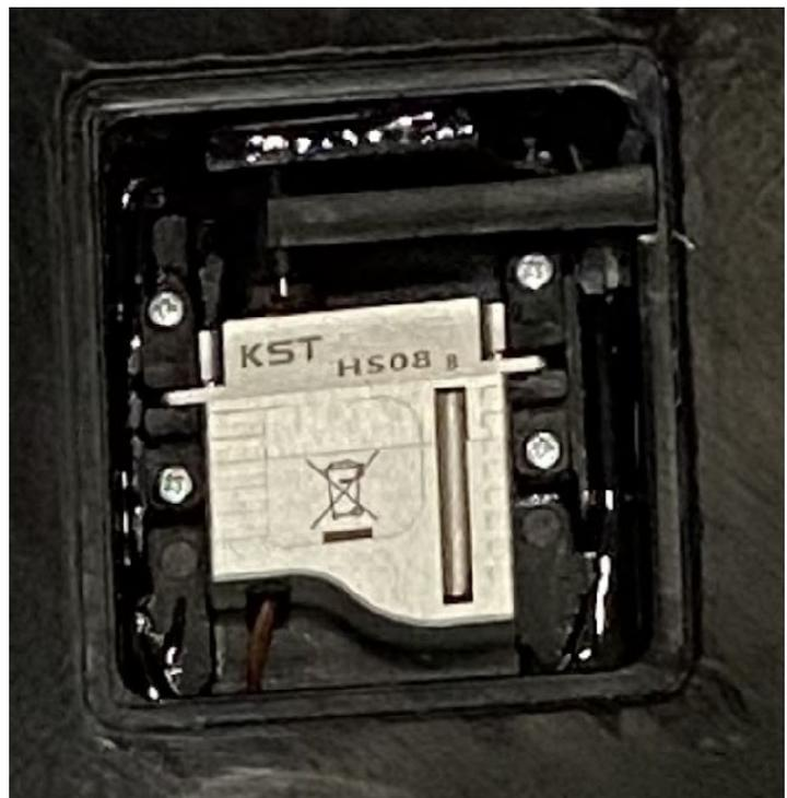
Glue the Servotrays in and make sure that it glued in well all arround. You have for wing Setup pattern teaching for Flap and Ailron. With the X10 and the second servo horn, you have ca 20% offset, with smaller servos more (40-55%)
