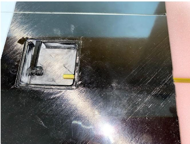
It is necessary to mount the IDS Servo mount before you install the Servobays
