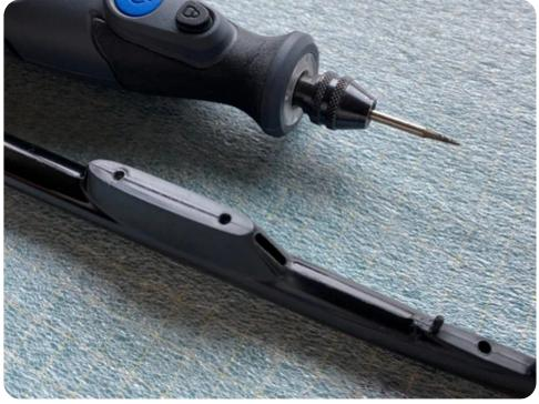
2. Mask the right side of the boom under the elevator mount. Draw a line down the centre, and cut a thin slot roughly 15-20mm long. This is for the pull-wire for the rudder.
