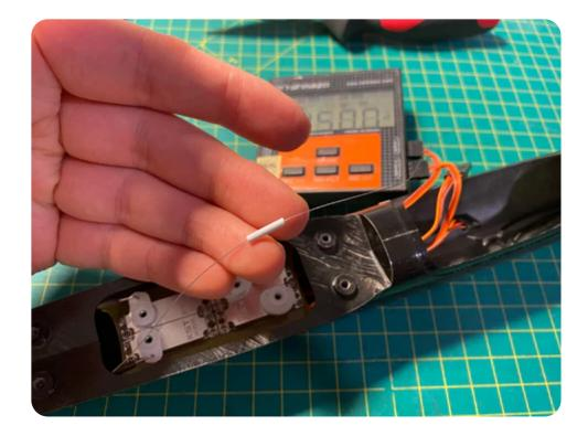
25. Plug the rudder servo into the servo tester and centre the servo. Thread the pull wire through the pulley or servo arm and wrap it around the servo screw. Tighten the screw to hold the wire in place. Cut off the excess wire.
