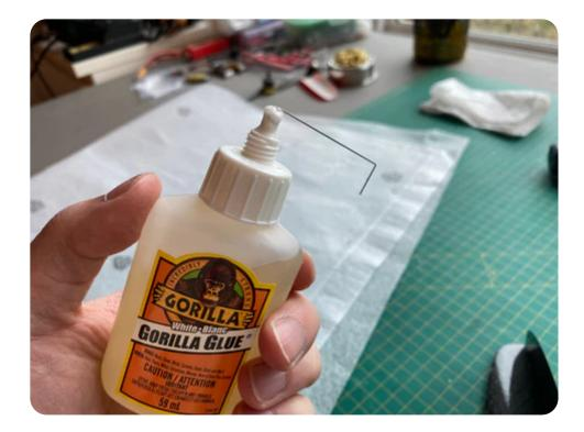
Note 2, the white Gorilla Glue expands and foams up as it cures. This helps the concentrated load from the thin spring wire spread to a larger surface so it doesn't rip through the core material and potentially poke out the skins.
