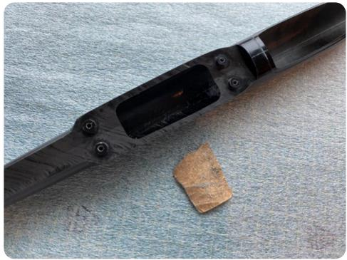
7. Mount the servo tray (with servos) into the fuselage, then glue with super thin CA. Once cured, create a fillet with medium CA.
