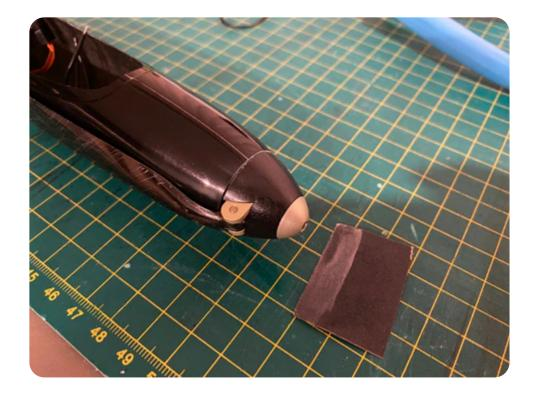
14. Remove the spinner and take the motor assembly out of the fuselage. Apply glue to the outside edge of the motor mount and reinsert it into the fuselage. Attach the spinner assembly to make sure the motor mount is in the correct position as it cures.
