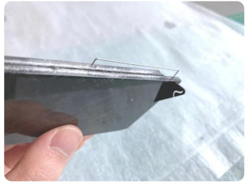
5. Dip the two legs of the spring into white Gorilla glue, then insert them into the tail. Repeat for the stabilizer.
