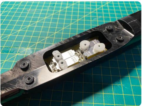
4. To prepare the servo arms for the wing servos, plug a wing servo onto a servo tester and make sure it is entered. Take one of the cross-shaped arms and put it on the servo with one of the long arms facing out. The goal is to have the arm pointing straight out. If the arm is coming out at an angle, flip the servo arm 180° and try the other long arm. Cut off the remaining arms, and shorten the remaining arm to the innermost hole.
