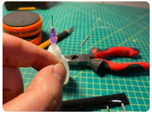
24. Insert the front of the wire through a plastic guide tube, and glue the guide tube inside the fuselage so the wire doesn't interfere with the pushrods.
