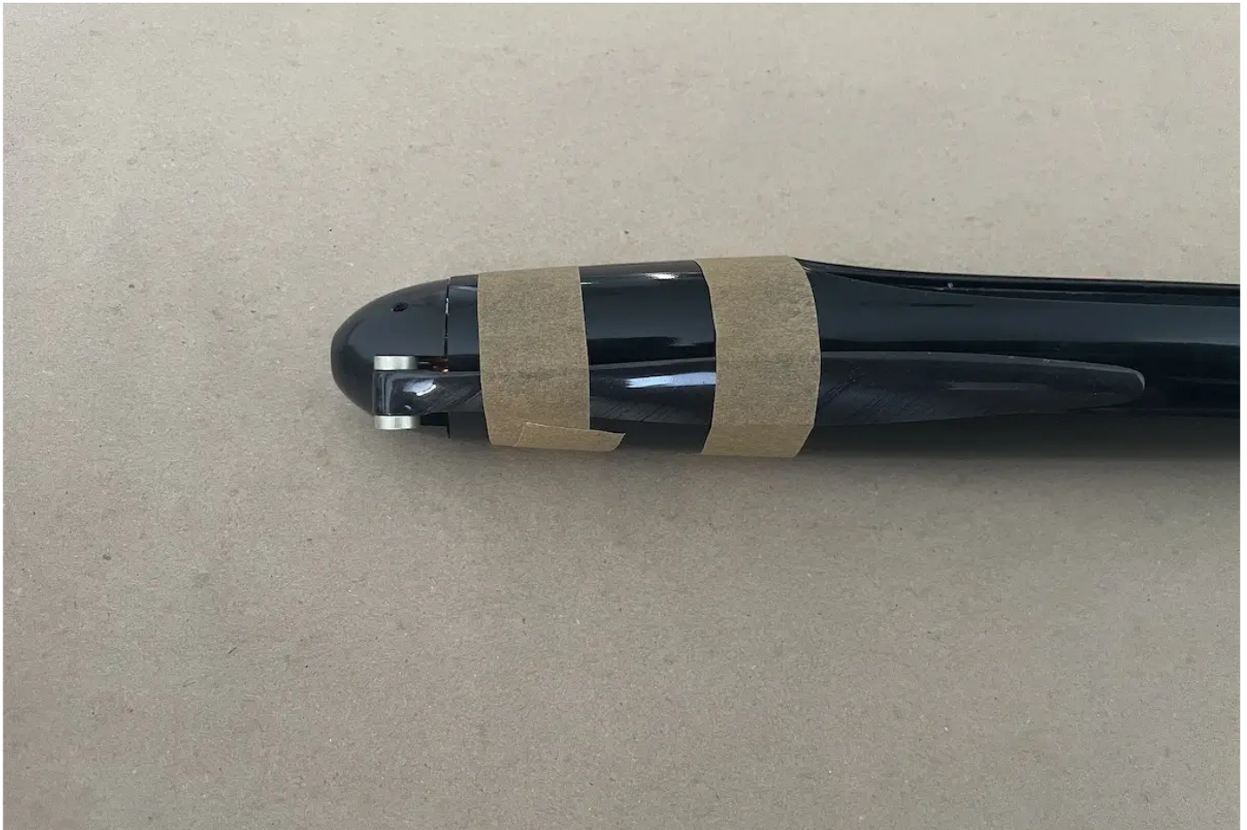
Position the motor inside, install your spinner w/ prop, fix it in place and glue the firewall in.
