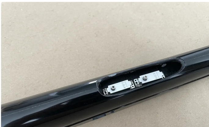
Position the servo plate inside the fuselate, as close to the "top" of the fuselage as possible
