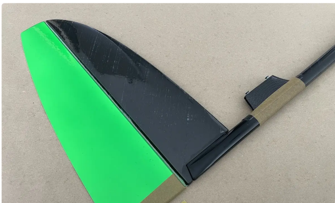
Mask the Rudder and the boom where the cable opening will be
