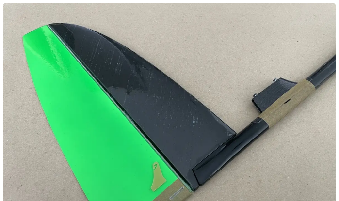
Make an openings with the sharp knife. The rotary tool with diamond bit/disc will come in handy as well
