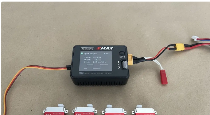
Center the servos, trim and install the servo arms. For ailerons, you might want to make a hole as close to the shaft as possible.
