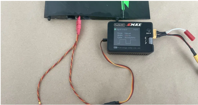
Connect your servo to a servo tester with a provided harness and dry-fit your control horns
