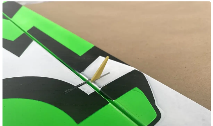
Install control horns onto the L-bands and clue the last in place
