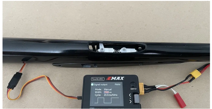
Center the Elevator (front) servo and install the servo arm. Make nice tension on the cable and crimp it with pliers
