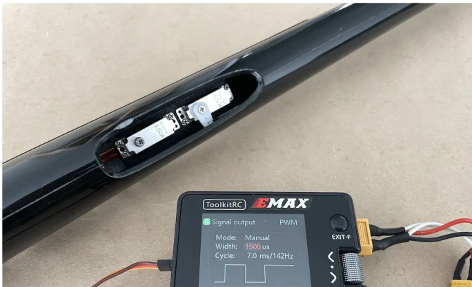
Center the Rudder (rear) servo and install the servo arm on the servo shaft
