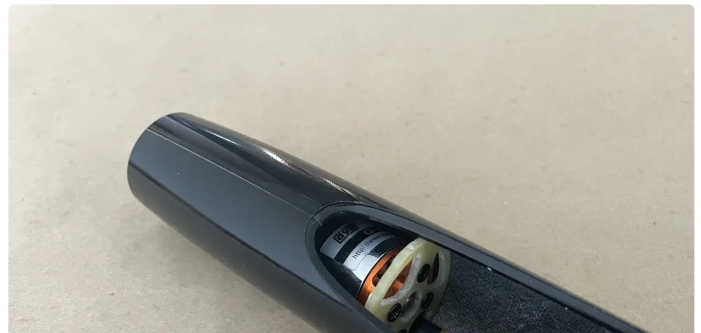
Put the both parts into the fuse separately and attach the firewall onto the motor once inside. Pay attention to the fuselage seam location and as well as the corresponding spots on the firewall.
