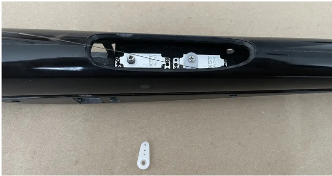
Trim the elevator servo arm, you'll need a long one to have a good deflection
