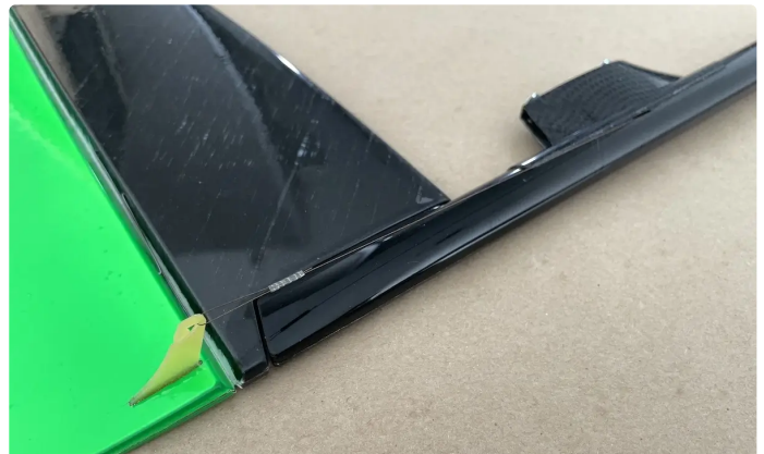
Center your Rudder make a nice tension on the cable and crimp it with a provided tube
