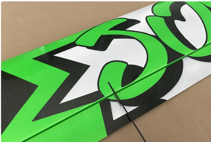
Make a pushrod channel with a provided 2x1mm CF tube
