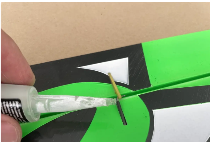
Put a drop of CA on the link to remove any possible slop
