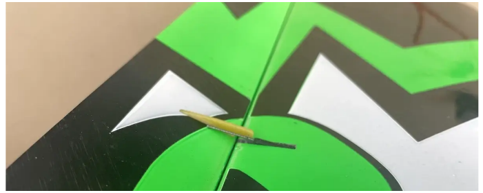
Set Flap servos to Full-Up, move your Flap accordingly, and mark the place where you need to make an L-band. Center the Aileron servo and flatten the control surface with the wing bottom for Ailerons.
