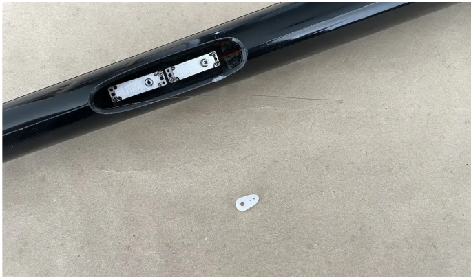
Trim and the Rudder servo arm
