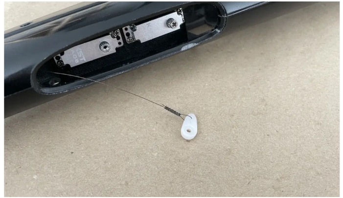
Crimp the cable on the servo arm
