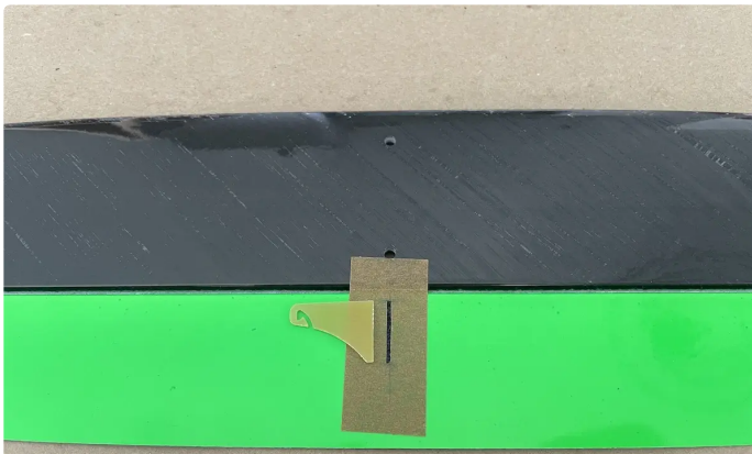
Mask, mark and cut the opening for the control horn in the elevator
