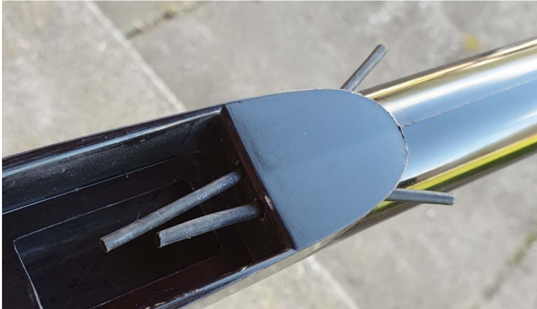
Antenna holes / guidance tubes
