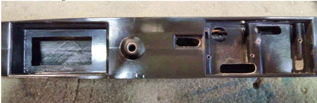
Cutting holes in fuse before assembly
