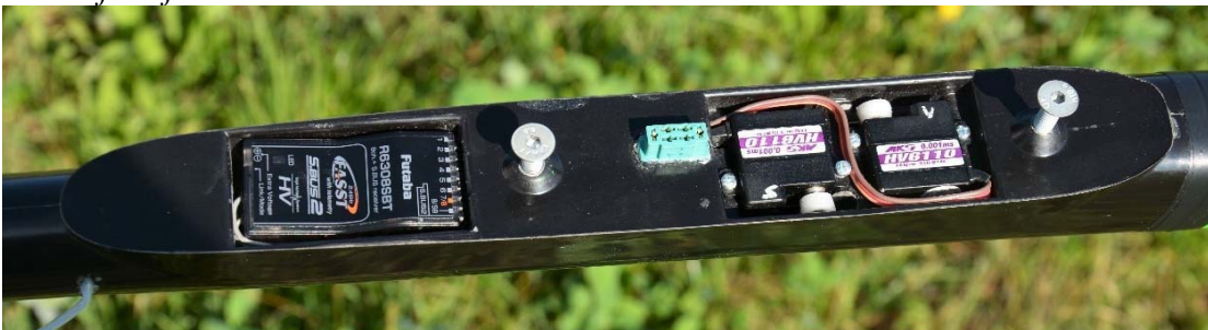
Servos and receiver installed in fuse
