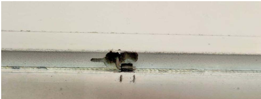
Distance aileron to pin is 0,5mm
