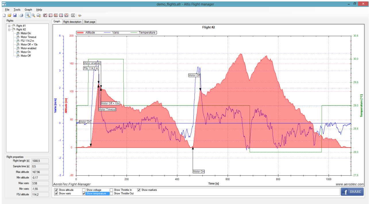
Fig. 2. AerobTec Altis Flight manager PC application main window
