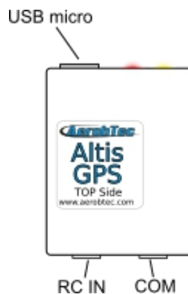
Fig 2: Connectors of your Altis GPS
