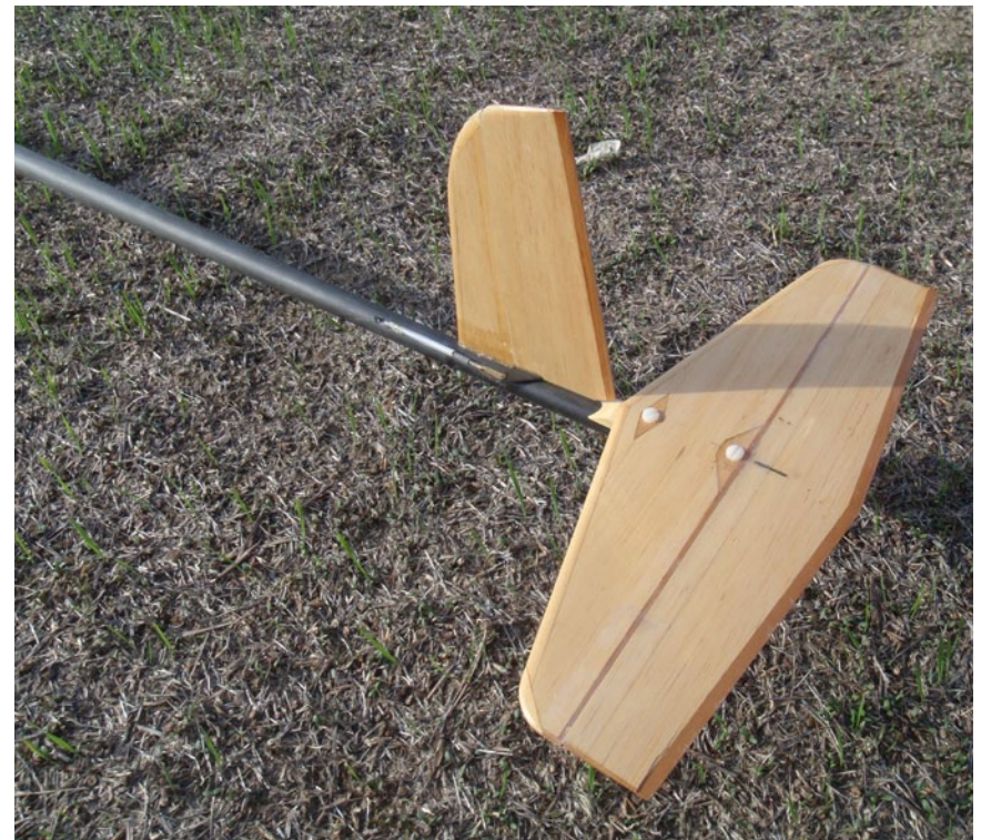
The Version 1 tail group. It's built from light quarter inch contest balsa with spruce leading edge and trailing edge inserts. All tail surfaces were sealed with clear dope.
