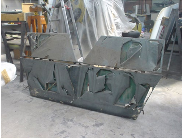
Above: The Zögling horizontal stabilizer before the commencement of the reconstruction process.
