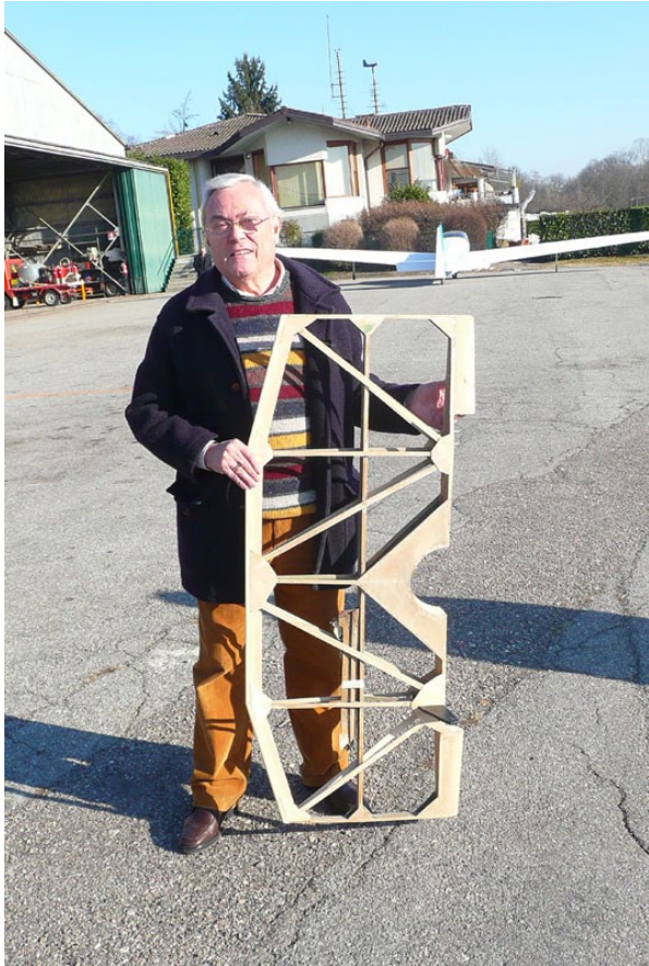
Above: The author with the rebuilt stabilizer.
