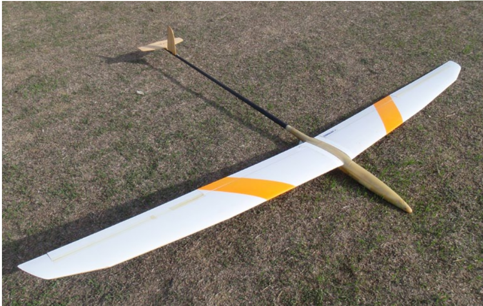
Version 1 ready to fly. The long boom and small tail group area is readily apparent.
