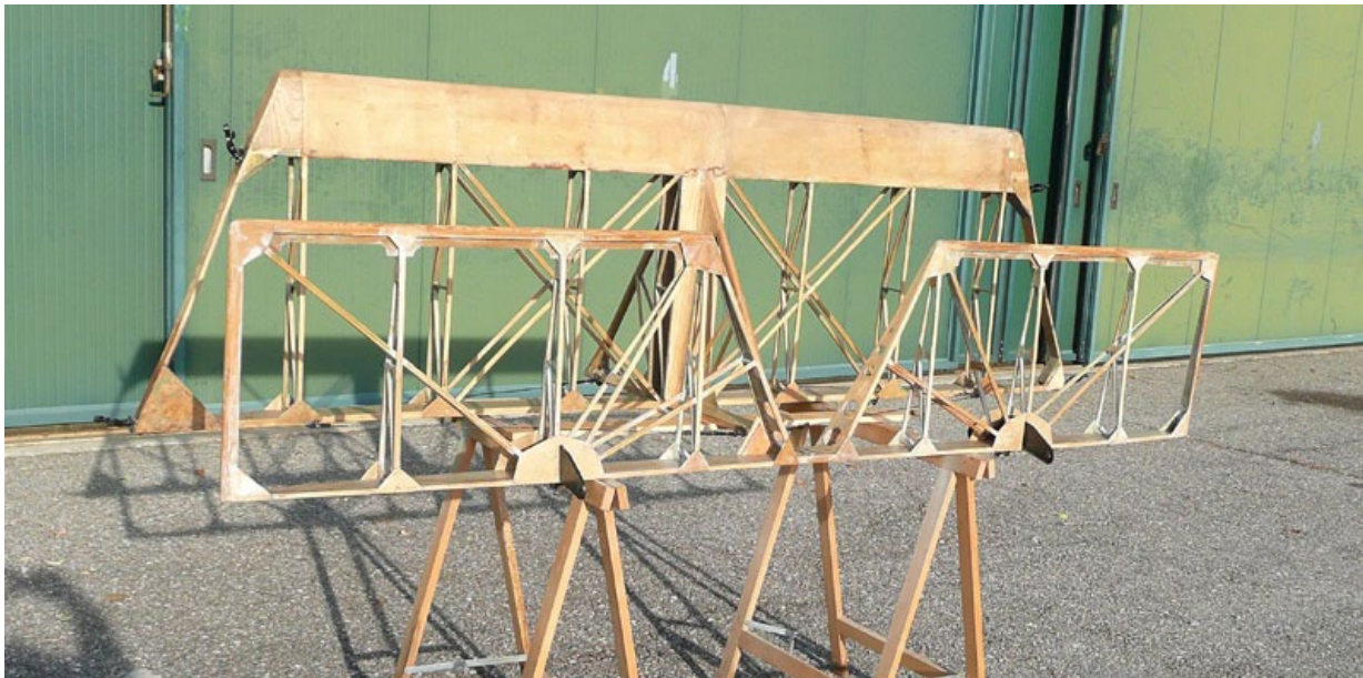
Below: The rebuilt stabilizer and elevator are ready for covering.
