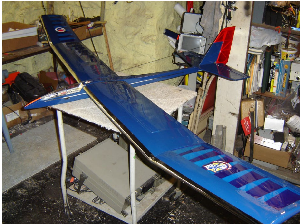
The Scepter is covered and ready for flight. The center of gravity turned out to be very close to the plans location but I had to move the tow hook forward about 3/16th inch to get a stable launch.
