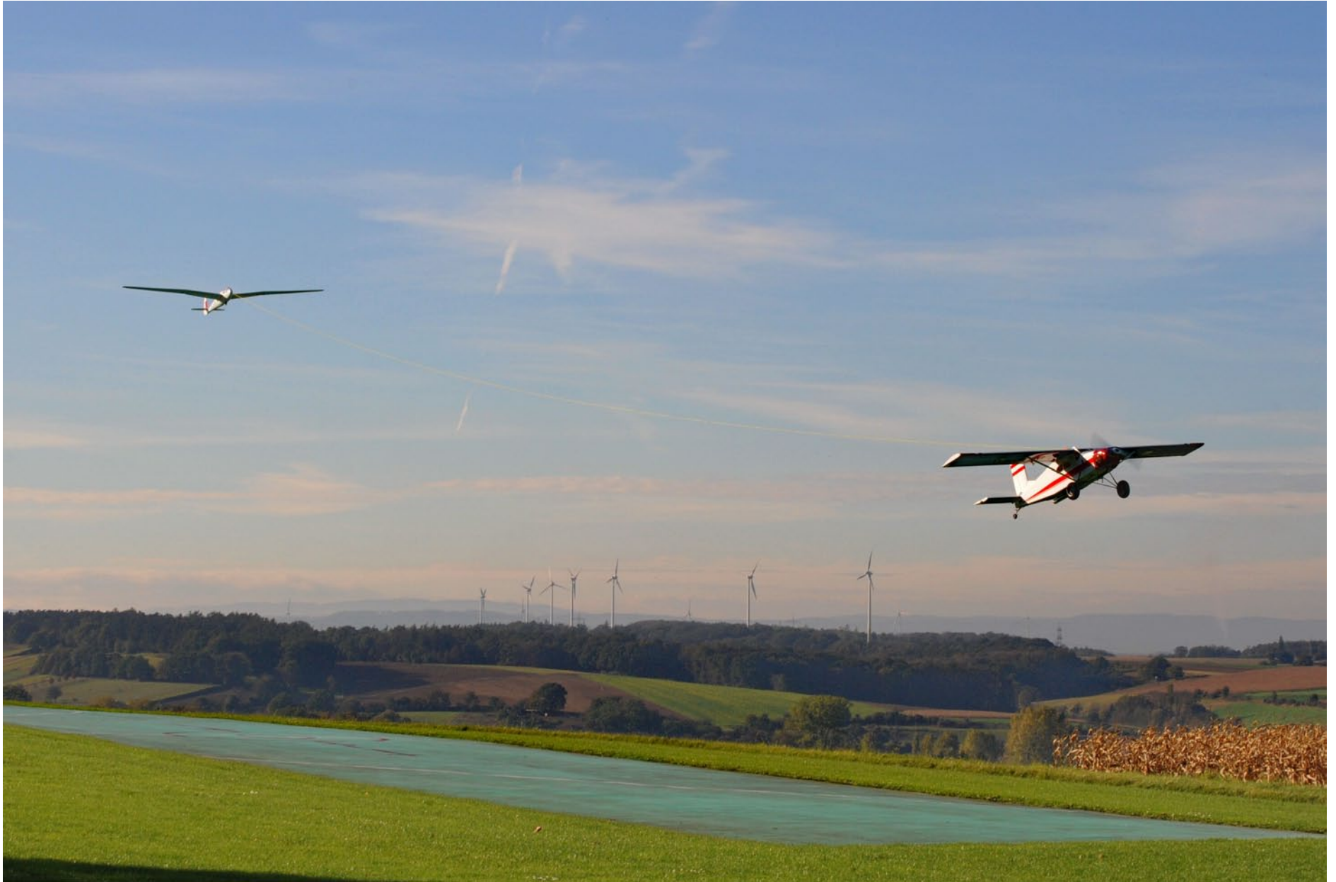
Usually we are towing our gliders with a tug. It's a semiscale model of a Pilatus Porter PC6 equipped with a 35ccm gasoline engine.
