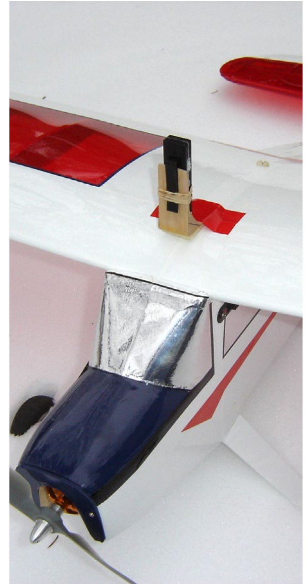
The camera was initially mounted to the wing on the DeBolt Champ for flight testing. It was high enough so that the prop wasn't visible in the pictures.
