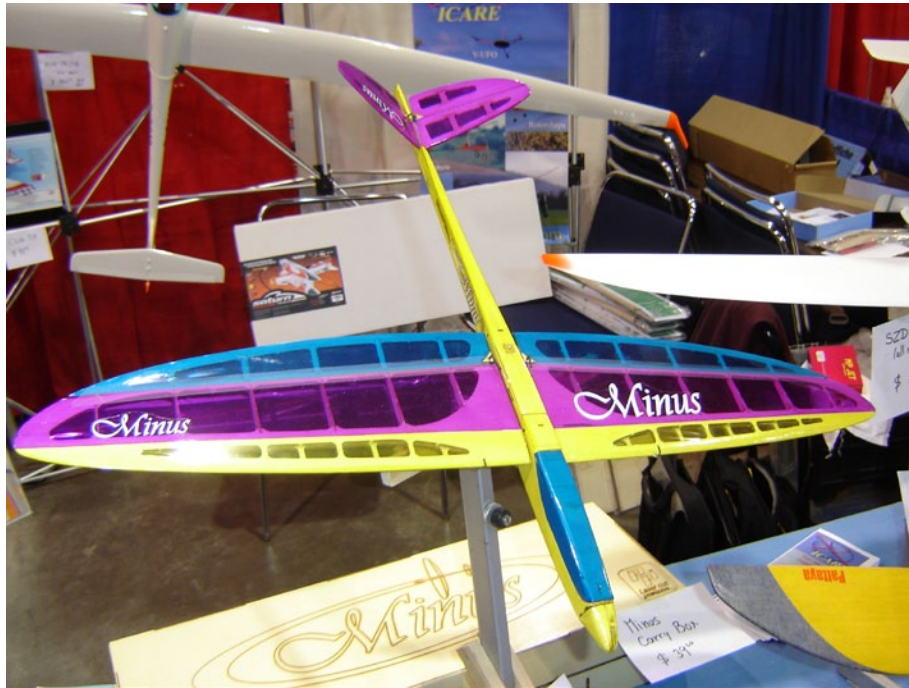
Above: This Minus electric was a good example of the laser cutting of parts that has added a next level of performance to small ships. Pete Carr
