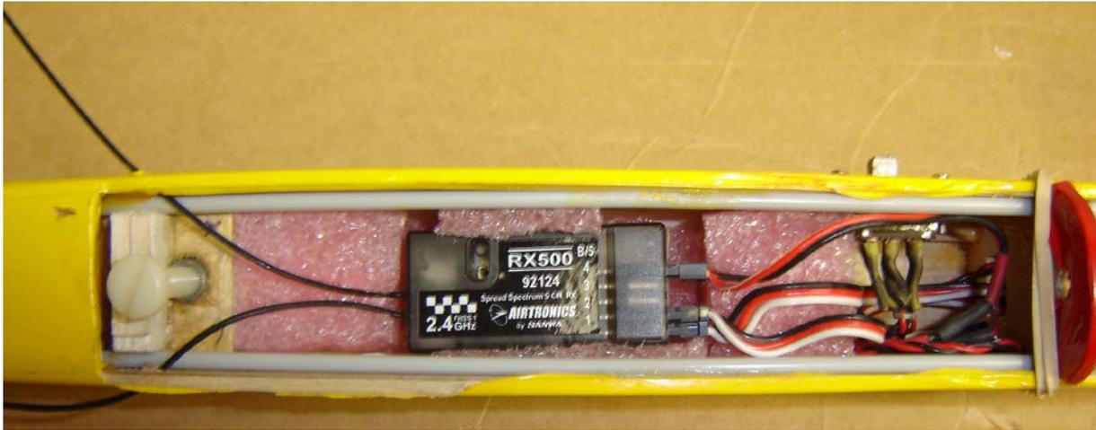
*Because of the small fuselage width the receiver is mounted under the wing. I punched small holes in the sides and routed the two antenna through them. One antenna is taped to the side while the other is taped to the bottom of the wing at a 90 degree angle.*
