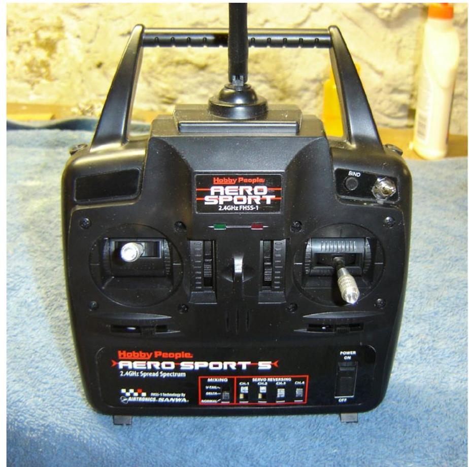
*All the controls are located on the front of the transmitter. Mixing and servo reversing switches are at the bottom while the Bind button and channel five toggle switch are at the upper right.*
