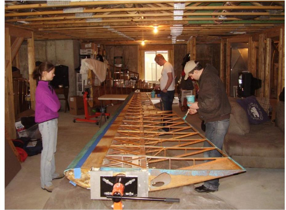
*I knew the general Stewart's process from doing the control surfaces but had never covered anything nearly as big as a wing before. We started out by cleaning the wings with the heavy duty cleaner, and then painting glue around the perimeter of the*
