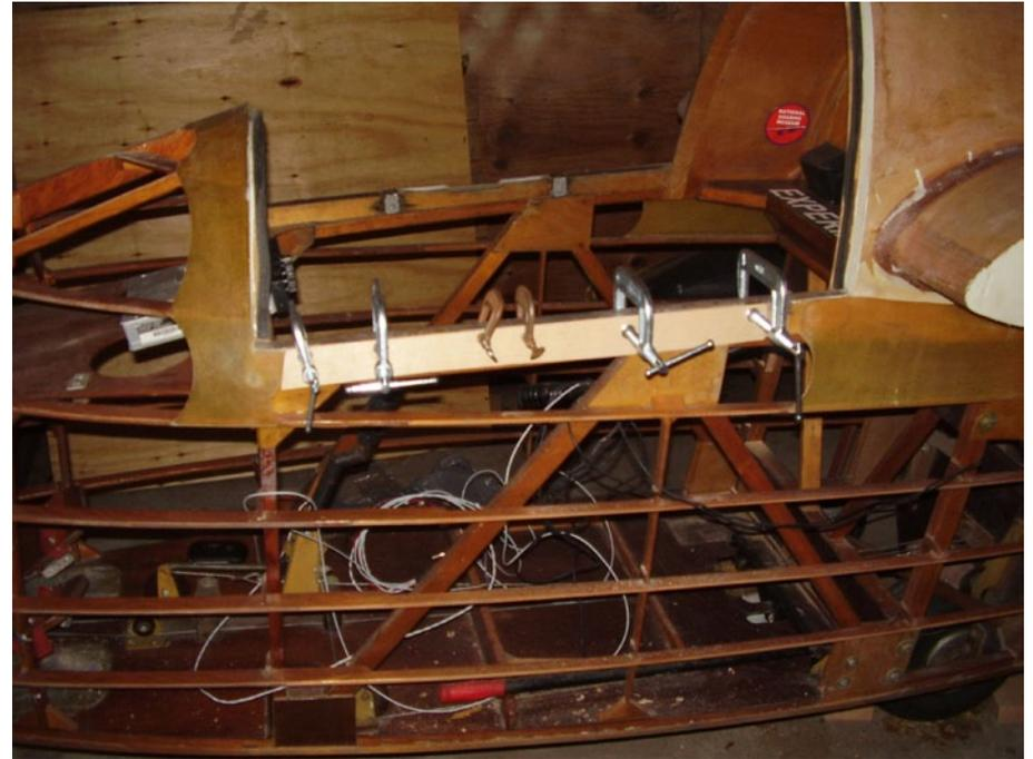
*Well after inspecting Dean Gradwell's glider at the SSA Convention I decided to bite the bullet and cut out the shelf in my Cherokee. Getting to the point where about the only thing that I have left to do on the fuselage is some epoxying and new varnish on areas where there is new wood or we have sanded.*
