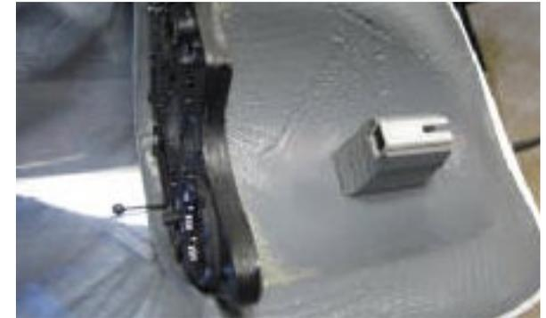
*Canopy removed to show the canopy hinge in the up position. The hinge is glued to the fuselage interior with shoe Goop.*
