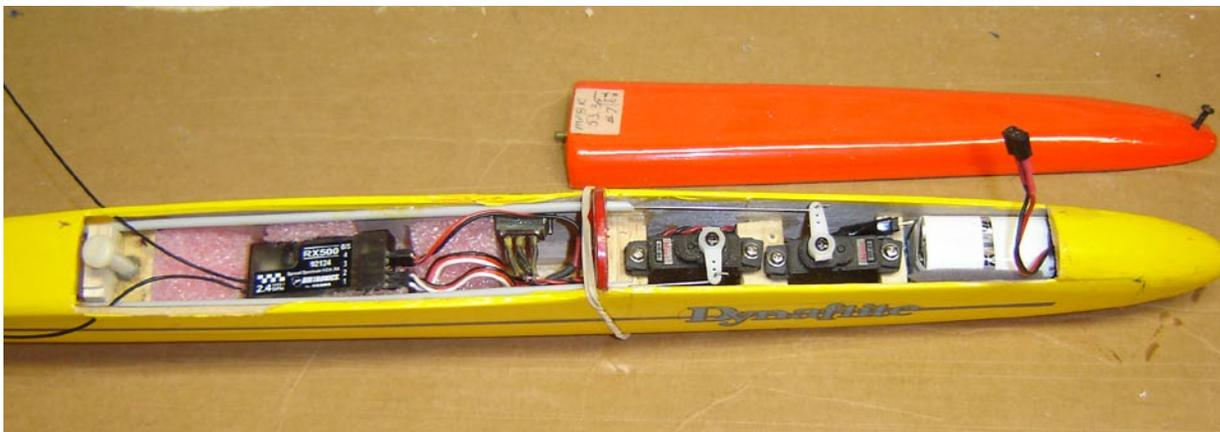
Next, I removed the channel 04 receiver, an old FMA unit, from the aircraft and dropped the new one in. The servo connectors plugged right in and the front panel servo reversing function on the transmitter got the two surfaces going in the right direction.
