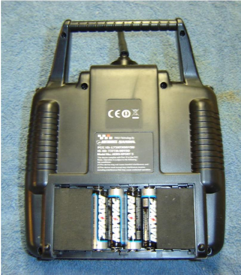
*Left: The rear battery cover is removed from the transmitter and four AA size dry cells are installed. The low battery count makes the transmitter very light and easy to hold.*
