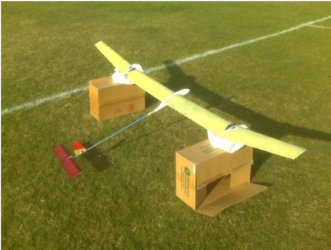
*F1A is a FAI free flight glider class. It is also known as A/2 or Nordic Class. The model must have a projected area - wing and stabilizer - of between 32 and 34 dm<sup>2</sup> (496 - 527 in<sup>2</sup>), and a minimum weight of 410g (14.46 oz.). Launch is by hand tow using a 50m line. F1H is the smaller glider class, also known as A/1. These gliders are required to have less than 18 dm<sup>2</sup> (279 in<sup>2</sup>) total projected area and weigh at least 220g (7.76 oz.).*
