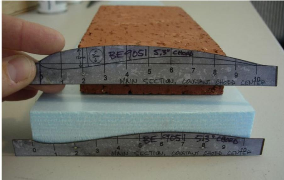
Metal templates for the root of the KB18 wing tip. BE 9051 airfoil, 5.3" chord. Spar location marked forward of 30% chord.
