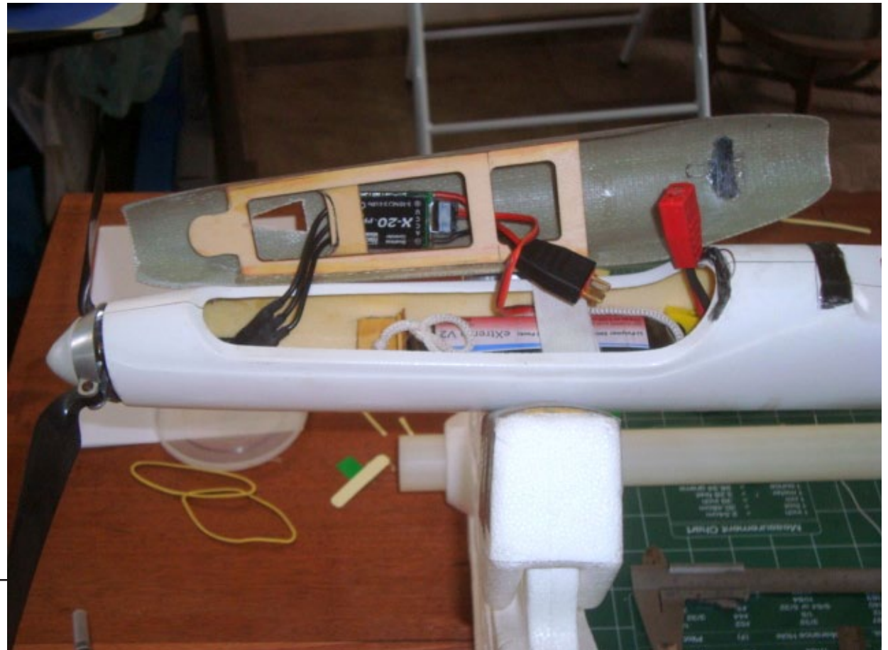
The speed controller is mounted in the canopy with the wiring guided through the lightening holes. Easily accessible.
