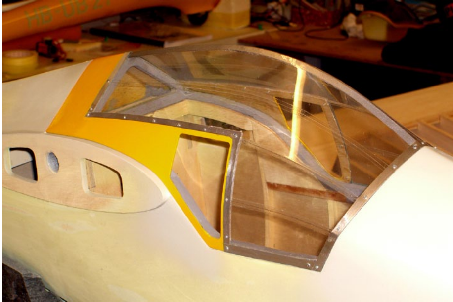
Above: The canopy is constructed of clear plastic strips, just as the original.
