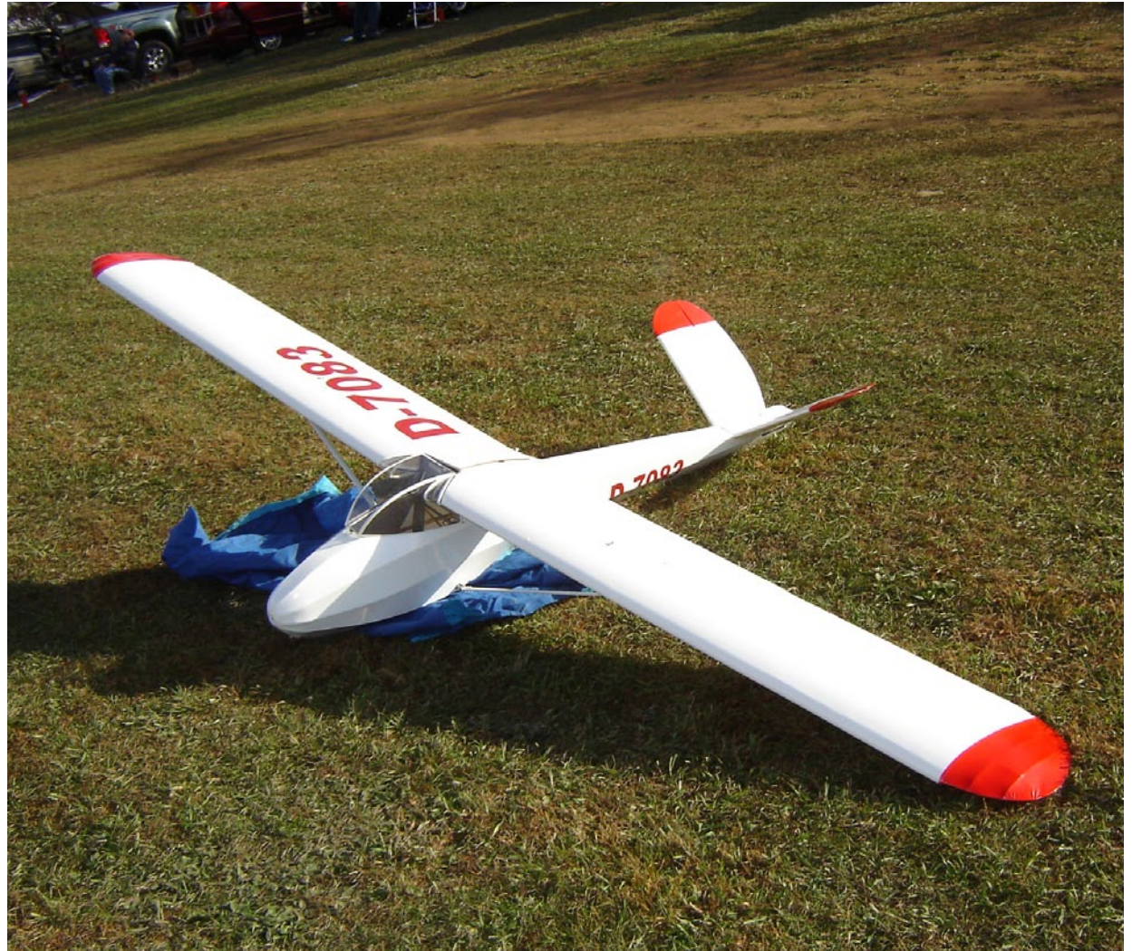
This V-tailed sailplane, a Schleicher Ka 3, had a span of about 120 inches. It was towed very easily by the Hanger 9 Piper Cub electric tug. It had a fixed belly wheel and made easy takeoffs from the short grass.
