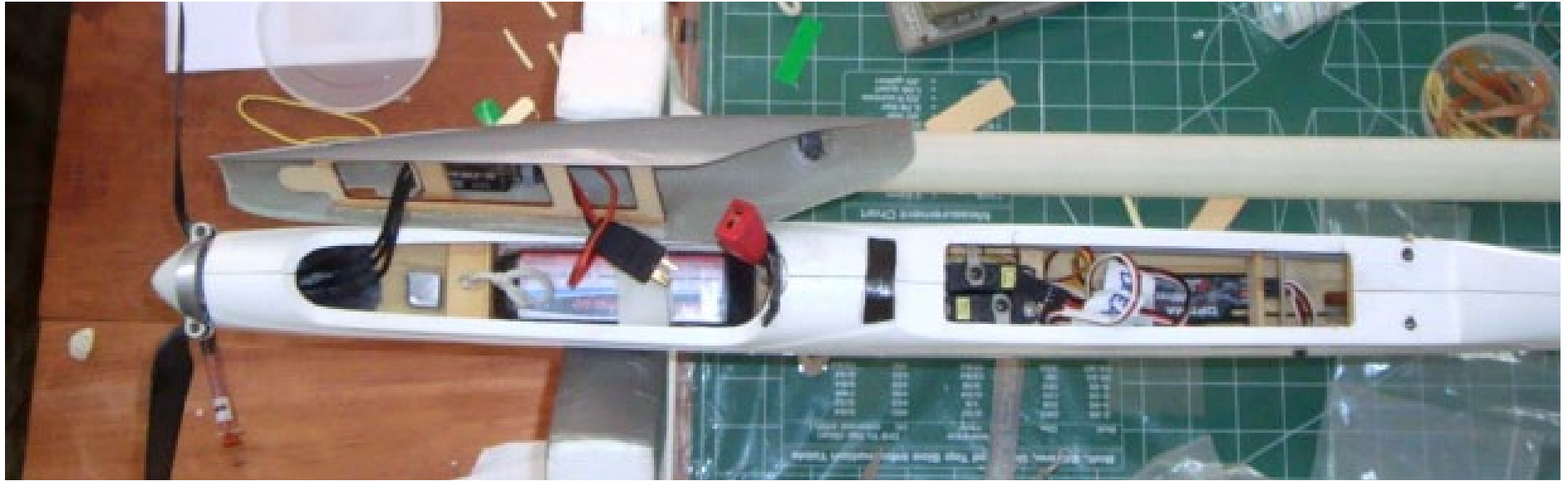
Equipment arrangement: motor, battery and speed controller, servos, receiver and antenna. All in sequence from nose to tail.
