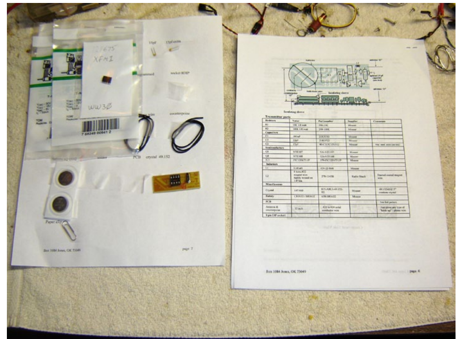
The tracking transmitter in kit form. The individual parts are taped to sheets of paper with the name and value called out above each one. The physical diagram indicates the location of each part. In addition, should you need a replacement part, each one is referenced to a part number on www.mouser.com .
