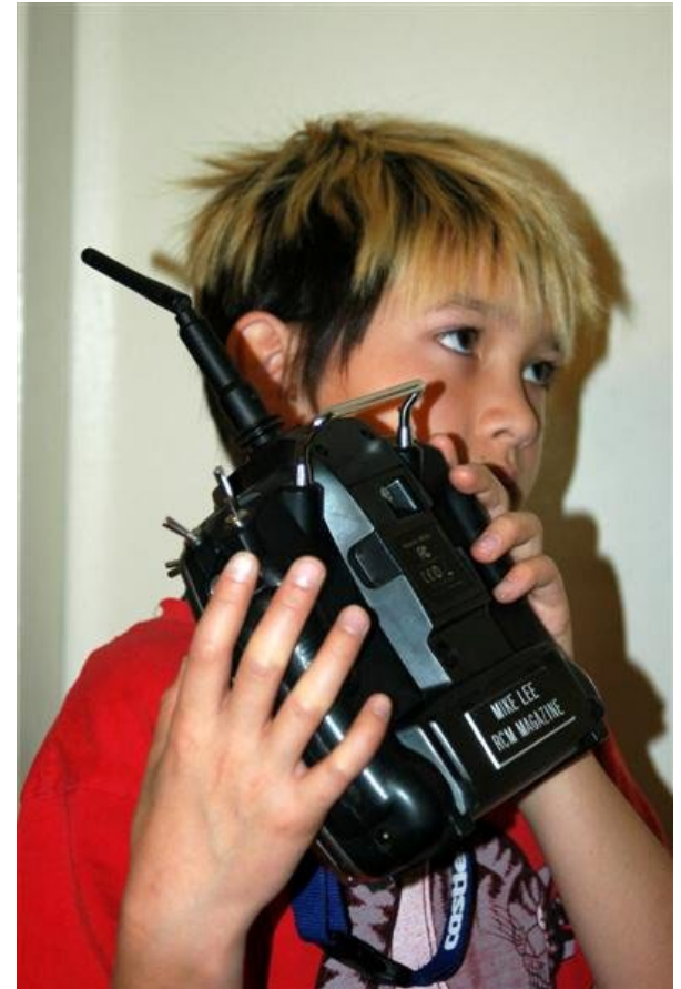
EXAMPLE 3: For those pilots who use body English, or just get animated with holding the Tx, this angle is also a no-no. It goes that like the earth, there is a polarity to the radiation pattern of an antenna. So, if there is a North Pole being at the tip of the antenna, then there is a South Pole at the bottom. Therefore, if there is a Cone of Silence at the top, there will be another one at the bottom! Want to prove this to yourself? Do some flights with a Flight Log device and you will find out!
