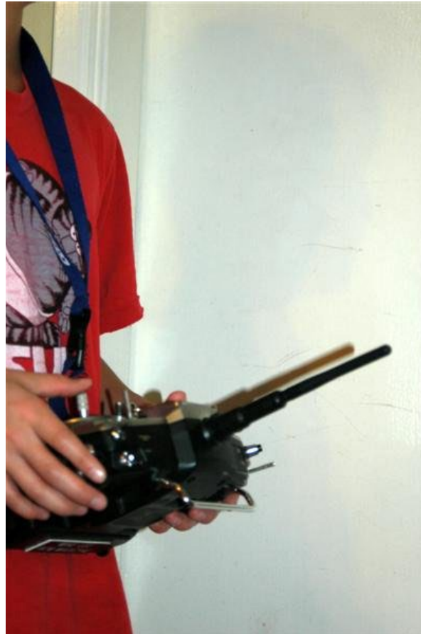
EXAMPLE 2: This how NOT to have the Tx antenna when you hold the Tx like this as it aims the tip of the antenna directly at the plane, allowing the plane to enter into the "Cone of Silence".
