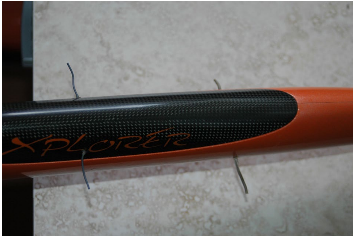
My NaN Models XPLOREER with an AR7000 Rx and one remote Rx installed. Note the antenna placement... not what is recommended, but it has been flawless in operation.
