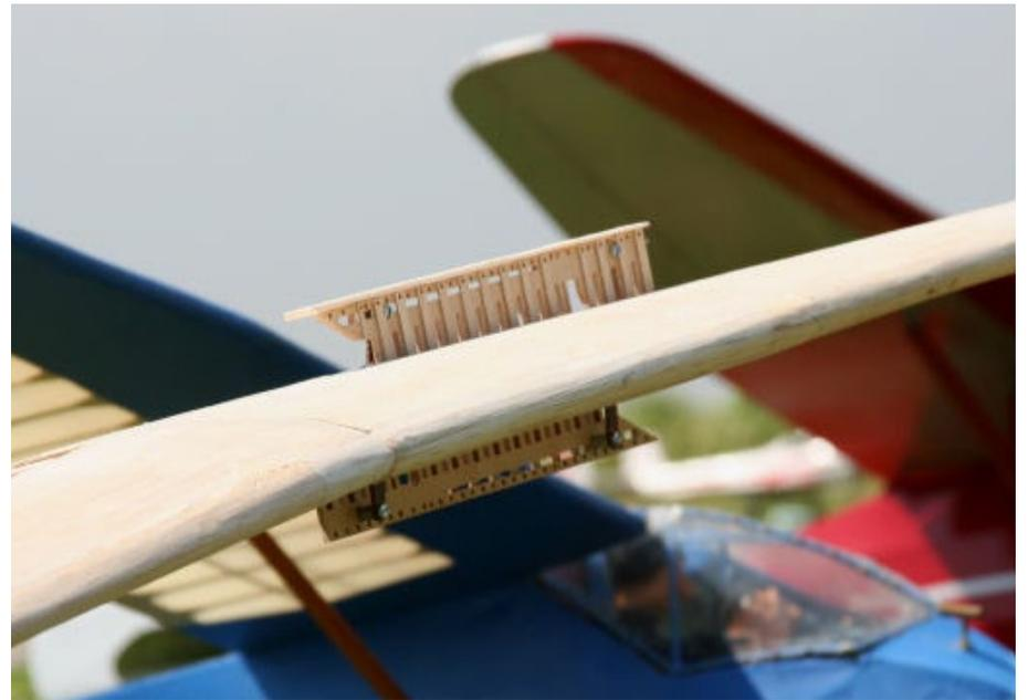
*The intricate "double comb" airbrakes.*
