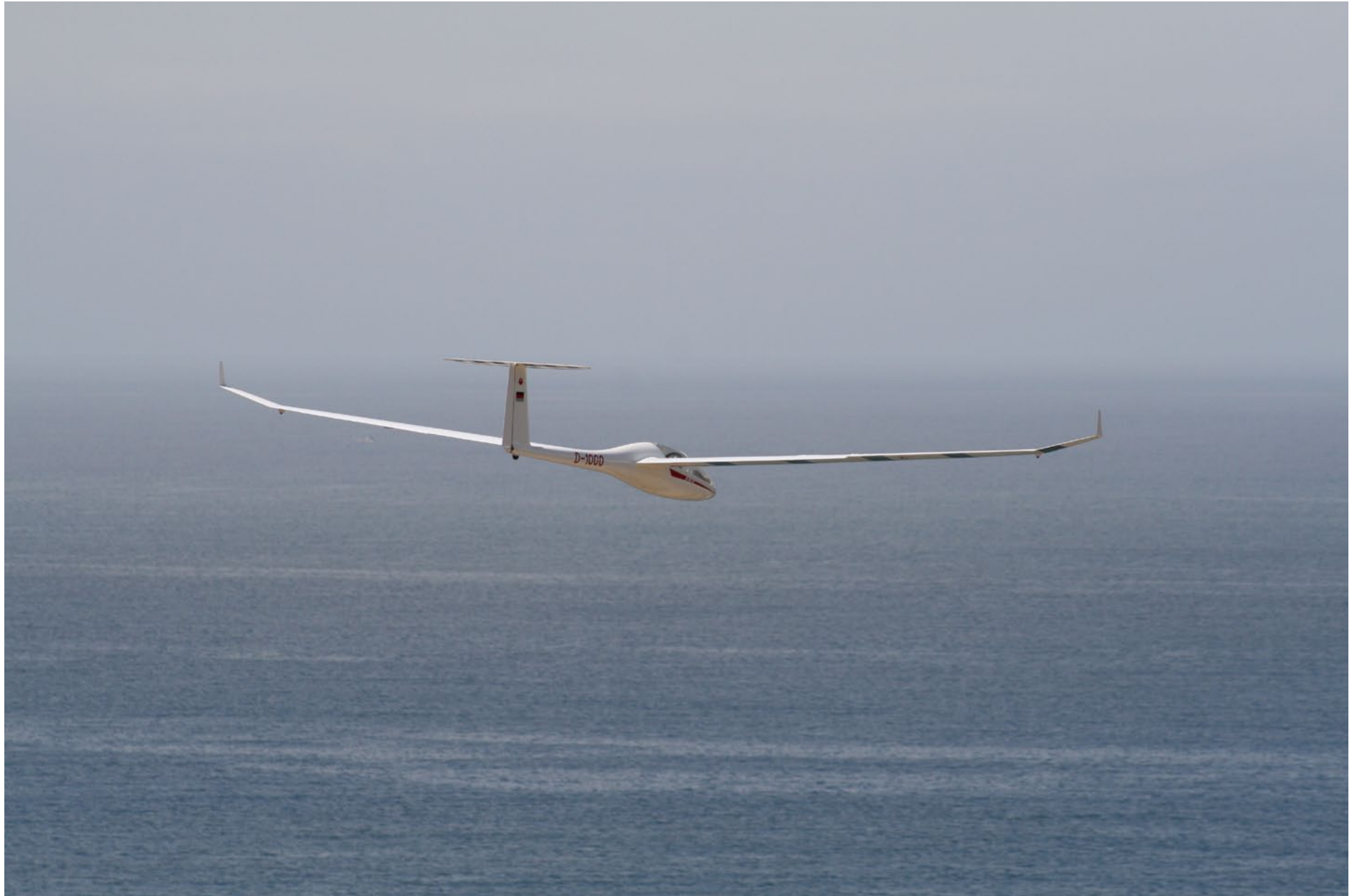
The model has foam core wings sheeted with obechi, spoilers (no flaps), water ballast, and retract.
