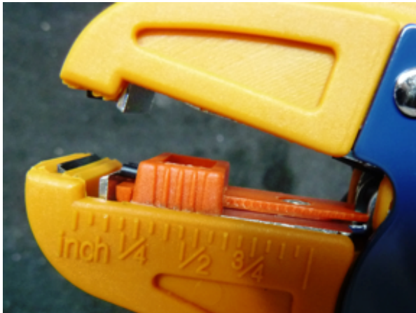
The depth of the jaw is adjustable so the same amount of insulation is stripped each time.
