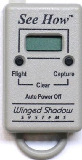
and retrieves the series of recorder data points at the end of the flight. It can capture and report up to nine altitude or airspeed readings captured at pilot-commanded points, plus the maximum altitude or airspeed for each flight.
