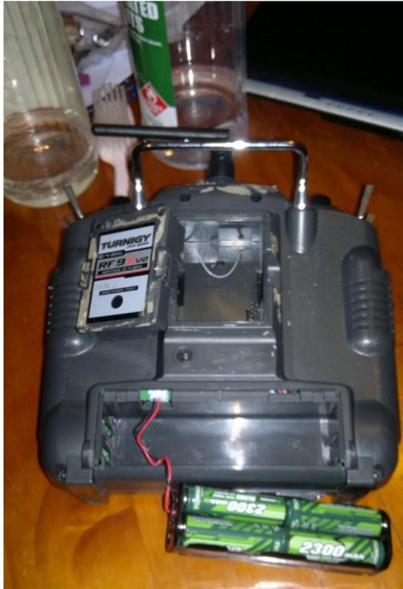
*Rear of the Turnigy 9X showing the battery pack and open module compartment.*
