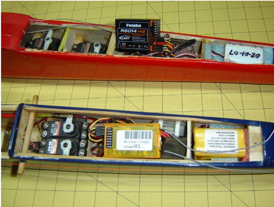
The top fuselage is a 9-servo sailplane so the 14 channel R-6014 receiver gets a workout. The Orange 2.4 GHz FASST receiver in the Oly II fuselage is about the same size as the Futaba receiver but slightly thinner. The two coaxial leads used on each receiver are identical. Current drain was also about the same for each receiver with the servos unplugged.
