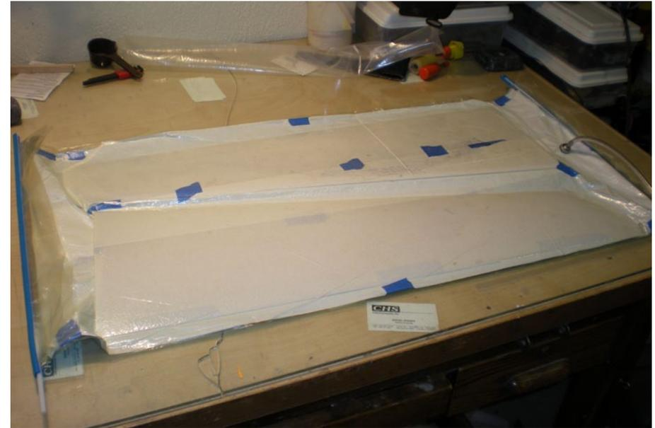
*The top layer of glass being vacuum bagged.*
