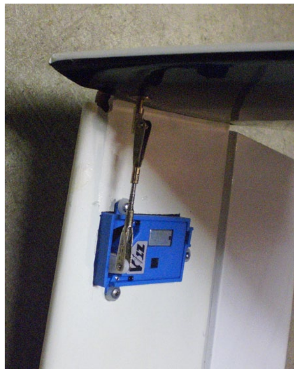
Above and left: Strong Volz metal geared digital servos in the tail for both the rudder and the stab, making them rock solid.
