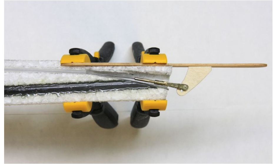
Dave's modification to better align the elevator pushrod clevis with a lower control horn hole. The CF stiffening tube was trimmed with a roto-tool grinding bit and the foam passageway was tapered to allow the pushrod to bend downward.
