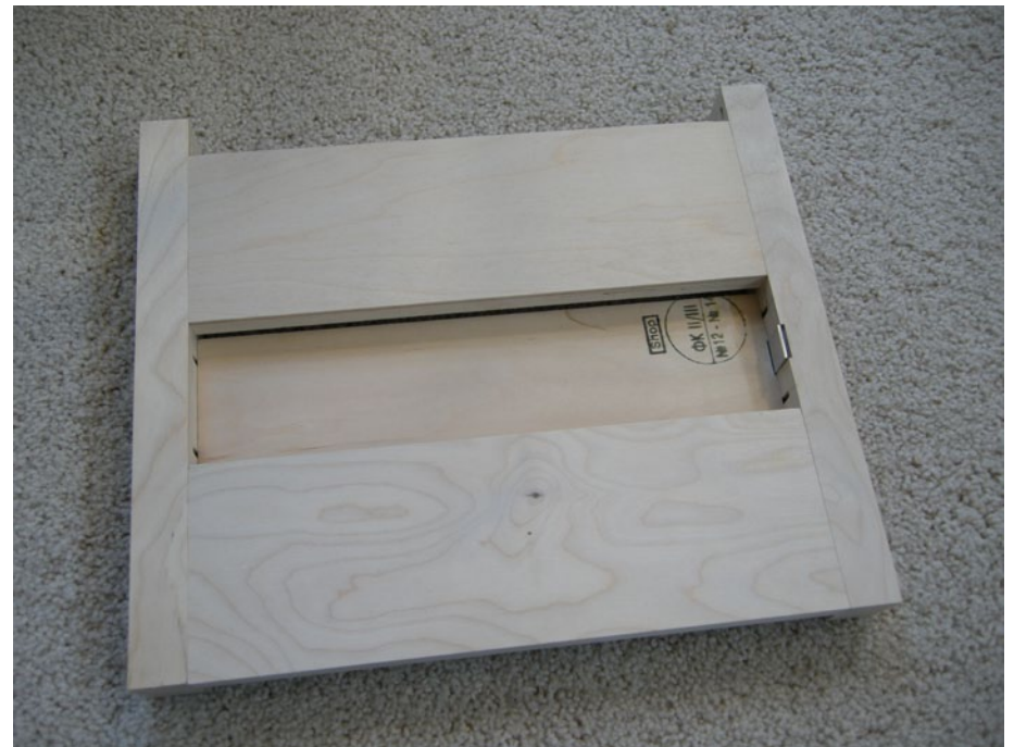
Cutting sled top view shows headstock in the foreground and adjustable tailstock in the background while the cutting bed is shown in the lowest position. The aluminum tension tab on the right rail keeps material tight between the rails.
