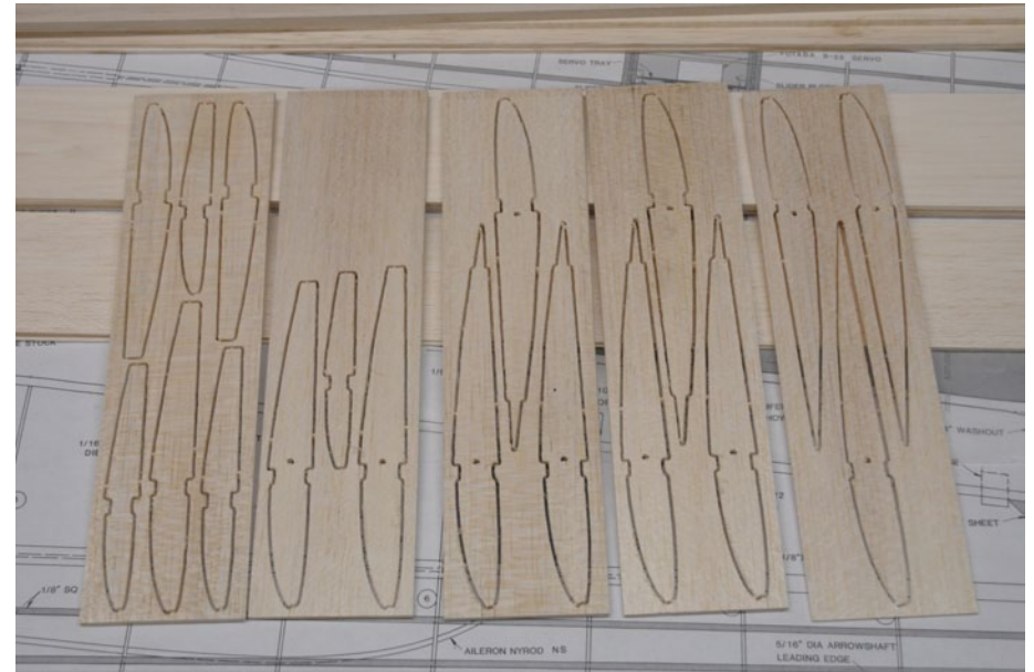
Bobcat wing ribs in stacked pairs of sheets after cutting in the CarveWright
