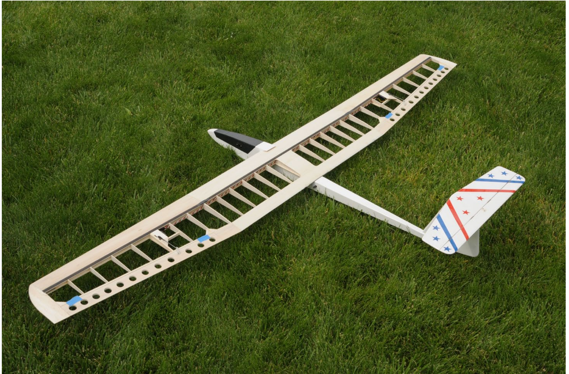
New AG34 airfoil Bobcat wing construction complete and ready for covering
