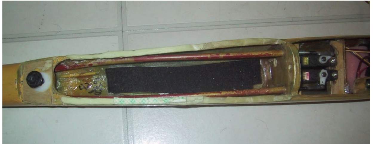
Illustration 4: The epoxy shims simply popped off the wing saddle. Sometimes, I just get lucky, but all that the ease of removing the shims did was entice me into continuing to clean up and rebuild the fuselage.
