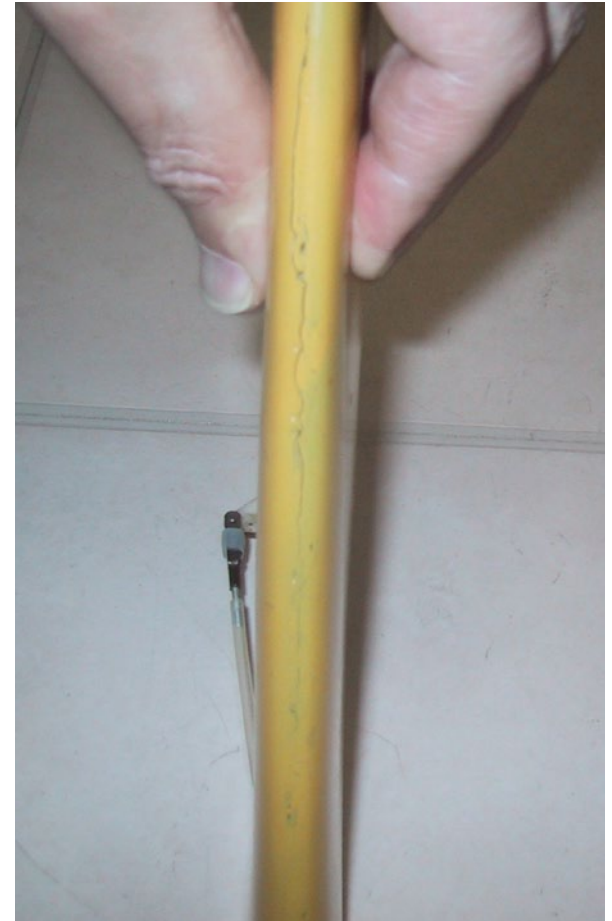
Illustration 7: Under pressure the vertical fin reveals its little secret: it's cracked from top to bottom. This is the result of the vertical fin bending and vibrating sideways on hard landings.
