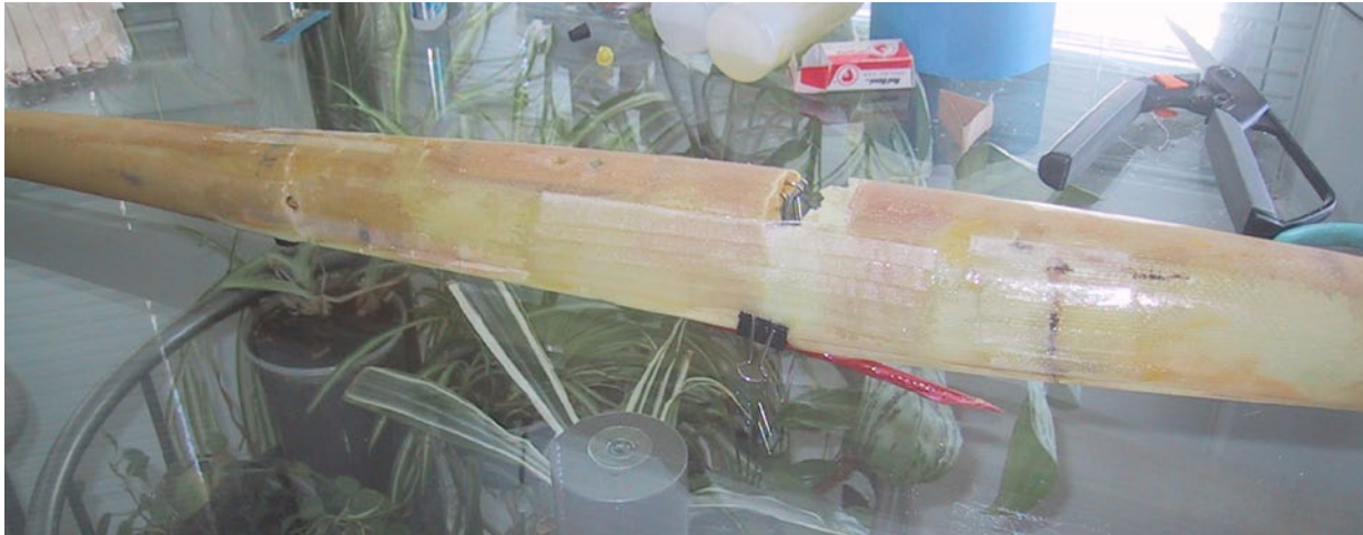
Illustration 6: Much cleaner and lighter. Narrow strips of heavy fiberglass, to be able to follow compound curves, are CA'd to the fuselage, both inside and out, to hold the broken sections together. These repairs have held up to numerous high impact landings.
