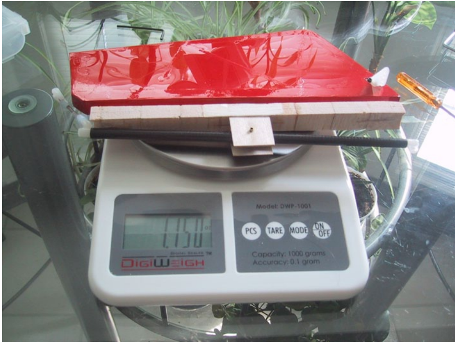
Illustration 16: The rudder assembly built for the new fuselage is even heavier than the first rebuilt one by 15 percent. I did mention that I'm not a builder.
