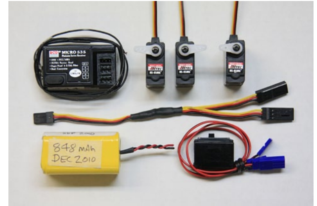
On-board radio gear in Dave's plane included a Hitec 535 receiver, three Hitec HS-85MG metal gear servos, a Y-cable, a 700 mAh NiCad battery pack and an Airtronics on/off switch.
