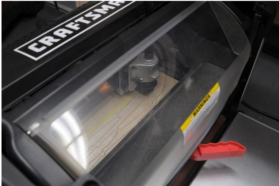
CarveWright at work cutting wing ribs for the improved Bobcat thermal wing
