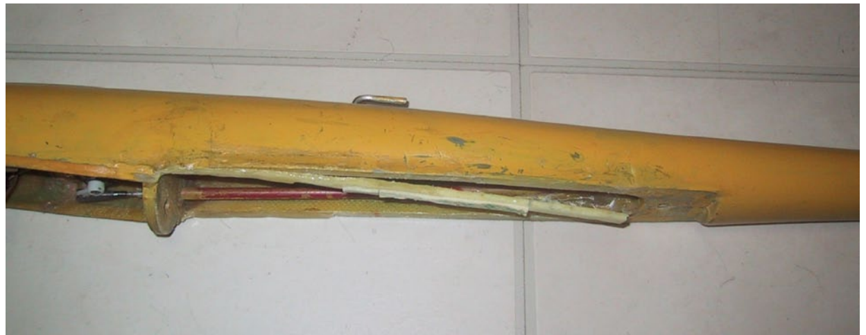
Illustration 5: The original fuselage had layers of epoxy repairs built up over the decades. If they could be seen edgewise it would be like looking at the stratified layers of the Grand Canyon. Removing them was like peeling an onion... from the inside out.
