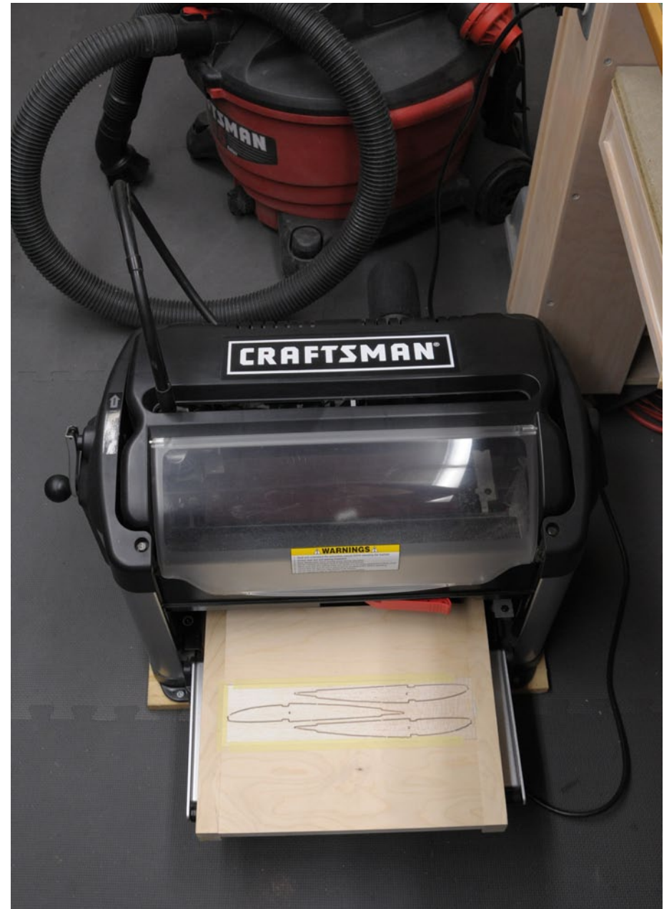
Wing rib cutting completed on Craftsman CompuCarve called the CarveWright by the company that makes them.
