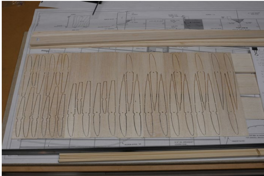
Wing rib sheets separated into individual sheets
