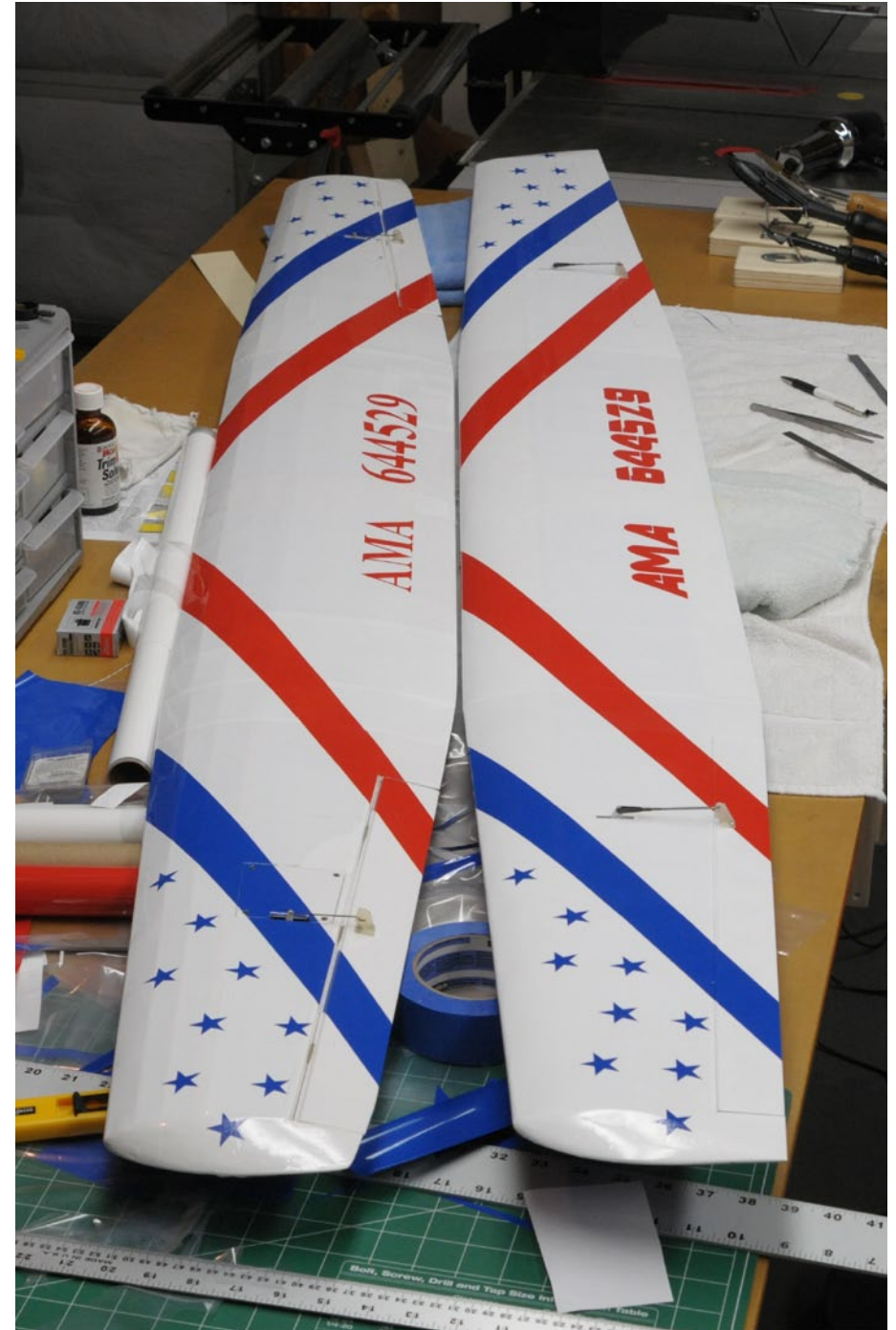
Original turbulated Bobcat airfoil wing on the left compared with new AG34 airfoil wing with increased polyhedral on the right.
