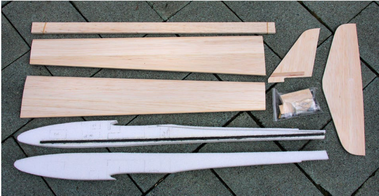
Magnum Models Duster kit contents. Note the balsa sheeting applied to the wings at the factory, with leading edge and sub-trailing edge stock glued in place. Also, the carbon fiber stiffening rod and elevator pushrod tube come installed. Suggested radio component layout locations are suggested as well.
