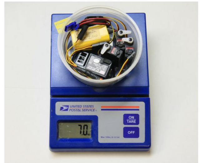
The on-board radio gear weighs 7.0 ounces. It could be lighter using modern 2.4 MHz receiver if the builder flew mostly in very light lift.
