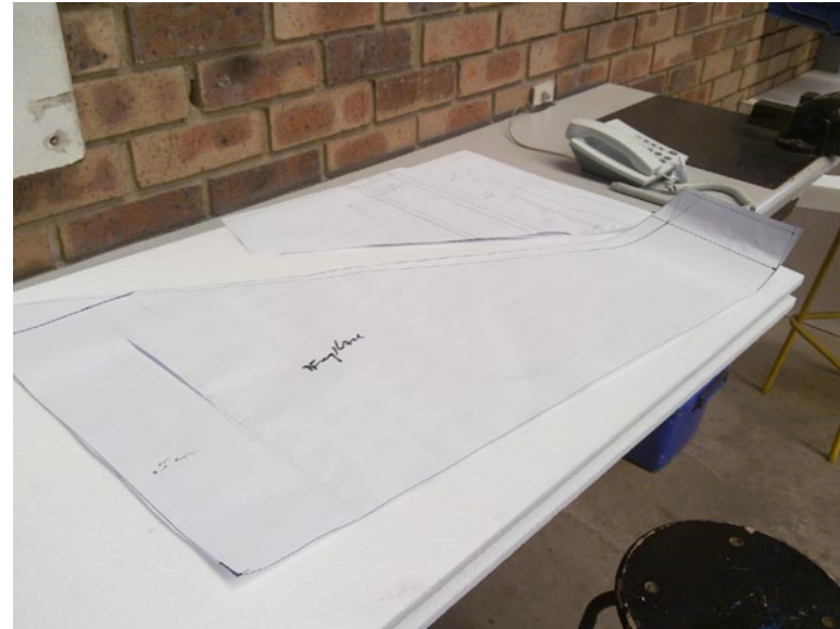
19. Wing block patterns. True scale was 1.4 m, I moved the tips out 15 cm each side giving a span of 1.7 m.
