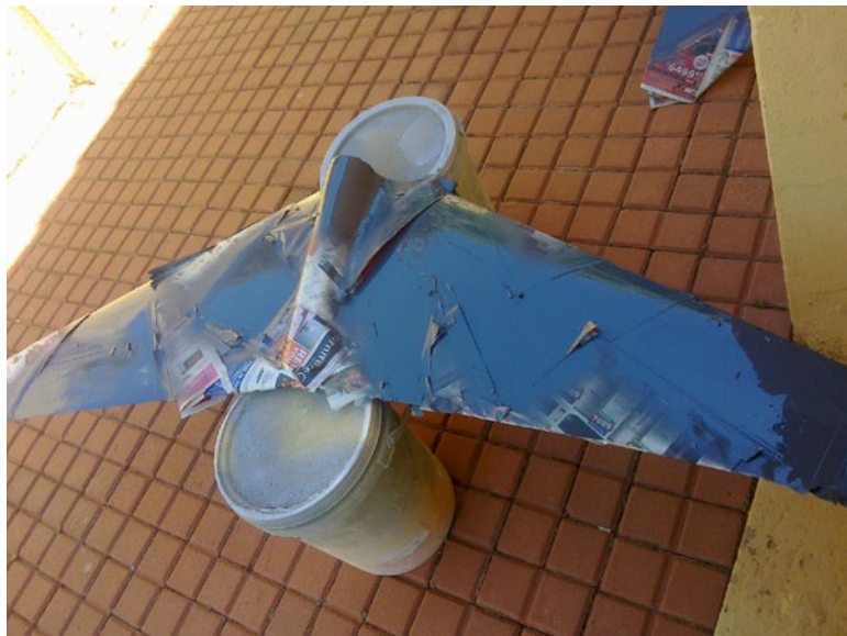
82. Mix up some dark grey paint and once happy with the shade mask again and spray.
