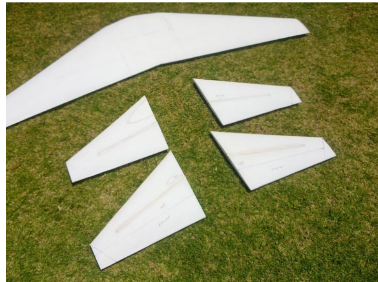
24. Tail feathers utilize a symmetrical section with "aerodynamic" leading and trailing edge, the middle is flat.
