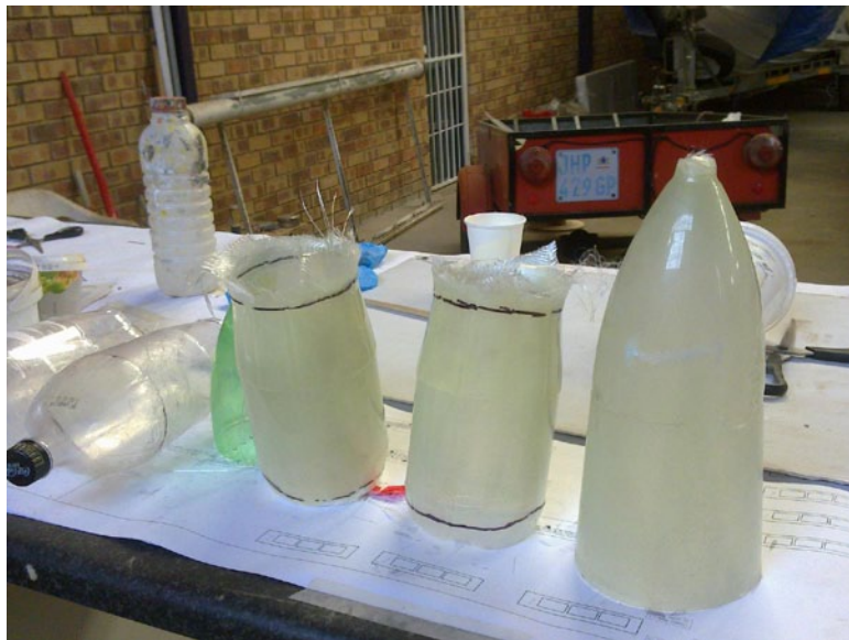
15. Waxed my plastic bottles and laid up some glass inside. Out popped some shapes.
