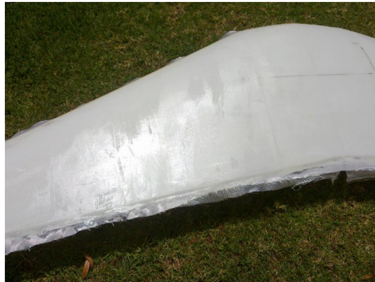
27. Now the top is glassed with cabosil in the resin. Rich shiny surface will be cut back before primer.
