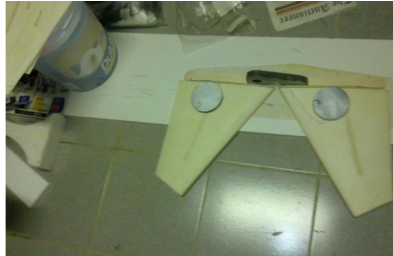
60. The tailfins epoxied on with strong epoxy. Note also that the tips have now been cut and shaped to scale.
