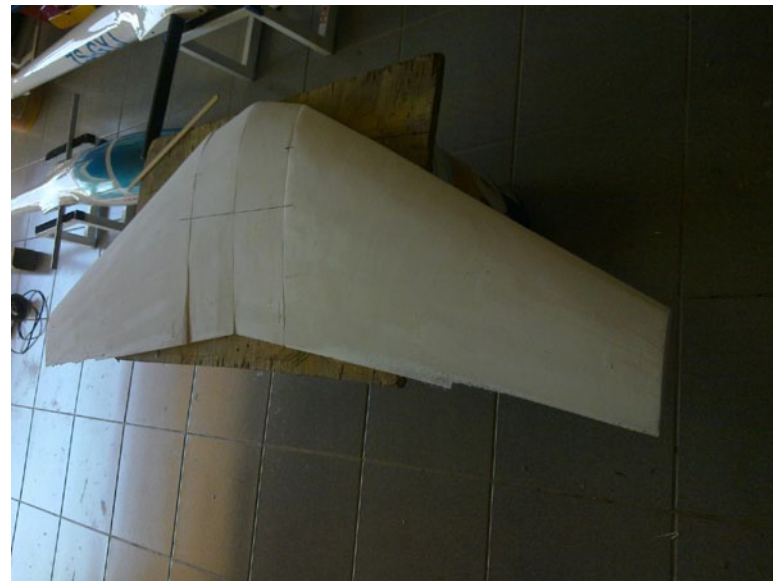
20. The raw cores joined with 5 minute epoxy prior to some sanding with a block.
