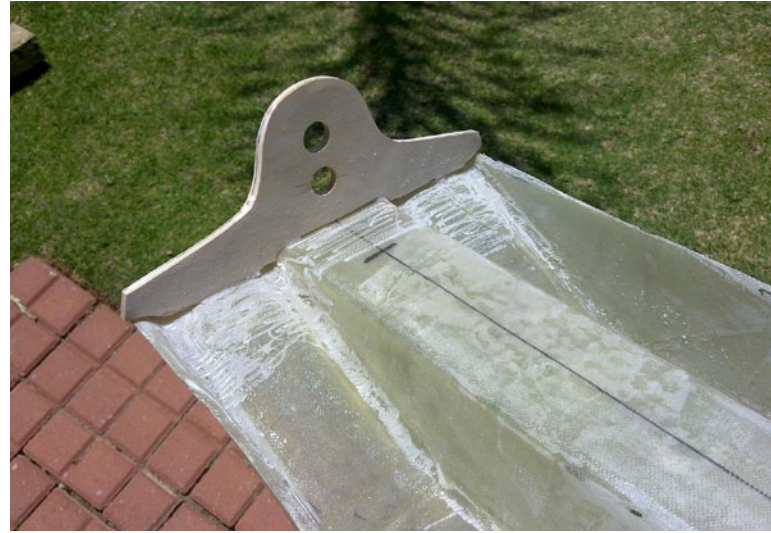
34. The plywood former is carefully sanded to match the glass shape and tack epoxied in place.
