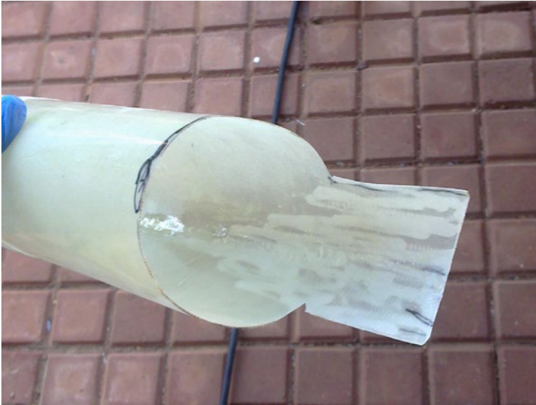
18. The fuselage tube molding which now matches the nose cone. All epoxy is cured with fast hardener and left overnight.
