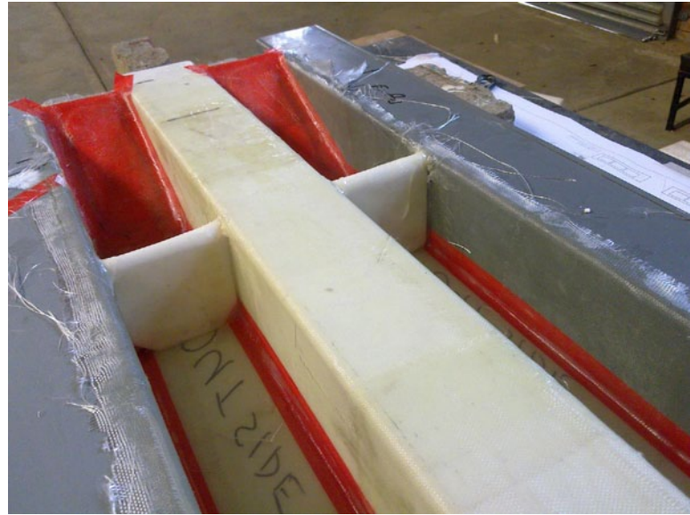
9. I have decided to glass in two temporary foam inserts to box and stiffen things.
