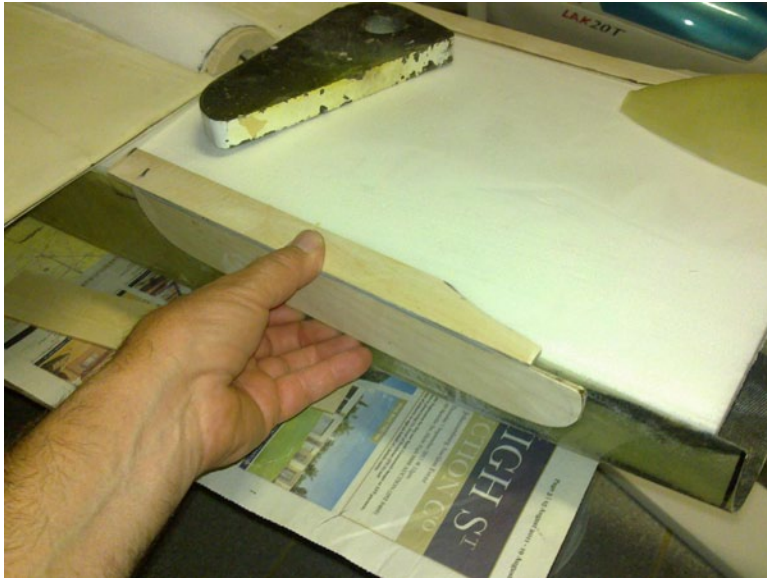
58. The plywood base which can move forward or backward on the square fuselage sides.
