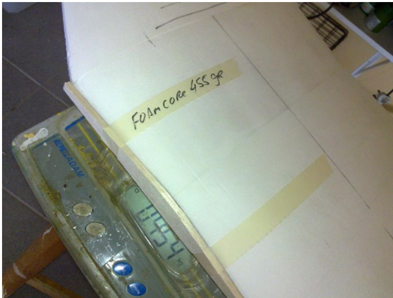
25. The wing is cut flat across the front at the width of the fuselage. Balsa piece glued to open edge.
