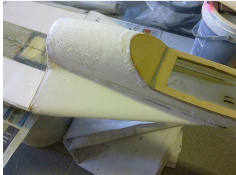
50. Finer sanding and some more filling around the canopy base.
