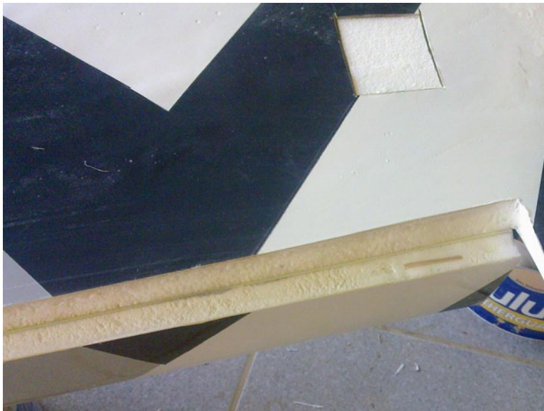
92. Control surfaces are cut out, the foam sanded back, and the edge V-shaped for movement. The dge has a layer of epoxy/flox scraped across it to the skins and there's a plywood insert for the horn.
