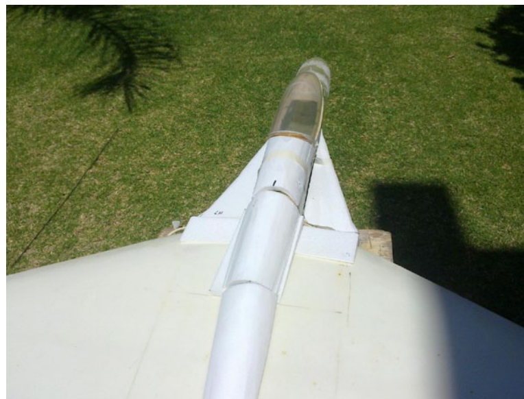
45. Added the web "strakes" and more to the fuselage ridge. Blocks smooth the entry up to the wing center section.
