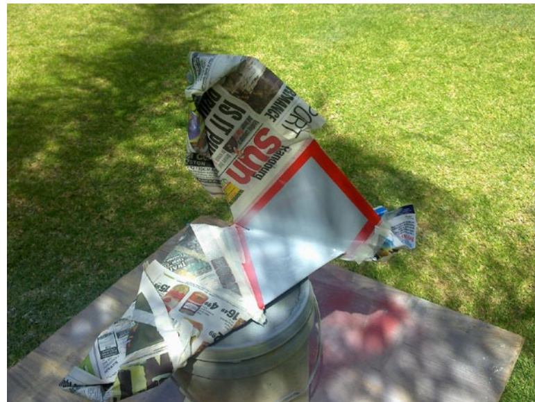
80. The whole aircraft is masked except for the white panels, trying to emulate the original closely.
