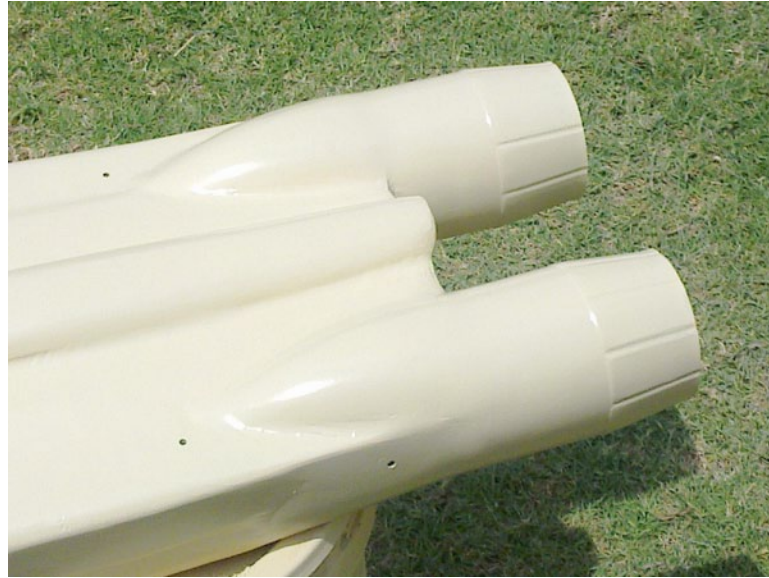
74. The fuselage primed.
