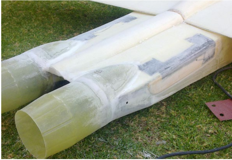
70. Added another piece of carbon cloth just ahead of the engine for the third attachment point and glassed on a piece of plywood to the fuselage sides.
