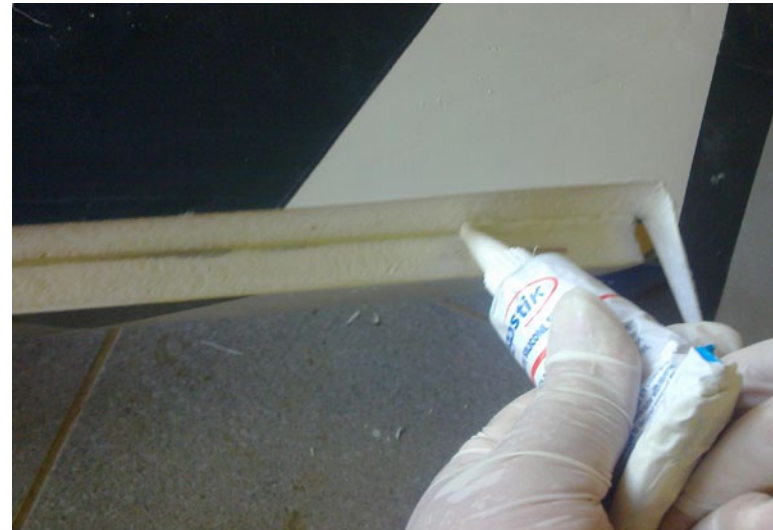
94. Control surfaces use a silicone hinge.
