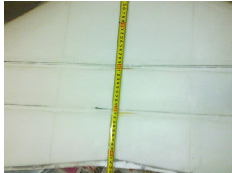
23. Important to record the exact positions of the spars shears as I want the servos between them.
