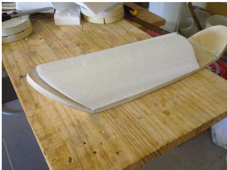
43. Some plywood blocks epoxied onto the top of the wing outside of the spars. These will be drilled and captive threaded nuts installed.
