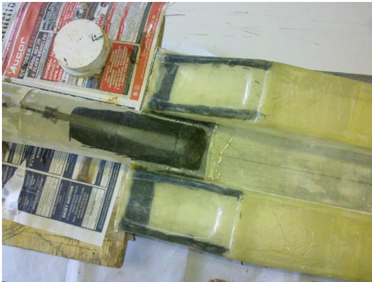
41. Glassing the tube to the plywood former. Two 200 g carbon again for strength, tacked and aligned with 5 minute epoxy first.
