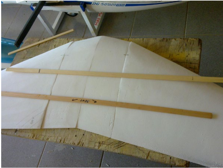
21. The spruce strips to stiffen up the wing.
