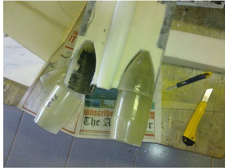
64. The foam is cut to the cone shape.
