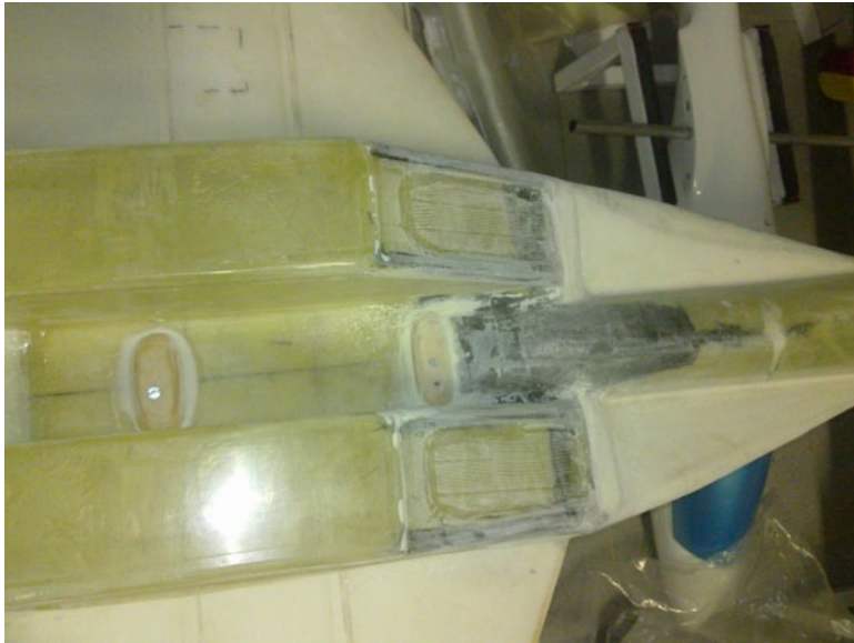
56. The two plywood bolt holes are reinforced and the edges all filled with micro balloons mix and then glassed.
