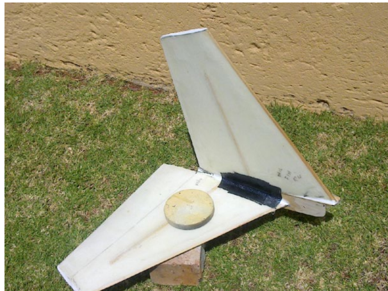
60. The tailfins epoxied on with strong epoxy. Note also that the tips have now been cut and shaped to scale.
