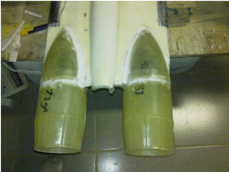
66. Some epoxy balloons to bond things in place and fill gaps.
