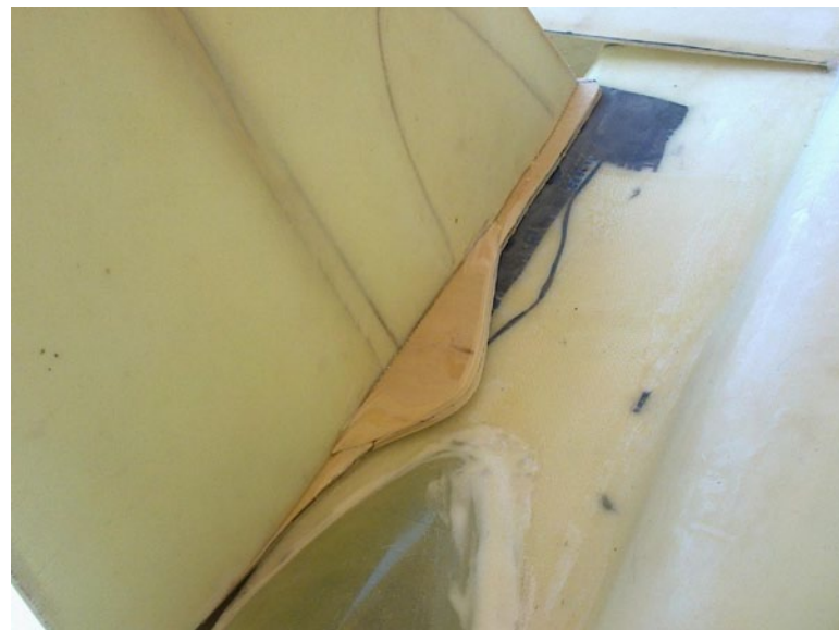
69. Sanded, the plywood clears the engine. This made the tail assembly stable. A piece of carbon cloth will add rigidity.
