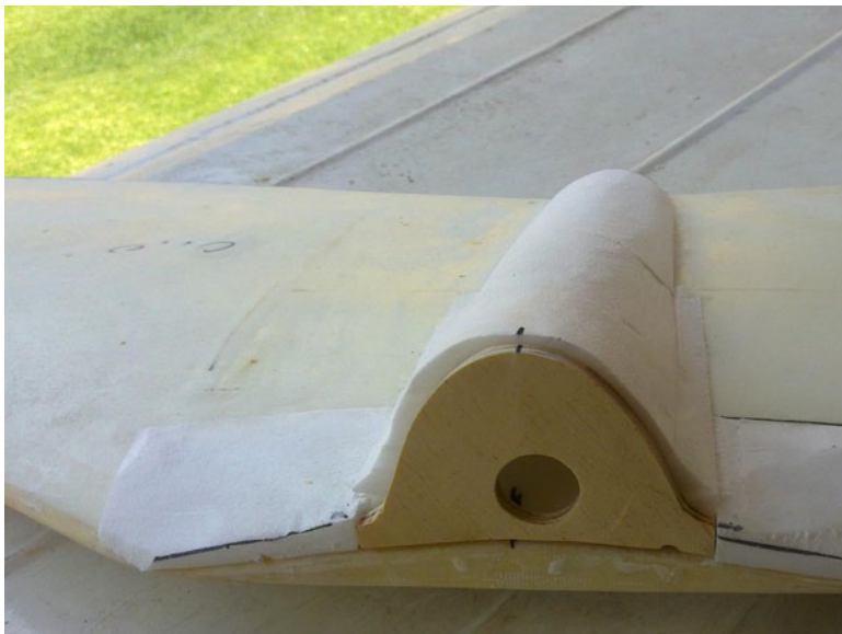
49. The hollow fuselage foam ridge is glued on. Provides wiring access. Captive nuts are inside.
