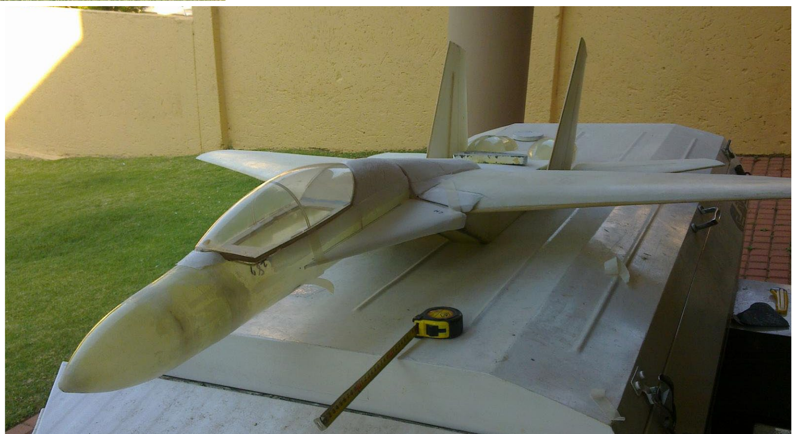
47. Some basic sanding of the foam and things are starting to shape up.
