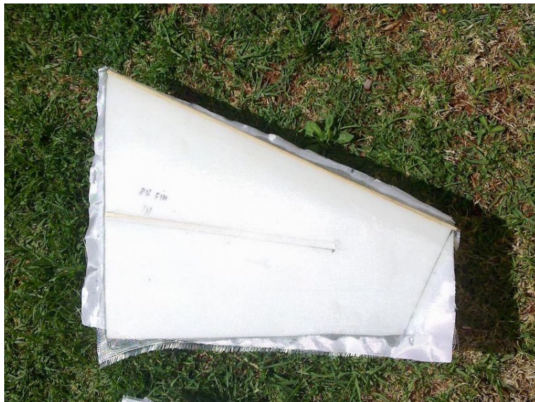
29. In this picture you can make out the 3/4 span balsa spine.
