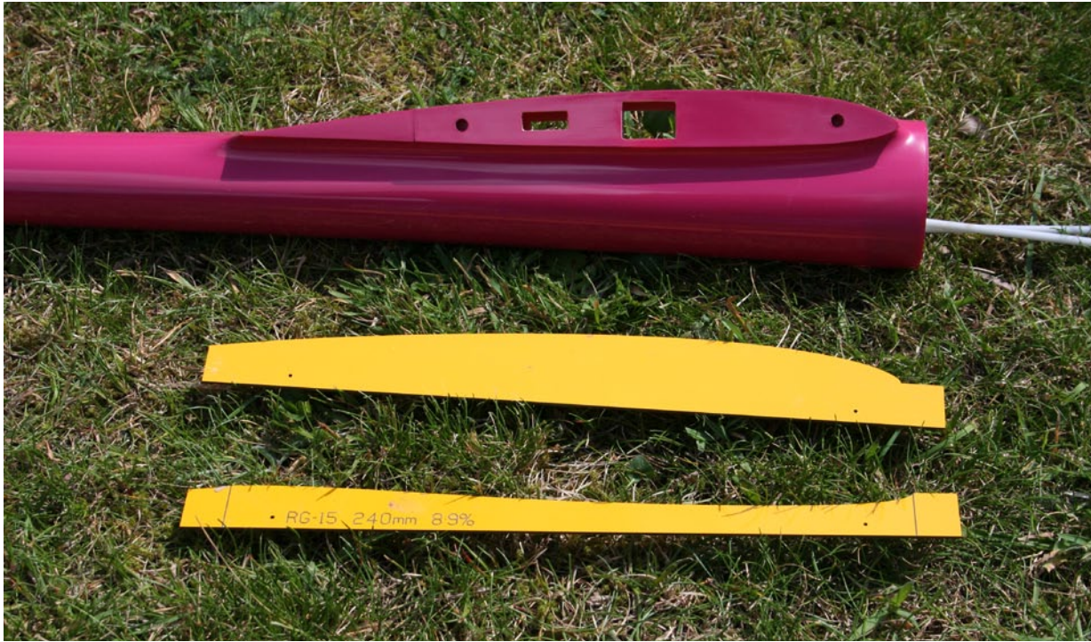
Mike Francie's wing templates are an excellent way of making wings. You can see the fuselage parts with the same profile.
