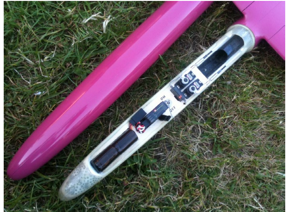
A simple, strong fuselage with ballast tube.
