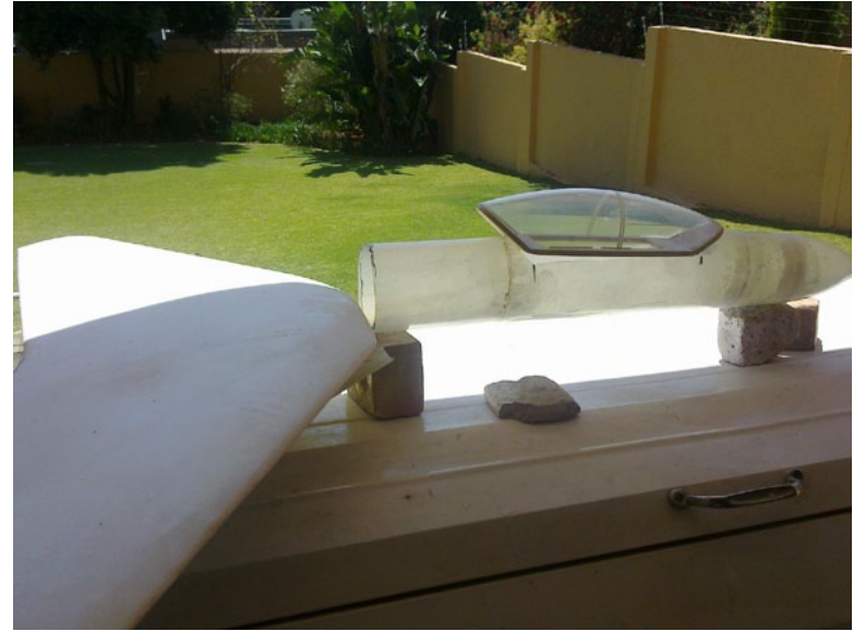
30. Back to the fuselage...Here you see the rough canopy position, the fiberglass tube and nose, and the wing.
