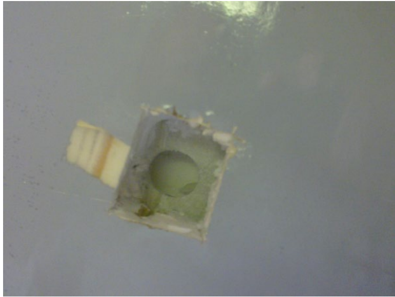
95. A hole is cut through to the fuselage tunnel. Masked spar position now clearly visible. Round hole is the top skin.
