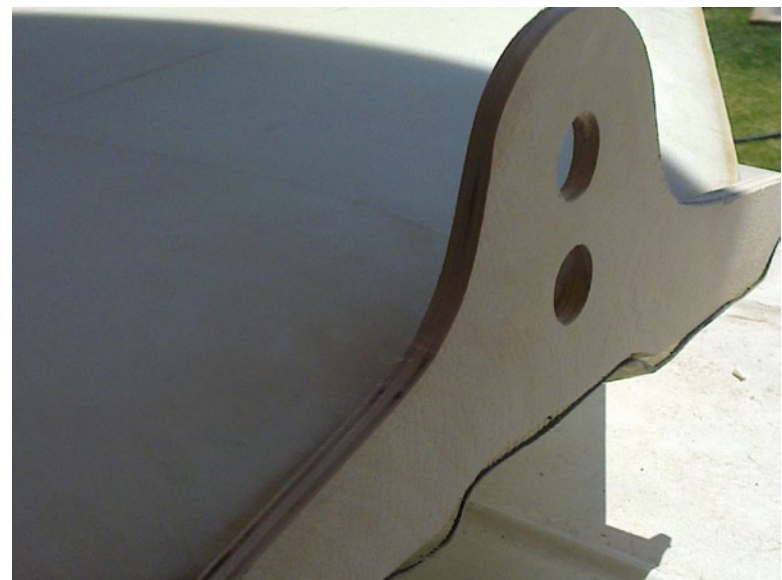
31. In front of the flat section of the wing will come this strong plywood former. The holes are for servo leads and access.
