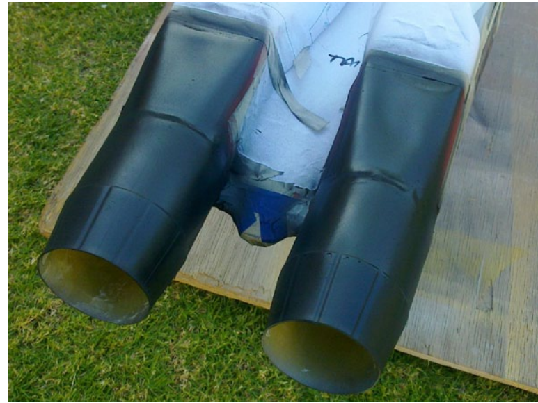
87. More hardener, no thinners, and spraying from a distance gave the normal 2k gloss a matte black finish for the tailpipes.
