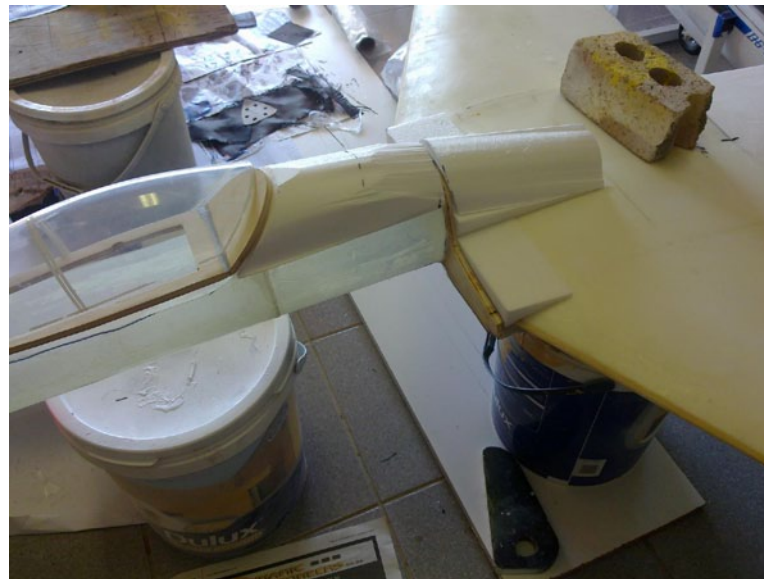
44. The correct foam infill behind the canopy and starting the foam on the fuselage section of the wing. Hollow for wiring.
