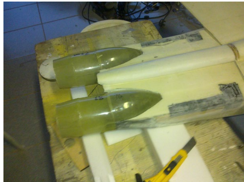
65. The jet outlets and cowls tacked in place.
