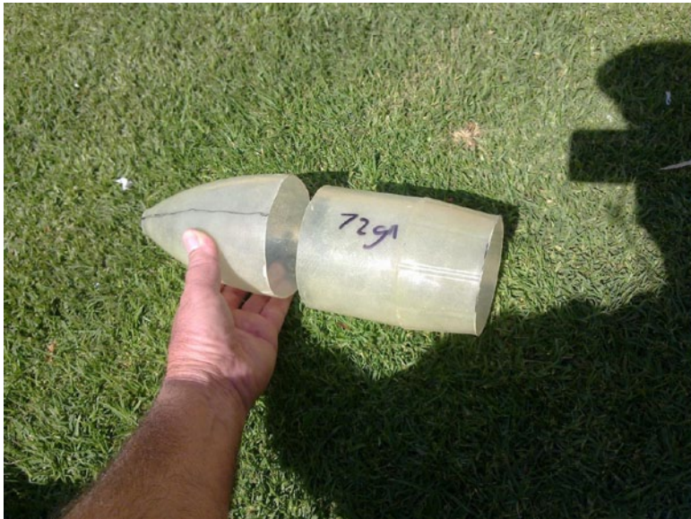
62. The Coke bottle jet exhaust molding and the green bottle nose cone molding.
