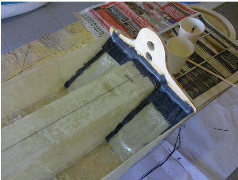
37. Still wet, two layers of 200 g carbon cloth is glassed in. I was concerned this might be a weak spot with a one piece wing.
