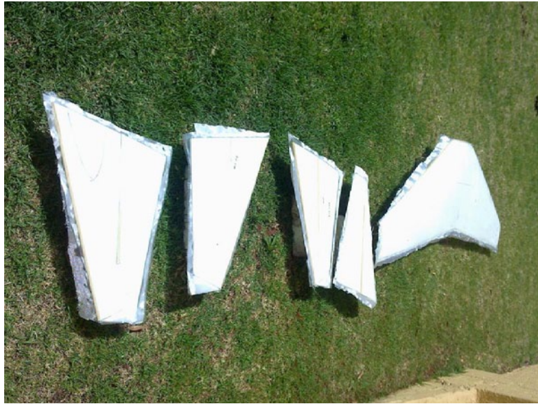
28. The smaller tail feathers are laid up with two layers of 104 g cloth with resin/cabosil mix on outer layer.
