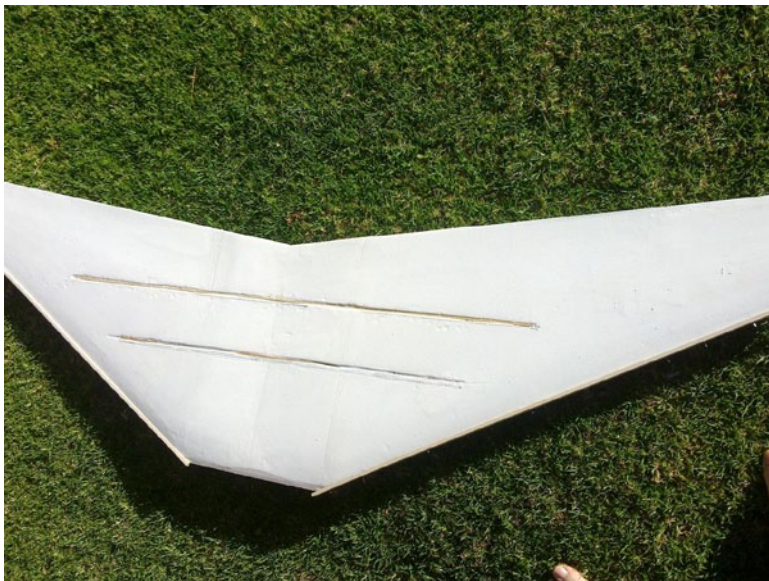
22. The spruce bonded into the slots with a resin and flox mix. I also added balsa strips to the leading edge.
