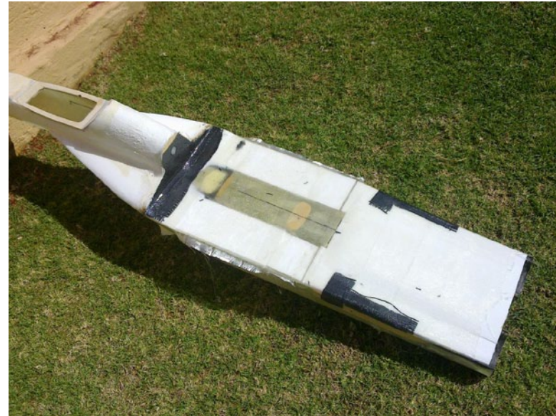
54. Foam back from the trailing edge. Sanded to shape, slopes slightly downward. Carbon where tail feathers attach.
