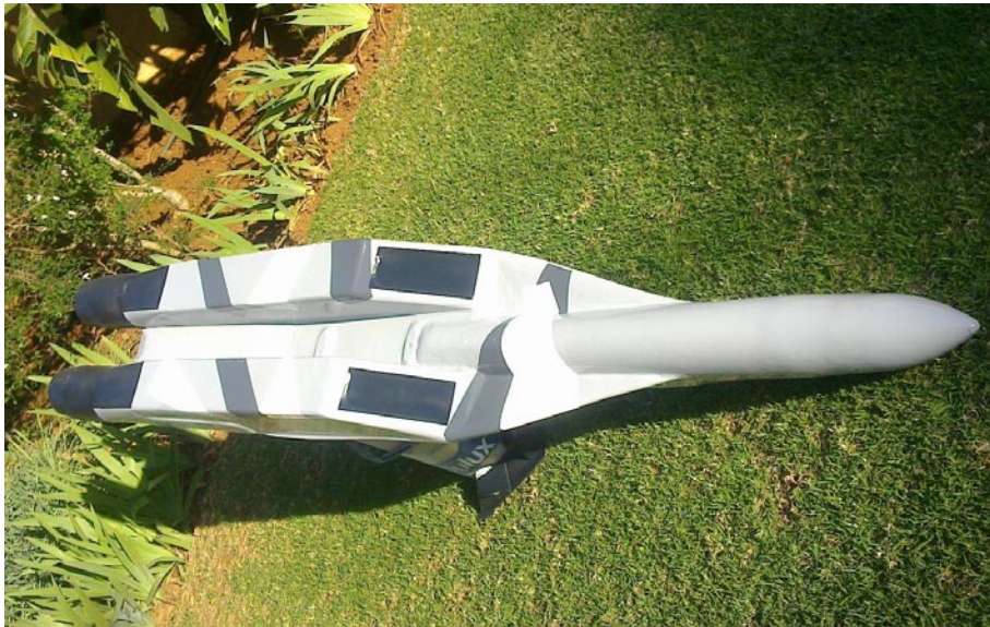
89. Intakes are painted. Someone asked about cutting them out and letting the air through, but that would increase drag.
