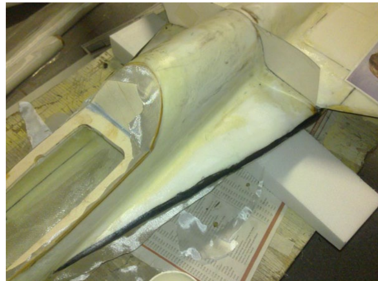
55. The "canard web" gets a carbon tow edge and is glassed.
