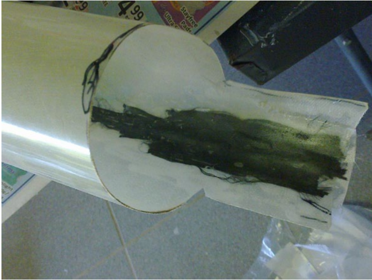
40. Adding tows and shaping the fuselage tube.
