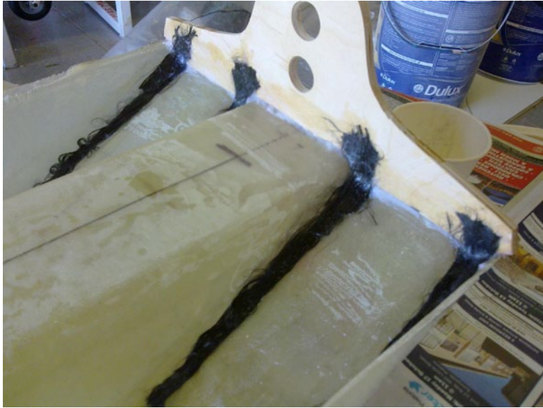
36. Some flox and resin in the joint hollows, then 48k carbon tows are laid in wet.
