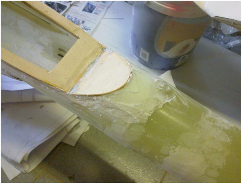
52. The front of the canopy is faired into the nose.
