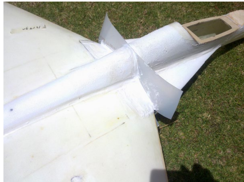
51. Using mylar on the split line. Micro balloons and flox mixed with epoxy is used to fill both sides to the break.
