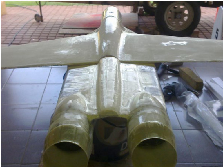
71. Started final filling which is epoxy/microballoons and some cabosil for a harder finish.
