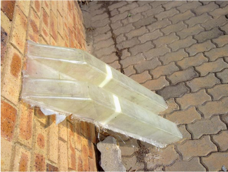
11. The first molding popped out and awaiting trimming. The jet motor intakes basically form the foundation.
