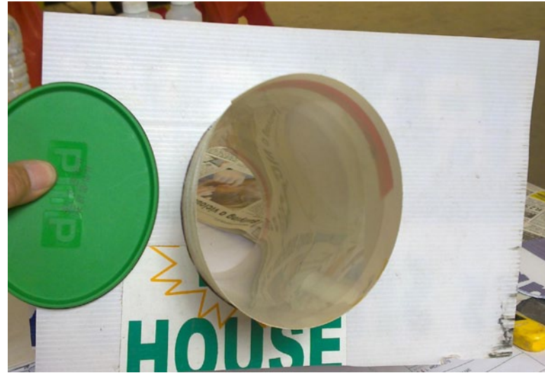
16. A yogurt container lid was used as a template and two end plates of Correx made with a mylar oval tube taped in place.
