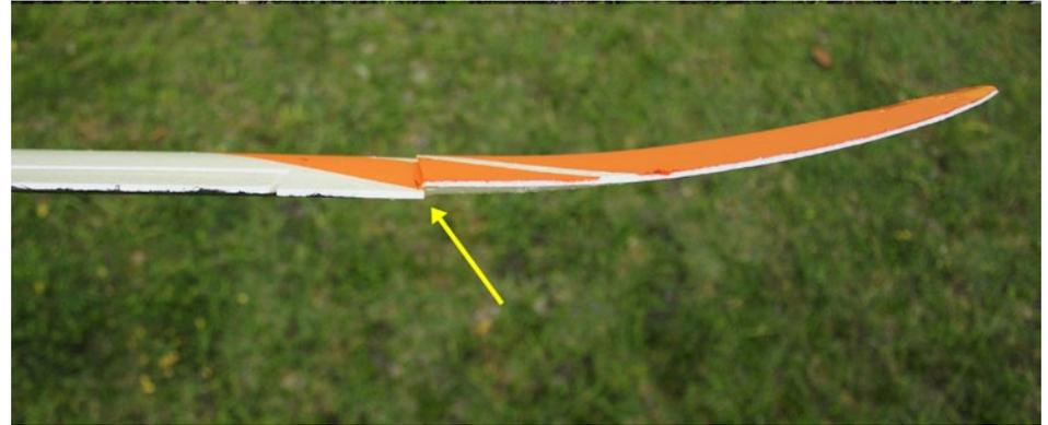
*Above: 1° was imparted into the wing tip using epoxy to reglue the joint.*
