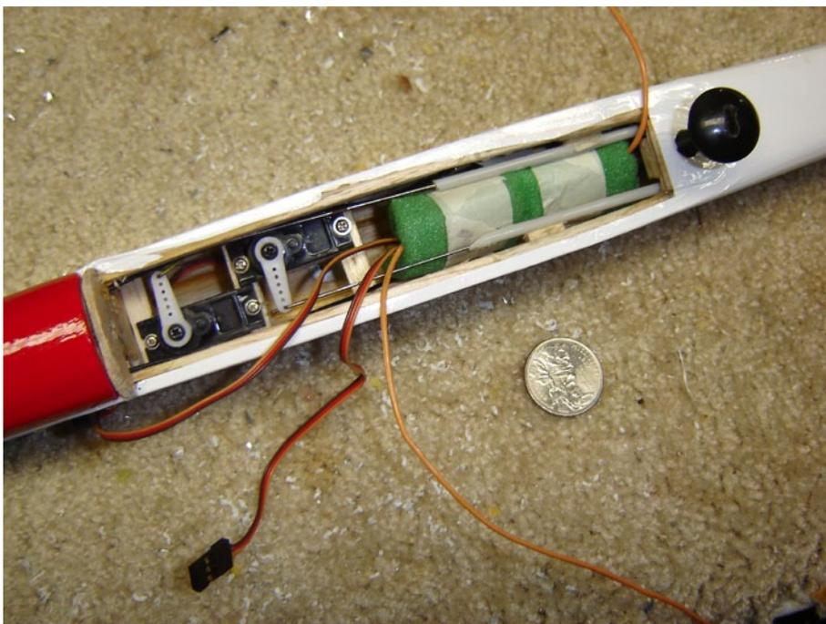
*The Scout and transmitter are wrapped in green foam and stuffed behind the servos. The aircraft is a 1.5 meter Skeeter sailplane. The addition of the Scout did not require the ship to be rebalanced. A quarter lays next to the fuselage for size comparison.*
