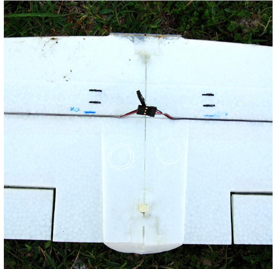
*Final location of the CG, 2 mm in front of the aileron wires.*
