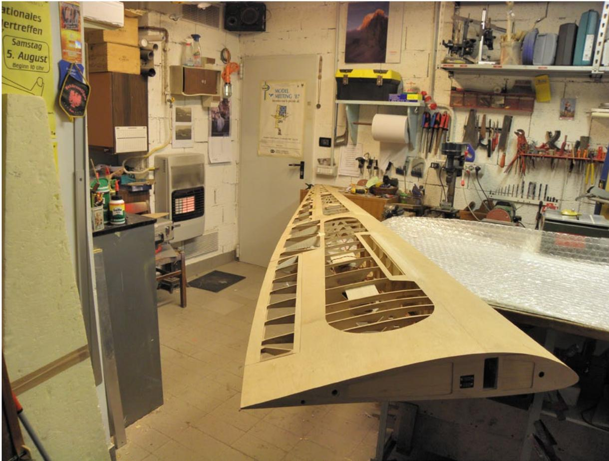
*The extra-large wing in the construction lab.*
