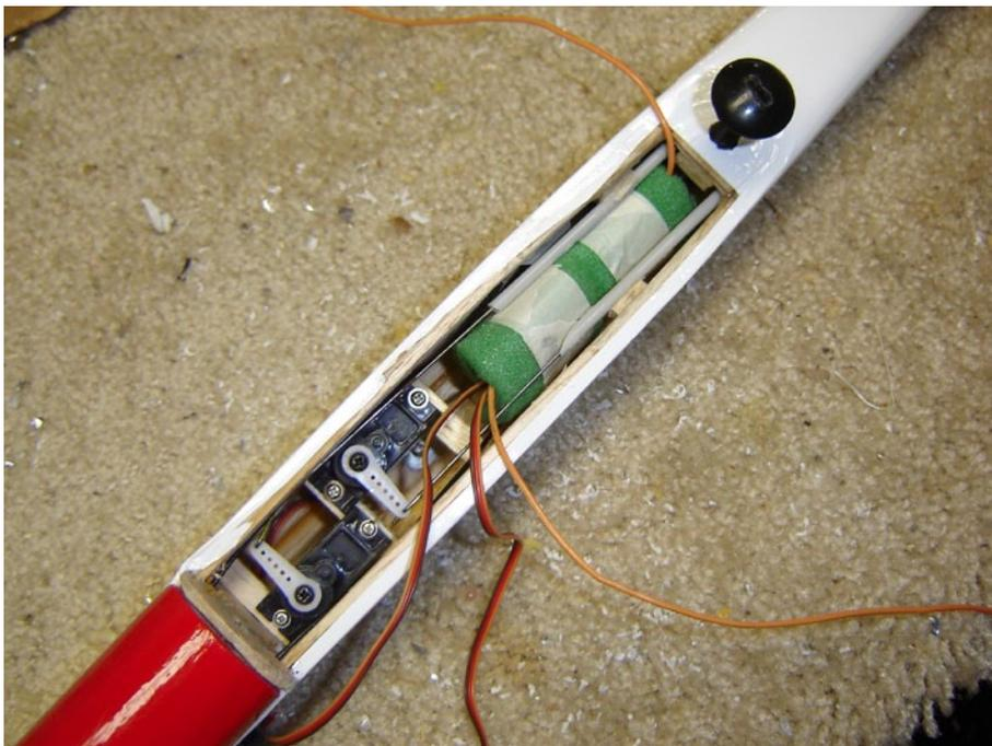
*The two orange wires are the Scout transmitter antennas. They should be taped to the bottom of the wing in a "V" pattern for best reception on the ground.*
