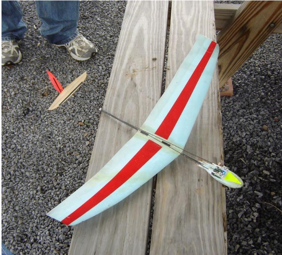
*A homebrew 36 inch span HLG was flown to check the fog ceiling. It has the radio from a Night Vapor and uses carbon pushrods. The front pod is soft styrofoam. Rotary launches resulted in the ship rolling inverted at max height but then it would roll out. This may be a whole new way of launching HLGs without a mixing type radio.*
