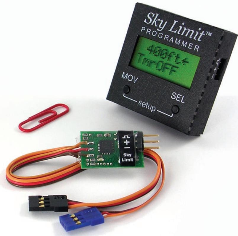
The Sky Limit consists of two separate parts, the airborne unit and a programmer. You don't need a PC to program the Sky Limit but you do need the programmer. It cannot be programmed, as some other limiters are, by moving the transmitter sticks or with a PC. However, one programmer can be used with any number of airborne units. So for example, a club could order as many airborne units as desired and just one or two programmers to share between the club members.
