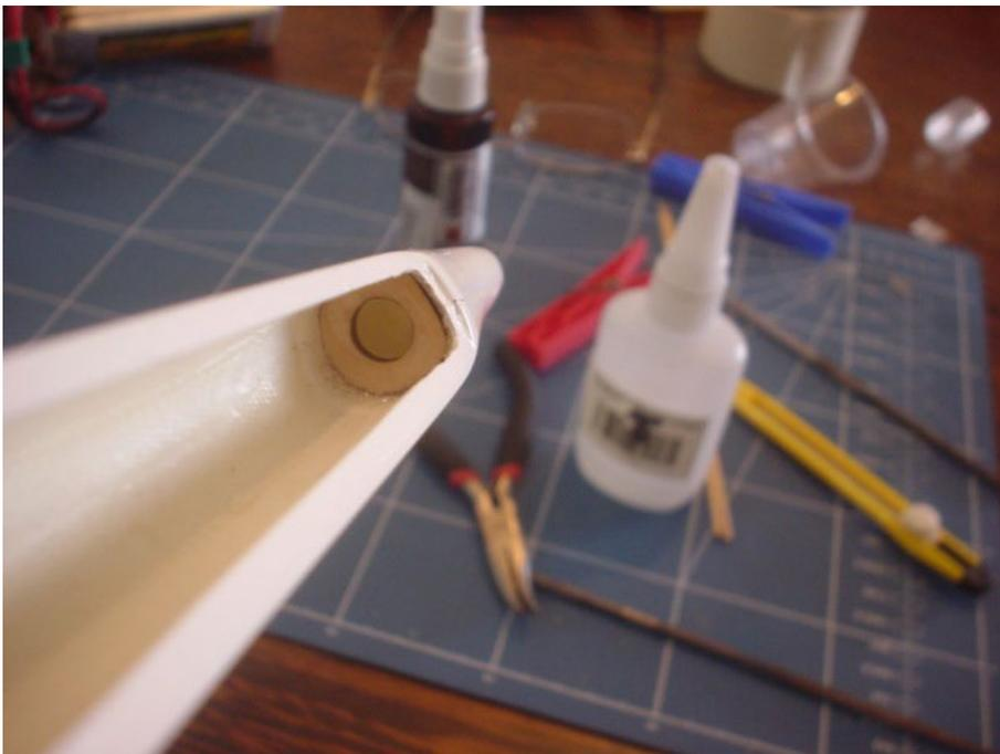
then re-assembled the wing, pod and boom again on the table. When all was leveled, centered, checked, and double checked, I drew a mark from the pod on to the boom. I dribbled some medium CA where the boom meets the pod and fixed it with a shpritz of kicker. Then, with thin CA, I saturated the ply ring inside the fuse to fix the boom permanently. I let this cure by itself (no kicker here!).
