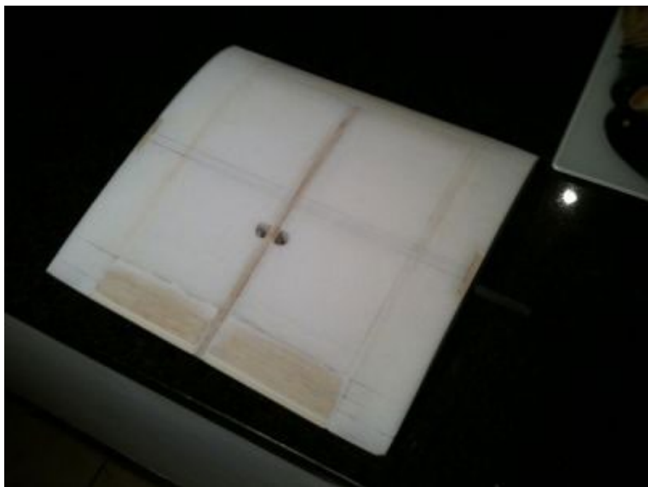
Above: Center wing panel being joined with servo lead holes in place.
