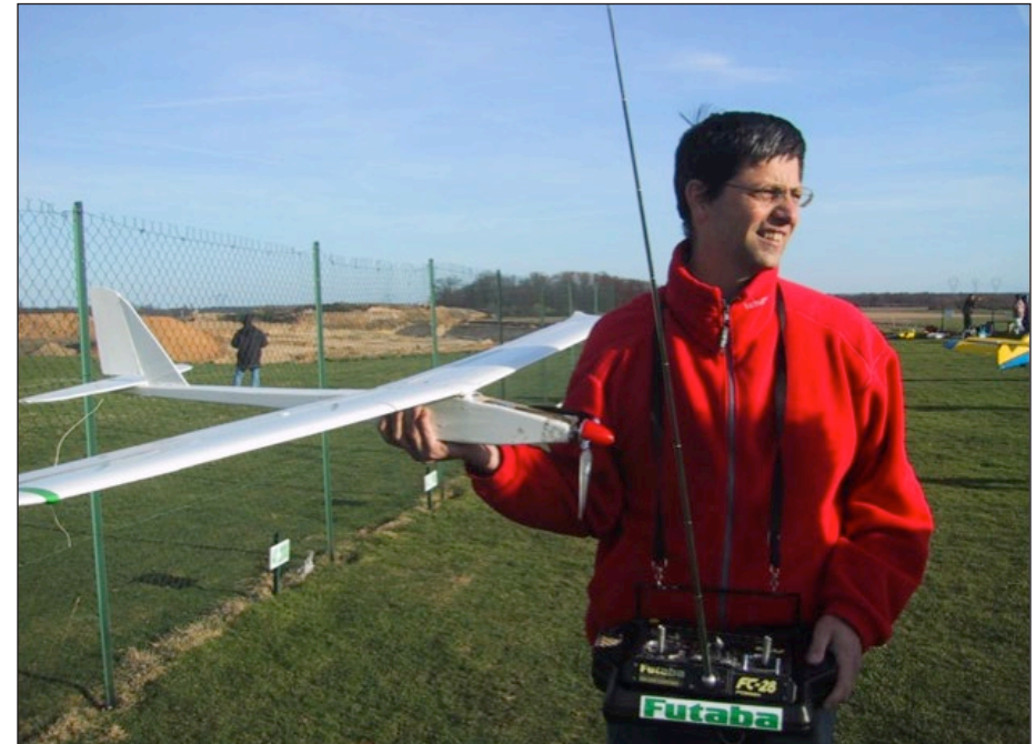
A 2 m airplane with a 200 W brushless motor and a controlled pitch angle propeller. This was in 2002.
