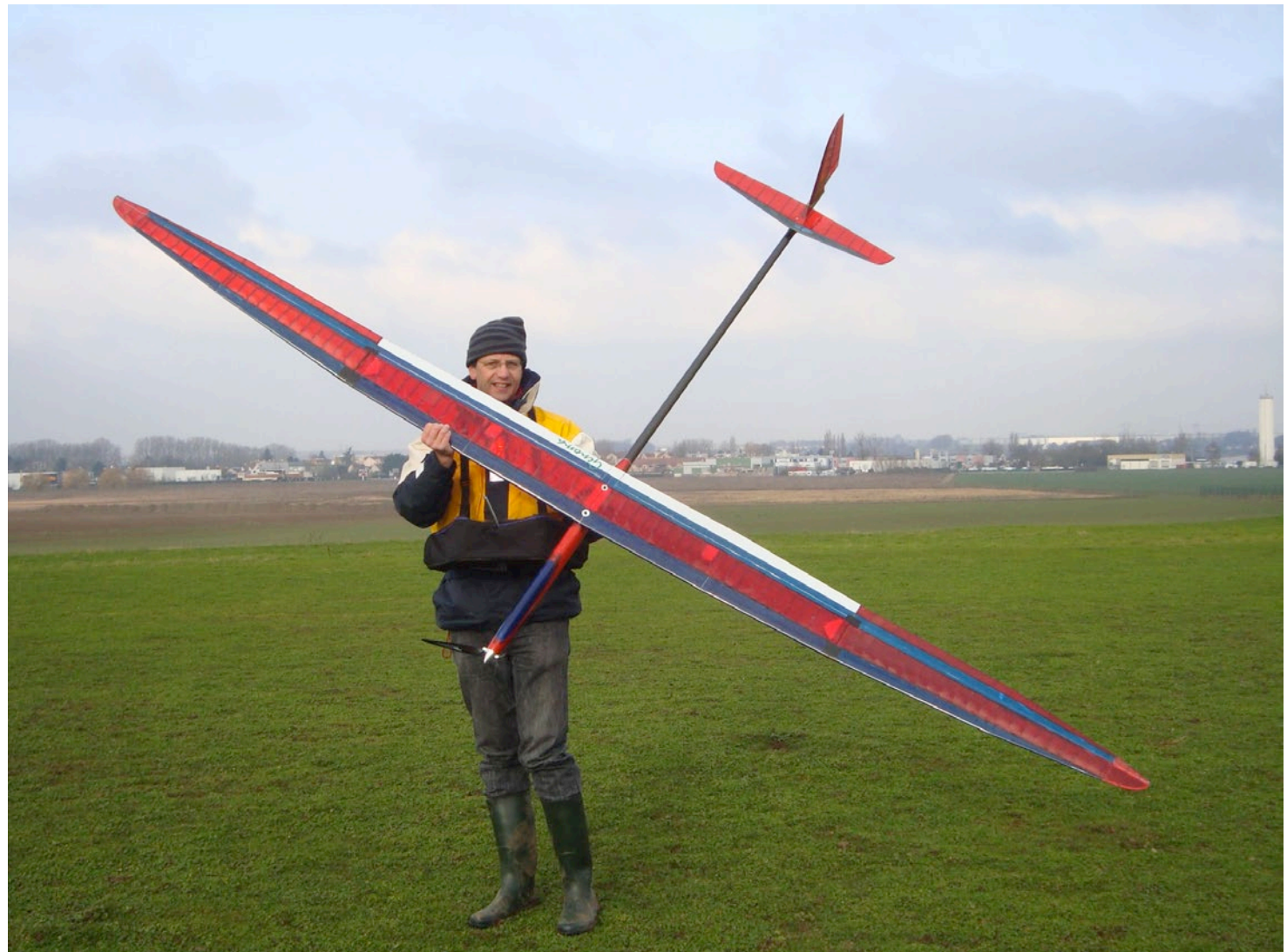
Figure 30: First flight of the Genoma (First version) was in January 2010. Since that time, this 1.9kg plane flies every week without trouble. It even succeeds to flying three minutes alone (without any control due to an electrical problem) and crash in a field after a 50m dive without any destruction. So light and so resistant!
