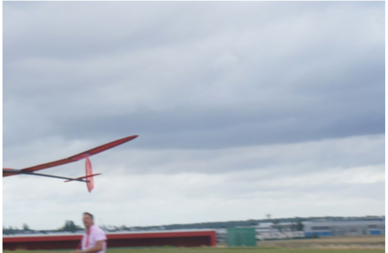
Figure 33: Genoma 2 for its first flight. Except few adjustments, it flies perfectly and I found immediately comfortable. It is even better in circling ability due to the possible low wing load (19g/dm 2 without ballast). Of course things needs adjustment (compensation, trim...).
