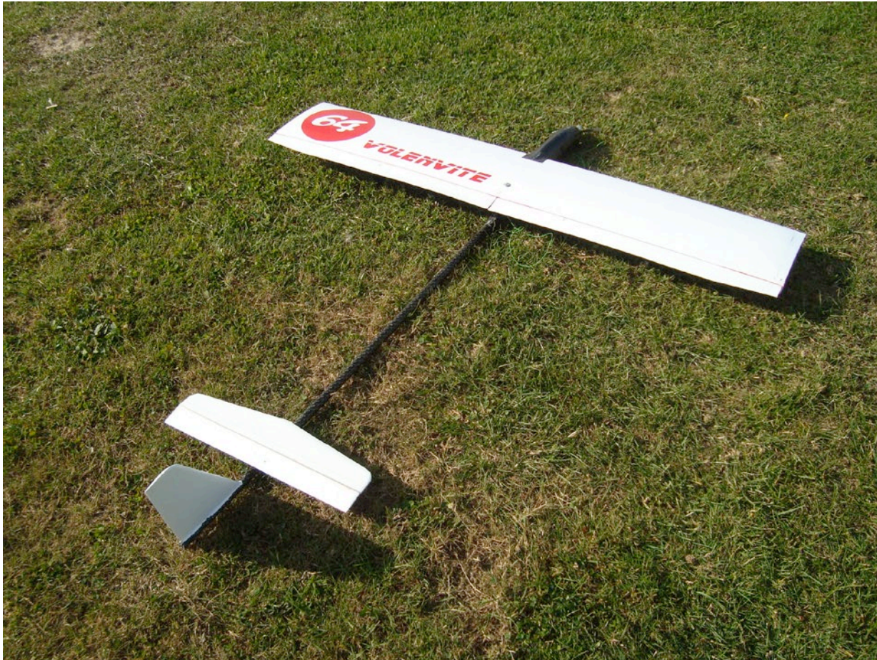
Figure 34: A small racer (1m span, 300w only) where the fuselage length is longer than the span. Despite the fact that this configuration disturbs our minds, it is not so unusual for real racing planes. The fuselage increase allows us to reduce fin and tail dimensions (and then drag) and to increase the stability. Flight is like an arrow — "on a rail."
