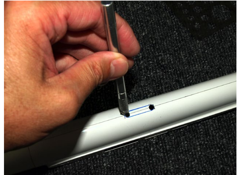
Twisting the knife: the easy way to drill holes in composite skins.
