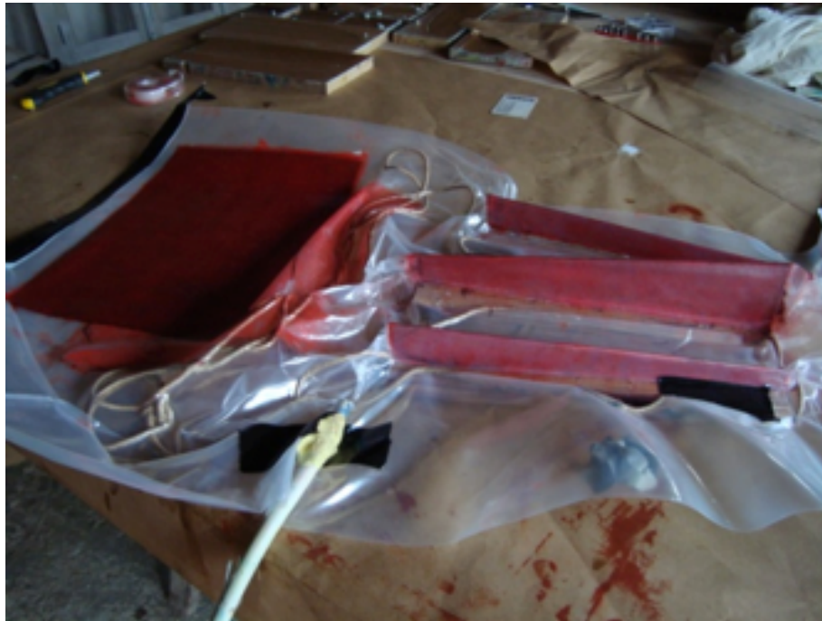
Figure 15a and 15b: How to mould the D-boxes? Easy. On a positive mould. Not much science behind this. For the wing, two layers of Kevlar of 60g/dm 2 is fairly sufficient (the wing can
