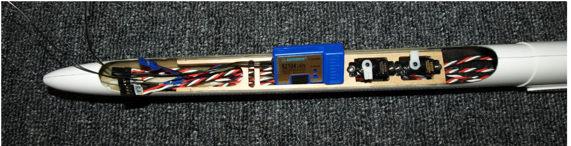
Laying out radio gear. Space is very tight so plan ahead for clevis clearance and nose weight.
