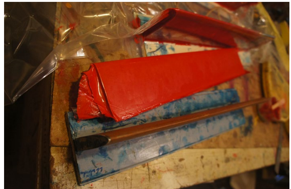
Lower right, Figure 23: View of D-box mold under process. On top, you can see the D-box bagged, in the center the D-box results and in the bottom of the picture the D-box mold.
