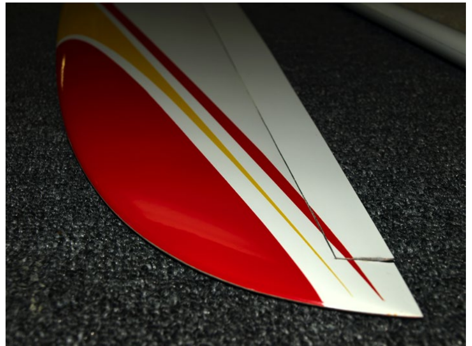
Above right: Top hinged aileron wiper. Lower skin recessed for servo cover with integrated pushrod fairing.
