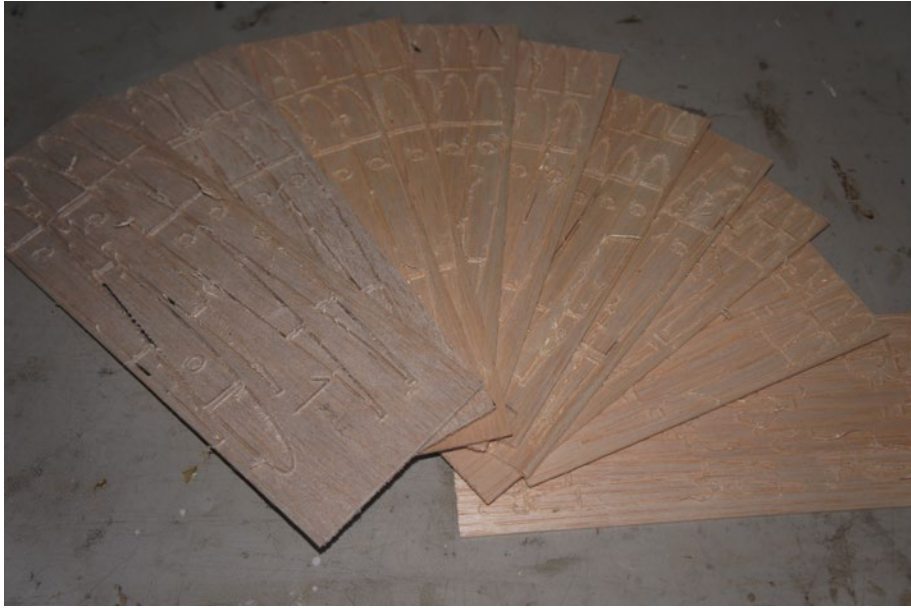
Figure 19: All balsa wood pieces have been realized on a CNC machine. Of course, on request, files can be provided.
