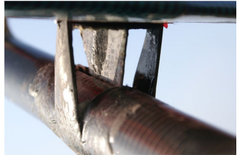
Figure 25: The details on how to fix the tail. Very similar as the Supra / Bubble Dancer ... Except that here, everything is inside the boom. Everything is made with very rustic moulds (and easy to be made). Nothing difficult!
