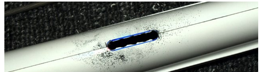
Drill a few more holes then clear it out with a chainsaw file.
