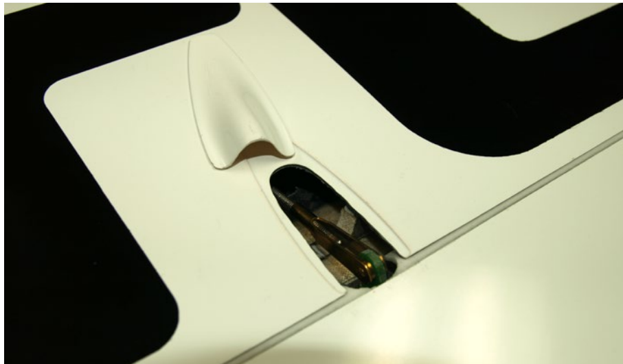
Flap pushrod installed. These are Sullivan clevises and 2-56 threaded rods rather than the supplied hardware.
