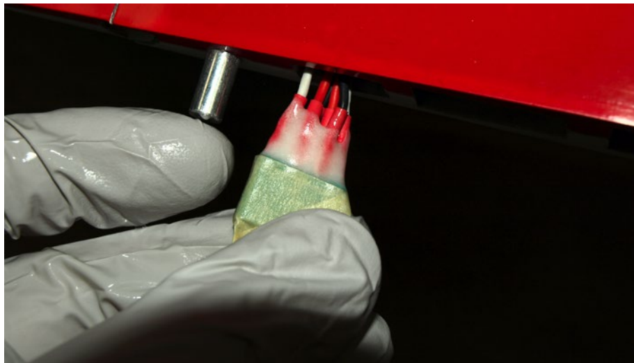
A little alcohol on a glove allows neat smoothing and shaping of thickened epoxy, here to firm up and protect the wires where they'll be handled during assembly/disassembly.
