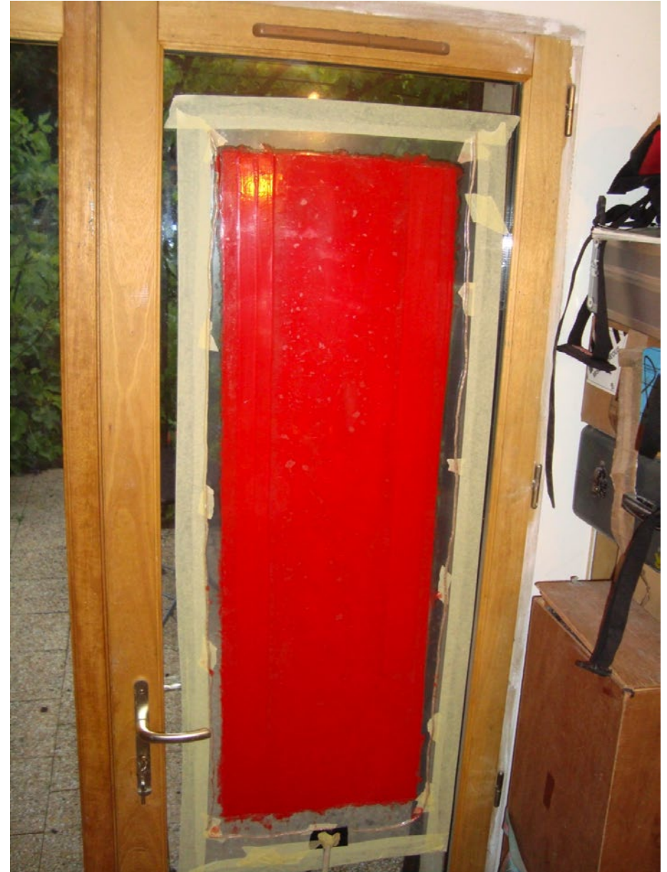
Figure 20: How to mould the flap and aileron D-boxes — on a window! Do not forget to “wax” it.
