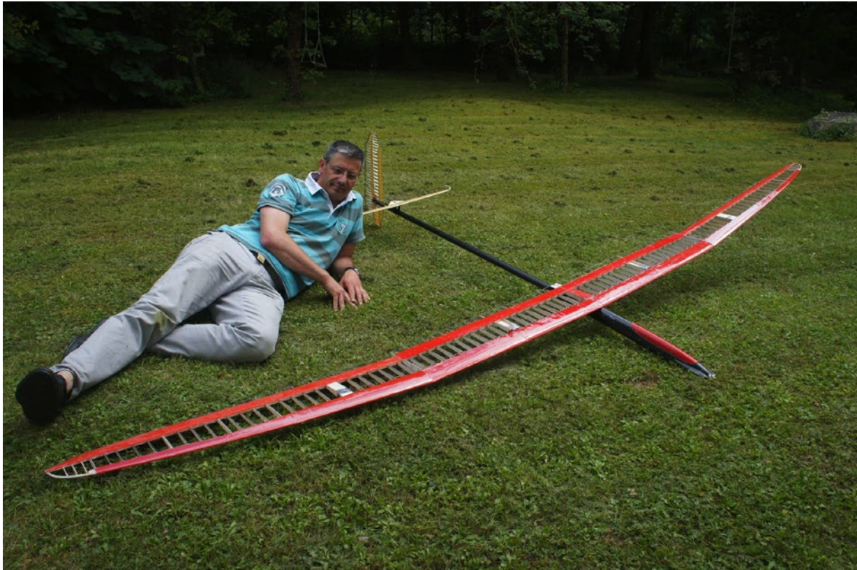
Figure 31: The man is 1.93m long. Quite a plane, no? The Genoma 2 weighs 1.6-1.7kg. It is 300g lighter than the Genoma for greater span and surface... The Genoma 2 is also able to make the barrel rollss in circles or any other aerobatic maneuver.
