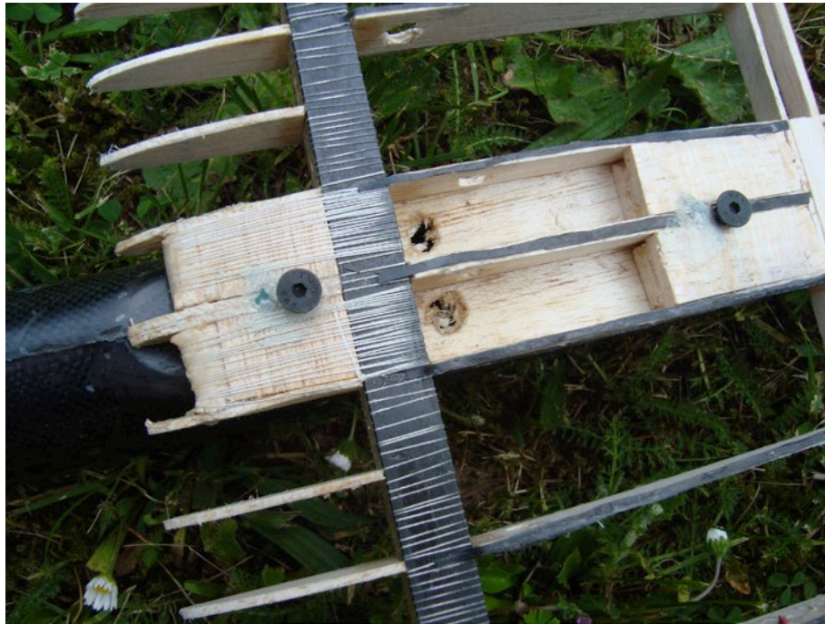
Above, Figure 21: Few detail of the wing to fuselage assembly system.
