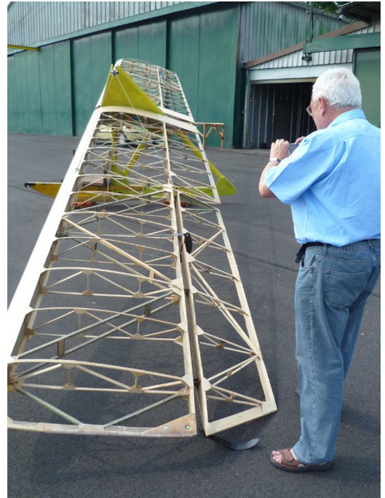
Ready to be covered.
