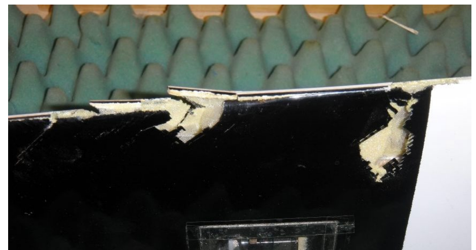
Bottom surface of the wing showing the two fracture points and the separated leading edge.
