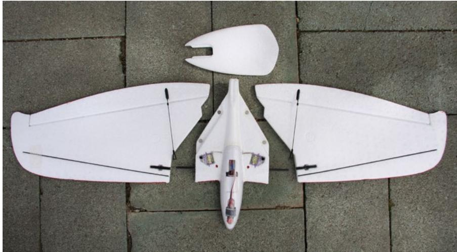
*Alula Evo airframe disassembled for transport, under side.*
