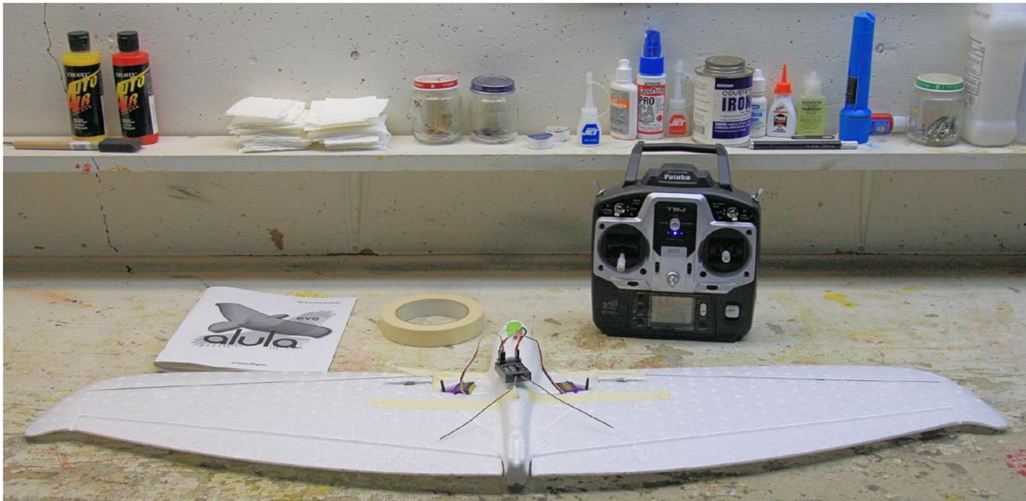
*Servos and receiver preliminary radio setup check. The Futaba T6J makes quick and easy work of setting up elevons that have small elevator throw and large aileron throw.*
