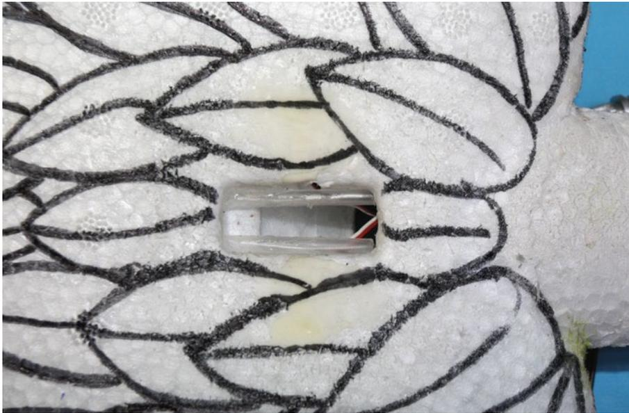
*Antenna tubes for dual 2.4 antennas installed along the sides of the opening at the center of the wing, view of upper side.*
