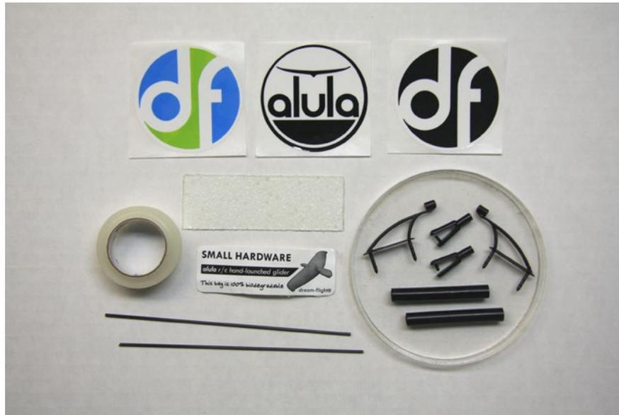
*Small parts include choice of decorative decals, clear “gripper” tape for tip-launch finger hold, wonderful 3M Blenderm tape, elevon control horns, matching clevises, CF elevon pushrods, and CF tube joiners.*
