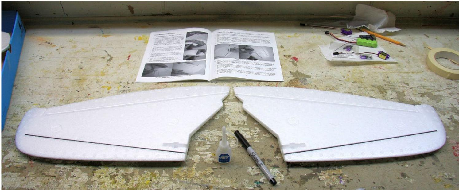
*Begin construction by installing CF strip wing spars into molded slots and securing with thin CA glue.*
