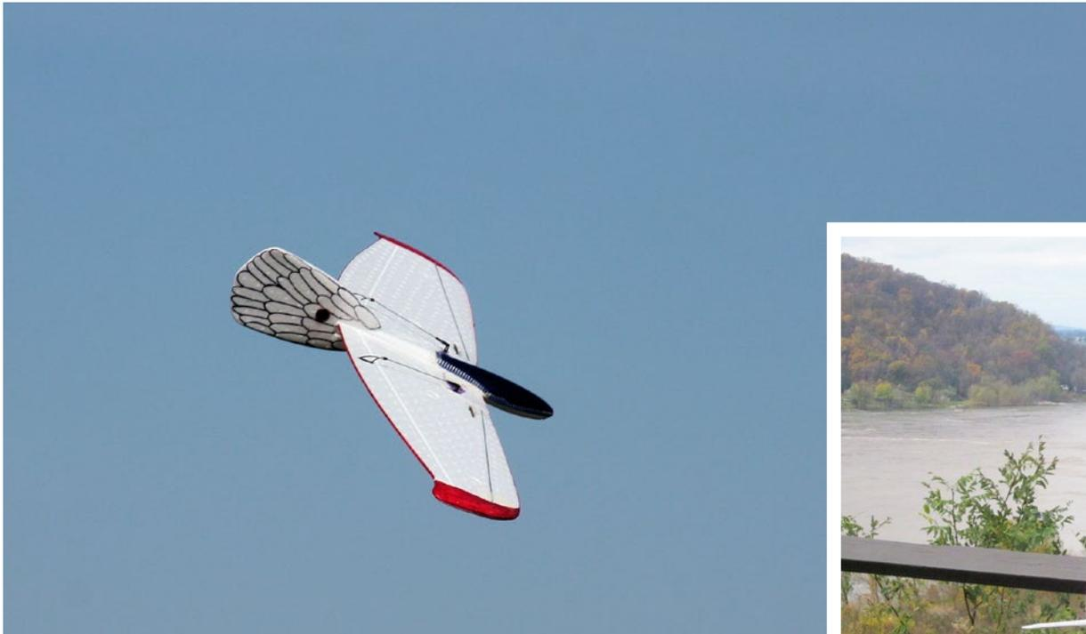
*Left: During inverted flight testing, OFB Joe Chovan found he liked the CG further back. The dark circle on the fin is a taped on quarter.*
