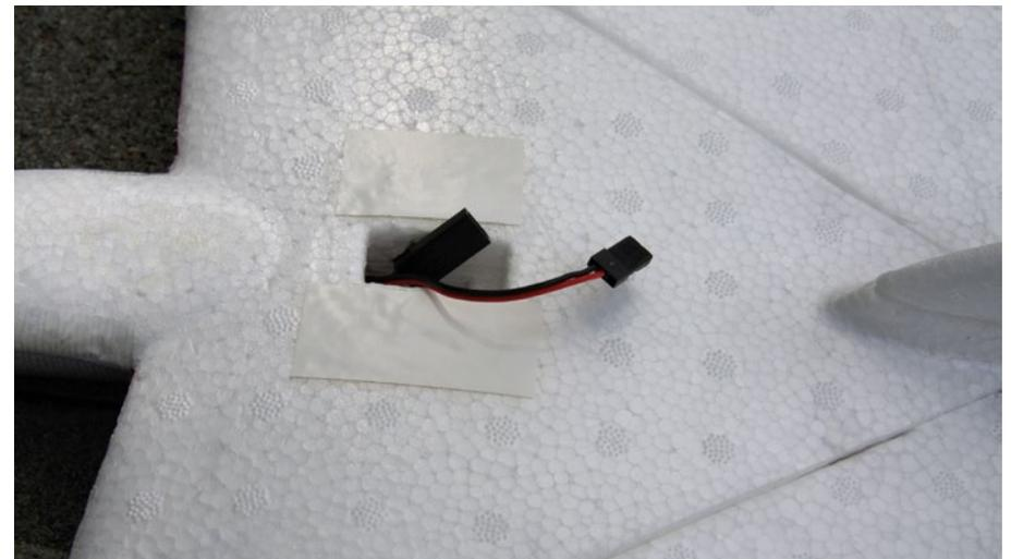
*Dave’s plug/unplug on/off switch at top side of the model. Additional openings filled with epoxy mixed with microballoons and/or covered with white tape.*
