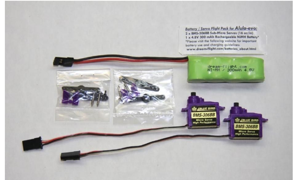
*Factory recommended on-board components for Alula Evo includes two Blue Bird BMS-306BB sub-micro servos, and a 4.8V 300mAh NiMH battery pack.*
