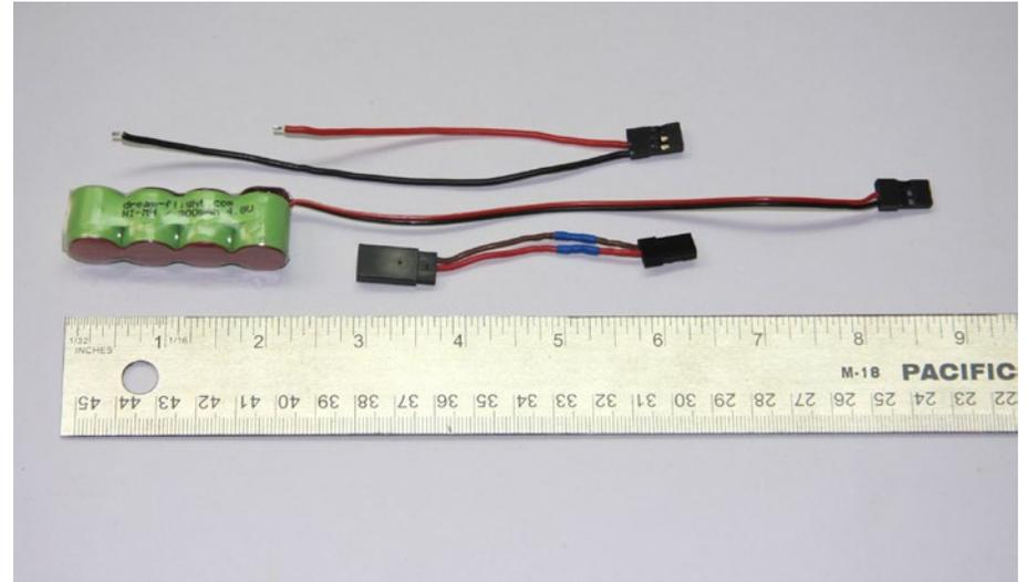
*Dave’s modification to battery pack lead to allow plug/unplug on/off switch at upper side of the model, rather than making a hole in the belly pan.*
