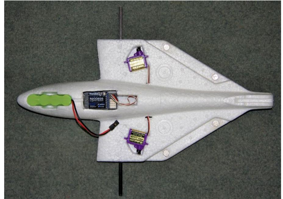
*Antenna tubes for dual 2.4 antennas, view from underside.*
