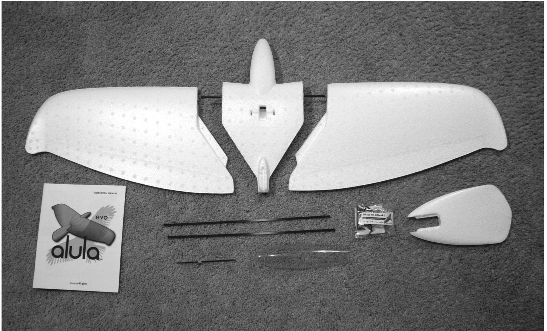
*Kit contents include molded fuselage, wings and fin. Also carbon spars, carbon pushrods, a molded clear belly skid, small parts bundle and the best instruction manual in the model airplane industry.*
