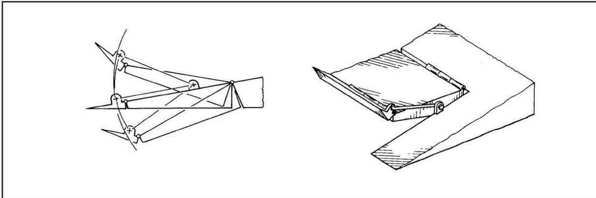
*The Kasper trim device geometry forces the tab portion of the control surface upward any time the control surface is not in its neutral position*
