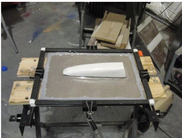
◀ Put the mold on the table, turn on the vacuum and quickly take the part from heating source (gotta be quick on cold days) and pull it down over the mold and onto the silicone seal.
