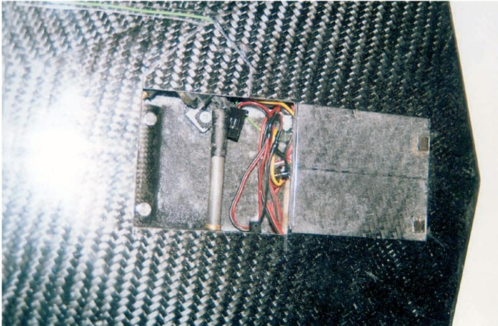
*Center section compartment and bayonet wing panel assembly.*
