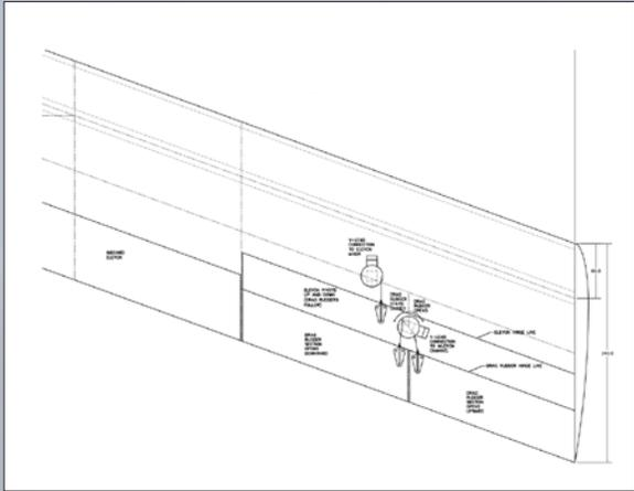
**Front cover:** A combination drag brake and elevon control system designed by Ken Stewart. A detailed description of this mechanism begins on page 38 of this issue.
