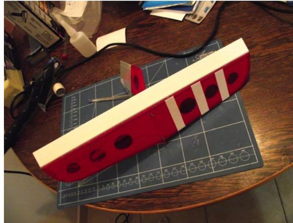
*Bottom of the tail group, two mounting bolts on the stab centerline.*
