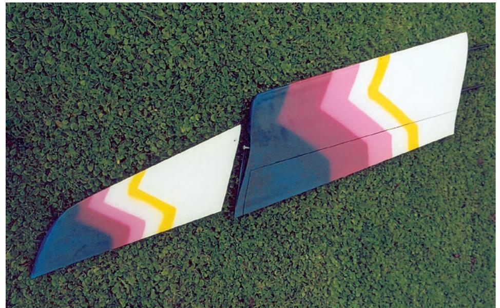
In fact, the operation of the winglets is much more complex than I have just described simplistically. In fact the not negligible increase of efficiency is also due to the fact that they change the distribution of lift increasing it at the ends.
