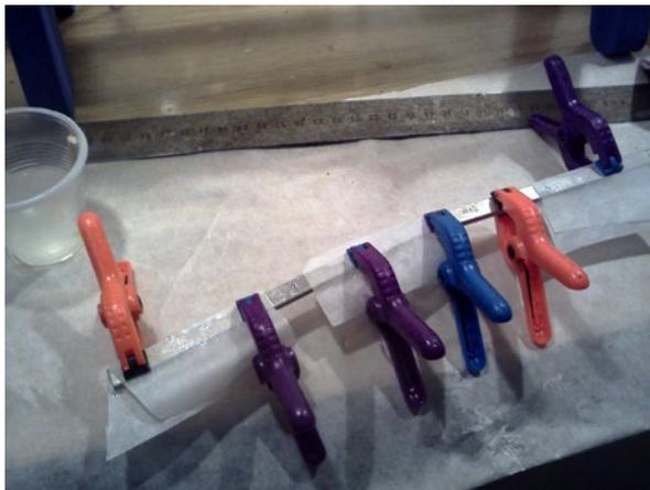
*Gluing the metal spar pieces together.*
