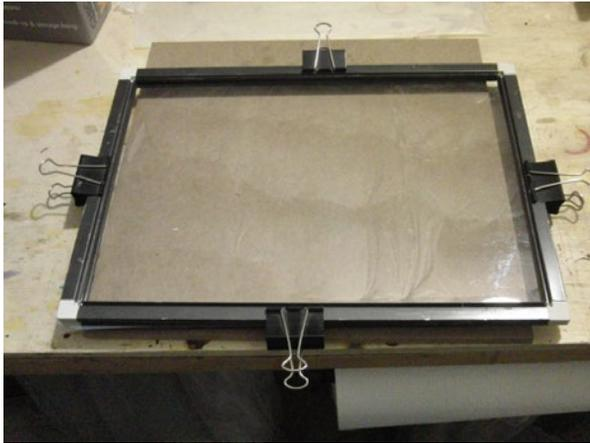
◀ Use clips to hold the plastic in the frame. You can get various thicknesses and types of plastic in rolls, or cut to size from Piedmont Plastics or your local supplier. I get both styrene (white or colors) and clear PET for most projects.
