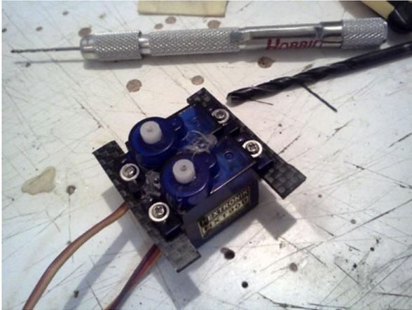
*Servos mounted on carbon fiber rails.*
