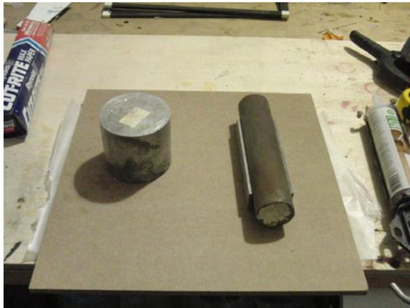
◀ Place a piece of wax paper on and put a weighted board on top. I let it set for 3 hours, then take the board and wax paper off and put it in the oven for one hour at 180 degrees. Or you can just let it set for 24 hours or until fully cured.
