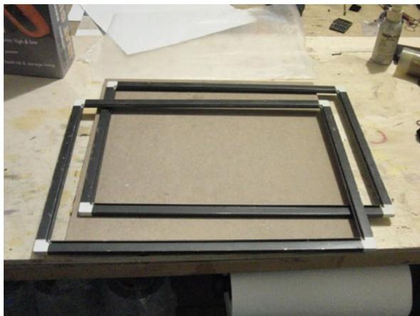
◀ Take and make a simple (2-piece) frame from metal screen frame parts from hardware store. You can make one out of wood or whatever, but I found this really simple. I made it 1/2" larger than the board, so I don't have to be as precise when placing it on the table.
