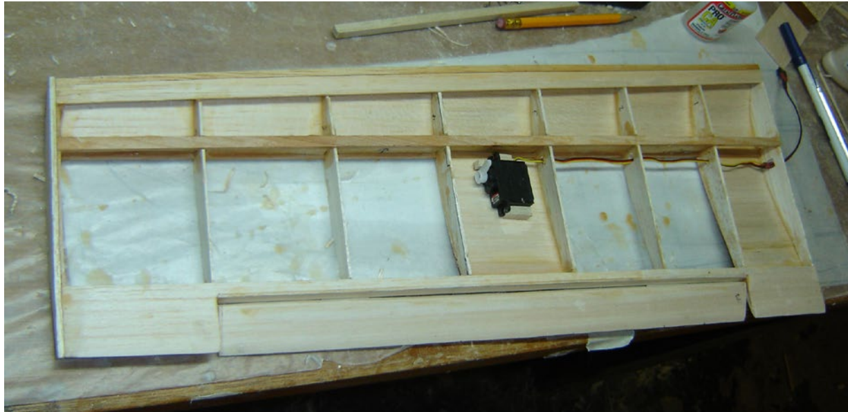
This is the outer wing panel of the Hitec. Wiring and a 3-pin Deans plug are connected to the servo. The inboard rib bay is covered in 1/16th balsa and excess wiring can be pushed into the resulting cavity when the entire wing is assembled.
