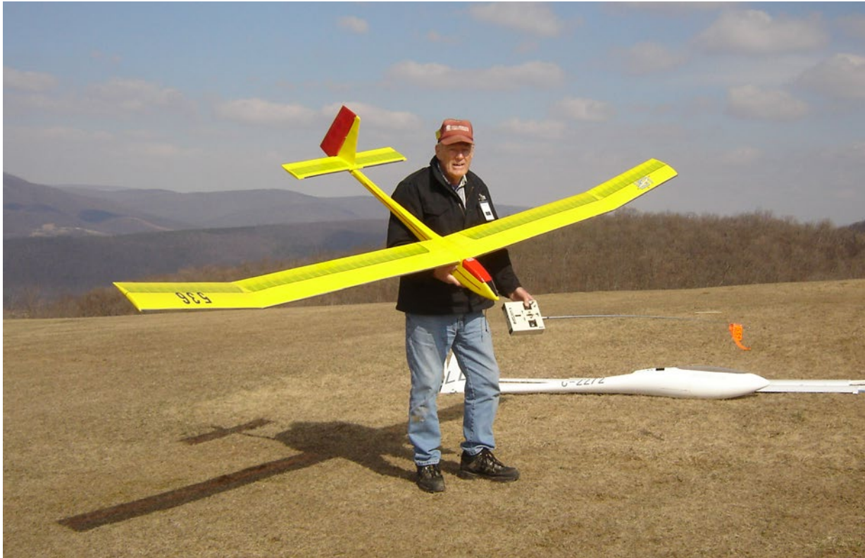
This is the author with his 12 foot span Thermal Queen 3-channel sailplane. The transmitter is a very old Proline operating on 53.3 MHz in the 6-meter Amateur radio band. The ship was constructed from a Skybench Aerotech short kit.
