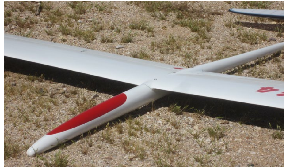
Ignore the "i4" moniker stenciled on the wing; this is the Royale. Opposite: Note the large flaps, here deflected about 80 degrees.
