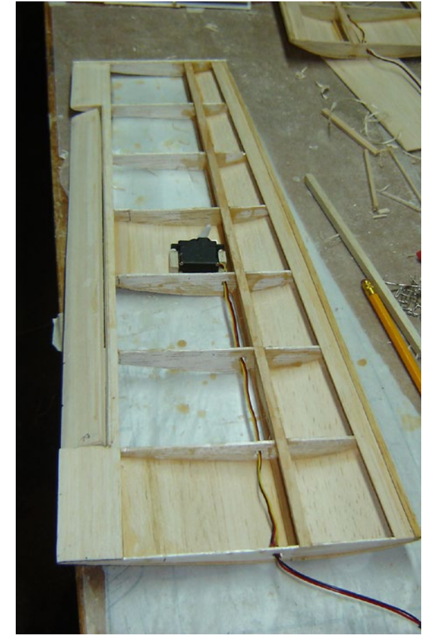
HS-82 MG servos are used on the ailerons. The setup of the servo arm was to give differential throw with much more up than down deflection. The servo is securely mounted to the top sheeting.
