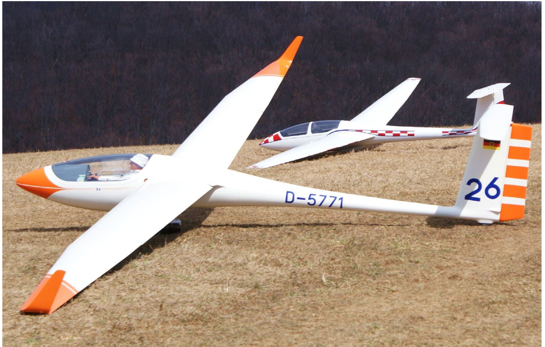
This Let Models ASH-26 spans 6 meters and was both a fantastic performer and quite aerobatic during Friday's heavy slope lift. It sports a huge solid carbon wing rod. Owned by Steve Pasierb of Connecticut, custom paint and graphics by Alvaro Corzo. Photo by Steve Pasierb
