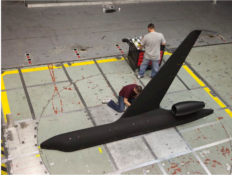
A semi-span jet model is scheduled to be tested in NASA Langley's 14-by-22 Foot Subsonic Wind Tunnel this winter to evaluate aircraft noise reduction technologies as part of the Flap and Landing Gear Noise Reduction Flight Experiment. Image credit: NASA Langley/Sean Smith
