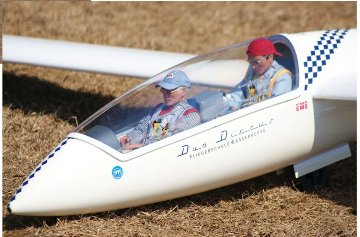
The front office of Steve Pasierb's stunning EMS Duo Discus. This 5.3 meter span sailplane has obechi wood sheeted over foam wings that were then glassed and painted with a custom harlequin design. Two Axel's Scale Pilots do duty at the controls inside a highly-detailed cockpit. Photo by Steve Pasierb
