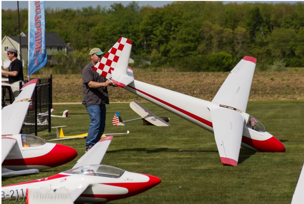
The 50% KA6 from Bill Hempel's Team Edge has become a popular giant scale choice around the world. Spanning 259 inches and weighing anywhere from 45-50 pounds, assembly is actually quite easy with obviously no fussy small parts to handle. Photo by Jeff Duhaime
