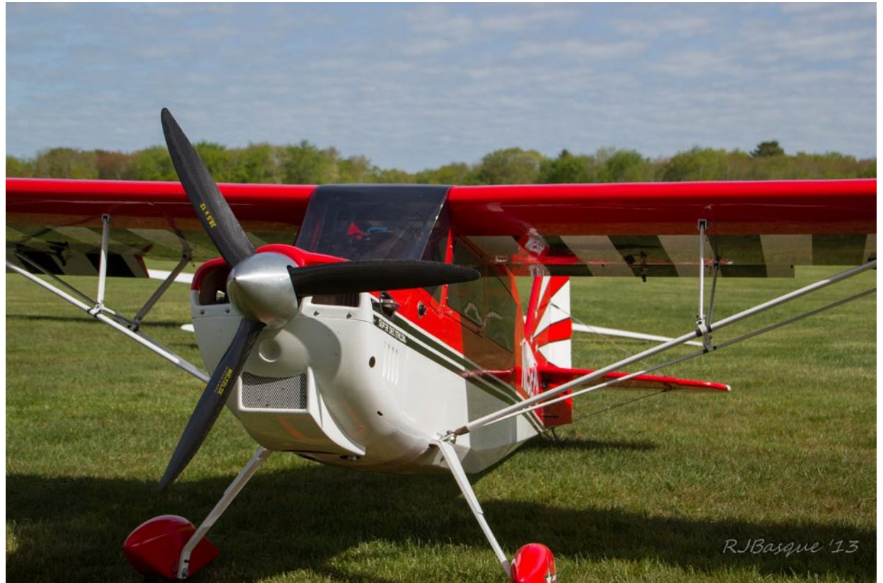
The business end of the 38% Hempel Decathlon tow plane. The huge cowl swallows up a Desert Aircraft DA170 motor with only the sparkplugs extending outward ever so slightly. The Hempel version and new Hangar 9 Decathlon are proving to be popular towing choices. Photo by R. J. Basque
