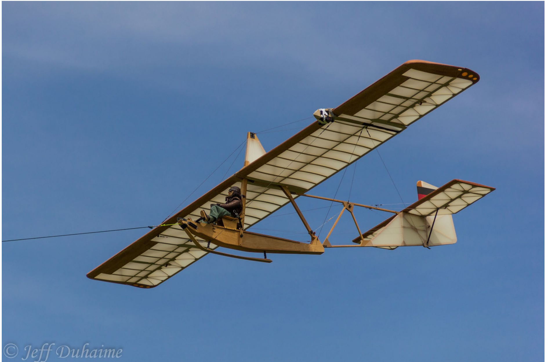
Erich Schlitzkus did a masterful job detailing his SG 38 and rigging a web of proper flying wires to support the structure. It is not quick to assemble at the field, but the work is richly rewarded. Photo by Jeff Duhaime
