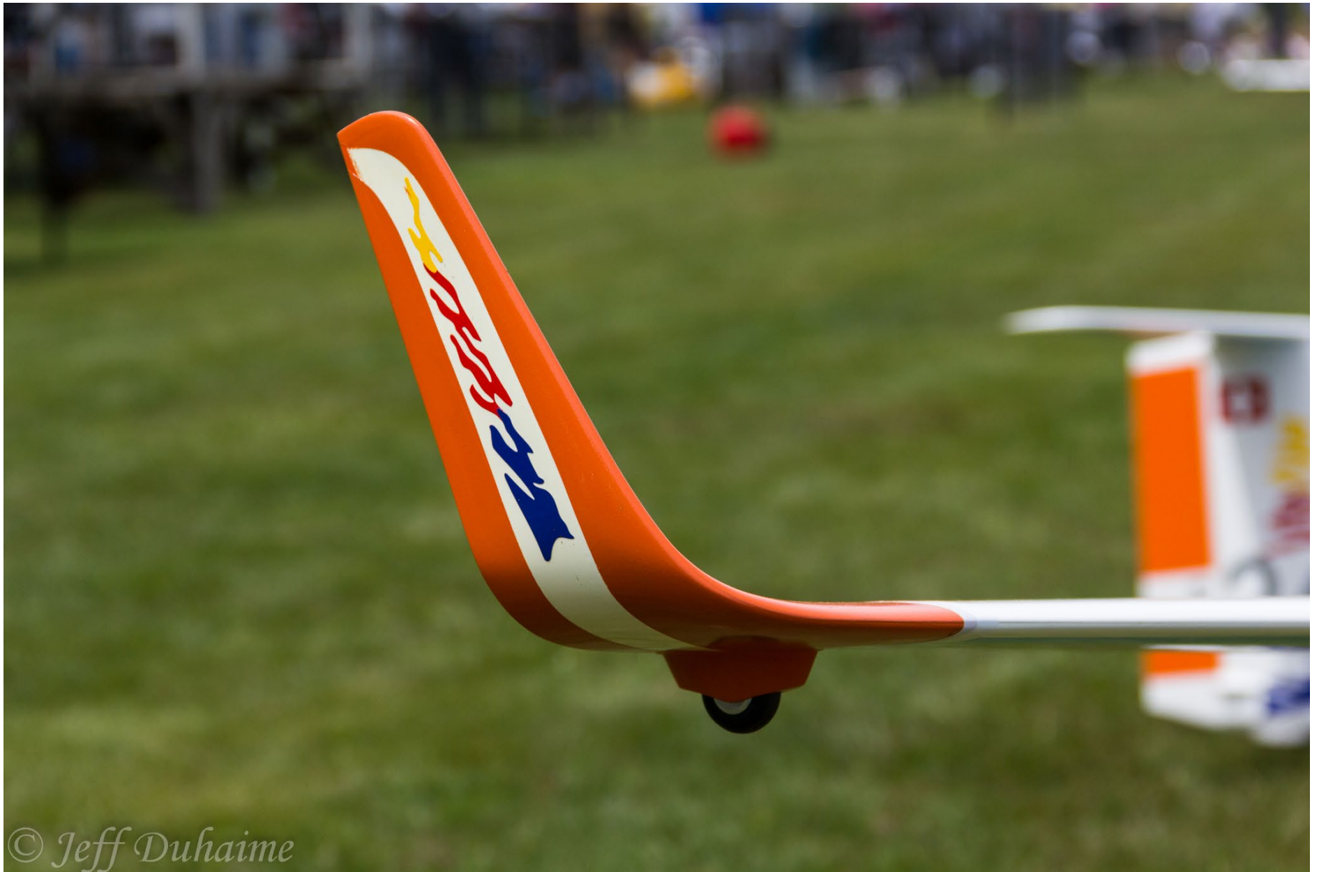
Don Chamberlain's ASH26 blends exterior schemes with the factory swirl artwork and a strong dose of anti-collision orange. Note the tip wheel for asphalt runways. Photo by Jeff Duhaime
