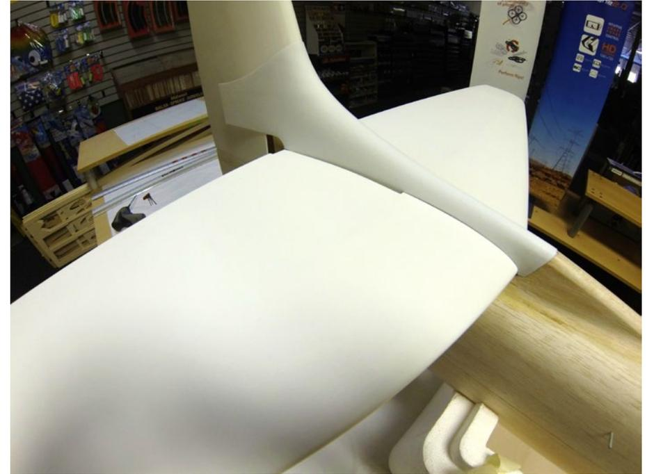
*Left: The balsa master plug for the tail fairing sits behind the finished vacuum-formed finished product of 0.060" styrene. Right: The formed fairing in place, held by magnets at the front and fasteners on the vertical fin. The size of the fairing required a 12 inch by 24 inch sheet of plastic, so a new vacuum box had to be constructed to form the part.*
