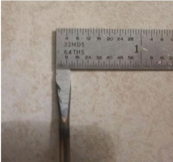
14. Now I needed a way to put the clevis back on. I flattened the other end to about 3/16".
