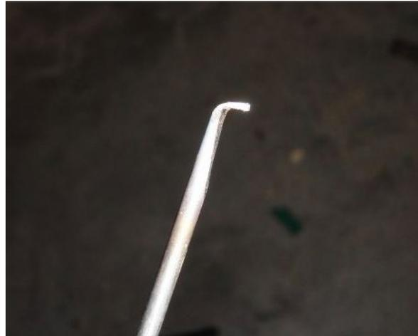
15. Bent it about 80 degrees. You can bend it up to 90, but the edge of my vise was a bit rounded. It actually turned out easier to remove, after installing the clevis, with less than a 90 degree bend.
