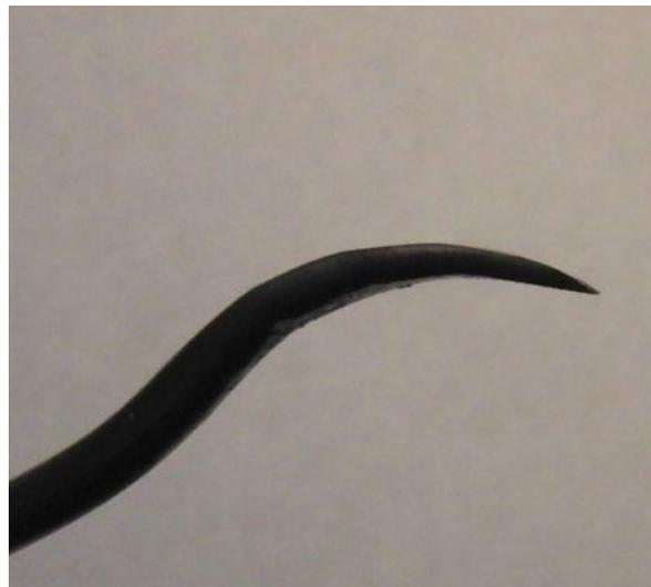
A final note: There's one last thing. Sharpen the end of the pry bar so it can more easily slide under the clevis.
