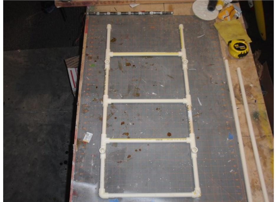
I assembled the whole unit and then used thin CA to keep it all together. See Photo 3.
