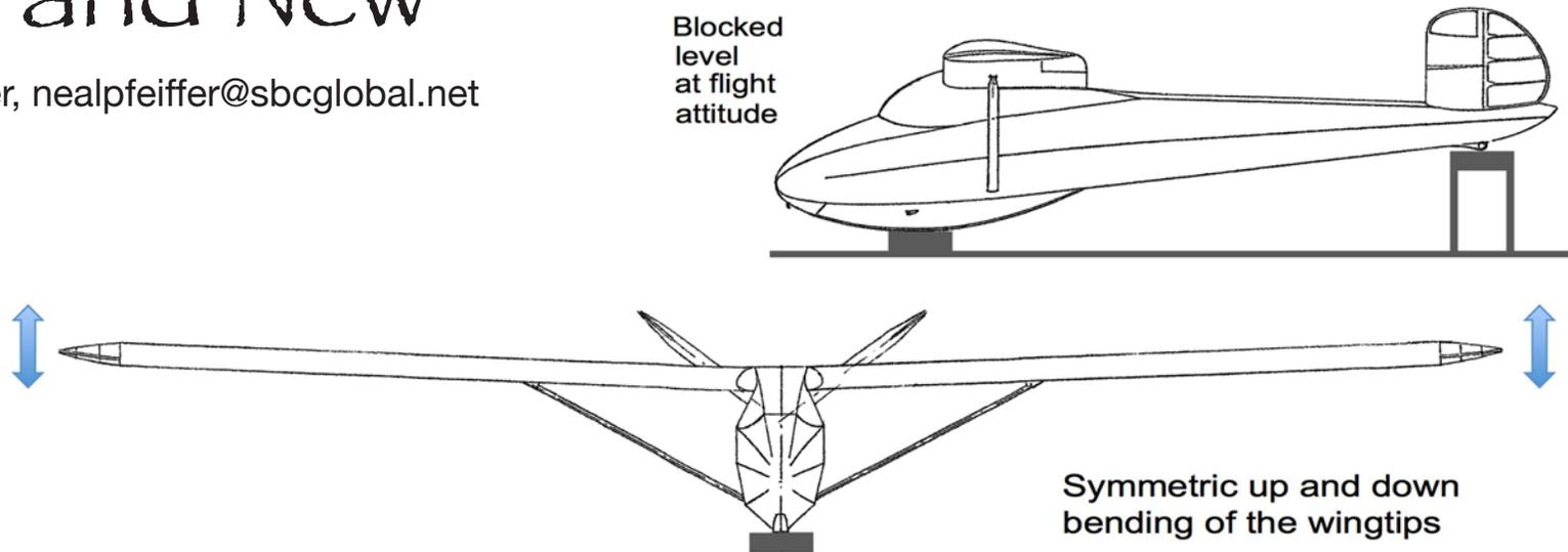
The inspection sheet used for gliders in Germany includes an interesting item, the oscillation frequency for wing bending. For inspection sheets in the original German, it is identified as “Flügelbiege – Schwingungszahl”, and in sheets written in English, it is called the “Wing warping rate of oscillation.” In either case, the value is defined by some number of oscillations per minute.
