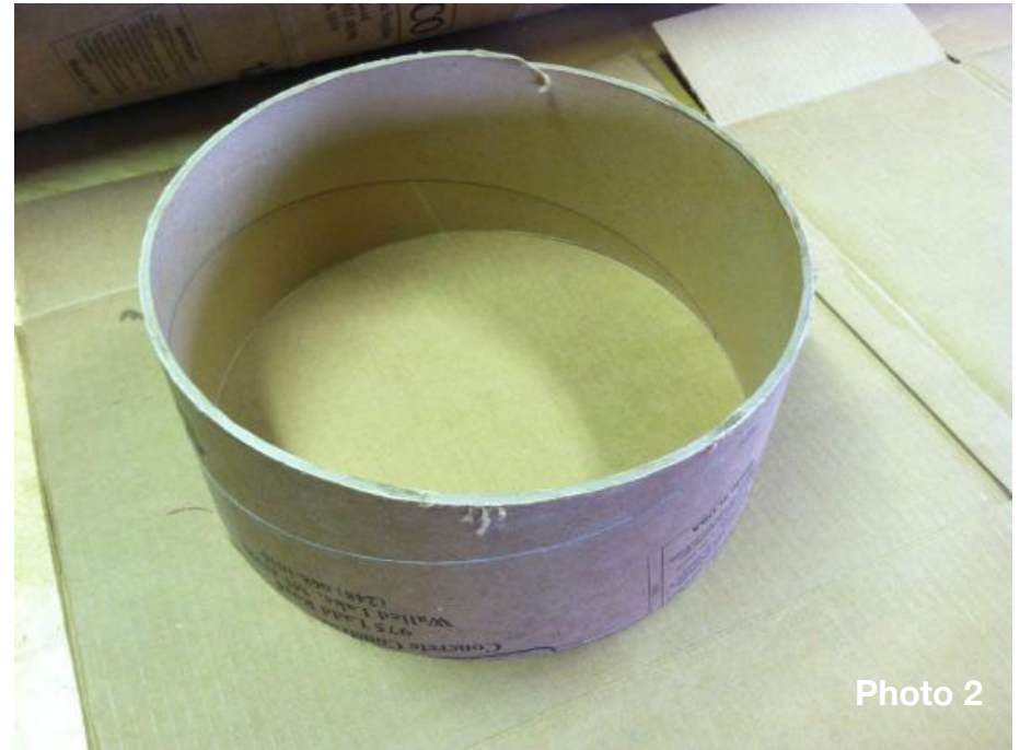
Template for cutting bulkheads and ends.
