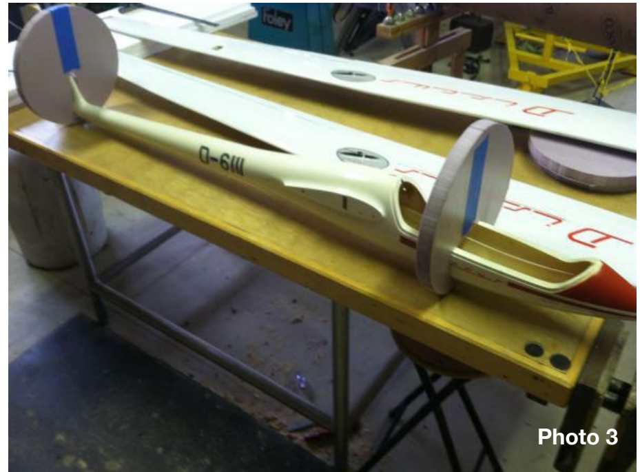
The bulkheads on the fuselage and laying out the location for the wing.
