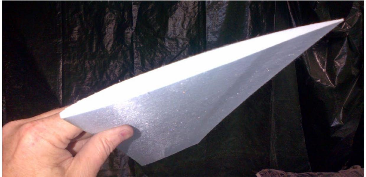
*The wing core showing the thin section used.*
