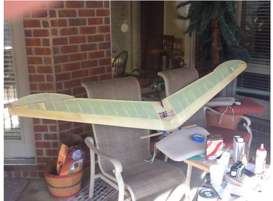
*Right: Center section closed out. The square patch? A moment of carelessness before it was covered. I flipped the wing over on the work bench and a tube of Titebond punched a hole in the "D" box... Arrrrgh! It gets a folding prop later.*
