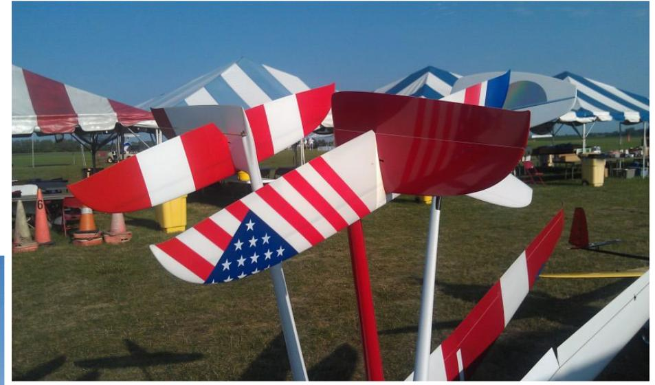
*On the field, the Multi-Stand can be configured for either conventional tails or V-tails by turning around one side panel. The cant angle can be adjusted by making shorter and/or longer stretcher bars in the shop. Might be nice to have a couple of lengths made up ahead of time.*
