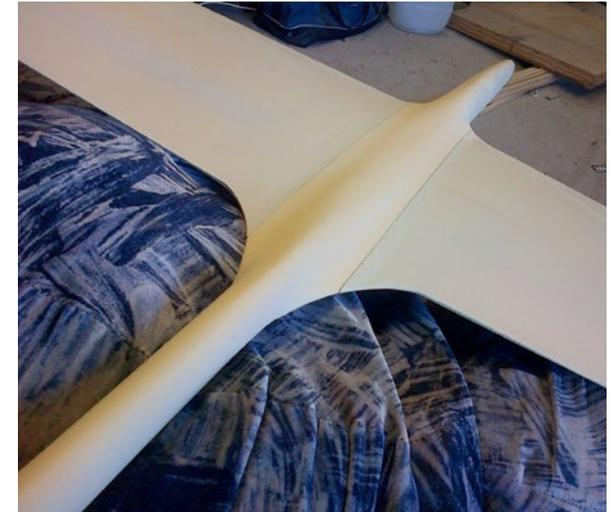
▲▼ *Fairings provide for a very smooth wing-fuselage junction*
