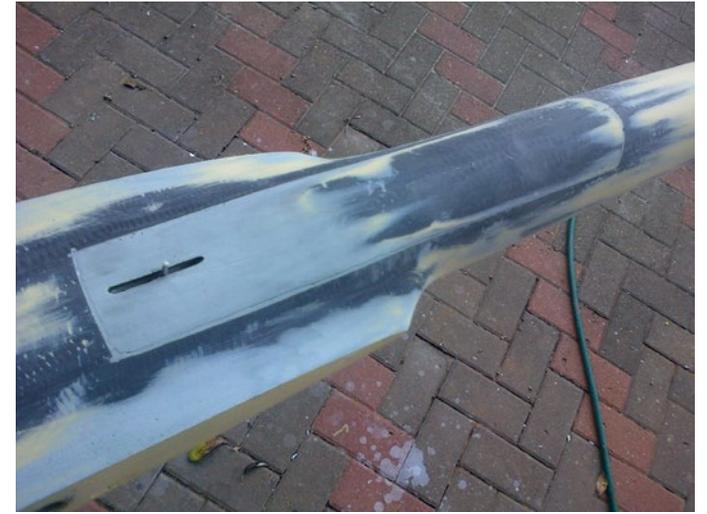
▲ *Fuselage access hatch*
