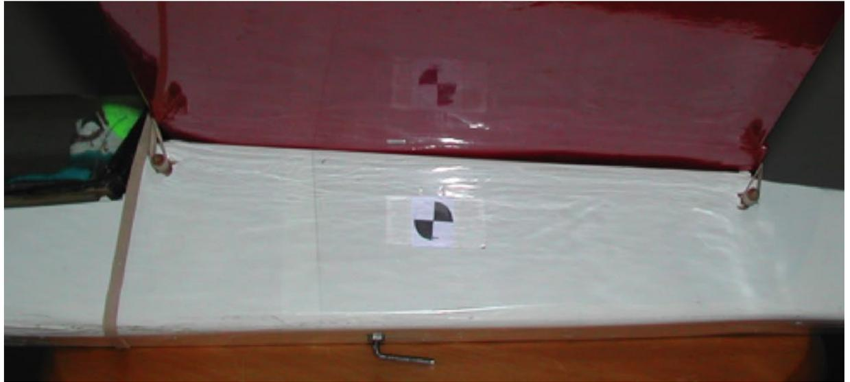
*This Sophisticated Lady was made 5 ounces lighter by using a pair of CGAs. The natural CG of this plane without CGAs is 1.5 inch aft.*
