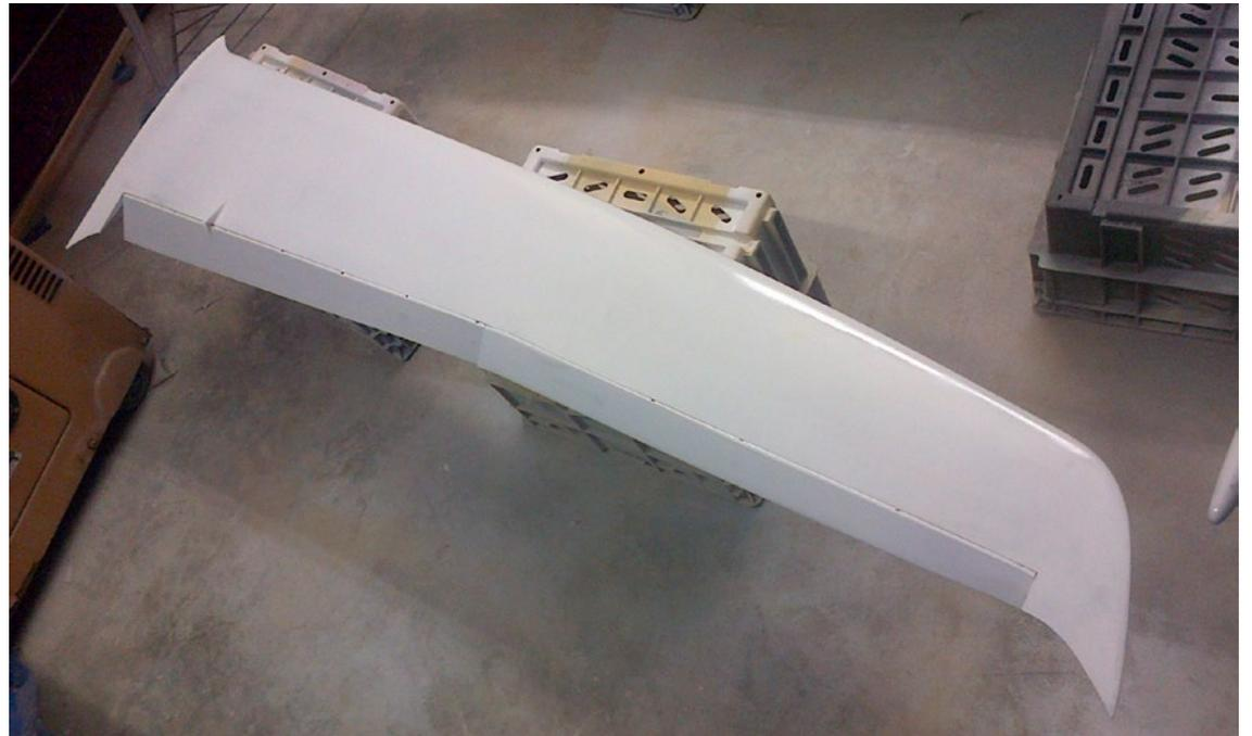
Glass the concave hinge areas with 49g/m<sup>2</sup> cloth. This helps as a sub spar and anchors the hinge pins. Give it a light sanding when cured.
