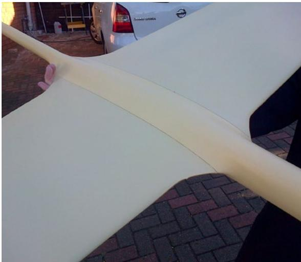
▲► *Fairings provide for a very smooth wing-fuselage junction*
