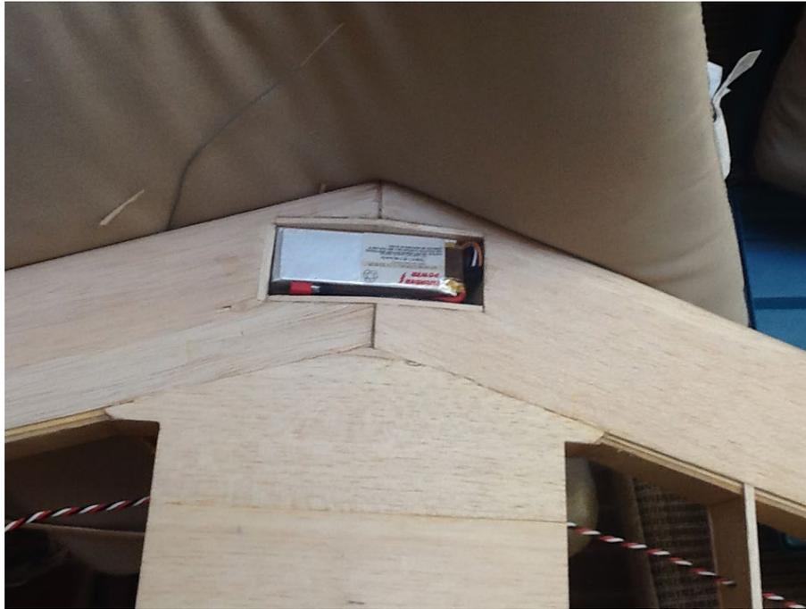
*Above: Battery box on the lower skin.. 2100mah... Overkill but we had the batteries on hand and it needed the weight.*
