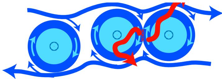
*Figure 7. Unevenness in shearing flows can create vortices of similar rotation. When close together they conflict, creating either turbulence (shown) or vortices of opposite rotation.*
