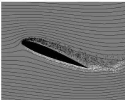
T = 3.50: Upper boundary layer is beginning reverse -- it is turning white, indicated by counter-clockwise turbulence elements.
