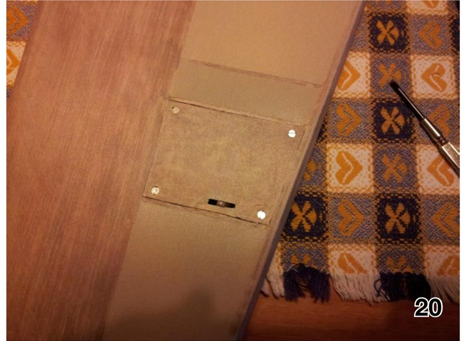
you can have a torque of 4 or 5 kg-cm in very little servos, hence I moved the position of the servo to in front of the aileron, between two ribs where balsa coverings were already foreseen on both upper and lower airfoil surface. (pic 20)
