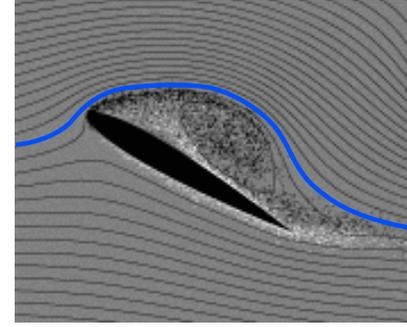
T = 9.00: A new clockwise vortex has formed. Streamlines are still exiting downwards, indicating mid lift pulse. The cycle of lift pulses will repeat until angle of attack is lowered.
