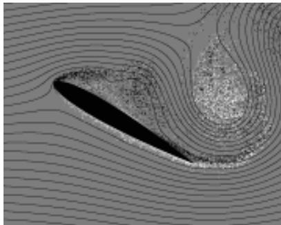
T = 7.75: Bubble reattachment. The shedding CCW vortex is still disrupting lift.
