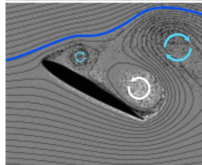
T = 7.00: Clockwise vortex shedding. Streamlines are no longer curved downwards, indicating loss of lift. A new CW vortex is forming at the leading edge.
