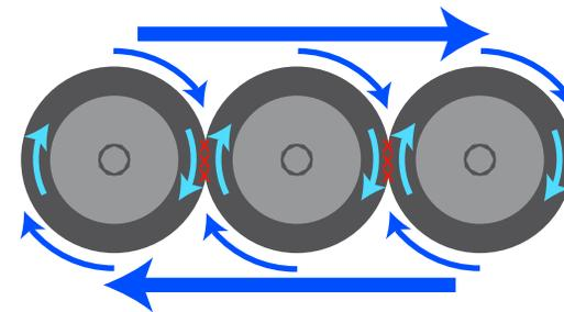
*Figure 8: When vortices of similar rotation come close to each other they conflict, like oversize tires on an eighteen wheeler. Trivia nerd tidbit: The historical concept of a 'vortex sheet' was a falsity. As illustrated by the truck tires, any such arrangement of vortices would have torn itself apart.*
