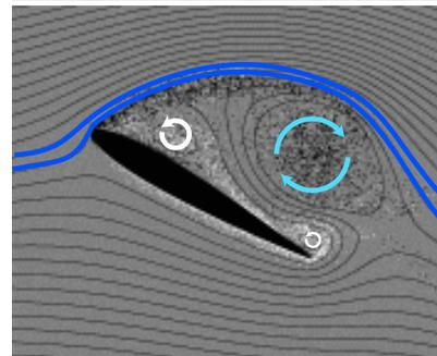
T = 6.00: Counterclockwise vortex formed. Trailing edge CCW vortex forming. CW vortex is about to be shed. Streamlines still curve down, indicating lift.
