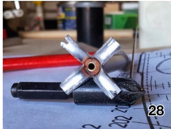
glued the brass tube inside the beech rod and then inside the aluminum tube that I drilled in order to put the steel rod transverse.
