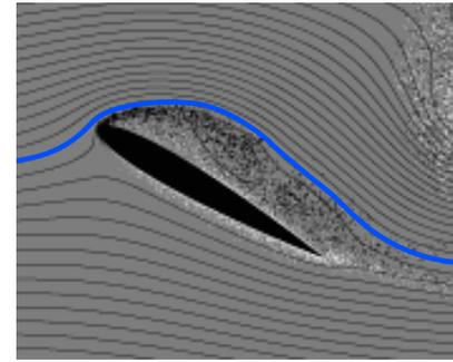
T = 8.50: The CCW vortex is far enough into wake so that streamlines over the wing again exit downward, indicating a new pulse of lift.
