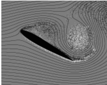
T = 7.50: The CCW vortex is being shed. Streamlines show loss of lift.
