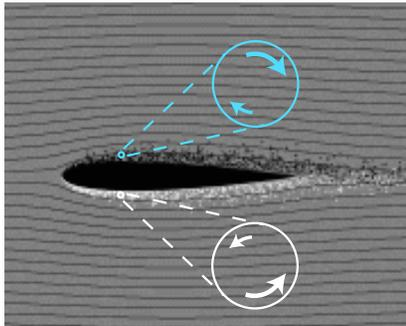
T = 1.00: Dr. Dommelen writes, "In the simulation, the boundary layer is represented as vortices (miniature tornadoes, which are displayed as black or white dots, depending on direction of rotation.)" Real turbulence is more chaotic.
