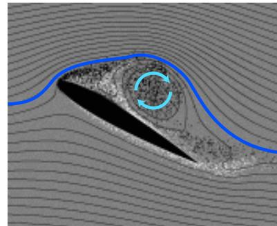
T = 5.00: Clockwise vortex formed. Counterclockwise vortex forming. Even with a CW vortex formed, upper streamlines still curve down, indicating lift, though with high drag.
