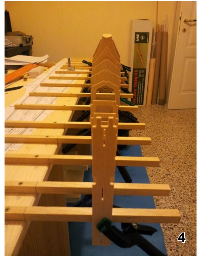
Then, I started the fuselage by conveniently fixing all the bulkheads on a flat building board through obeche strip (pic 03 and 04). Once aligned at right height and distance, I glued the four fuselage spars that run through all its length. (pic 05)
