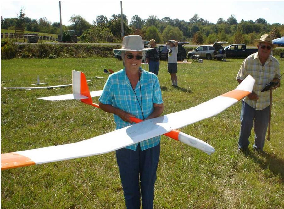
fuselage given to me by Roy Simpson at the 2000 Nats. It was a very clean fuselage with a very heavy molded fin. I cut off the fin and substituted a balsa fin from my Aurora cutting over two ounces from the tail. The second change was to switch to the more fashionable Schumann wing planform
