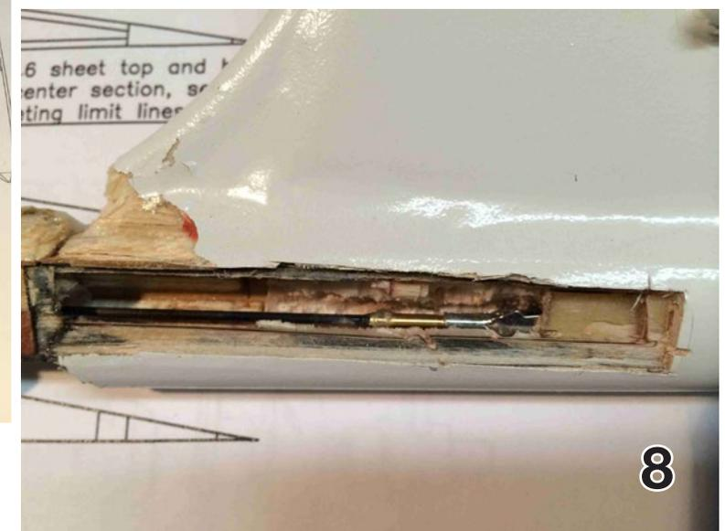
bit of twirling of the left hand in a tight spot, I was able to get the new rod screwed tight into the clevis which was already attached to the bellcrank.
