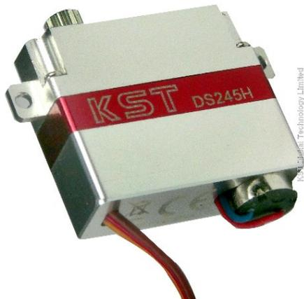
*The DS245H sports horizontal mounting tab positioning and a truncated case which partially exposes the 7mm diameter coreless motor. The DS245H shares the same gear train as the DS245MG and performance specifications are identical.*
