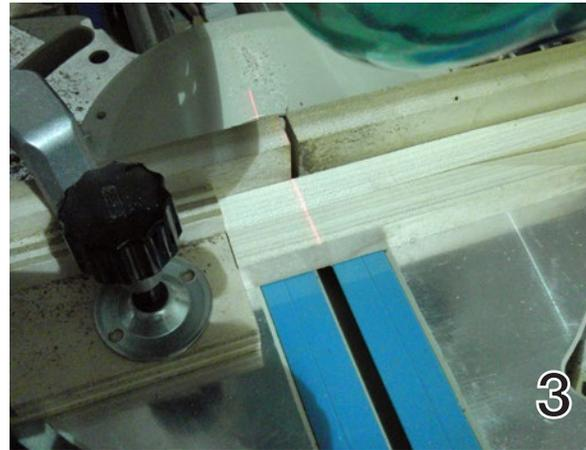
First cut the stock to length and cut jaw blocks. See Photos 2 and 3.
