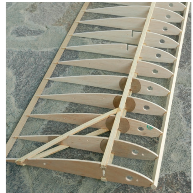
Photo 5: The left wing panel showing spar, ribs and spoiler bay cut-out.
