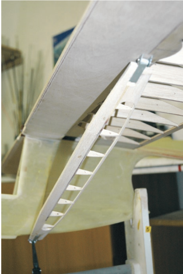
Photo 6: One of the ribbed struts.
