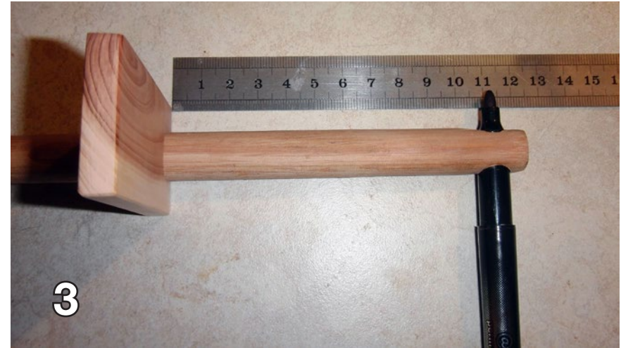
Photo 4 The block goes at the front of the wing at the root and the marker marks the spot.
