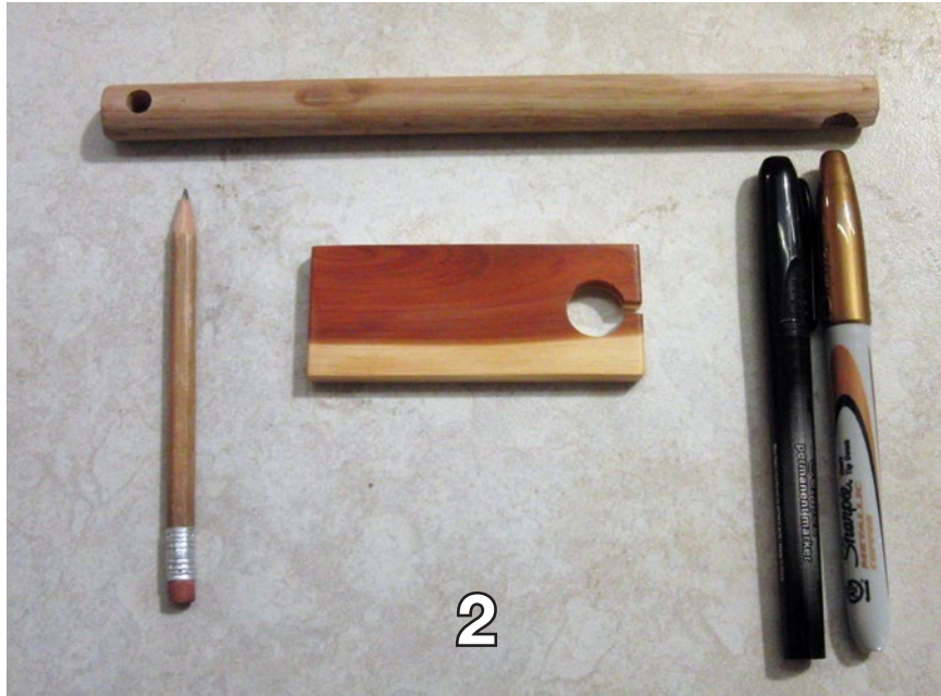
Photo 4 The block goes at the front of the wing at the root and the marker marks the spot.
