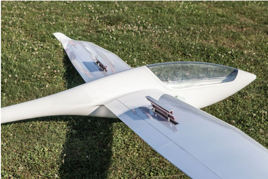
Spoilers 500mm from German manufacturer Schambeck < http://www.klaptriebwerk.de >.
