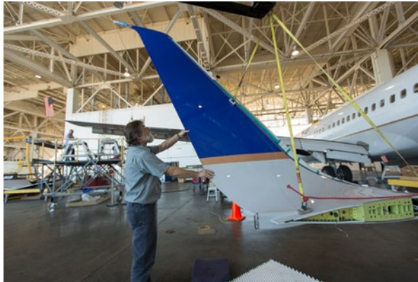
United technicians at Orlando International Airport install the new Split Scimitar Winglet on a Boeing 737-800.
