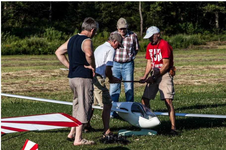
Checking center of gravity before first flight.
