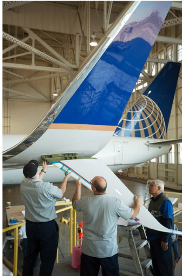
Retrofitting Blended Winglets to Split Scimitars involves adding strengthening spars, aerodynamic “scimitar tips,” and a large ventral strake.
