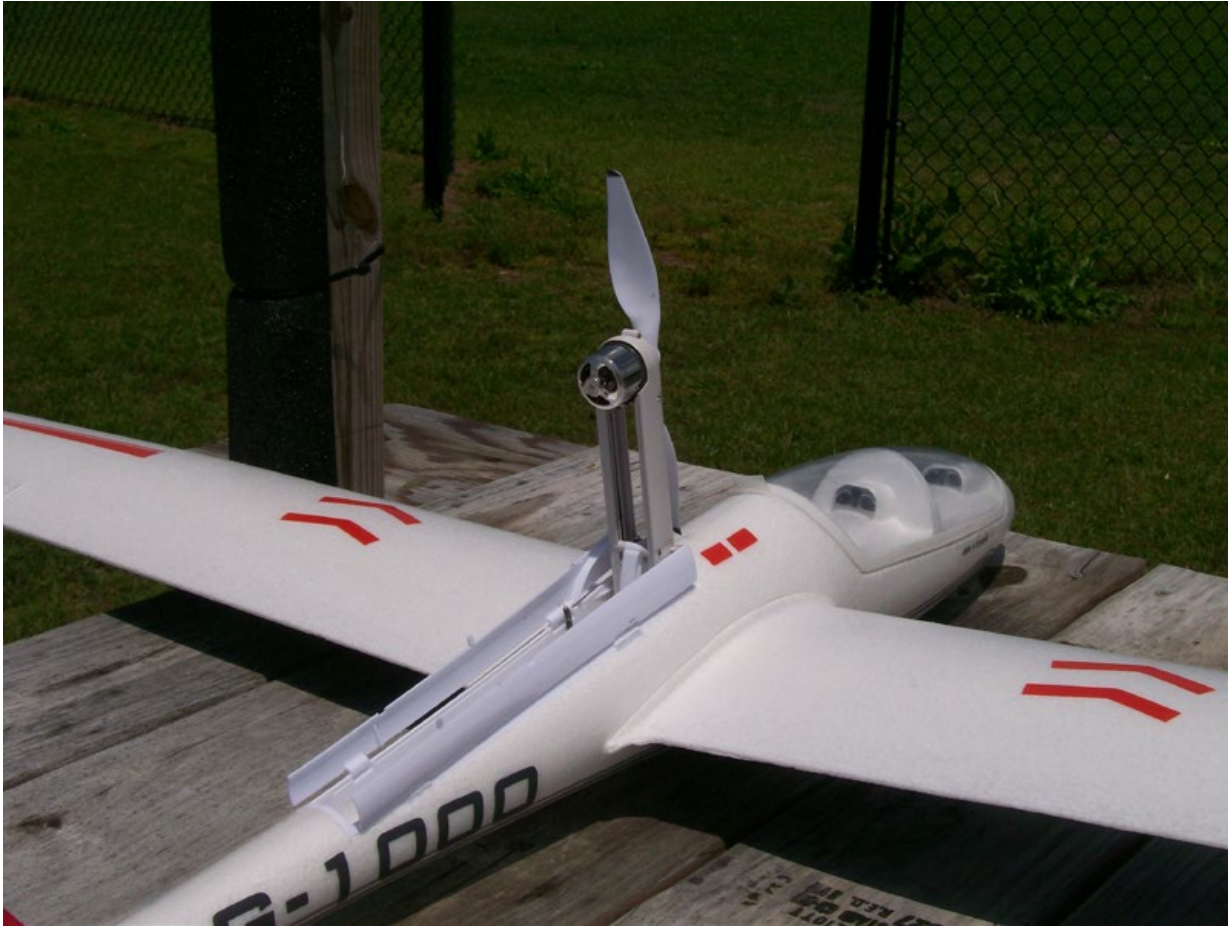
The clam-shell doors open, the RMS rotates upward and forward, and the motor starts. Reversing the procedure creates a clean rear fuselage and , making it more of a sailplane than a glider.
