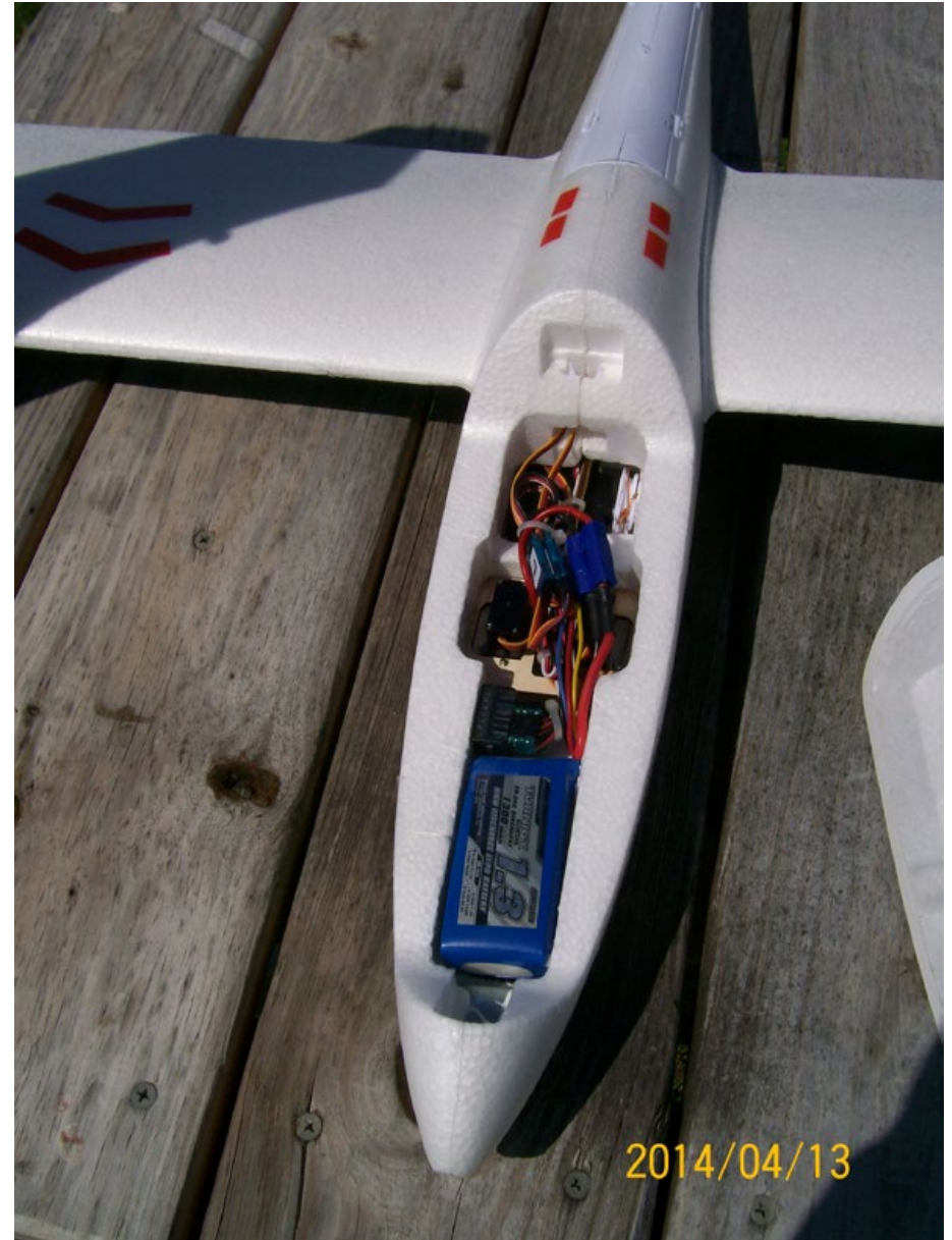
My 1300 mAh 3-cell LiPo battery fits perfectly in the molded battery space. You can see the clam-shell doors for the RMS at the wing trailing edge.
