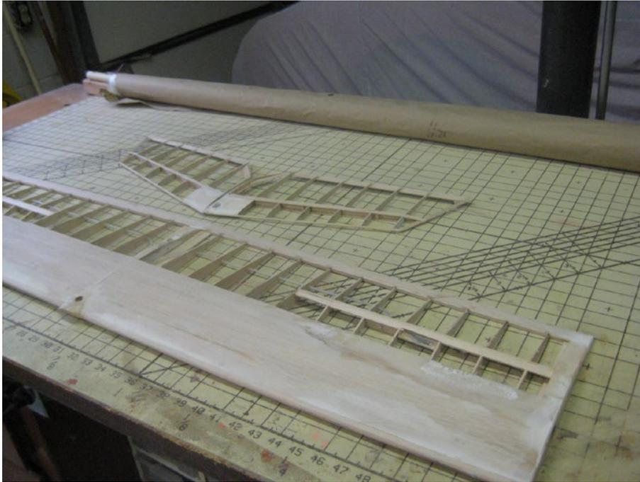
*Photo 5: The new center panel and stabilizer halves.*
