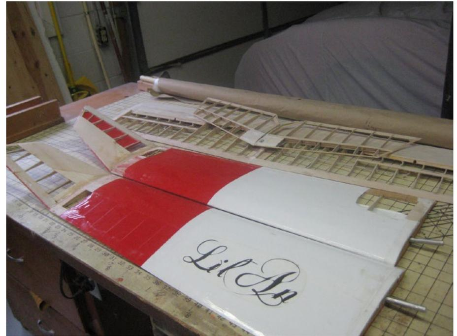
*Photo 10: Wing repaired complete, waiting for recovering.*
