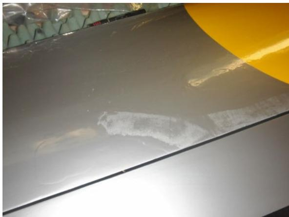
◀ The alcohol doesn't dissolve the adhesive, but releases it from the surface. Keep the towel wet and it goes fast. ▶
