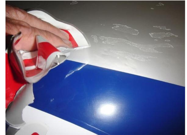
▶ For the small bits, I used the removed decal and just tapped and pulled the adhesive off. It's a very clean way to do it. ▶
