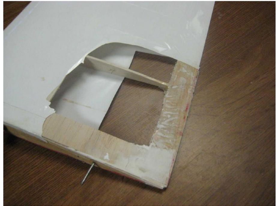
*Photo 8: Right wing panel root repair.*
