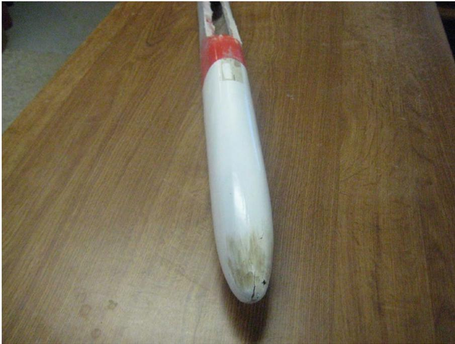
*Photo 7: Nose cone damage.*
