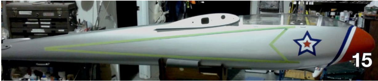
Photo 15: Next I used green painter's masking tape.
