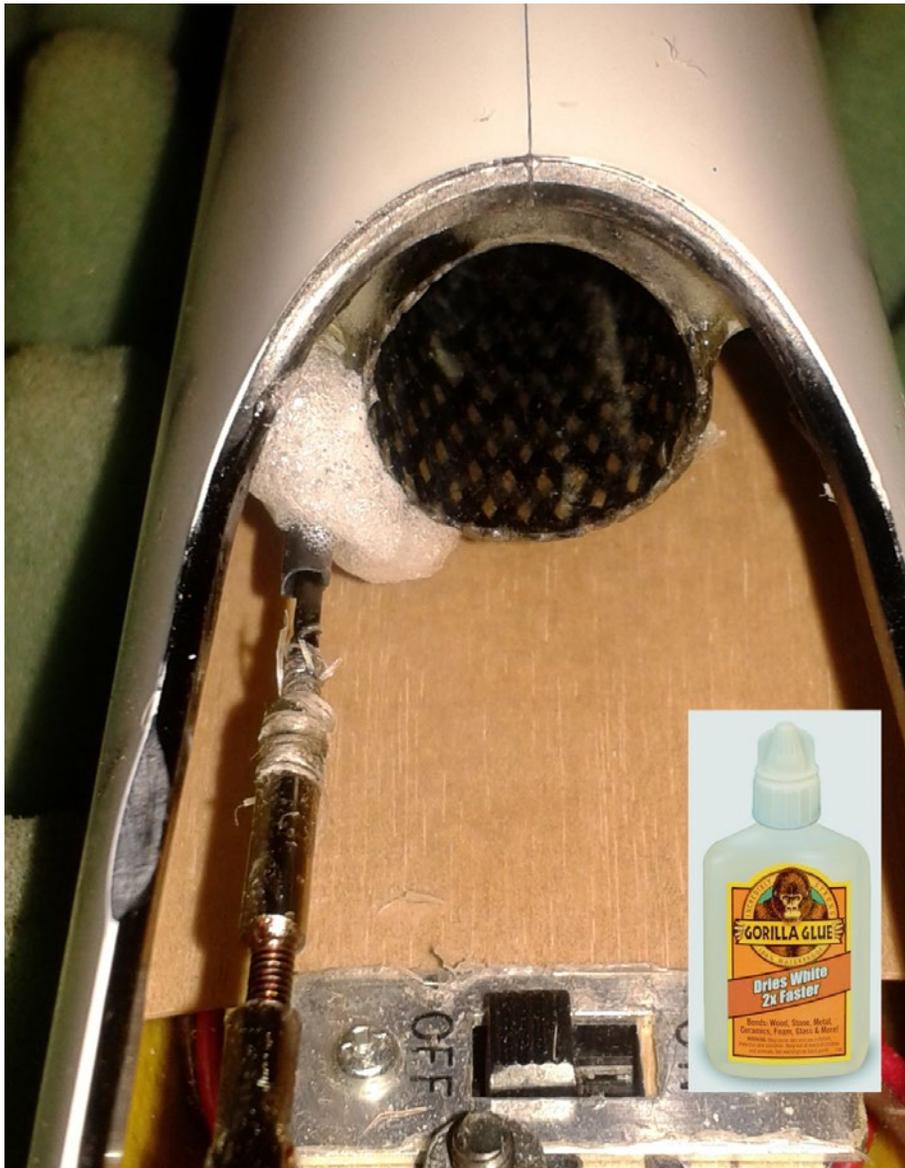
To glue those floating control rods, I use a couple of drops of Gorilla Glue White. Doing so keeps them straight instead of pushed over to the side.
