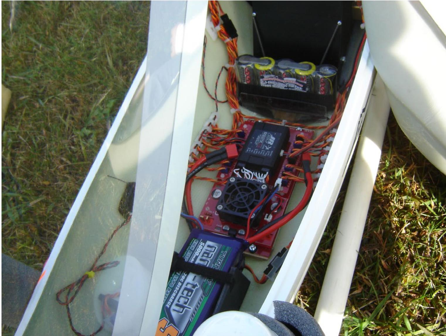
*This is the radio room of Steves sailplane. The radio is JR with satellite receivers installed to assure rock solid reception. The radio and servos are powered by the enormous LiPo batteries (2) that are mounted just*
