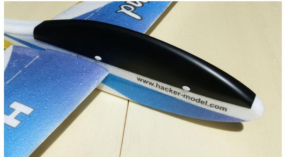
*The canopy is locked with four plastic clips. These clips are glued on the canopy to not loose them.*
