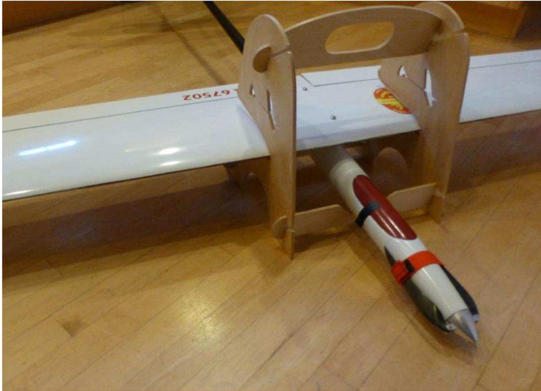
Jim Loughran used his CNC machine to cut ours out of 6mm plywood. I would think that cutting and sanding by hand using the Adobe plans (pdf) would work well, too.
