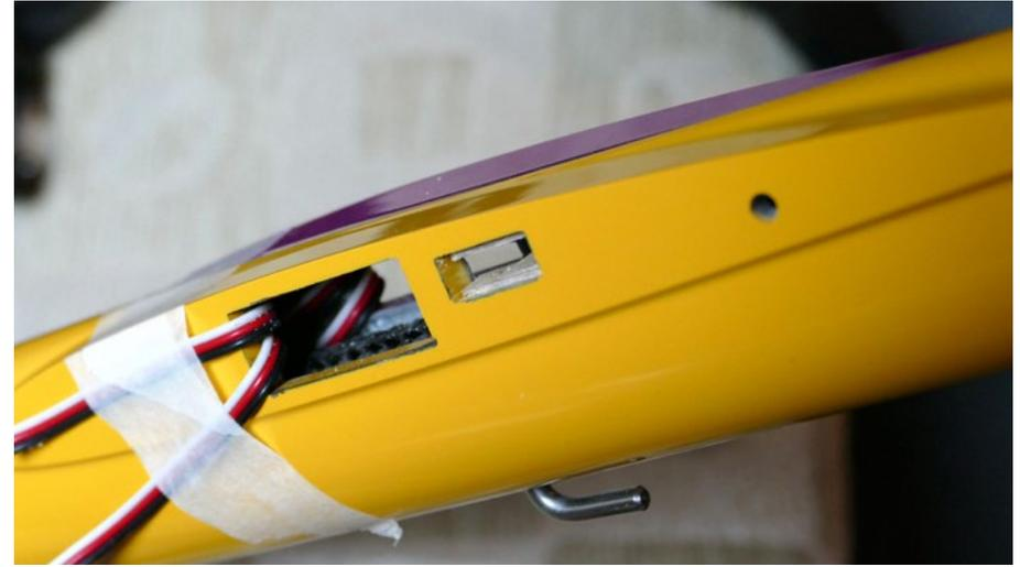
*The wire routing in the fuselage is tight and requires some attention. To strength the connector fixation, I built an upper and lower side to side tray with thin plywood*
