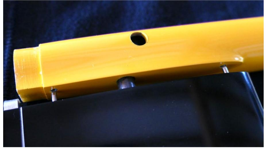
*Simple tail plane mounting without any tube, just holes in the fuselage, and where joiners are shifted.*
