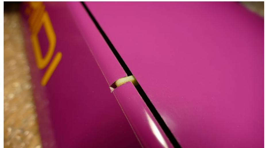
The control rod is fiberglass and totally integrated into the wing
