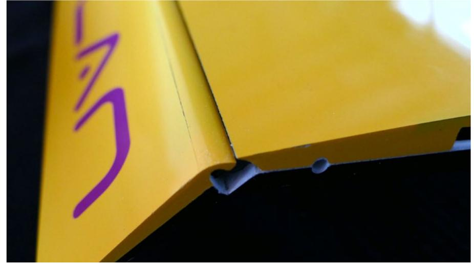
*Wipers are molded at the same time than the rest of the wing, which means that ailerons/flaps are position with an angle in the molds.*
